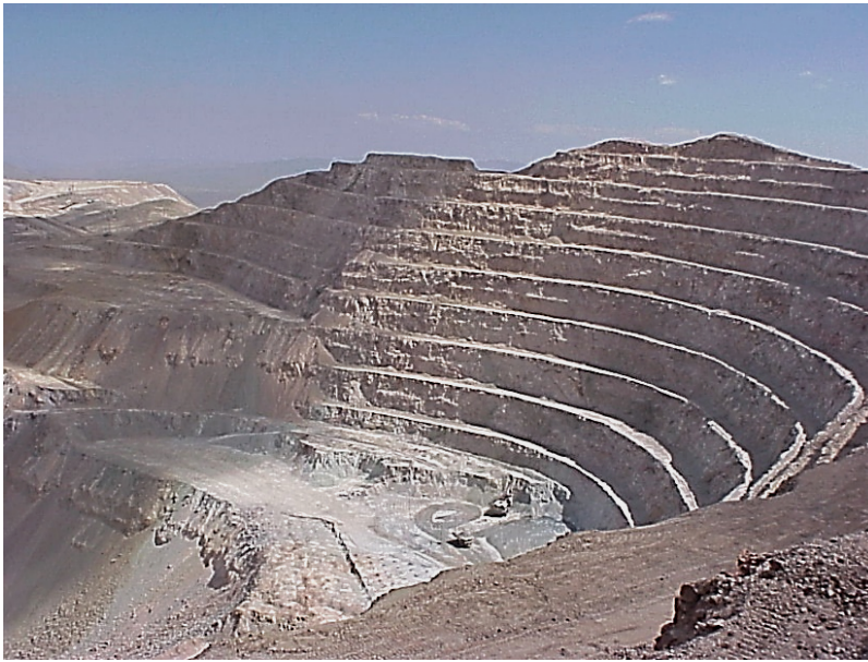
Figure 10: Benches created by pre-split blasting.
