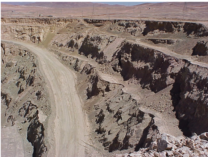
Figure 9: Bench faces created by normal production blasting.
