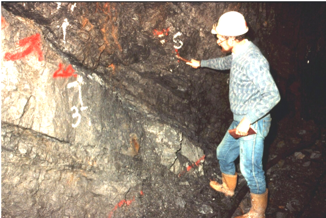
Figure 3: Sandstone and siltstone sequence exposed in and underground exploration adit. A thick bed of massive sandstone can be seen in the centre of the photograph and this is sandwiched between bedded sandstones and siltstones of moderate quality. The contact surfaces between these different beds are frequently heavily sheared.
