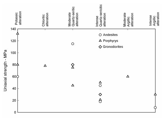
Figure 5: Relationship between intact rock strength and degree of alteration.
