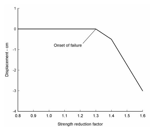
Figure 14: Plot of displacement of monitoring point in Figure 13 against factor of safety.
