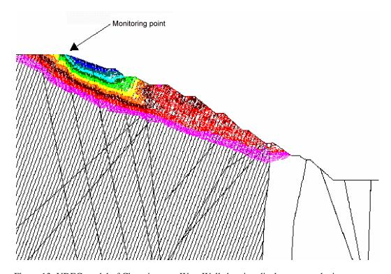
Figure 13: UDEC model of Chuquicamata West Wall showing displacement velocity contours.
