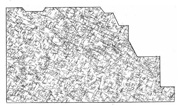
Figure 3: Joint map for the rock mass forming the foundation of the Three Gorges Dam in China.
