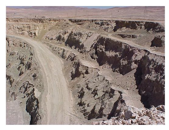
Figure 9: Bench faces created by normal production blasting.
