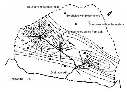
Figure 7: Extent of potential slide with layout of drainage gallery and drainholes drilled from underground. Contours indicate the drawdown of the groundwater levels achieved by the drainage programme.
