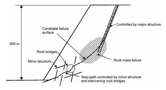
Figure 4: Candidate failure surface involving a number of different shear failure mechanisms.
