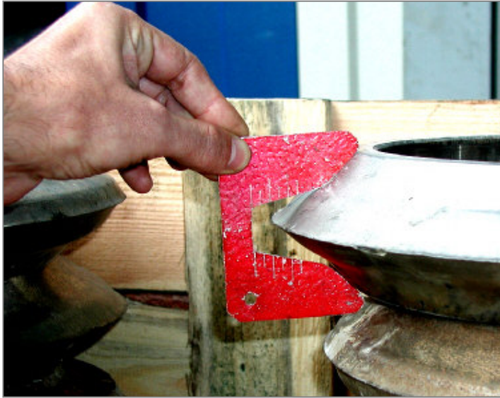
Figure 10: Typical wear of the disk cutter showing that the flanks of the disk are worn as quickly as the cutting surface.
