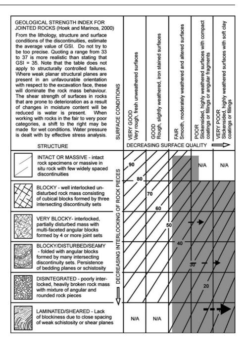
value for a typical rock mass. In all but the very simplest of cases, GSI is best described by assigning it a range of values. For analytical purposes this range may be defined by a normal distribution with the mean and standard deviation values assigned on the basis of common sense.
