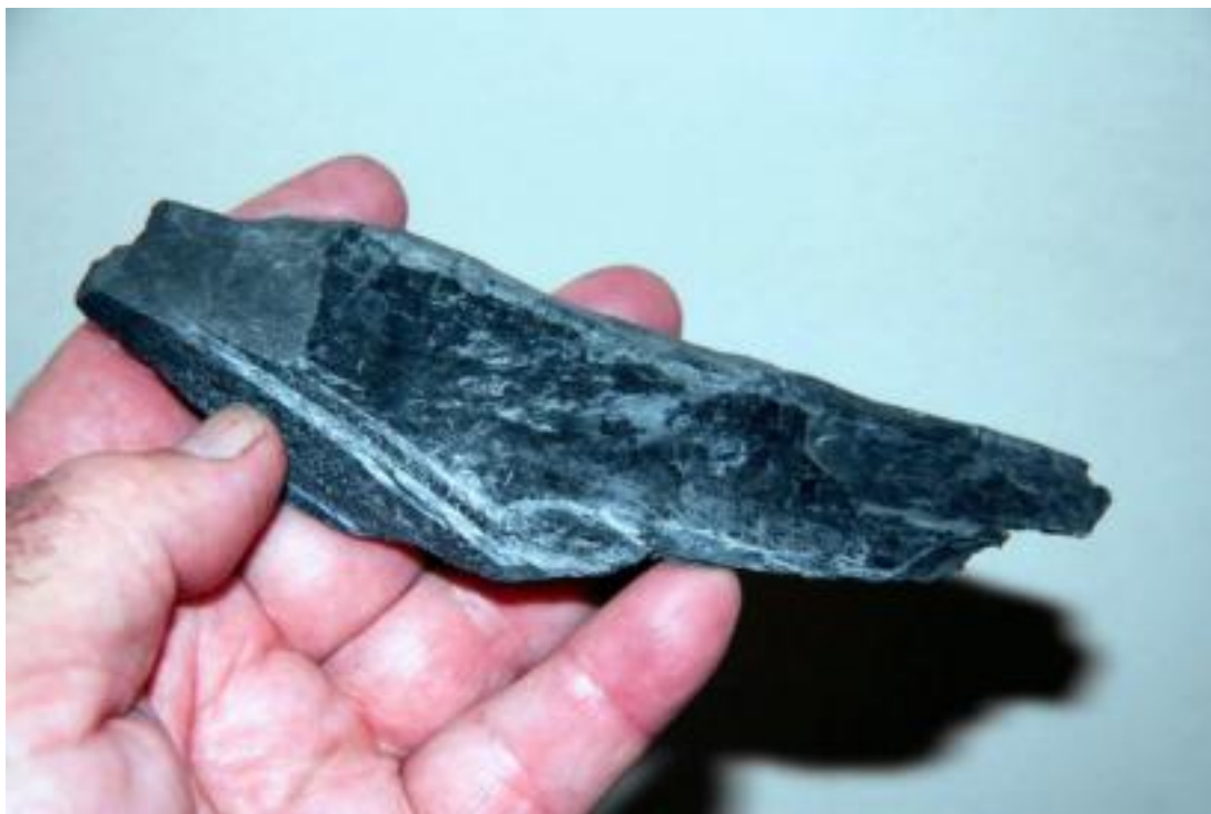
Figure 11: Intact sample of graphitic phyllite from Yacambú-Quibor.
