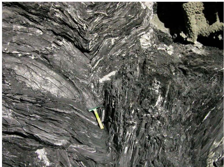
Figure 5: Tectonically deformed graphitic phyllite at the tunnel face.
