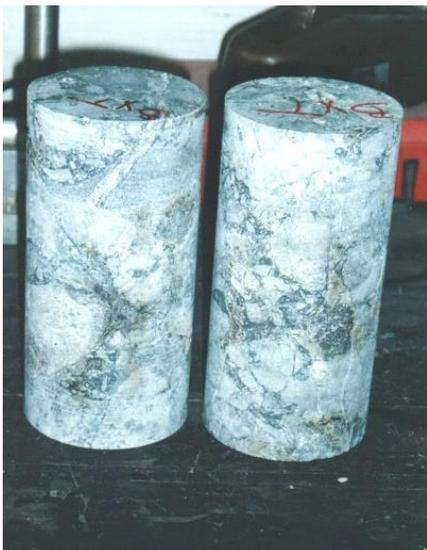
Figure 24. 100 mm diameter by 200 mm long specimens of Braden Breccia from the El Teniente mine in Chile.
