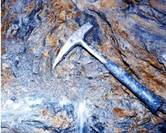
Figure 31: Appearance of the very poor-quality Athenian Schist at the face of the side heading illustrated in Figure 29.
