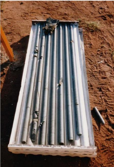
Figure 25: Excellent quality core with very few discontinuities from the massive gneiss of the Rio Grande project in Argentina.
