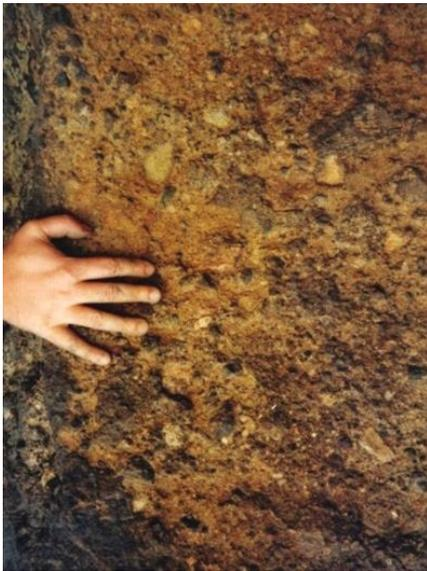
Figure 23: Braden Breccia at El Teniente Mine in Chile. This rock is a cemented breccia with practically no joints. It was dealt with in a manner like weak concrete and tests were carried out on 100 mm diameter specimens illustrated in Figure 24.
