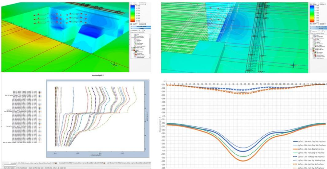
**Figure 15: RS3 full staged excavation model predicted effects on the railway line leaving a rock buttress below the railway wall to be excavated last and introduction of corner propping and additional anchoring.**
