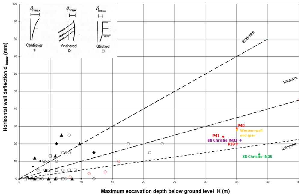
**Figure 8: Field performance with different retention systems**
