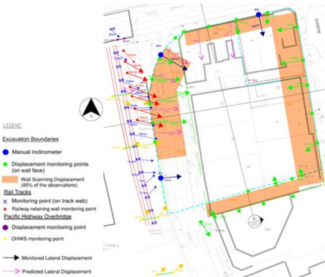
**Figure 17: Instrumentation plan and measured displacement**
