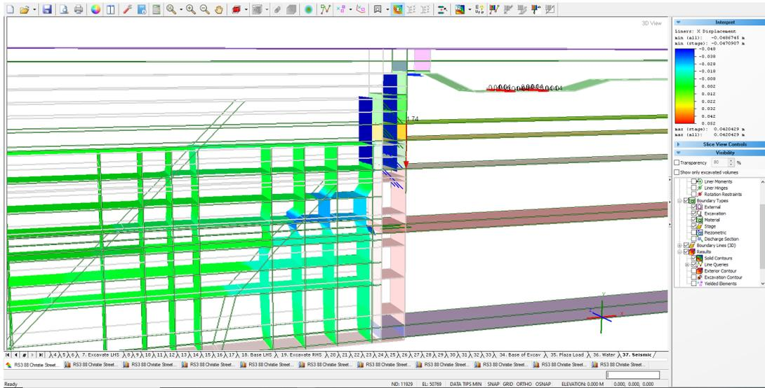
**Figure 12: RS3 slice model with shale bands calibrated showing effect on movement of building floor slabs and walls**
