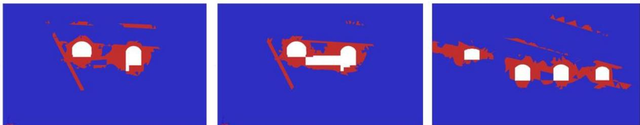
The cavern that presents the most critical issues, mainly because of the vicinity with the major fault system, is the PH. In particular, in correspondence of the upstream wall as highlighted in Figure 5, total displacements up to 35 cm have been computed. In that zone proper countermeasures shall be adopted in order to mitigate the risk of collapse, also in anticipation of the installation of generation technological units.
