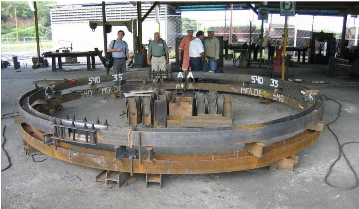
Figure 10. Assembled steel set with two sliding joints in the site workshop
