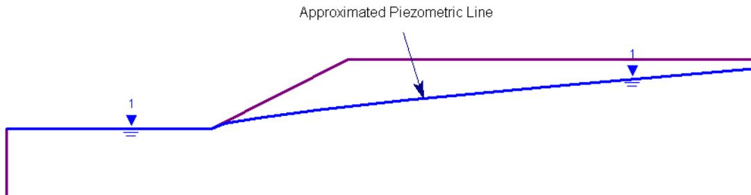
**Figure 2 – Approximated Piezometric Line Location**
