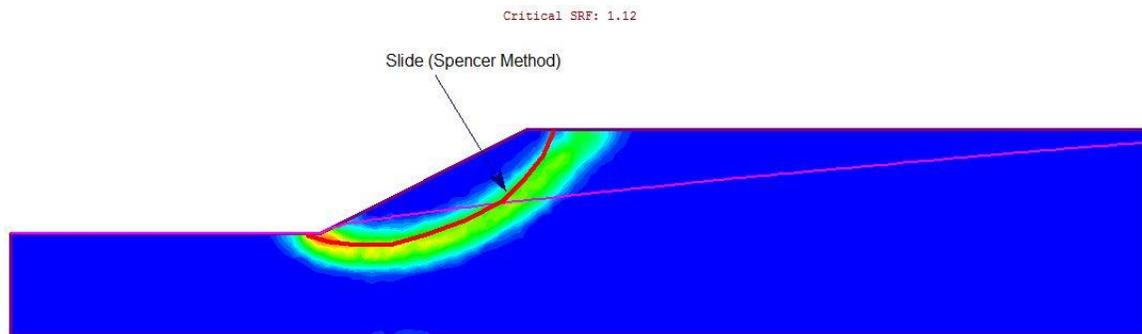
Figure 4 – Maximum Shear Strain Plot
