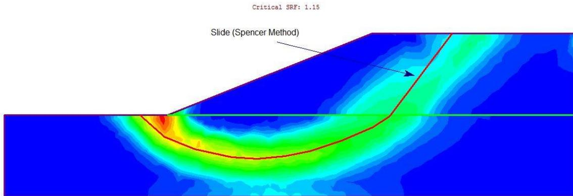
Figure 8 – Maximum Shear Strain Plot (Undrained Shear Strength Profile IV)
