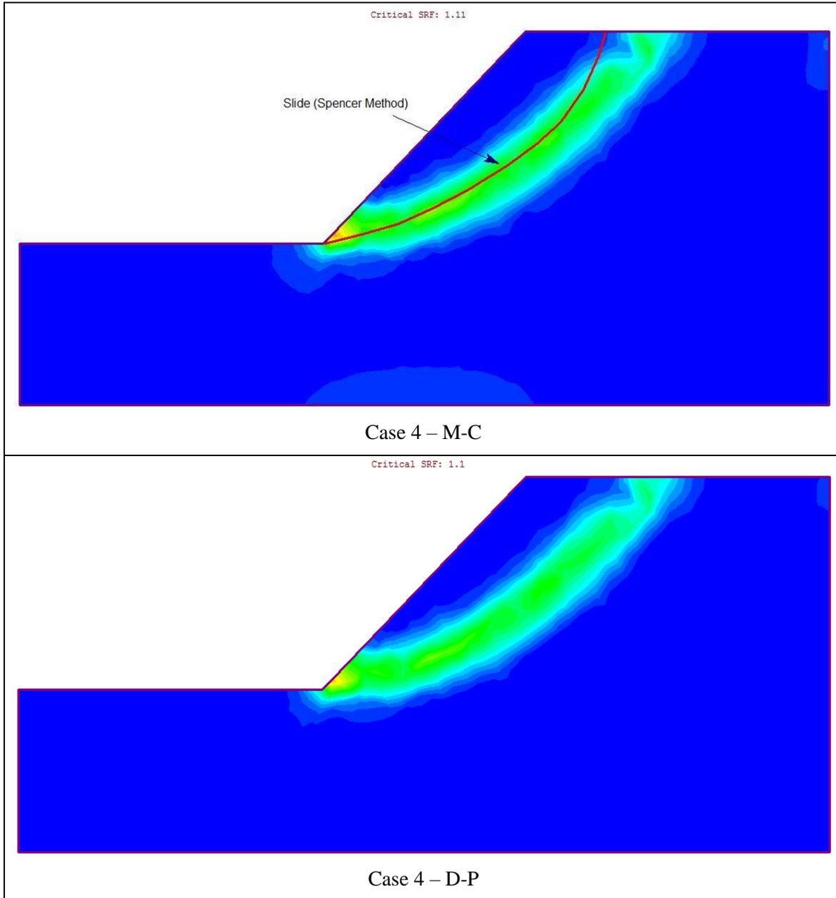
**Figure 8 – Maximum Shear Strain Plot of Case 4**
