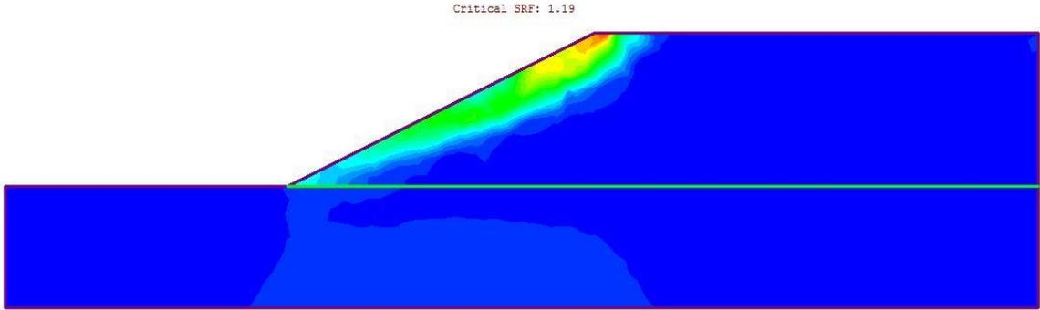
**Figure 2 – Maximum Shear Strain Plot (Very Shallow Slip Surface)**
