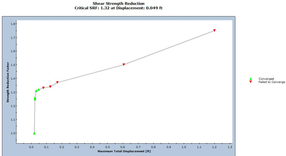
Figure 6 – SSR Convergence Graph (Undrained Shear Strength Profile II)
