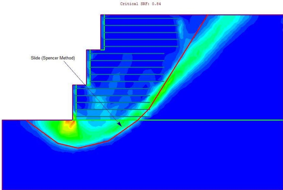
**Figure 2 – Maximum Shear Strain Plot**
