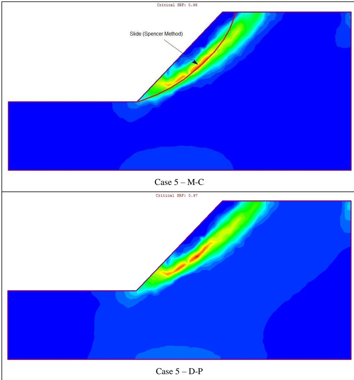
**Figure 10 – Maximum Shear Strain Plot of Case 5**
