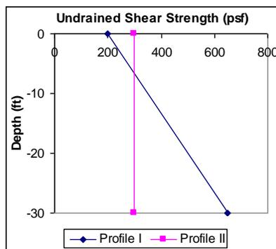
**Figure 1 – Undrained Shear Strength Profiles**
