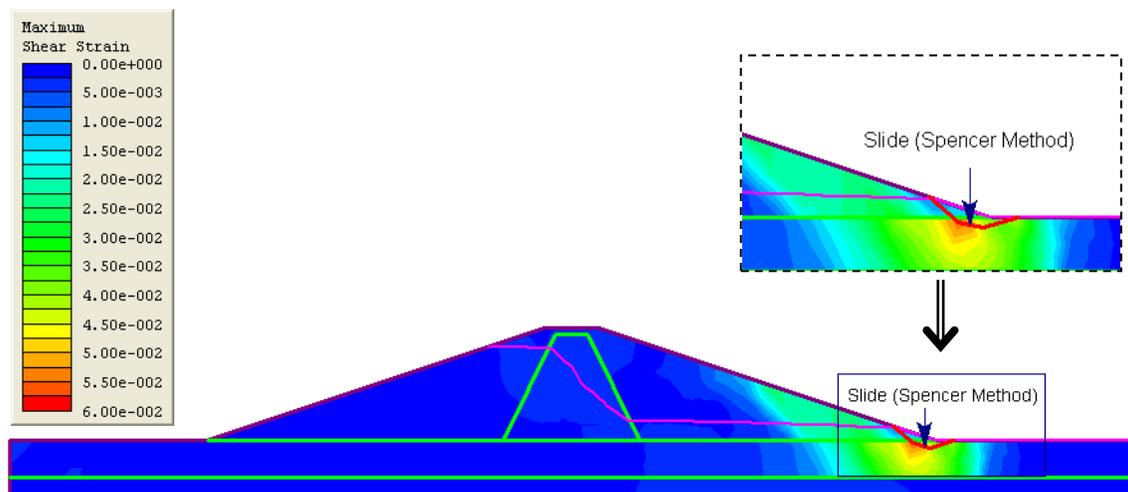
Figure 3 – Maximum Shear Strain Plot
