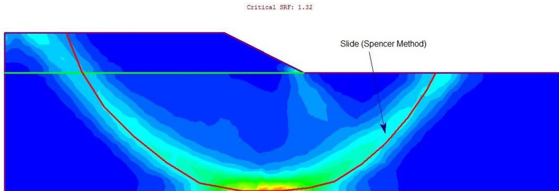
Figure 5 – Maximum Shear Strain Plot (Undrained Shear Strength Profile II)
