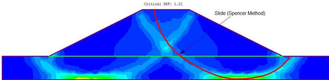
**Figure 2 – Maximum Shear Strain Plot**
