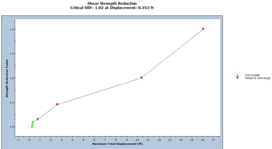
**Figure 7 – SSR Convergence Graph (60 feet-thick Foundation)**
