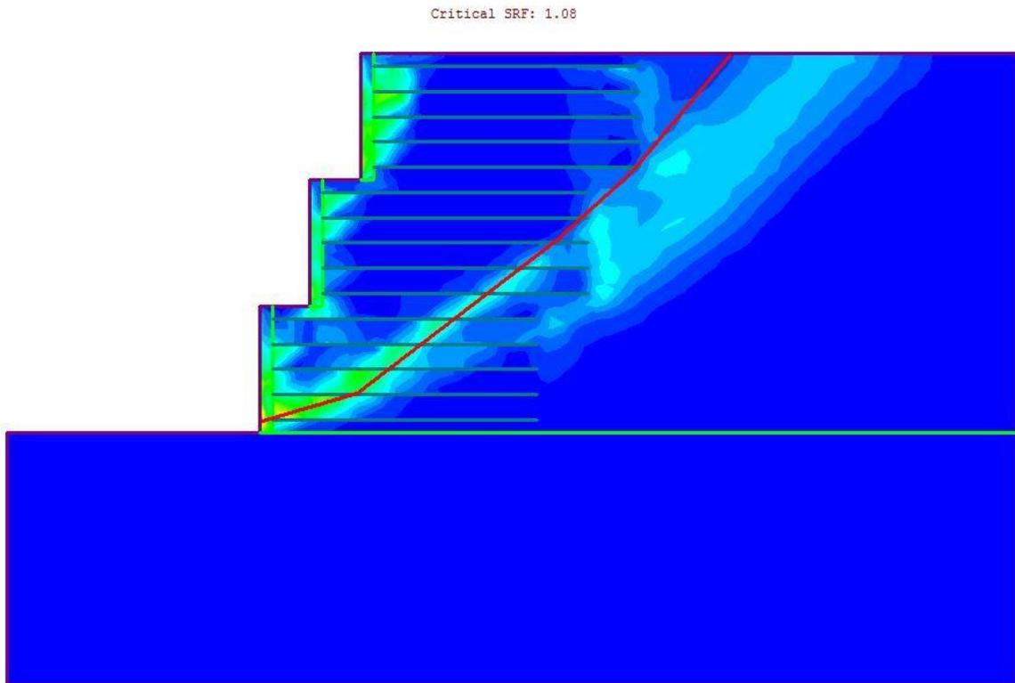
**Figure 2 – Maximum Shear Strain Plot**
