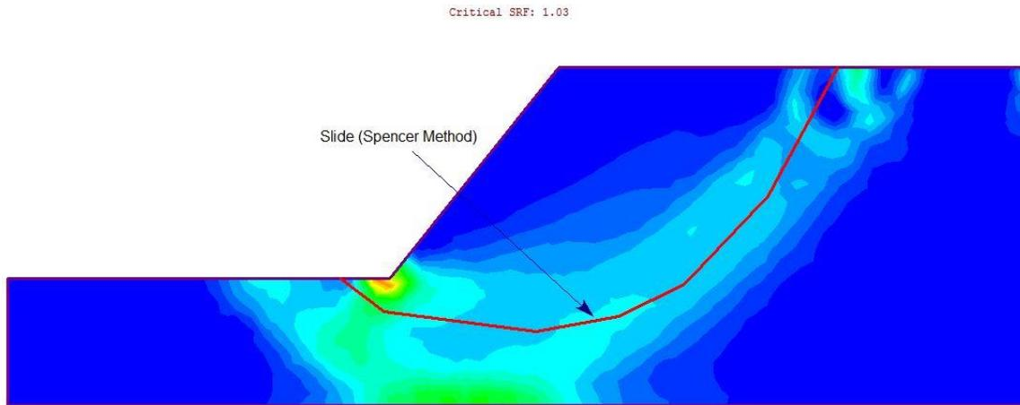
**Figure 2 – Maximum Shear Strain Plot (30 feet-thick Foundation)**
