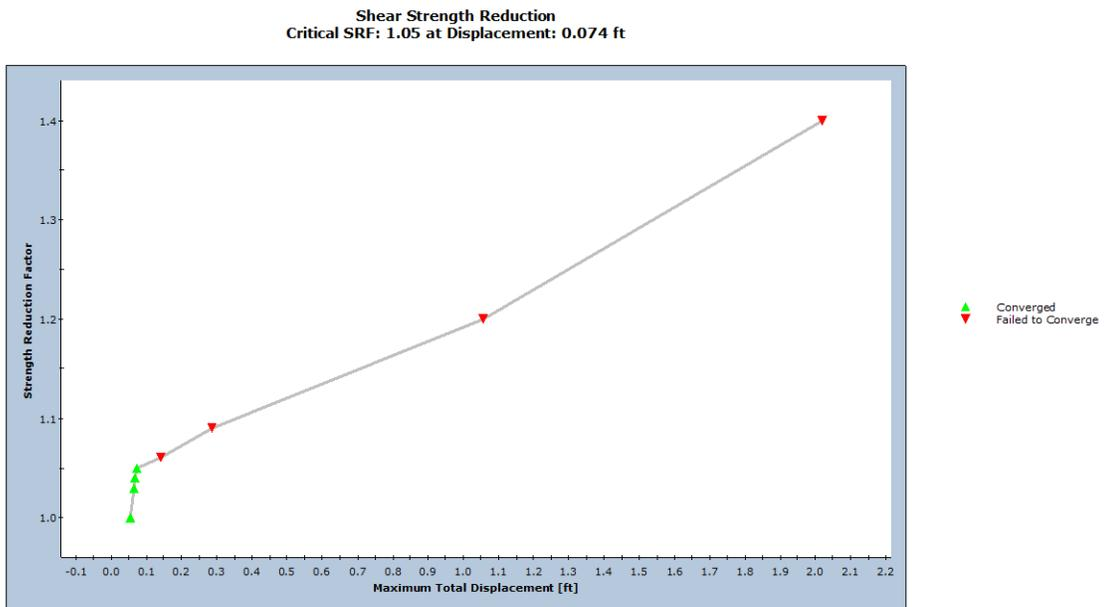
**Figure 7 – SSR Convergence Graph (Undrained Shear Strength Profile III)**
