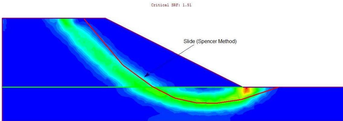
Figure 2 – Maximum Shear Strain Plot
