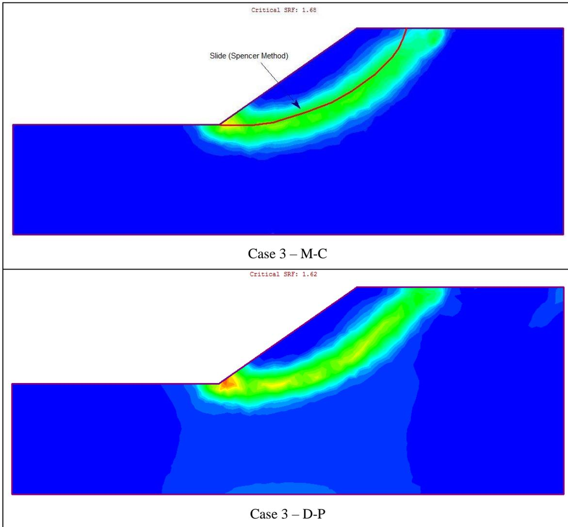
**Figure 6 – Maximum Shear Strain Plot of Case 3**
