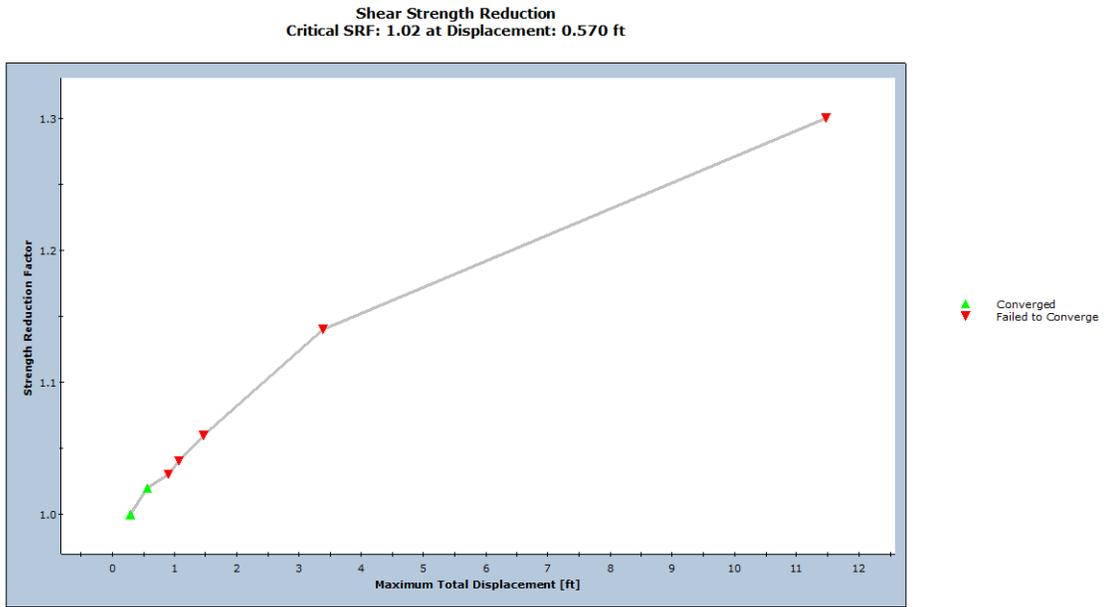
**Figure 5 – SSR Convergence Graph (46.5 feet-thick Foundation)**
