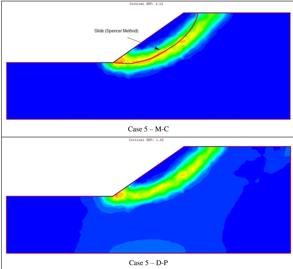
**Figure 10 – Maximum Shear Strain Plot of Case 5**
