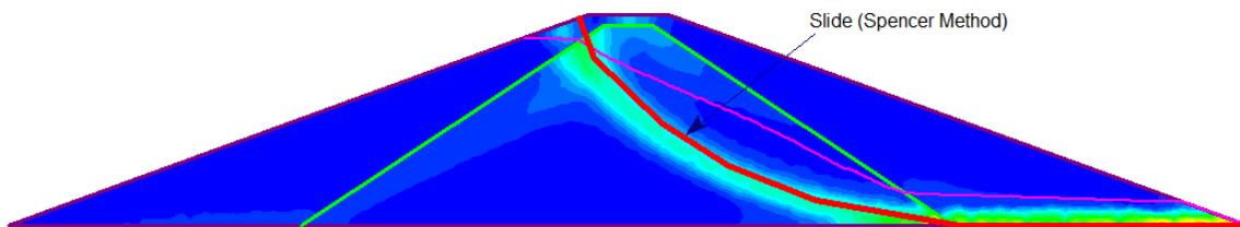
Figure 4 – Maximum Shear Strain Plot
