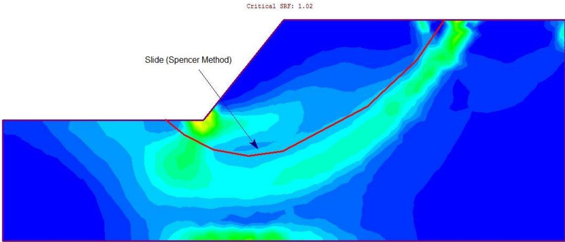
**Figure 6 – Maximum Shear Strain Plot (60 feet-thick Foundation)**
