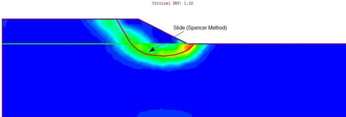
**Figure 3 – Maximum Shear Strain Plot (Undrained Shear Strength Profile I)**
