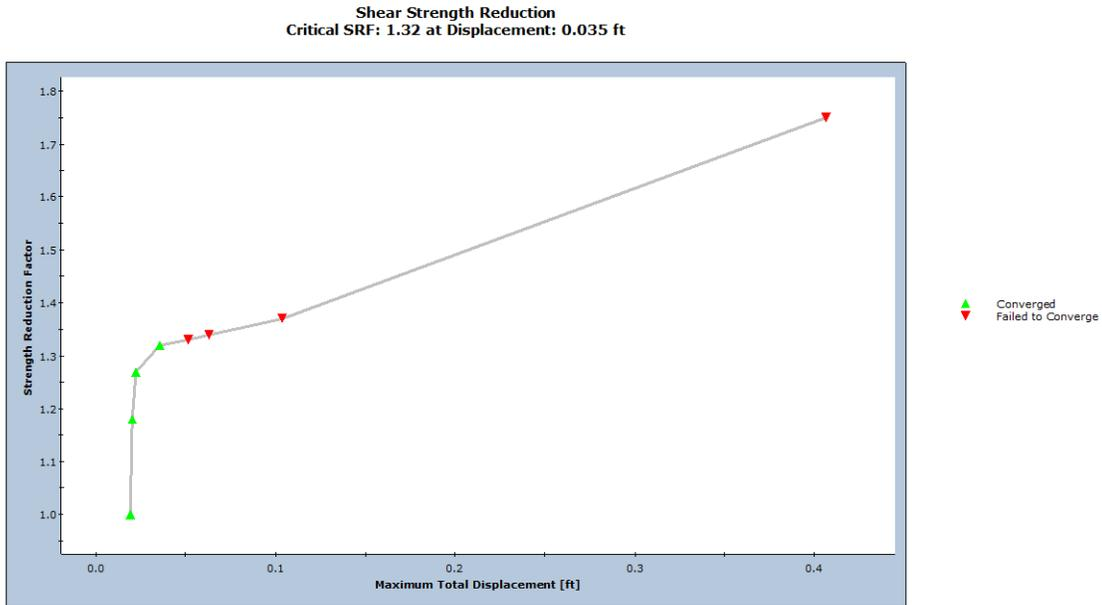
**Figure 4 – SSR Convergence Graph (Undrained Shear Strength Profile I)**
