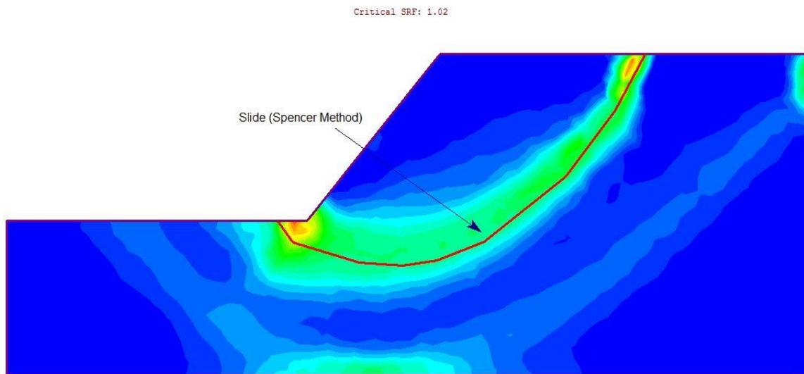
**Figure 4 – Maximum Shear Strain Plot (46.5 feet-thick Foundation)**
