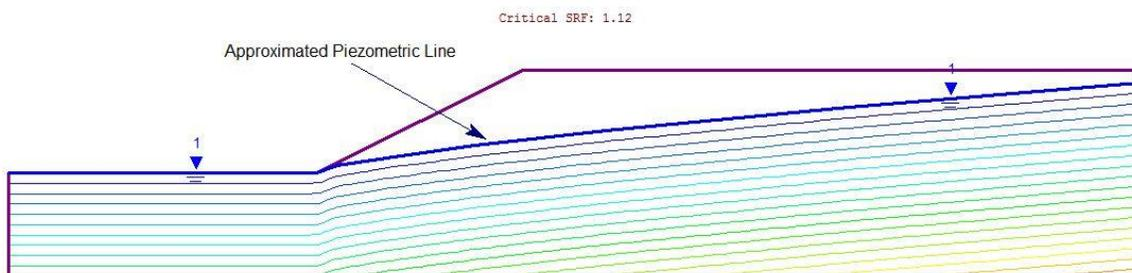
**Figure 6 – Pore Water Pressure Plot**
