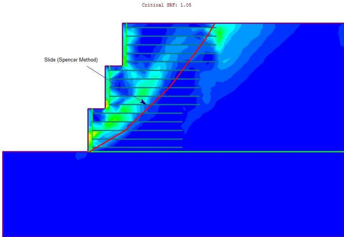
Figure 2 – Maximum Shear Strain Plot
