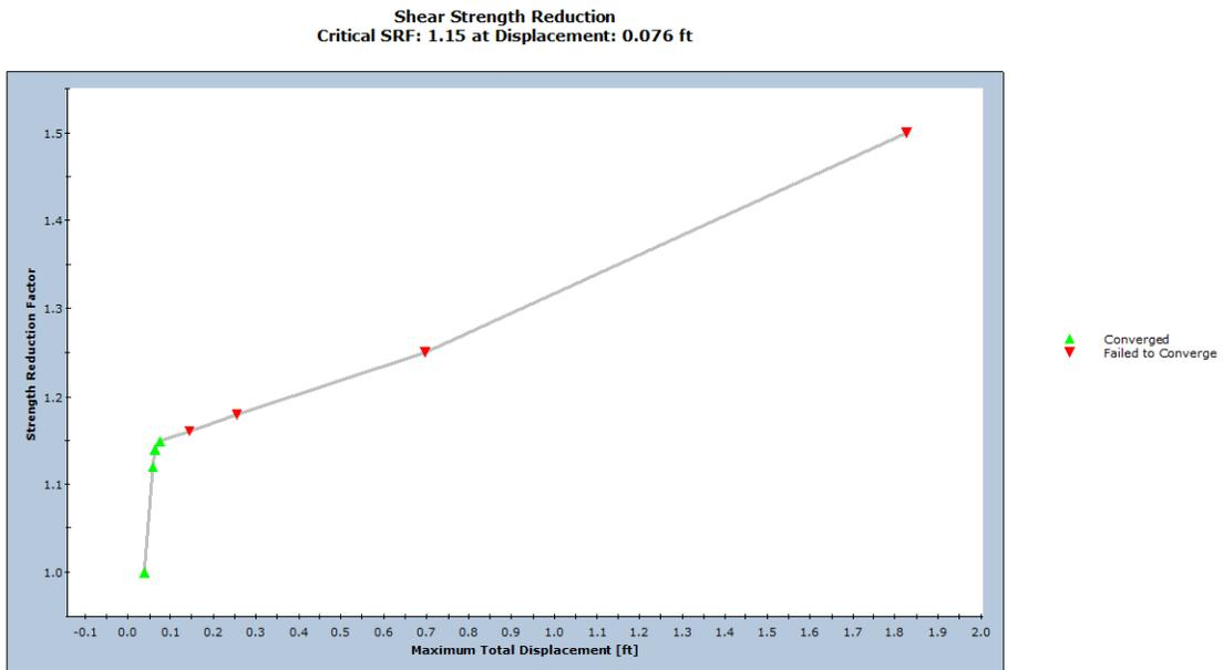
Figure 9 – SSR Convergence Graph (Undrained Shear Strength Profile IV)
