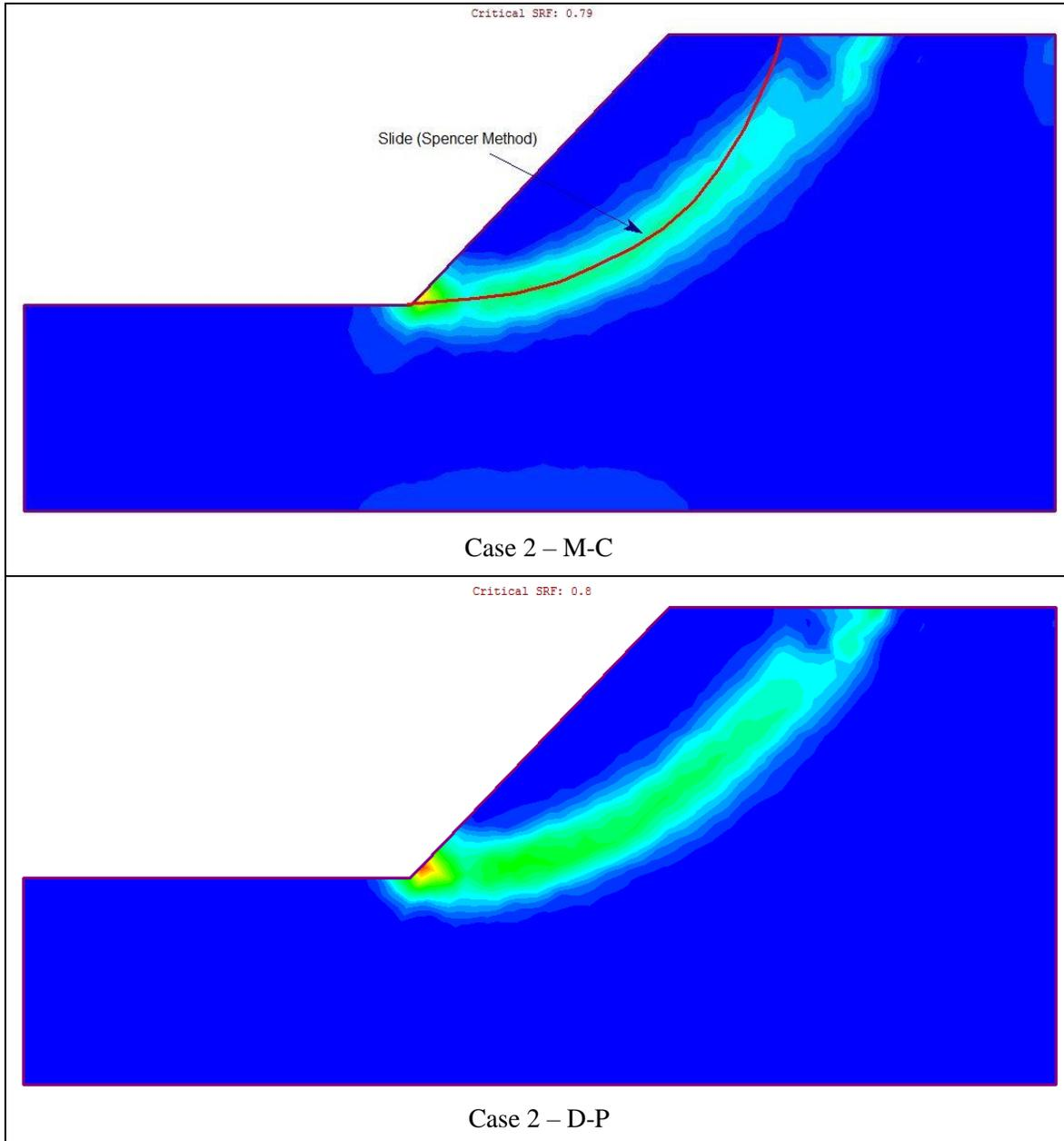
**Figure 4 – Maximum Shear Strain Plot of Case 2**
