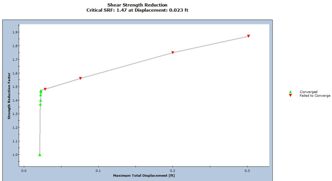
**Figure 3 – SSR Convergence Graph (Very Shallow Slip Surface)**
