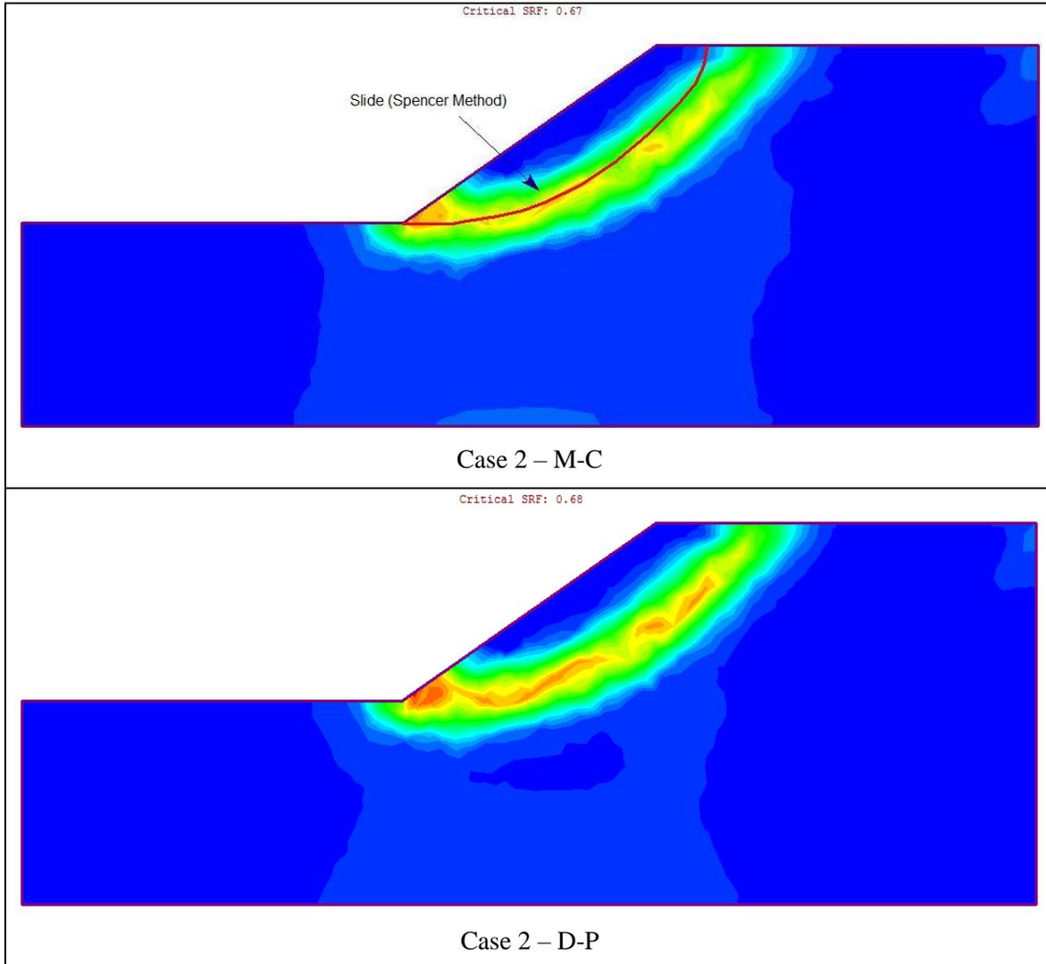
**Figure 4 – Maximum Shear Strain Plot of Case 2**
