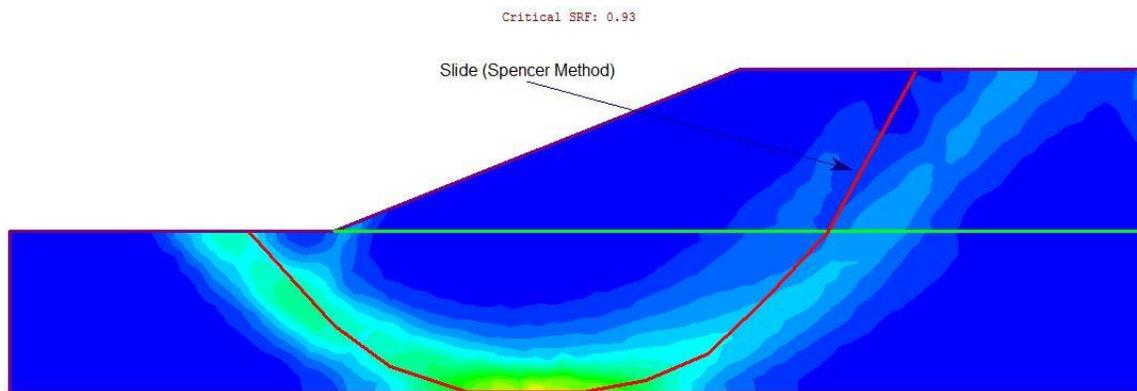
Figure 4 – Maximum Shear Strain Plot (Undrained Shear Strength Profile II)
