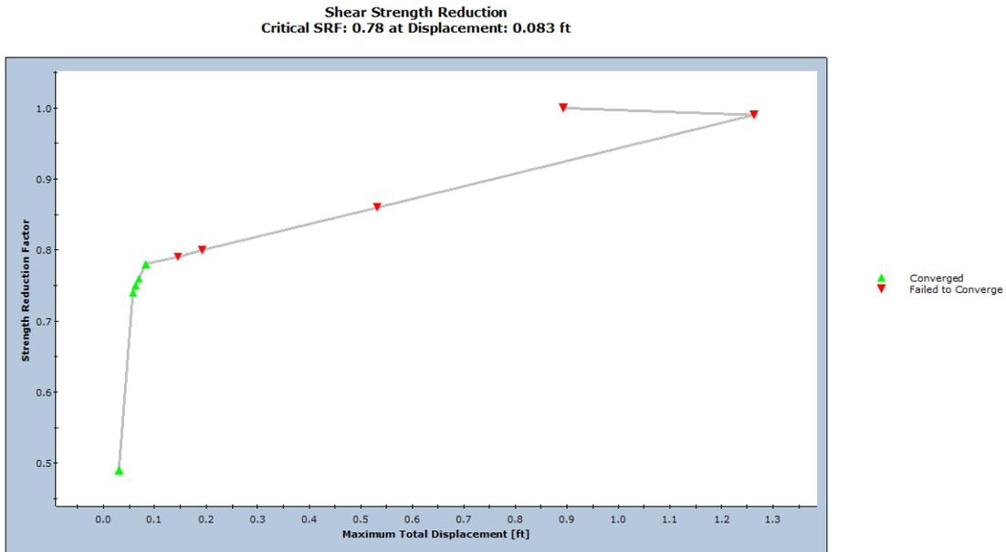
Figure 3 – SSR Convergence Graph (Undrained Shear Strength Profile I)
