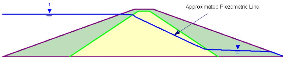
Figure 2 – Approximated Piezometric Line Location
