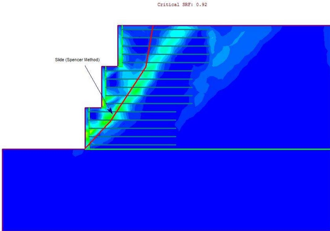
Figure 2 – Maximum Shear Strain Plot
