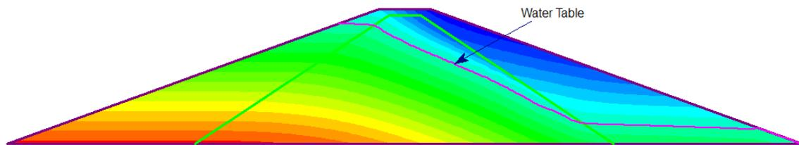
Figure 3 – Pore Water Pressure Plot
