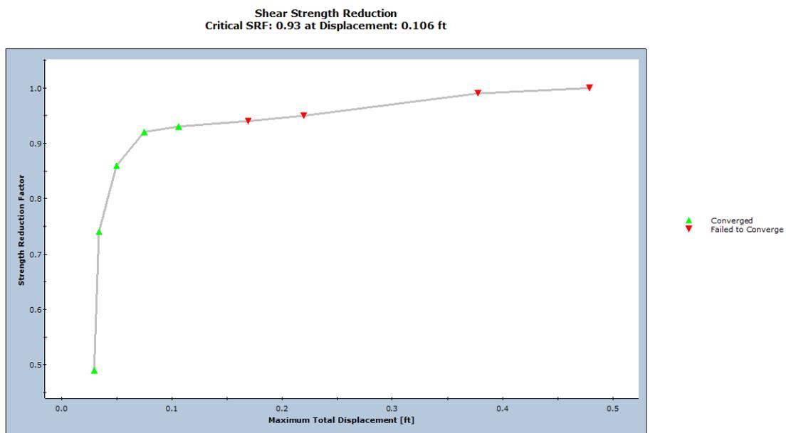
Figure 5 – SSR Convergence Graph (Undrained Shear Strength Profile II)
