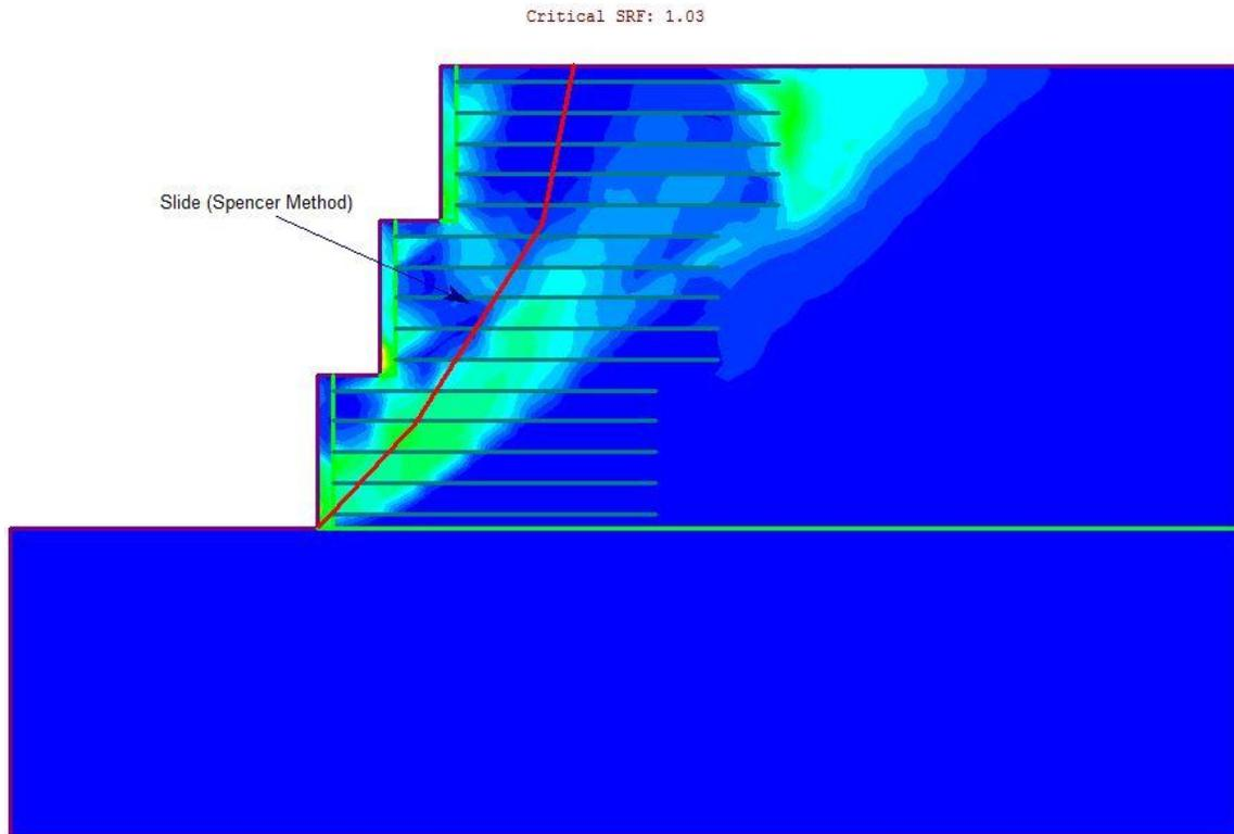
Figure 2 – Maximum Shear Strain Plot
