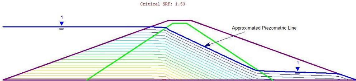
**Figure 6 – Pore Water Pressure Plot**
