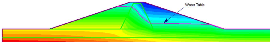
Figure 2 – Pore Water Pressure Plot
