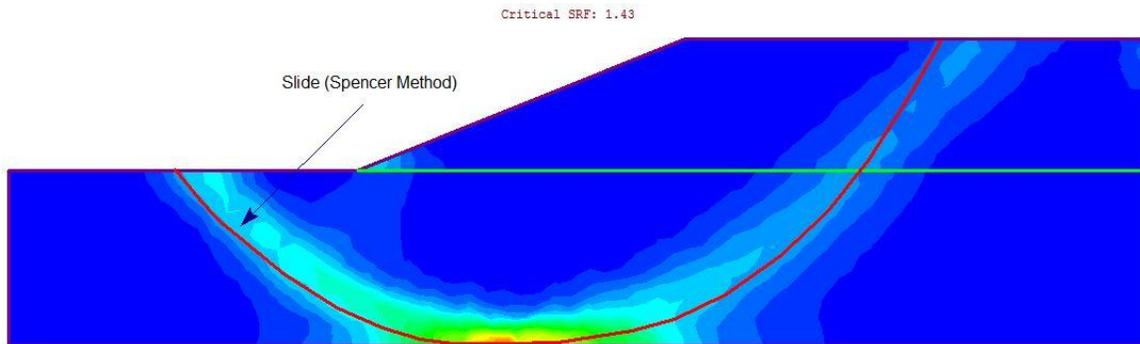
Figure 4 – Maximum Shear Strain Plot (Deep Slip Surface)
