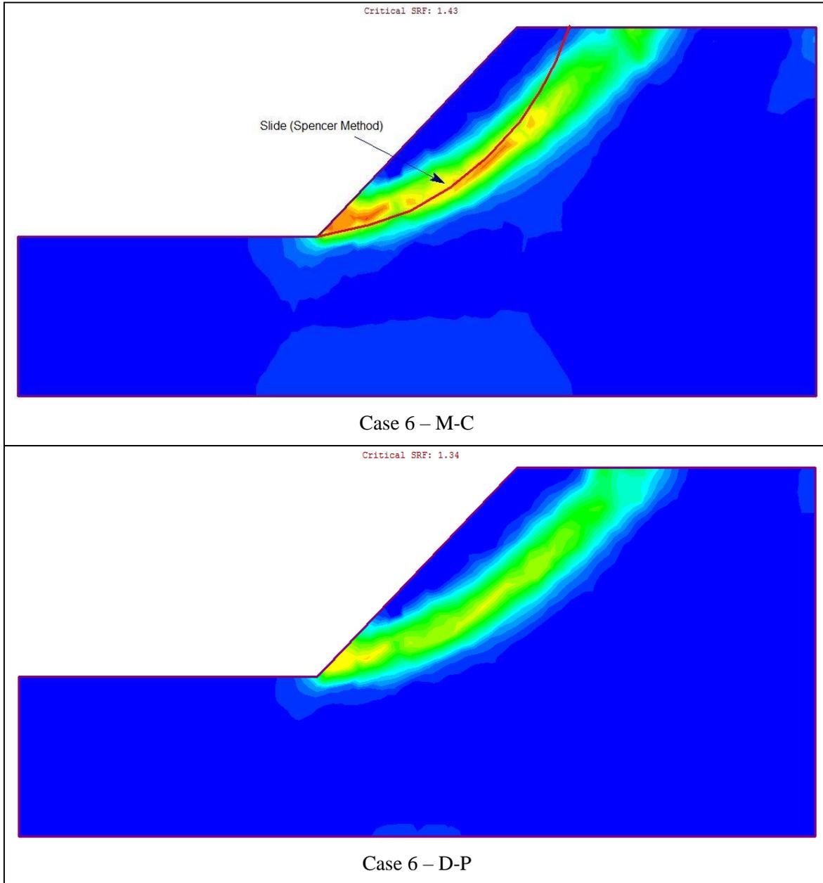
**Figure 12 – Maximum Shear Strain Plot of Case 6**
