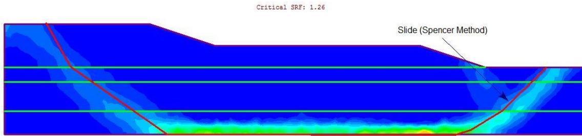
**Figure 2 – Maximum Shear Strain Plot**
