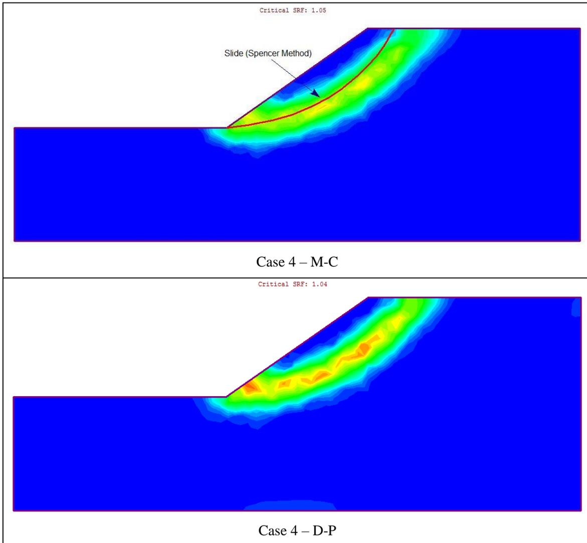
**Figure 8 – Maximum Shear Strain Plot of Case 4**
