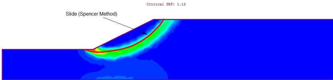
**Figure 7 – Maximum Shear Strain Plot**
