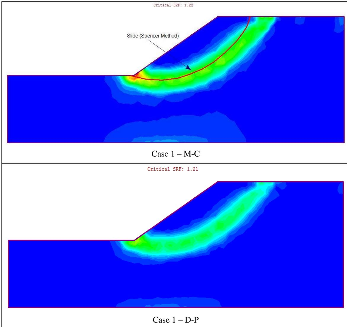
**Figure 2 – Maximum Shear Strain Plot of Case 1**
