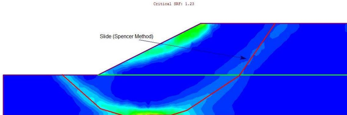
**Figure 4 – Maximum Shear Strain Plot (Deep Slip Surface)**
