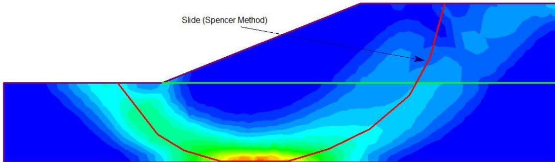
Figure 2 – Maximum Shear Strain Plot (Undrained Shear Strength Profile I)
