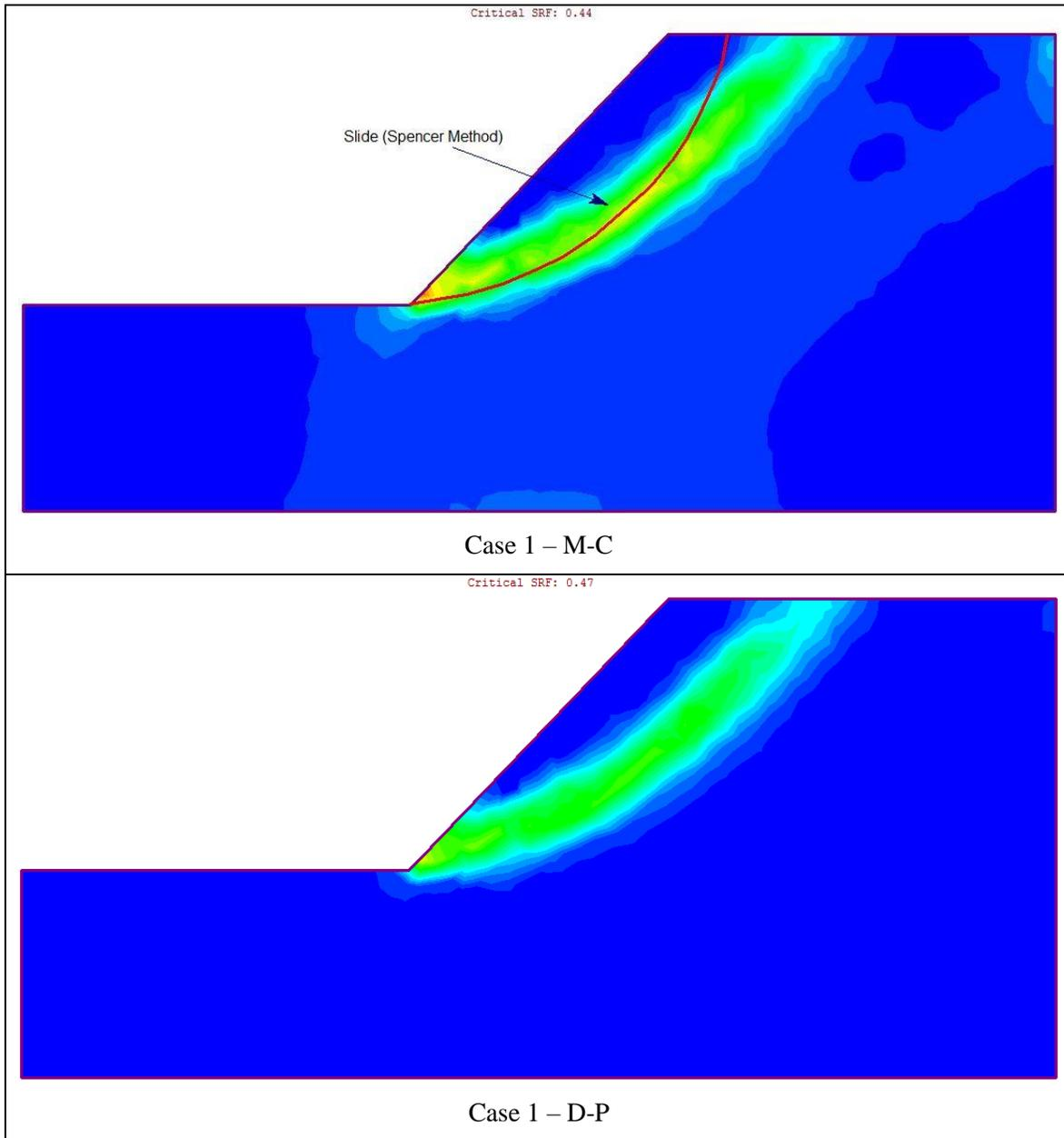
**Figure 2 – Maximum Shear Strain Plot of Case 1**
