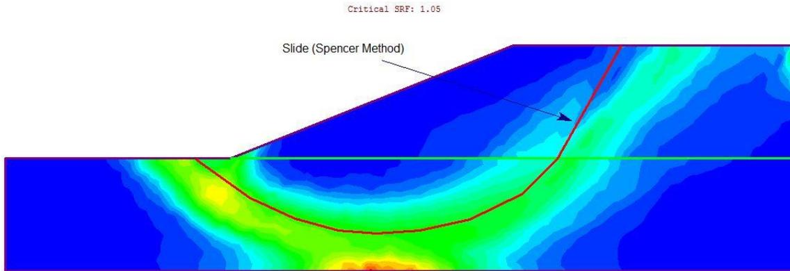
**Figure 6 – Maximum Shear Strain Plot (Undrained Shear Strength Profile III)**
