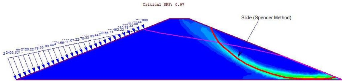
**Figure 3 – Maximum Shear Strain Plot**
