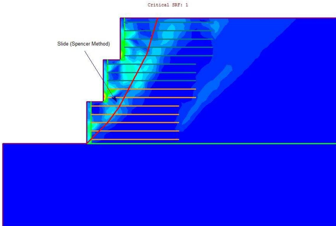
Figure 2 – Maximum Shear Strain Plot
