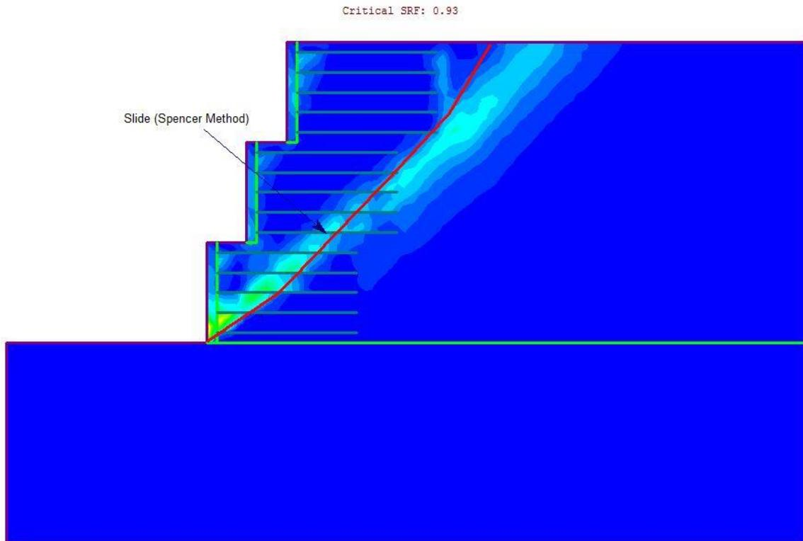
Figure 2 – Maximum Shear Strain Plot
