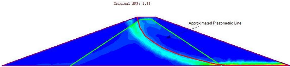
**Figure 7 – Maximum Shear Strain Plot**
