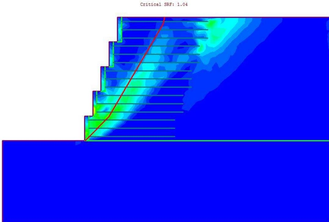
Figure 2 – Maximum Shear Strain Plot
