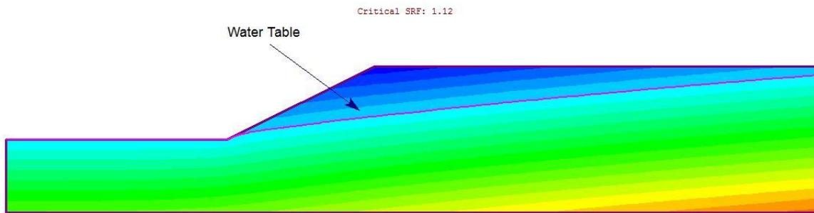
Figure 3 – Pore Water Pressure Plot
