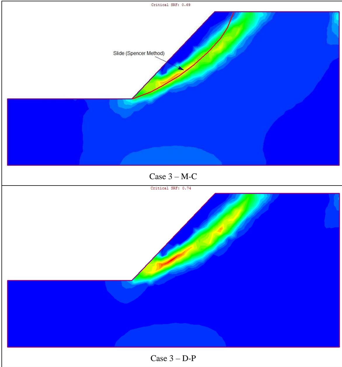
**Figure 6 – Maximum Shear Strain Plot of Case 3**
