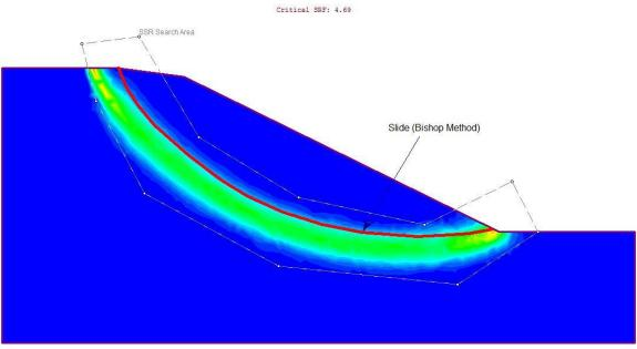
Figure 7 – Maximum Shear Strain Plot of Case 3
