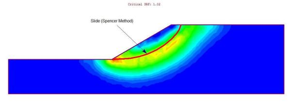
Figure 5 – Maximum Shear Strain Plot of Case 2
