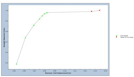
Shear Strength Reduction Critical SRF: 0.98 at Displacement: 0.082 m
