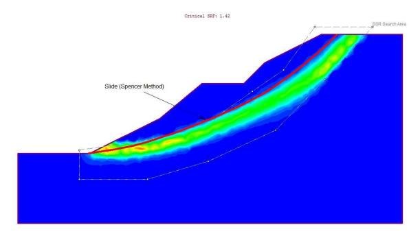
Figure 5 – Maximum Shear Strain Plot of Case 3
