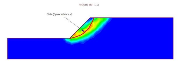
Figure 6 – Maximum Shear Strain Plot of Case 3
