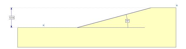
Figure 1 - Case 1, Geometry  $\beta = 15^{\circ}$
