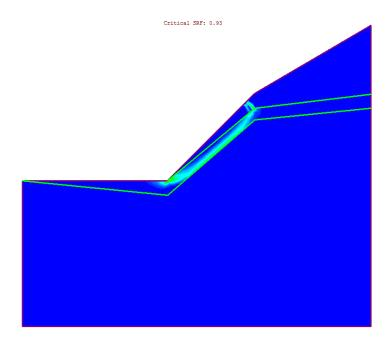
Figure 13 - Maximum Shear Strain Plot of Analysis III Case 2
