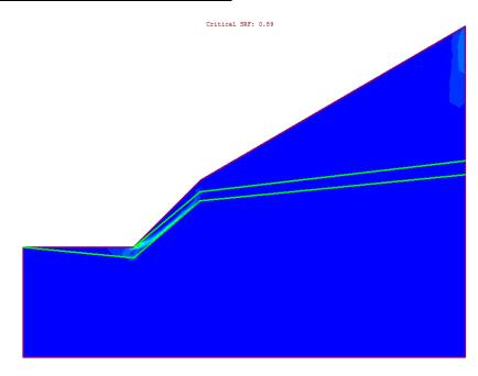
Figure 8 - Maximum Shear Strain Plot of Analysis II Case 1
