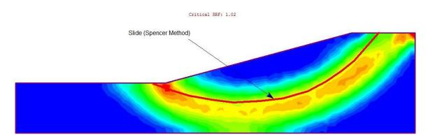
Figure 4 – Maximum Shear Strain Plot of Case 1
