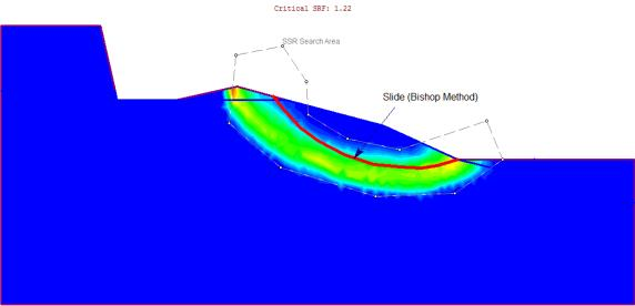
Figure 17 – Maximum Shear Strain Plot of Case 12
