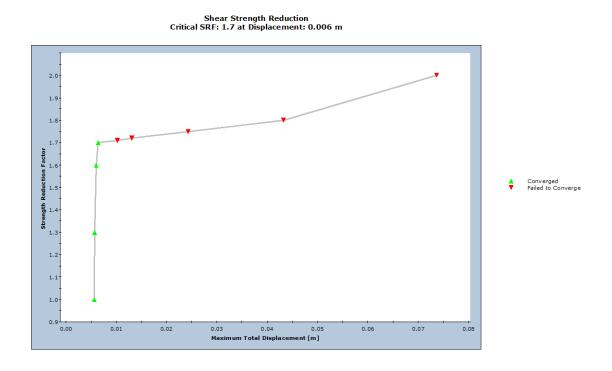
Figure 12 – Graph of Shear Strength Reduction for Case 7
