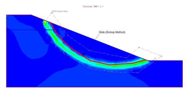
Figure 11 – Maximum Shear Strain Plot of Case 7
