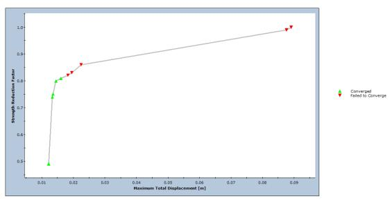
Figure 14 - SSR Convergence Graph of Analysis III Case 1
