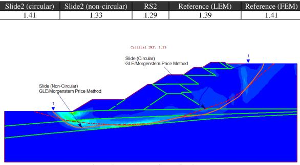
**Figure 2 – Maximum Shear Strain Plot**
