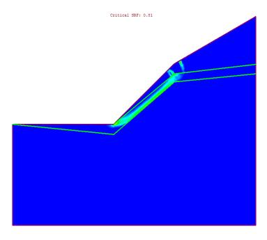
Figure 12 - Maximum Shear Strain Plot of Analysis III Case 1
