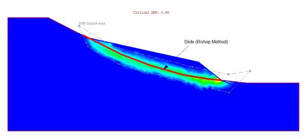
Figure 13 – Maximum Shear Strain Plot of Case 8
