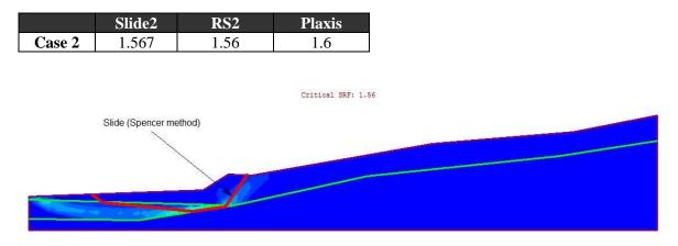
Figure 4 - Maximum Shear Strain Plot of Case 2
