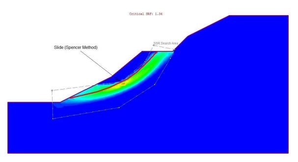
Figure 4 – Maximum Shear Strain Plot of Case 2
