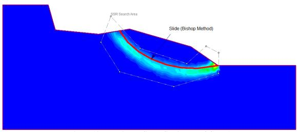
Figure 10 – Maximum Shear Strain Plot of Case 6
