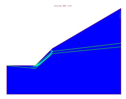
Figure 9 - Maximum Shear Strain Plot of Analysis II Case 2
