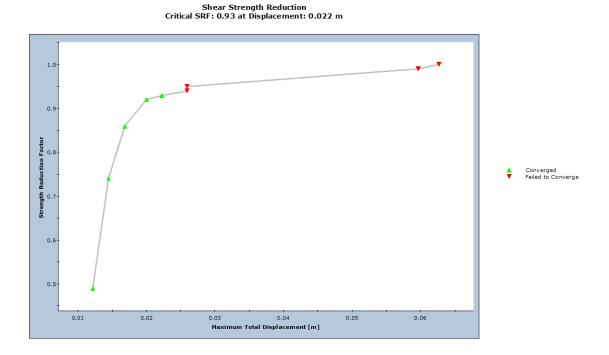
Figure 15 - SSR Convergence Graph of Analysis III Case 2
