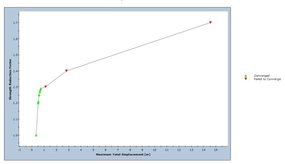
Shear Strength Reduction Critical SRF: 1.29 at Displacement: 0.735 m
