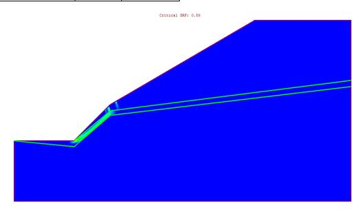
Figure 4 - Maximum Shear Strain Plot of Analysis I Case 1
