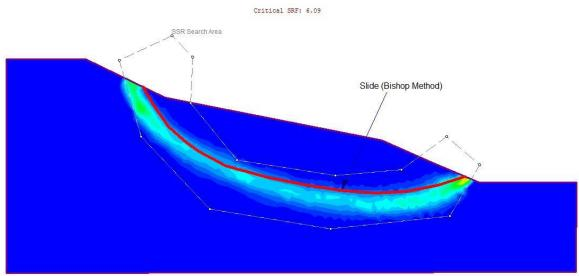
Figure 6 – Maximum Shear Strain Plot of Case 2
