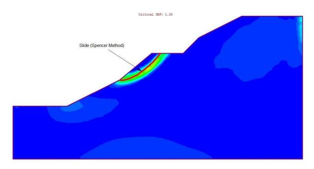
Figure 2 – Maximum Shear Strain Plot of Case 1
