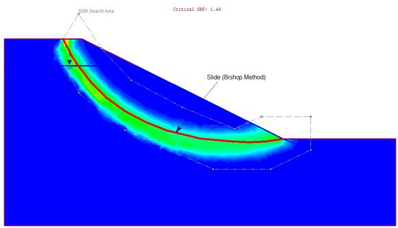
Figure 16 – Maximum Shear Strain Plot of Case 11
