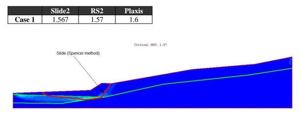
Figure 2 - Maximum Shear Strain Plot of Case 1
