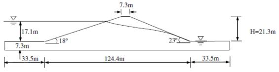
**Figure 1 - Dam Geometry**
