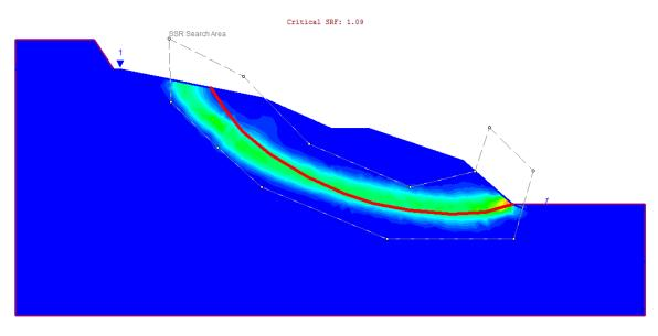
Figure 15 – Maximum Shear Strain Plot of Case 10
