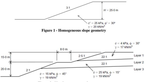
Figure 2 - Non-homogeneous slope geometry
