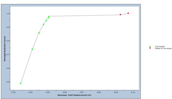
Shear Strength Reduction Critical SRF: 0.98 at Displacement: 0.051 m
