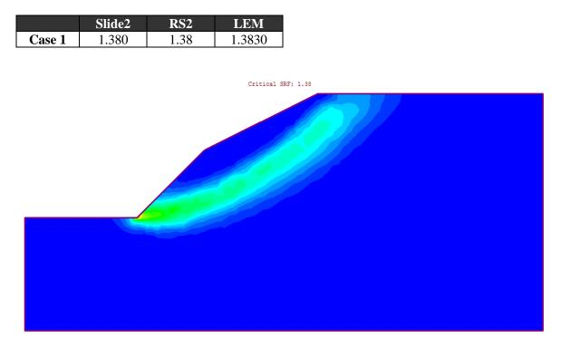
Figure 2 – Maximum Shear Strain Plot of Case 1
