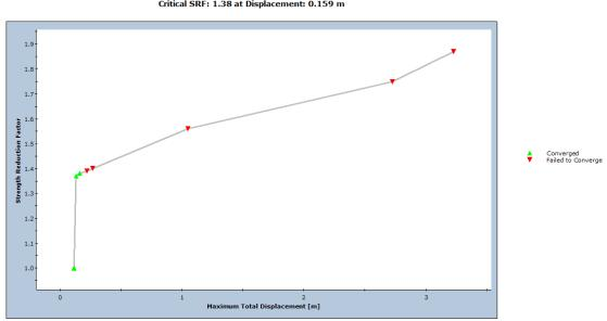
Shear Strength Reduction Critical SRF: 1.38 at Displacement: 0.159 m
