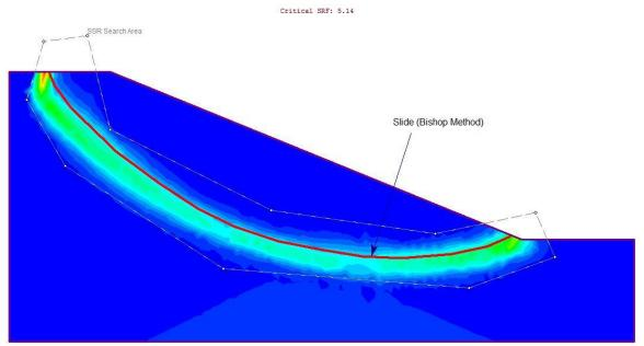
Figure 4 – Maximum Shear Strain Plot of Case 1
