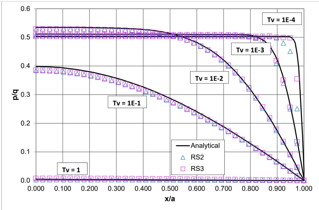
Figure 2-3: Pore pressure versus distance ratio from centre
