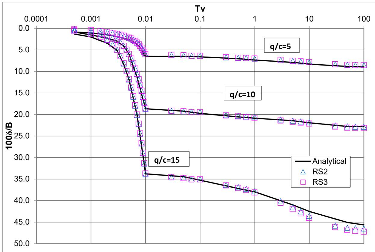
Figure 6-6: Settlement versus time factor for elastoplastic strip footing
