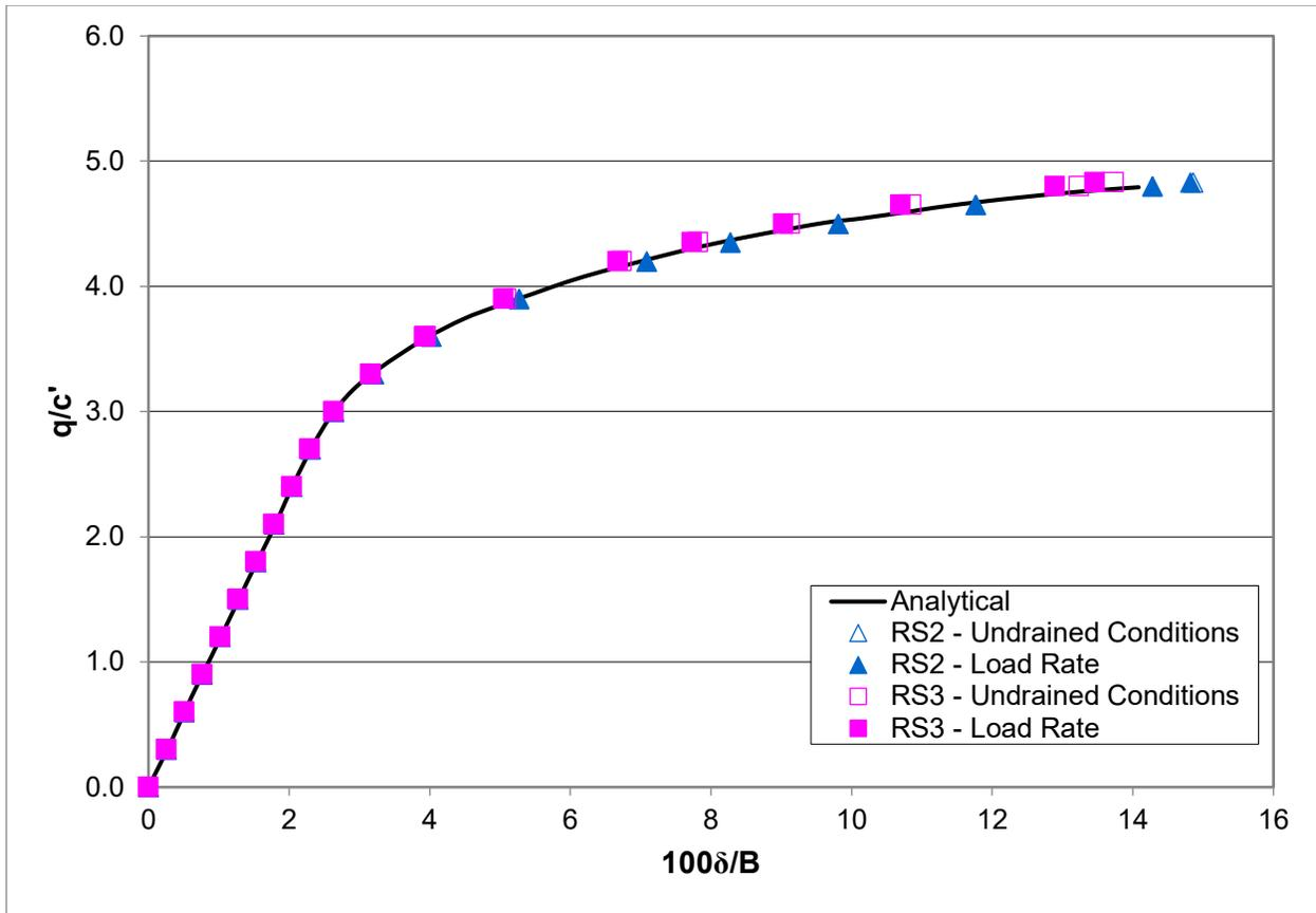
Figure 5-3: Pressure versus displacement for undrained loading
