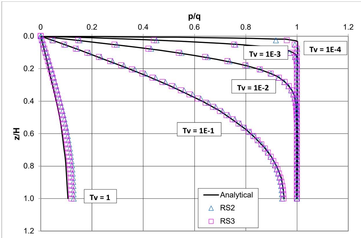
Figure 1-6: Pore pressure versus ratio of depth
