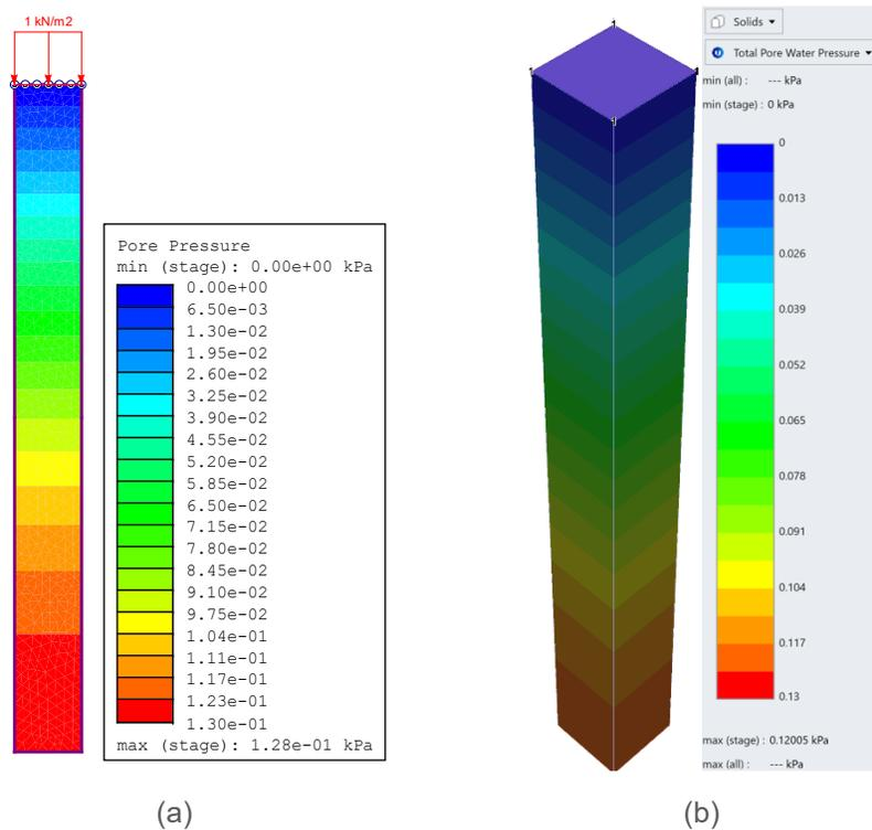
Figure 1-3: Pore pressure contour for  $T_v = 1$  as modeled in (a) RS2 and (b) RS3
