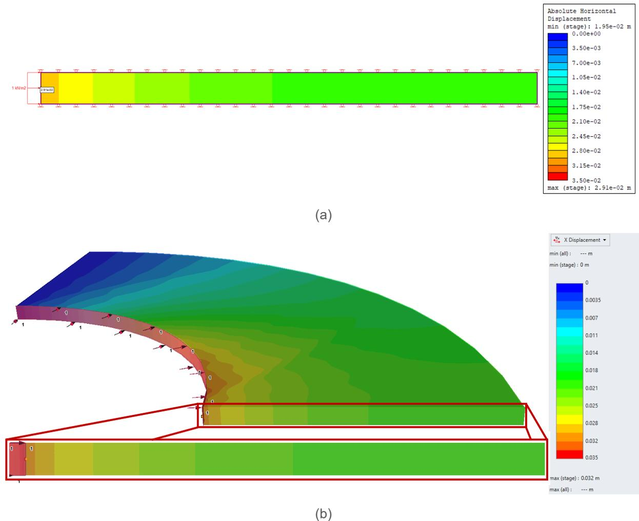
Figure 4-2: Horizontal displacement contour plot before peak load in (a) RS2 and (b) RS3
