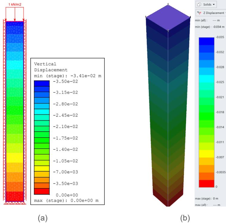
Figure 1-4: Vertical displacement contour for  $T_v = 1$  as modelled in (a) RS2 and (b) RS3
