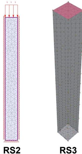
Figure 1-2 Model Geometry and Applied Boundary Conditions.
