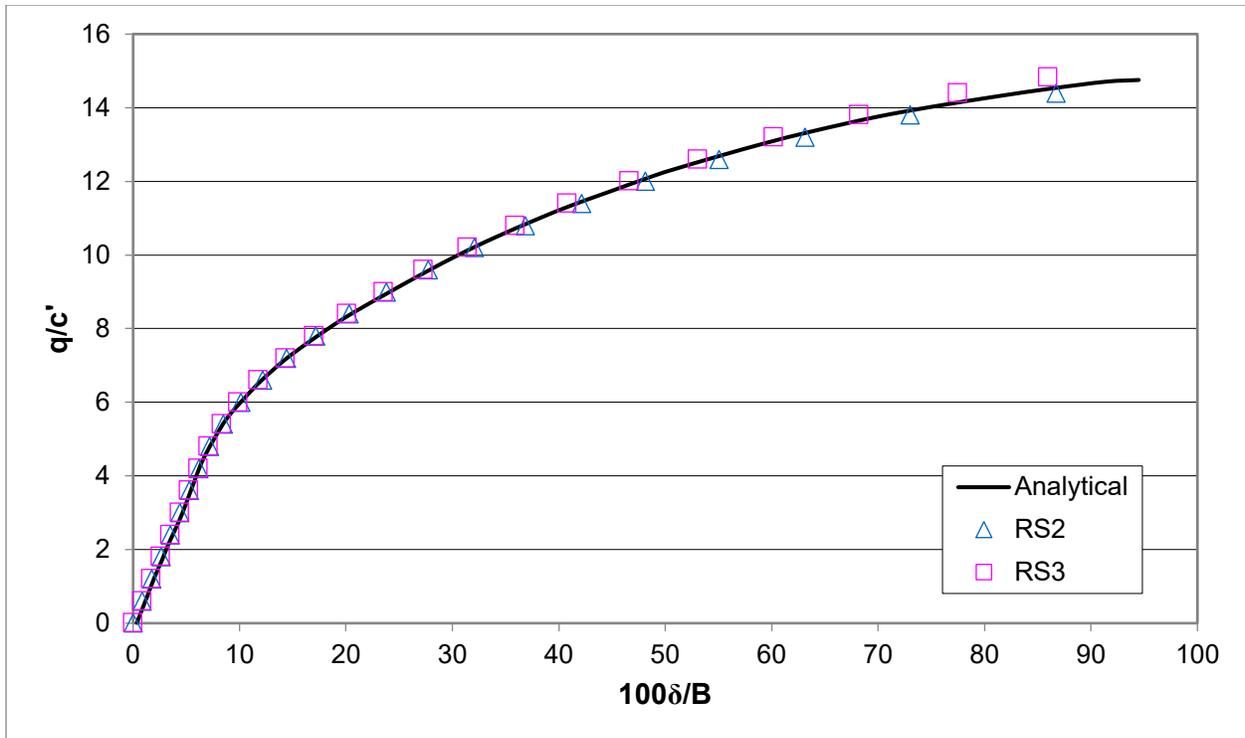
Figure 6-8: Pressure versus displacement for flexible strip footing with varying loading rates
