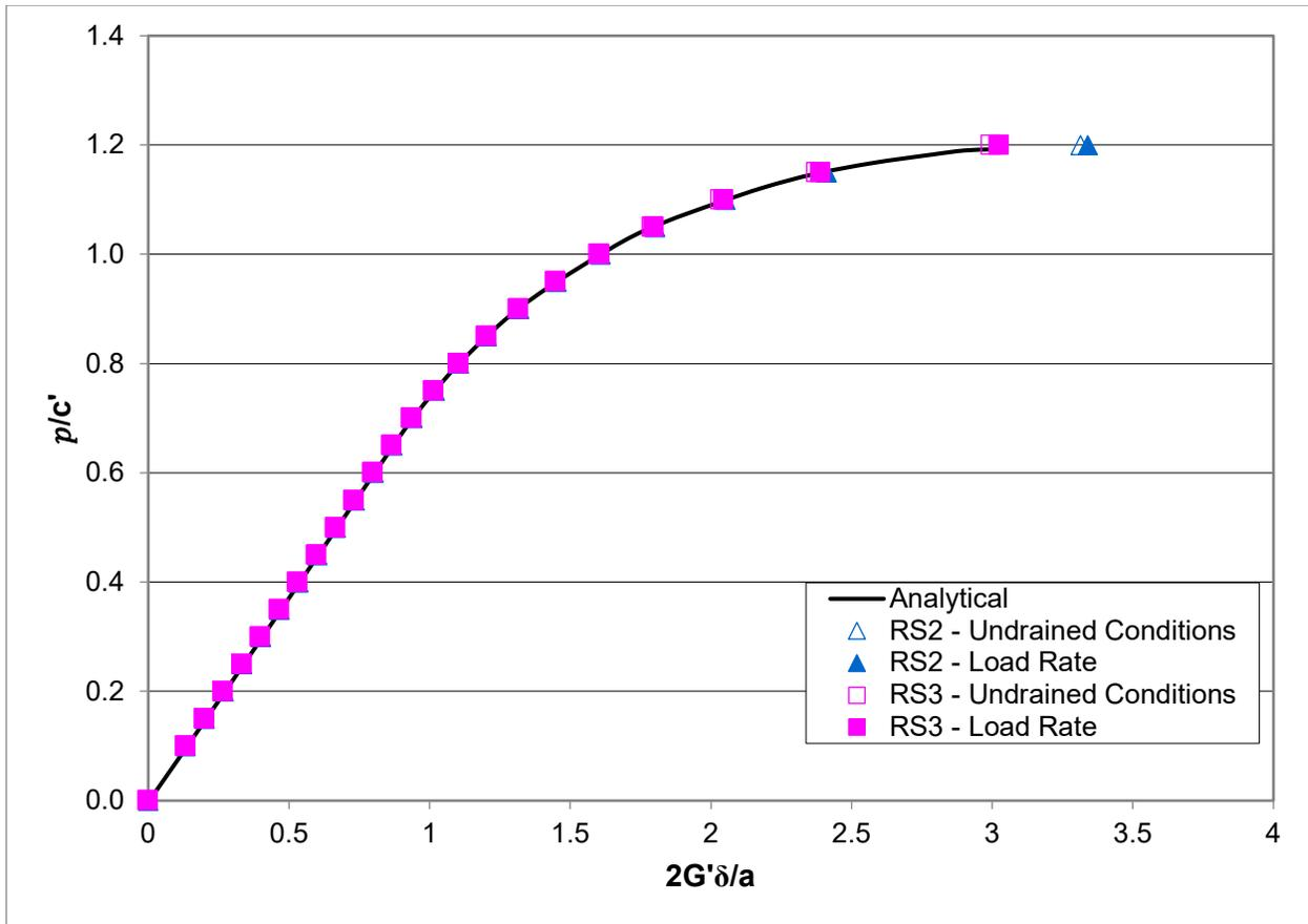
Figure 4-5: Pressure versus displacement for undrained loading
