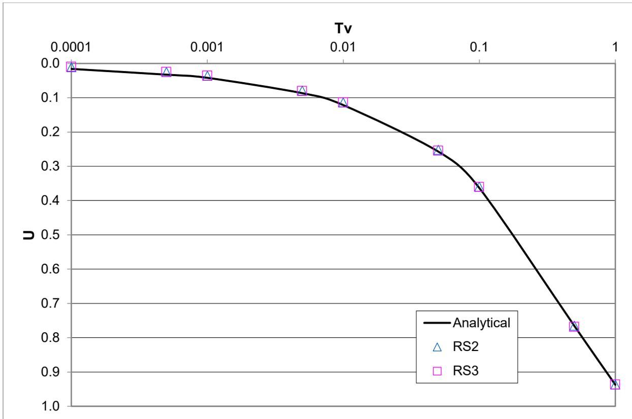
Figure 1-5: Degree of consolidation versus time factor
