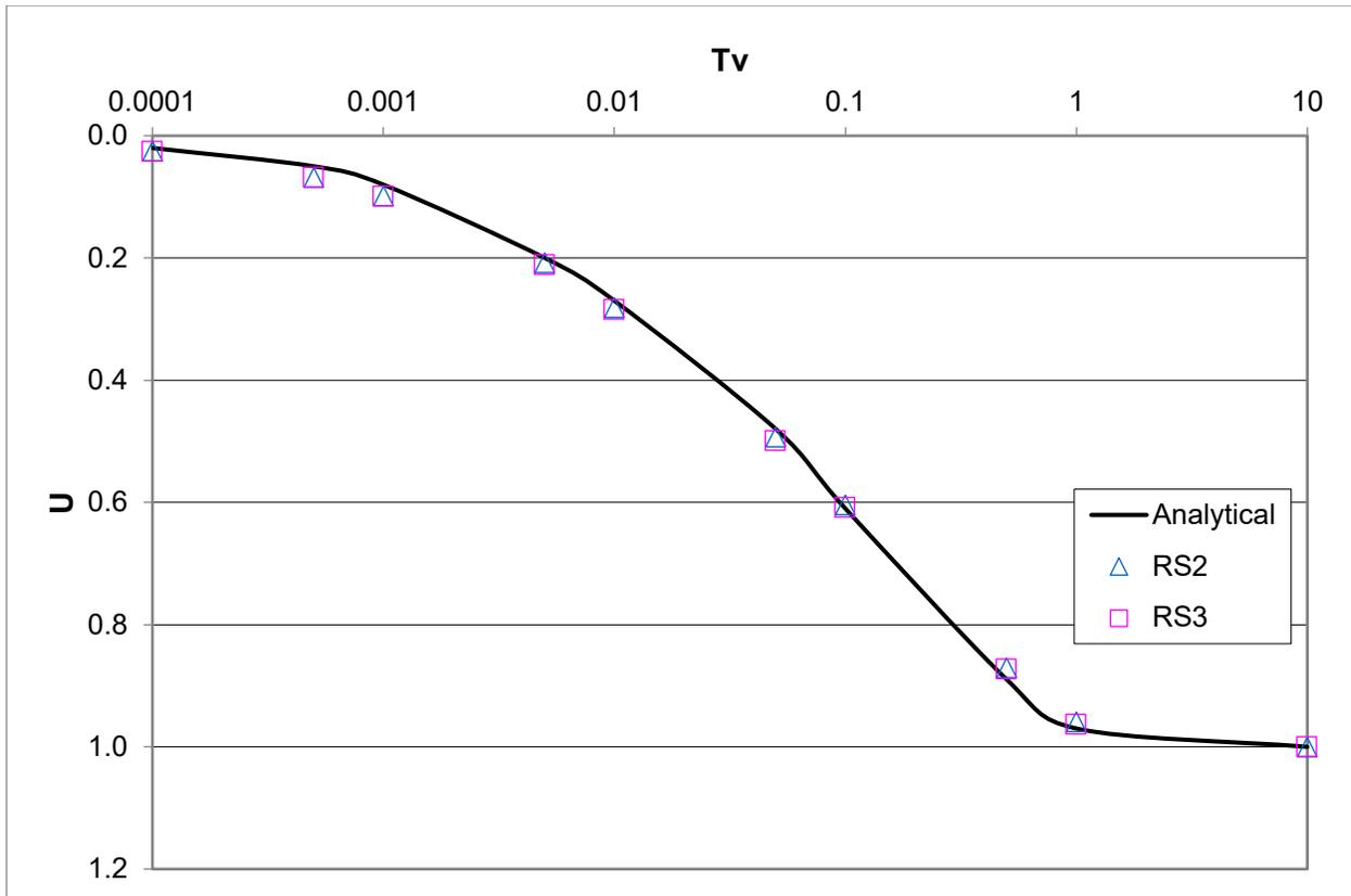
Figure 3-3: Degree of consolidation versus time factor for elastic strip footing
