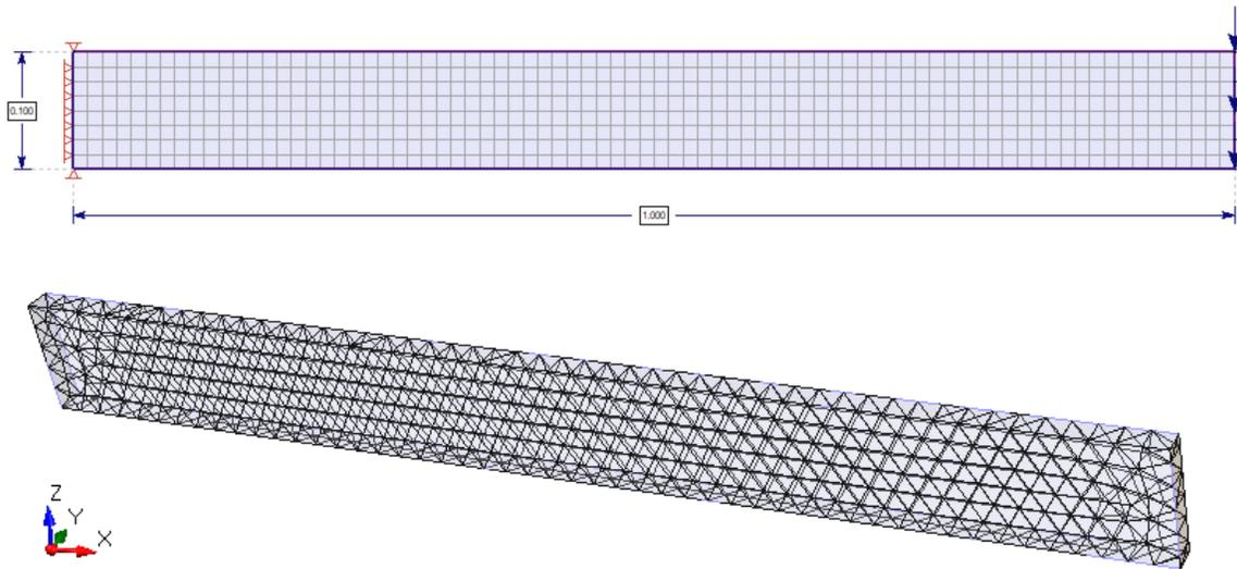
**Figure 4-1:** Cantilever beam modeled in **(top)** RS2 and in **(bottom)** RS3
