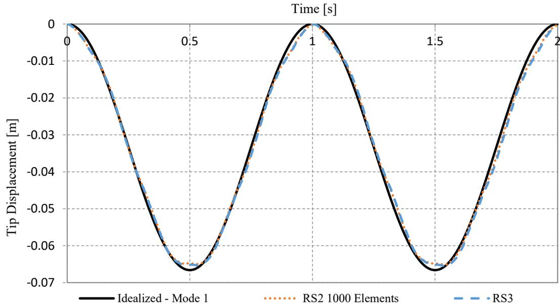
**Figure 4-2:** Cantilever Free End Vertical Displacement Response
