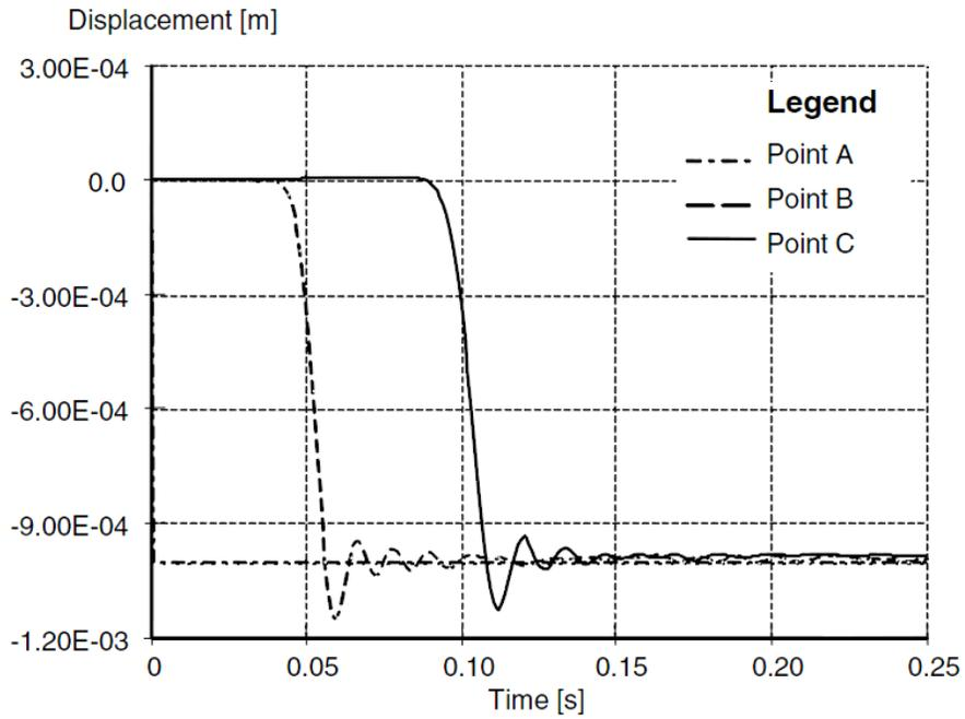
**Figure 6-5:** Displacements-viscous boundary (from Plaxis)
