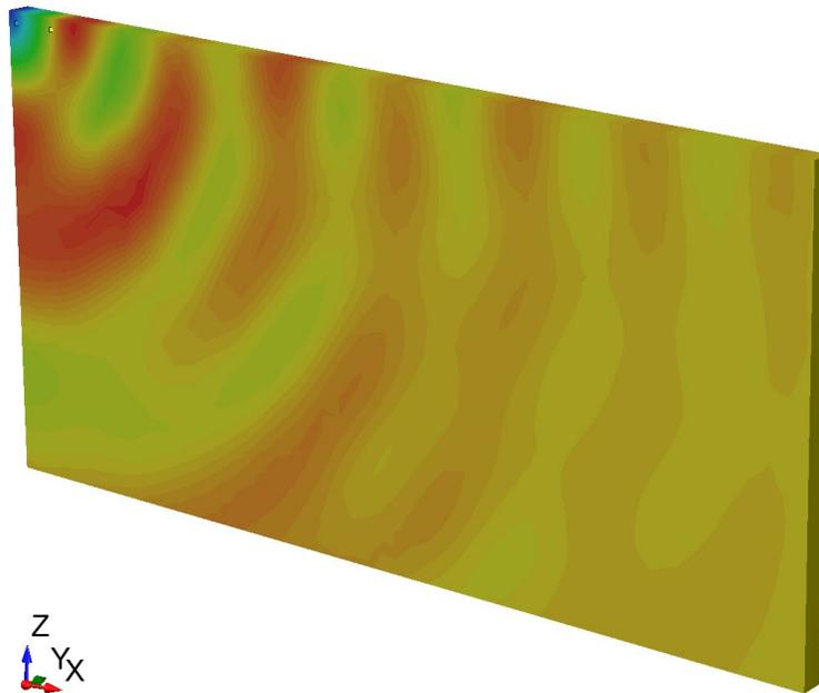
**Figure 10-2:** Vertical Displacement Results in RS3 for  $a_0=2.5$
