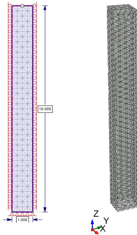
**Figure 1-1:** Soil column as constructed in **(left)** RS2 and in **(right)** RS3
