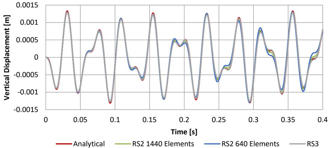
**Figure 2-2:** Vertical Displacement Response of the Midspan of the Beam
