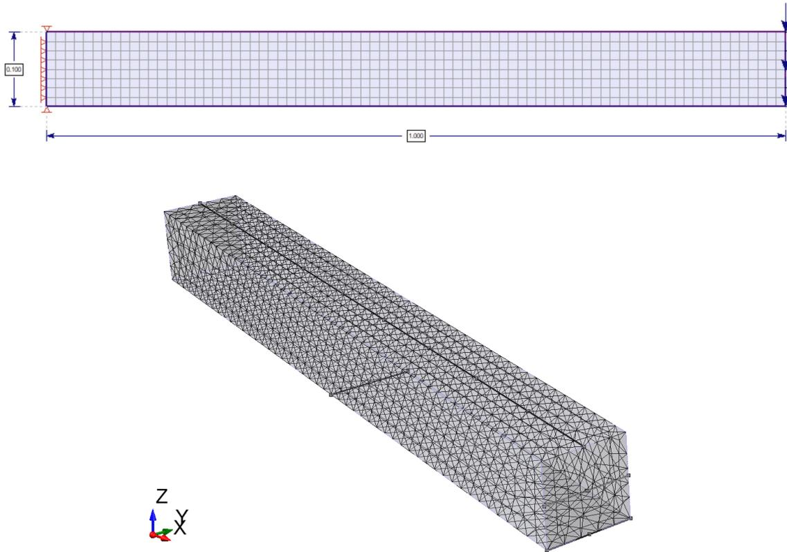
**Figure 3-1:** Cantilever beam modeled in **(top)** RS2 and in **(bottom)** RS3
