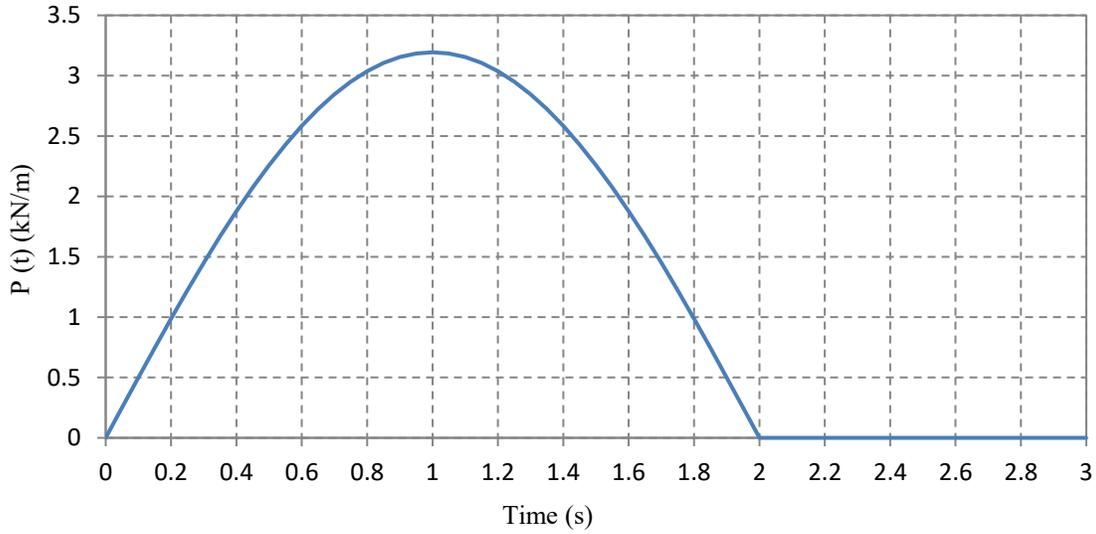
**Figure 3-2:** Harmonic load acting on the beam
