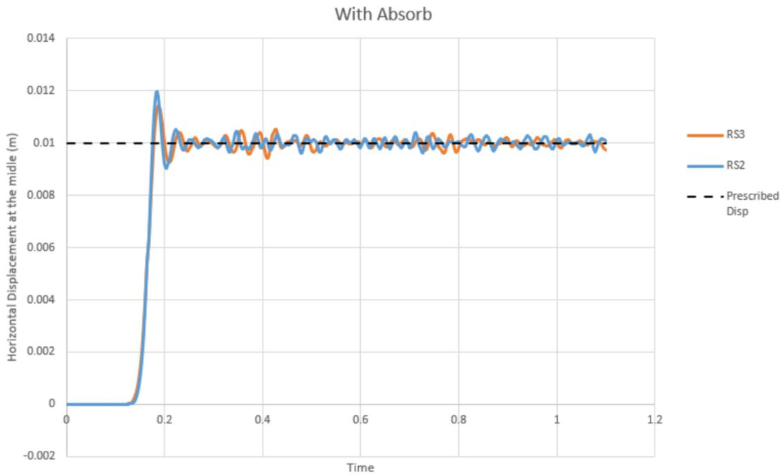
**Figure 6-3:** Displacement at the middle of the soil column-absorb boundary condition
