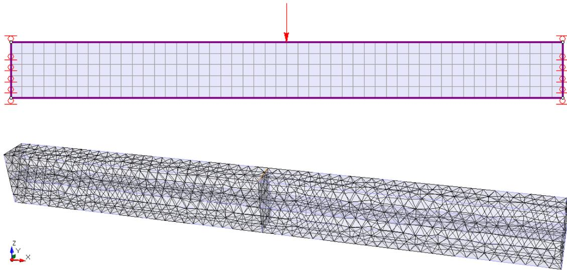
**Figure 2-1:** Simply Supported Beam Modeled in (top) RS2 and in (bottom) RS3
