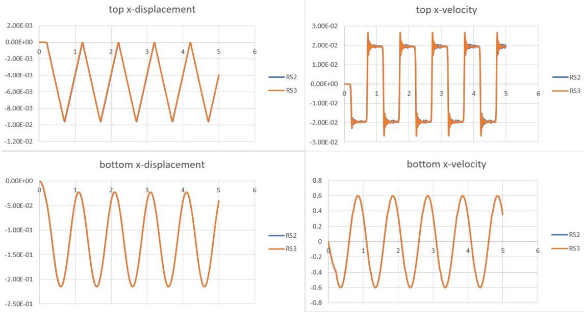
**Figure 8-3:** Comparison of horizontal displacement and velocity on top and bottom of the soil column for both RS2 and RS3 for the case of cohesion=0.1 MPa
