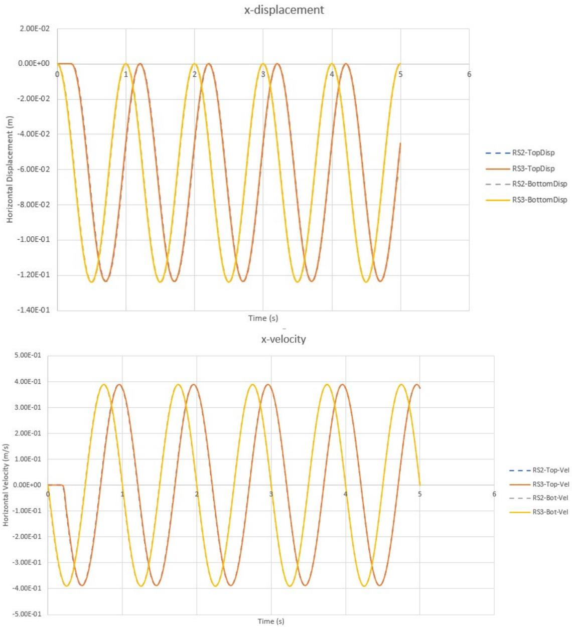
**Figure 8-2:** Comparison of horizontal displacement and velocity on top and bottom of the soil column for both RS2 and RS3 for the case of no slip
