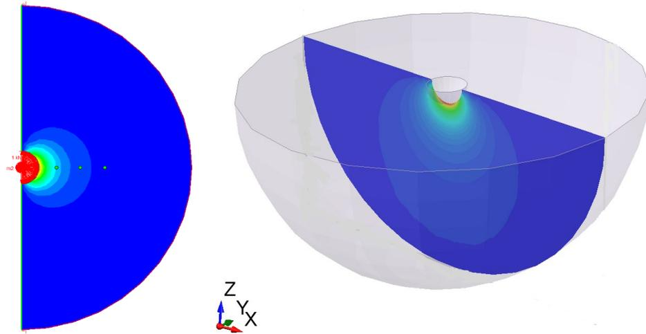
**Figure 9-2: (left) Horizontal displacement in RS2 and (right) Vertical displacement in RS3**
