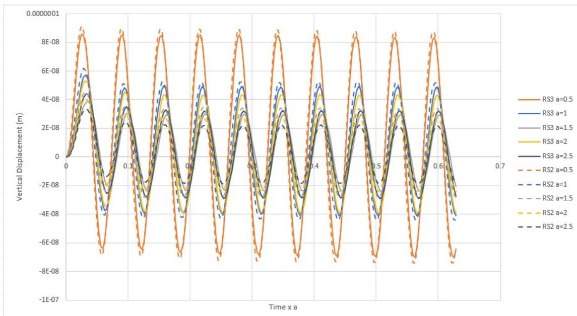
**Figure 10-3:** Comparison of vertical displacement between RS2 and RS3 for five study cases
