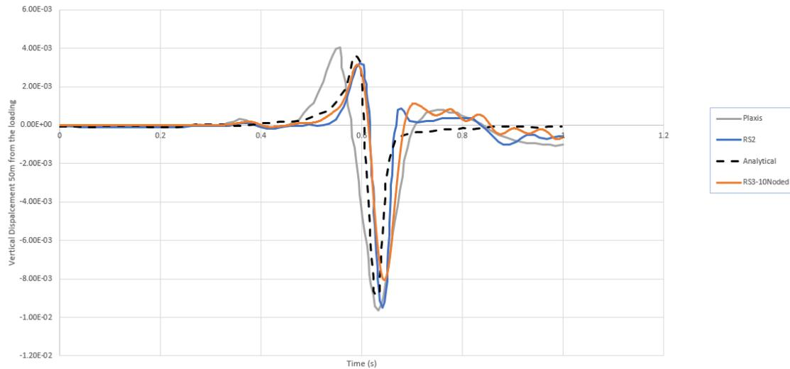
Figure 7-2: Vertical Displacement at x = 50m
