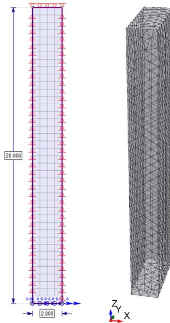
Figure 6-1: Model of a soil column in (left) RS2 and in (right) RS3
