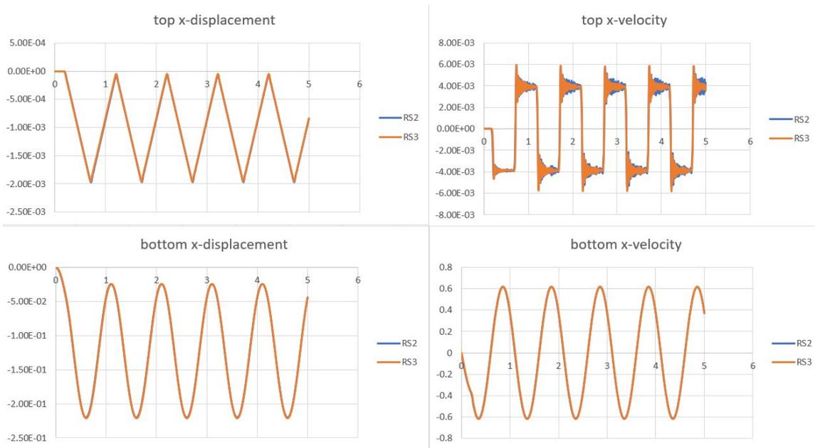
**Figure 8-4:** Comparison of horizontal displacement and velocity on top and bottom of the soil column for both RS2 and RS3 for the case of cohesion=0.02 MPa
