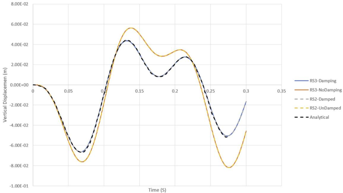
Figure 5-2: Damped and Un-Damped Displacement Response using Dashpot Dampers
