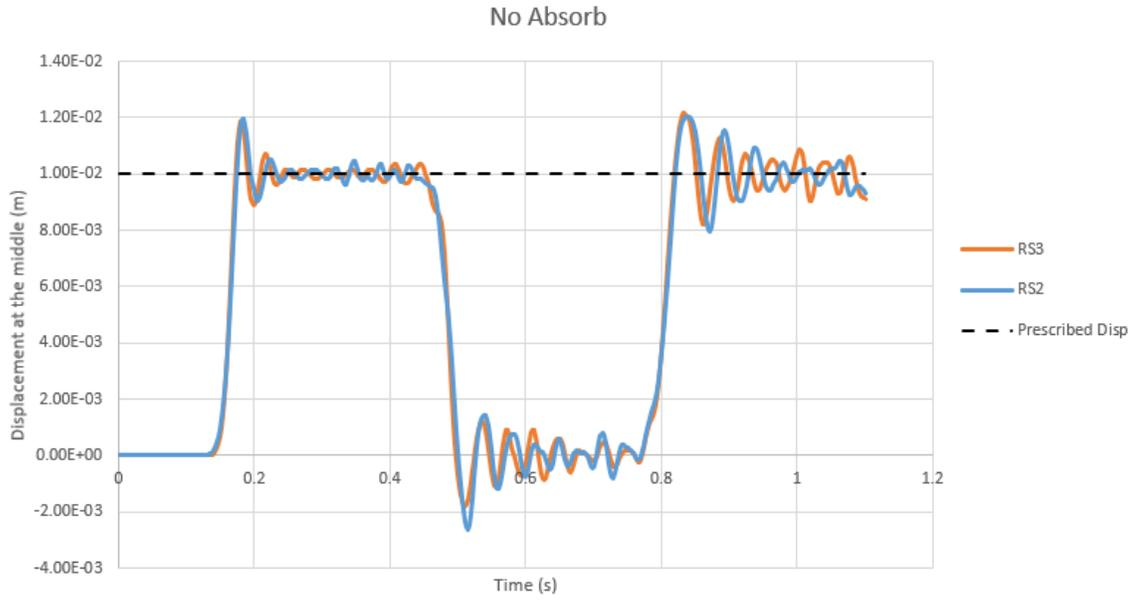
**Figure 6-2:** Displacement at the middle of the soil column-undamped fixed boundary
