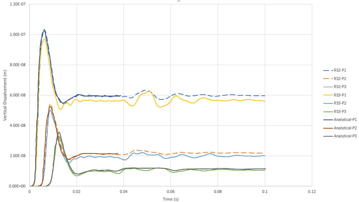
**Figure 9-3: Vertical-displacement vs time at different time queries in comparison with the RS2 and analytical Solution by Blake (1952)**
