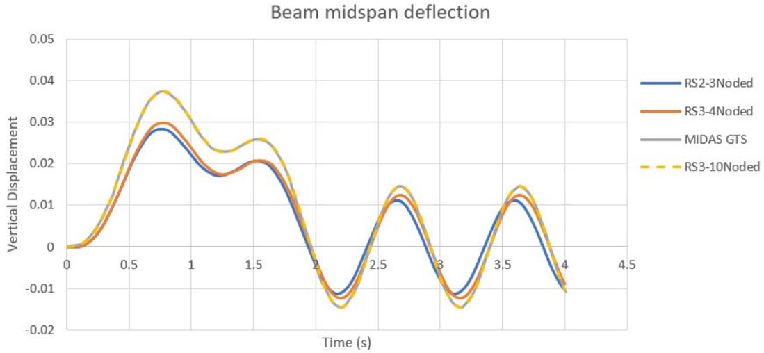
**Figure 3-3:** Midspan Displacement Response
