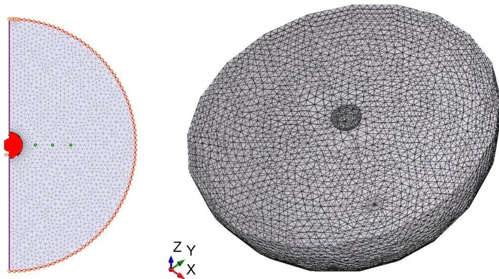
**Figure 9-1:** (left) axi-symmetric RS2 model (right) RS3 Model Geometry
