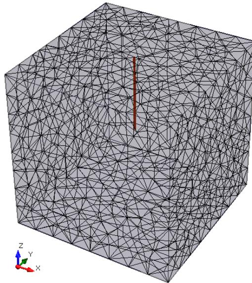
**Figure 6-1: Plain strand cable rockbolt as modeled in RS3**
