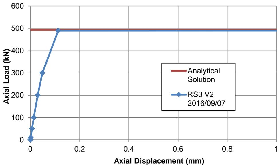
**Figure 6-3: Load-displacement response of piles considering skin resistance and end-bearing effects**
