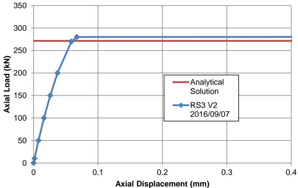
**Figure 6-2: Load-displacement response of piles considering only skin resistance**
