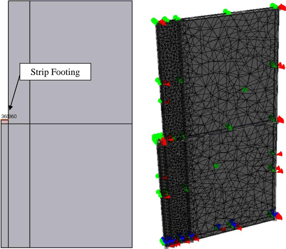
**Figure 13-1: Strip footing in sand as constructed in *RS3***
