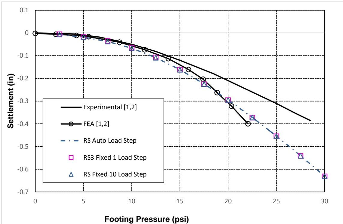
Figure 13-2: Settlement with increasing load as predicted by RS3 and [1]
