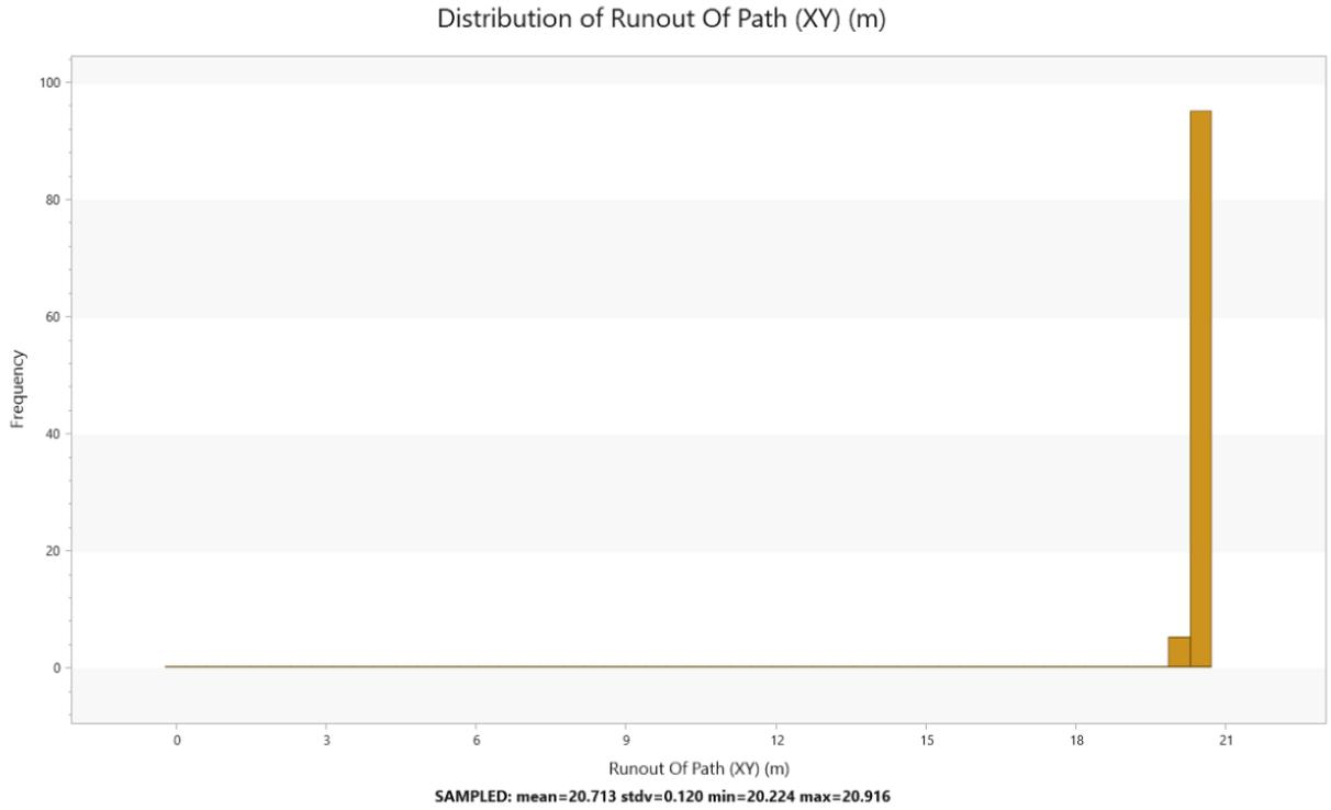
Figure 3-10: RocFall3 Scenario 2 Runout Distance Plot
