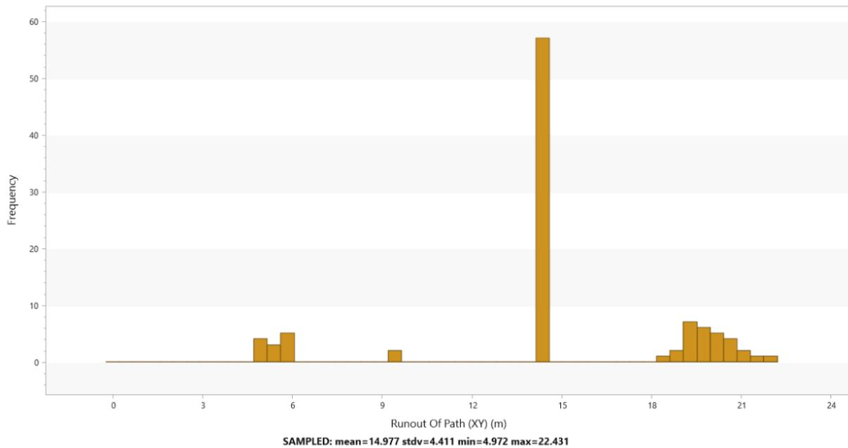
Figure 4-4: RocFall3 Runout Distances Plot
