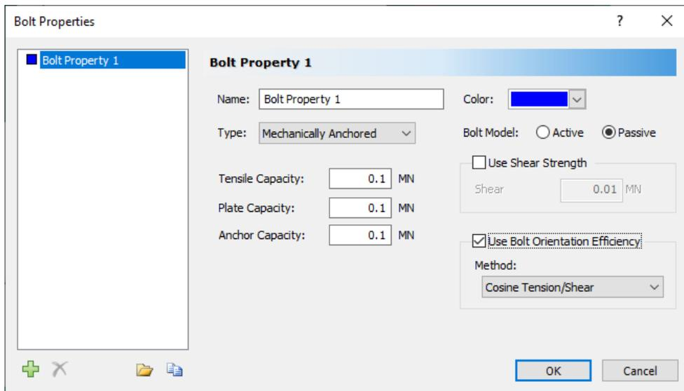
Figure 2.2.3: RocPlane Bolt Properties of Passive Bolt Model with Bolt Orientation Efficiency
