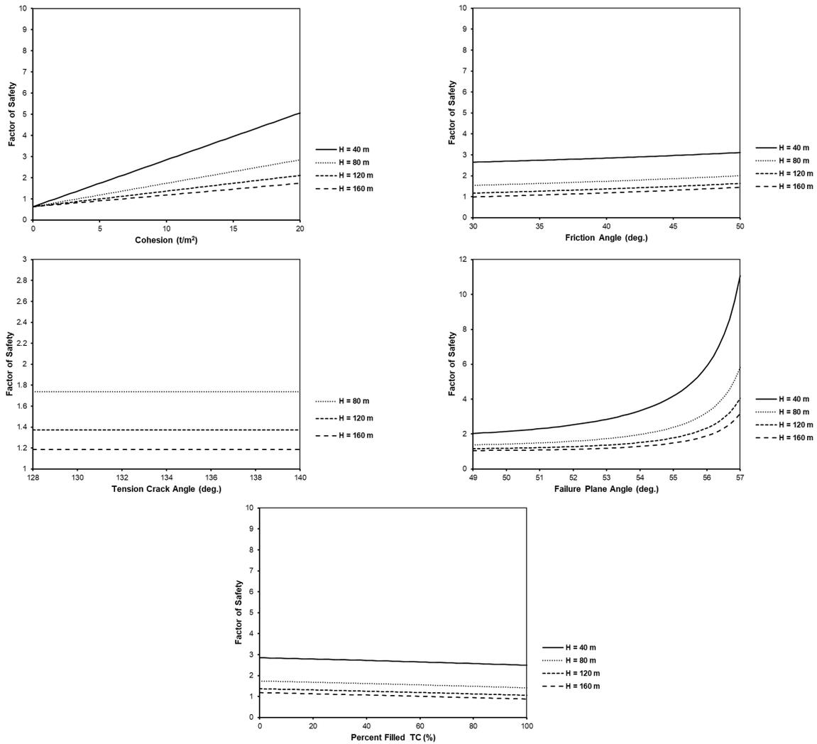
Figure 1.4.4: Sensitivity of Factor of Safety to Various Factors Causing Instability of the Failure Plane, with 0% Water Filled Tension Crack and No Seismic Loading
