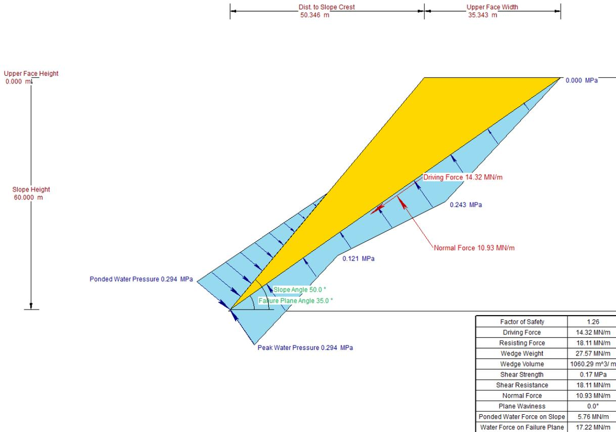
Figure 3.1.5: RocPlane Planar Wedge Stability Analysis Results with Ponded Water and Plane Water
