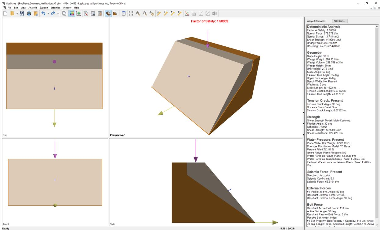
Figure 1.7.5: RocPlane Model with Tension Crack and with Bolt Reinforcement
