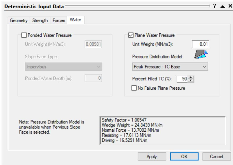
Figure 1.1.13: RocPlane Water Input Data for Slope with No Tension Crack
