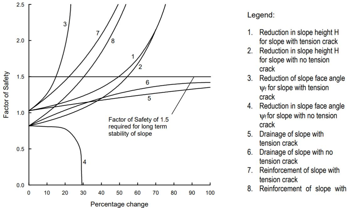
Figure 1.1.19: Evaluation of Remedial Options to Increase the Stability of the Slope by Hoek [1]
