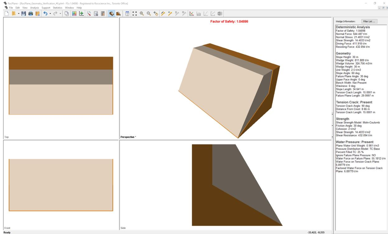
Figure 1.6.2: *RocPlane* Model with Tension Crack
