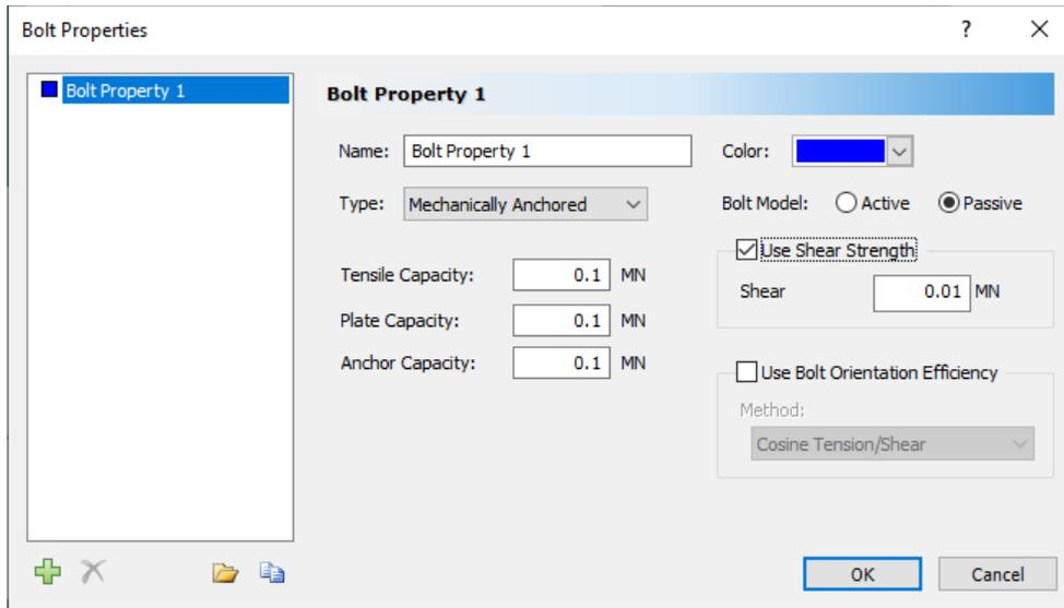
Figure 2.2.4: RocPlane Bolt Properties using Shear Strength
