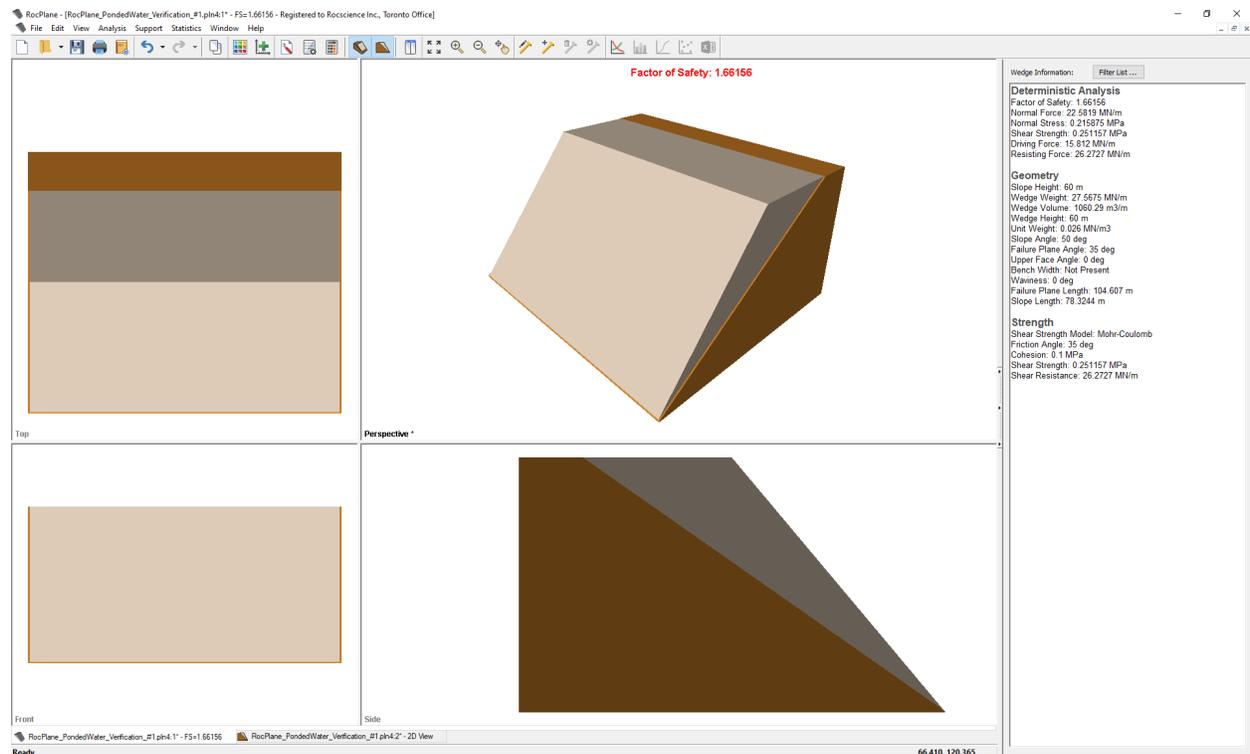
Figure 3.1.1: RocPlane Model with No Water
