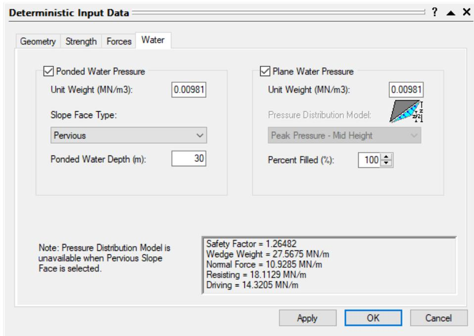
Figure 3.1.2: RocPlane Water Deterministic Input Data with Pounded Water Pressure and Plane Water Pressure
