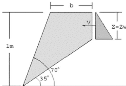
Figure 1.3.1: Plane Geometry of the Unstable Slope
