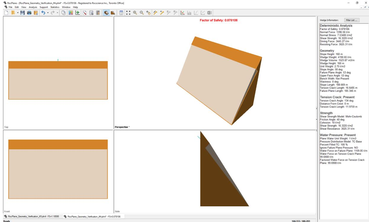
Figure 1.4.2: *RocPlane* Model with Tension Crack ( $c = 10 \text{ t/m}^2$ ,  $H = 160 \text{ m}$ , 100% Filled TC)
