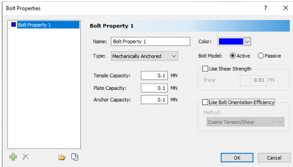
Figure 2.2.2: RocPlane Bolt Properties of Active Bolt Model without Bolt Orientation Efficiency
