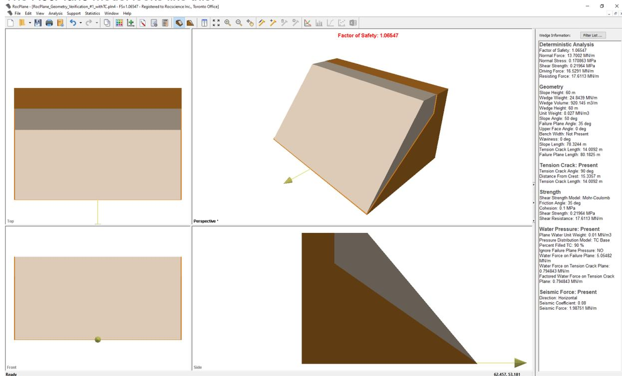
Figure 1.1.14: RocPlane Seismic Model with Tension Crack
