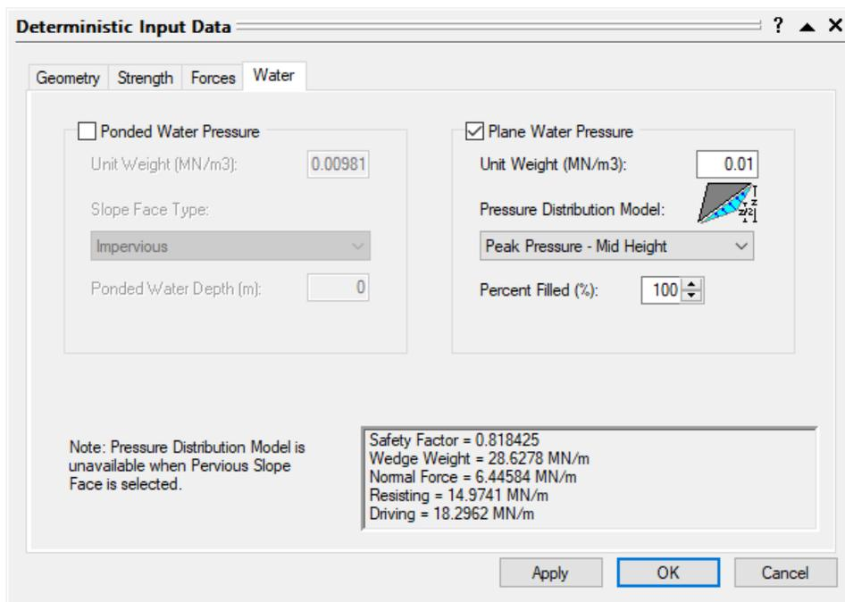
Figure 1.1.7: RocPlane Water Input Data for Slope with No Tension Crack
