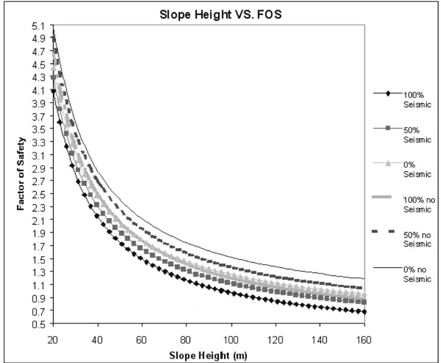
Figure 1.4.5: RocPlane Sensitivity Analysis with Slope Height Varied From 20 m to 160 m
