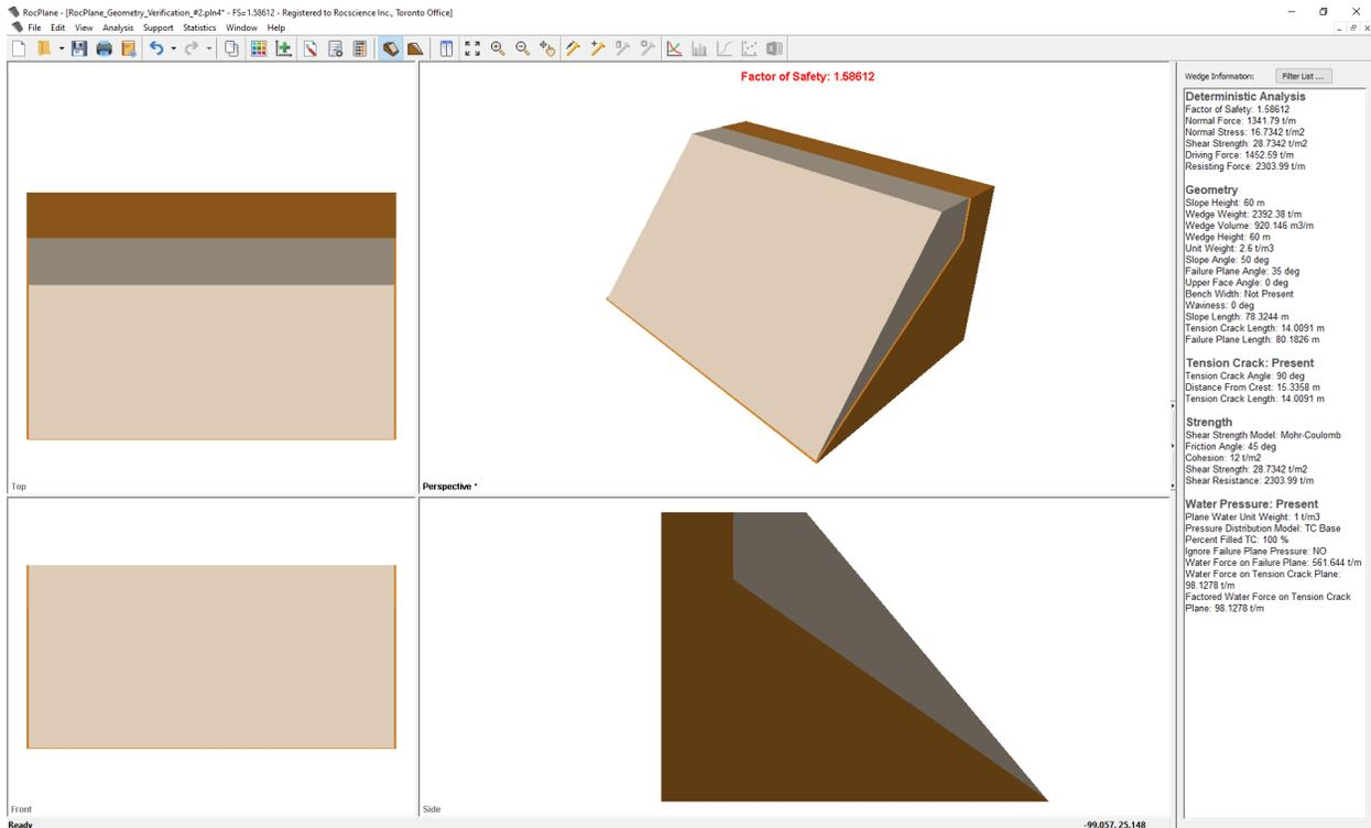
Figure 1.2.1: RocPlane Model with Tension Crack ( $\psi = 0^\circ$ ,  $\theta = 90^\circ$ , 100% Filled Plane Water)
