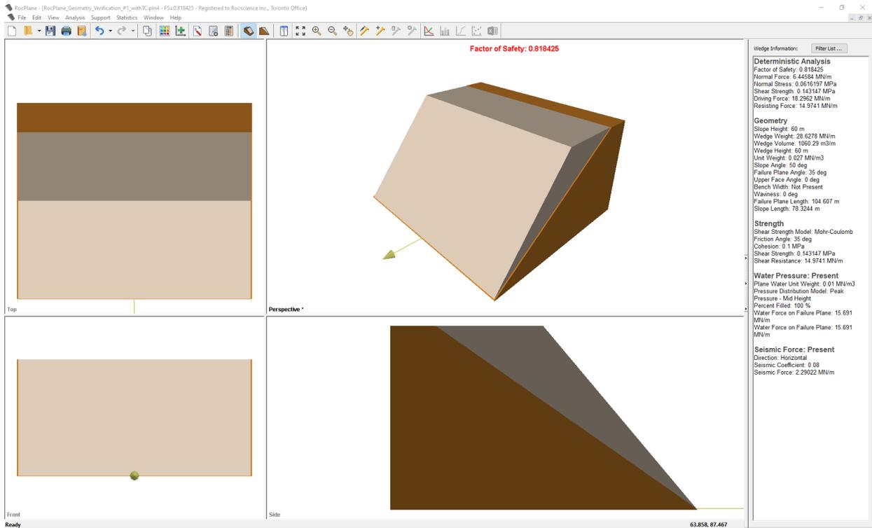
Figure 1.1.8: RocPlane Seismic Model without Tension Crack
