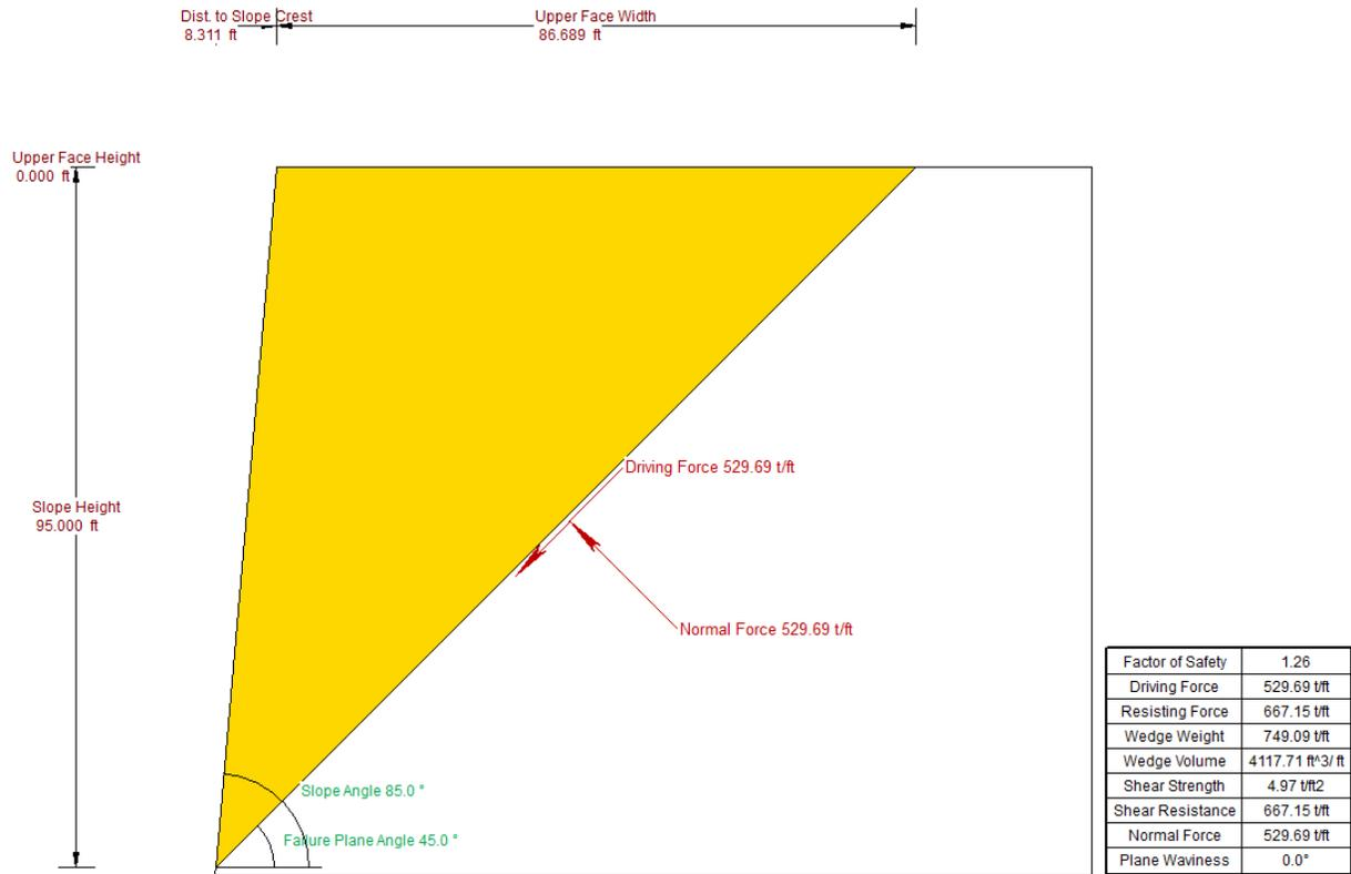
Figure 1.8.5: RocPlane Planar Wedge Analysis (Case 3)
