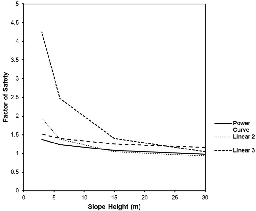
Figure 1.5.3: Sensitivity Plot of FS vs. Slope Height by *RocPlane*
