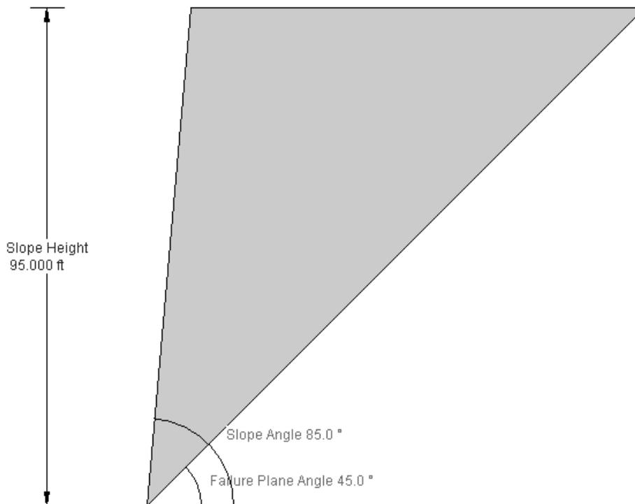
Figure 1.8.1: Geometry of Slope
