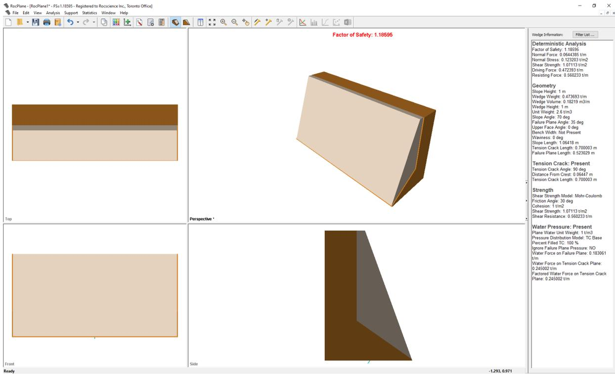
Figure 1.3.2: *RocPlane* Model with Tension Crack ( $b = 0.06447$  m,  $c = 1$  t/m<sup>2</sup>)
