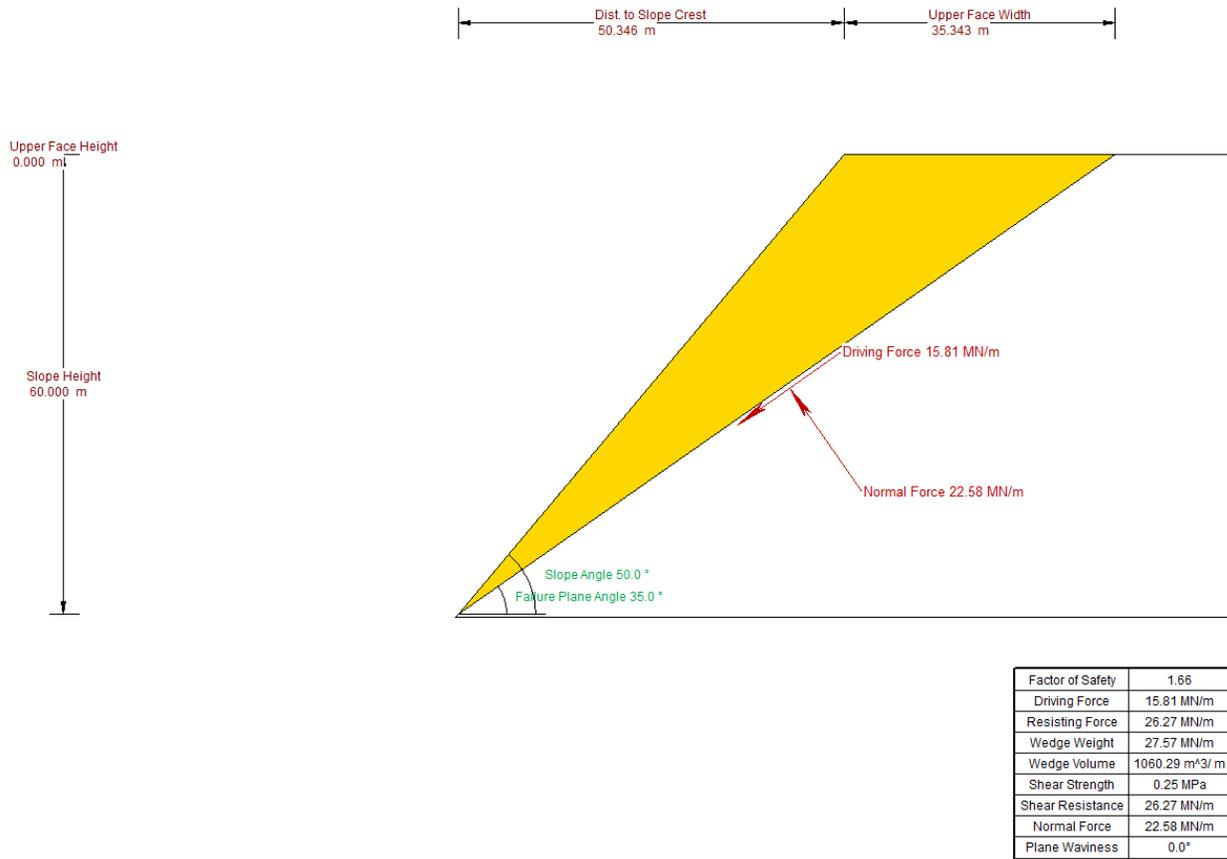
Figure 3.1.4: *RocPlane* Planar Wedge Stability Analysis Results with No Water
