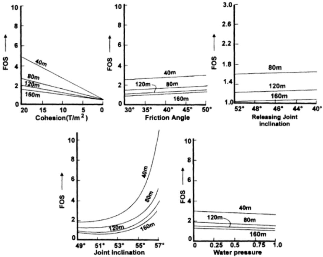
Figure 1.4.3: Sensitivity of FS to Various Factors Causing Instability of the Failure Plane by Sharma [4]
