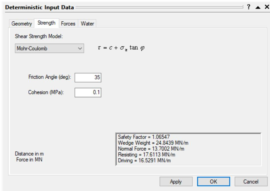
Figure 1.1.11: RocPlane Strength Input Data for Slope with Tension Crack
