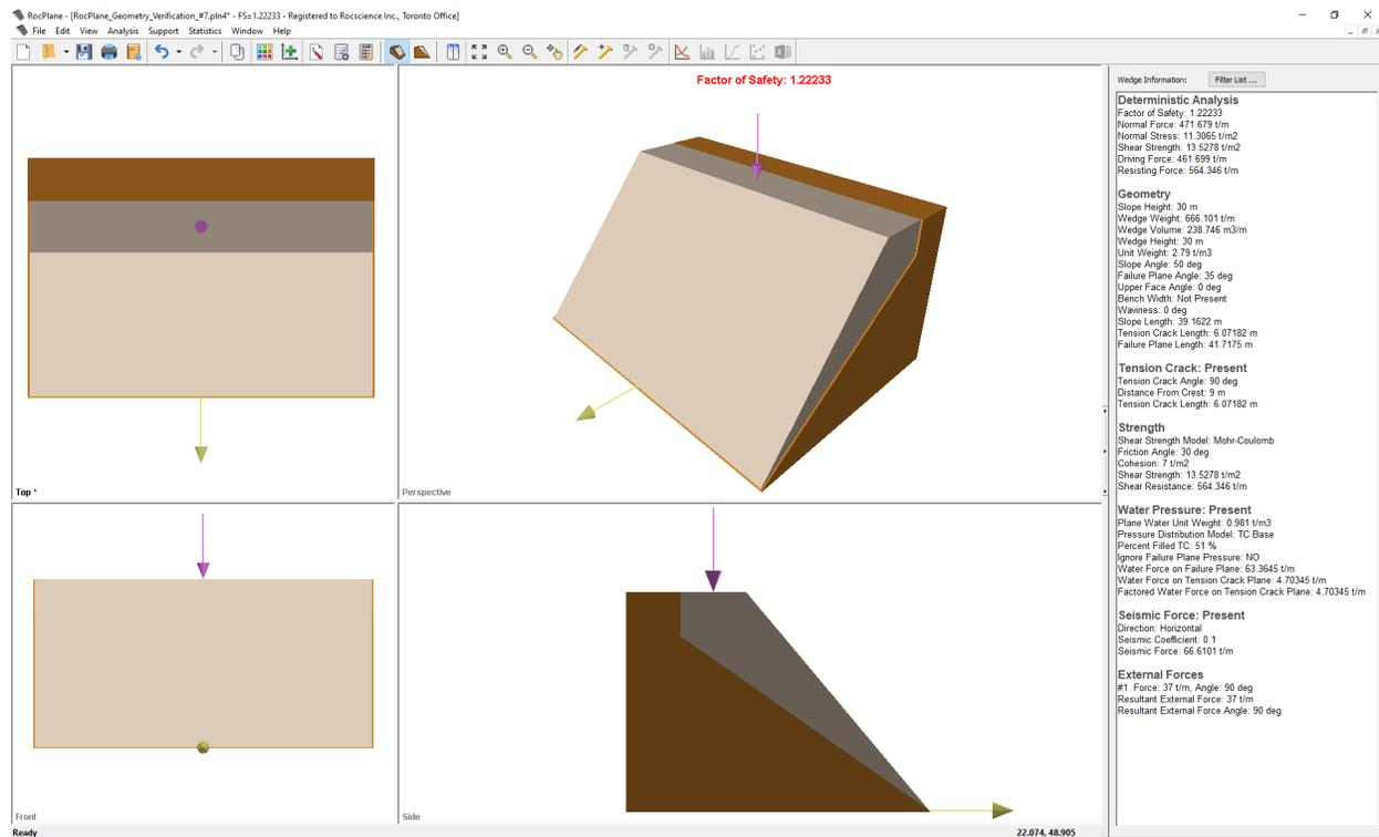
Figure 1.7.2: *RocPlane* Model with Tension Crack and No Bolt Reinforcement
