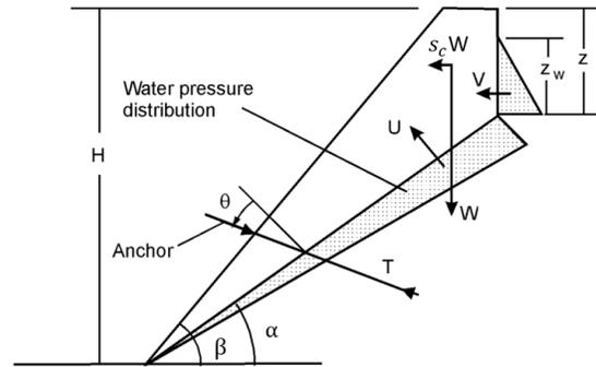
Figure 1.1.3: Slope with Tension Crack [1]
