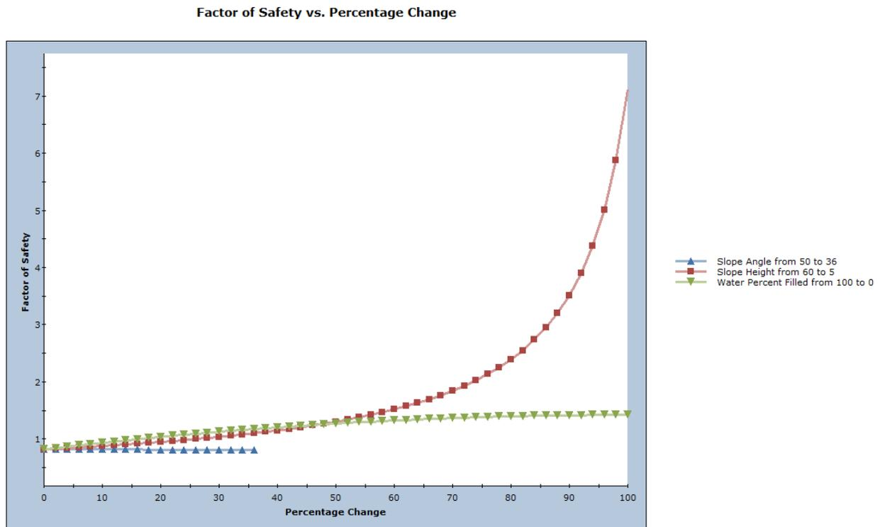
Figure 1.1.16: *RocPlane* Sensitivity Plot of Slope without Tension Crack
