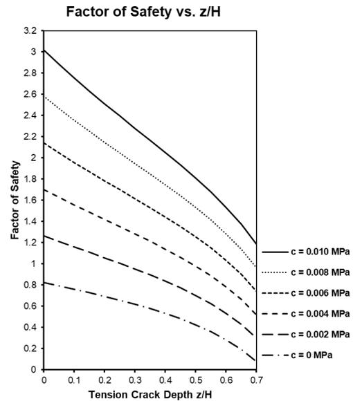
Figure 1.3.4: Factor of Safety vs. Z/H with Values Calculated Using *RocPlane*
