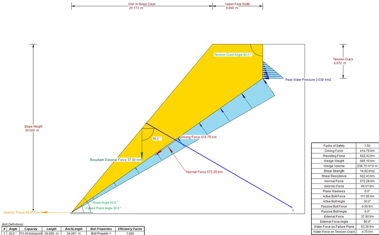
Figure 1.7.6: RocPlane Reinforced Planar Wedge Analysis
