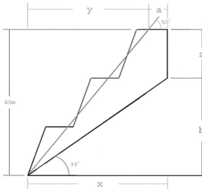
Figure 1.1.9: Geometry of the Slope with Tension Crack
