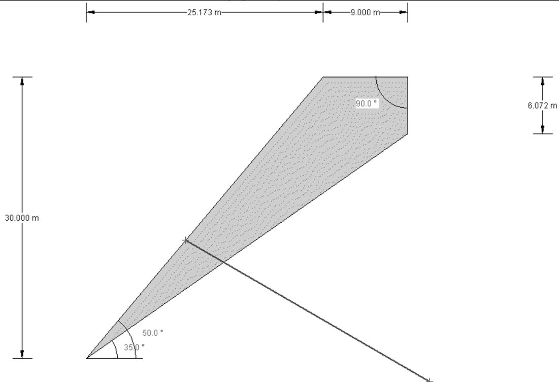
Figure 1.7.1: Slope Geometry
