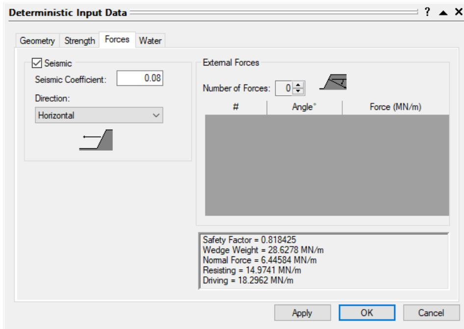
Figure 1.1.6: RocPlane Forces Input Data for Slope with No Tension Crack
