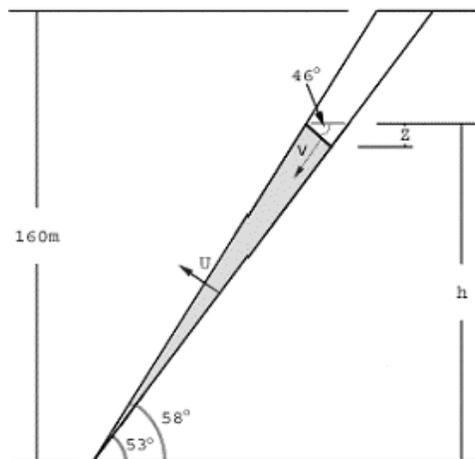
Figure 1.4.1: Geometry of Slope
