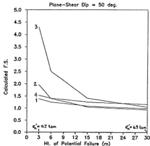
Figure 1.5.2: Sensitivity Plot of FS vs. Slope Height by Miller
