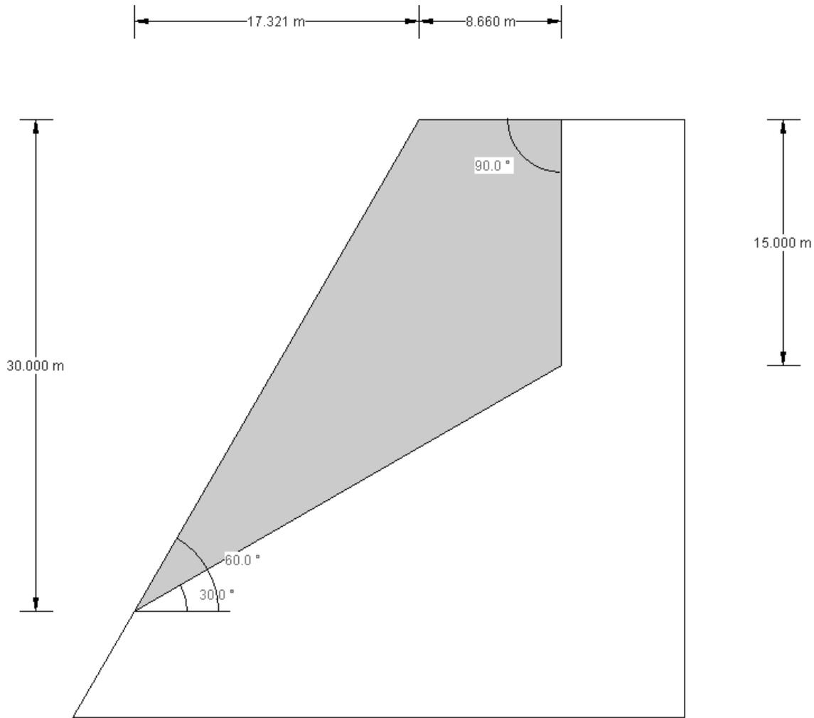
Figure 1.6.1: Slope Geometry
