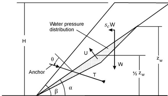
Figure 1.1.2: Slope without Tension Crack [1]
