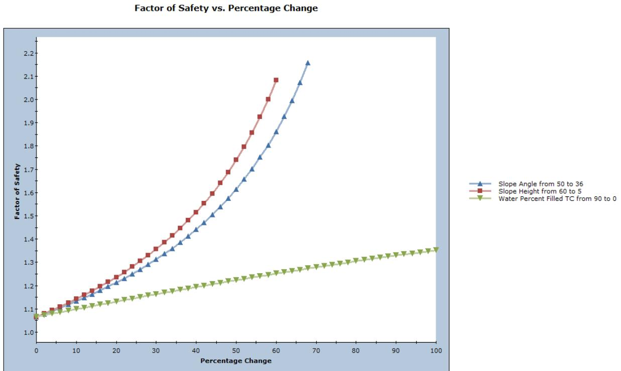
Figure 1.1.18: *RocPlane* Sensitivity Plot of Slope with Tension Crack
