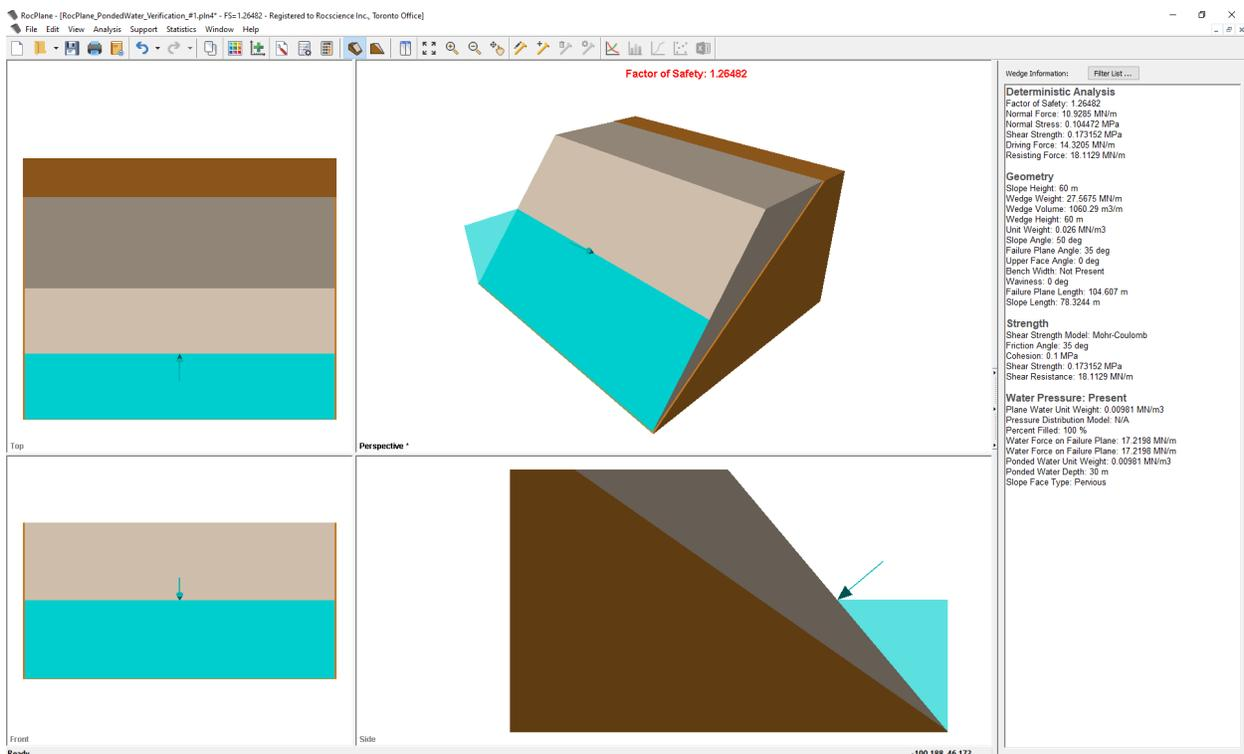
Figure 3.1.3: RocPlane Model with Partially Ponded Slope
