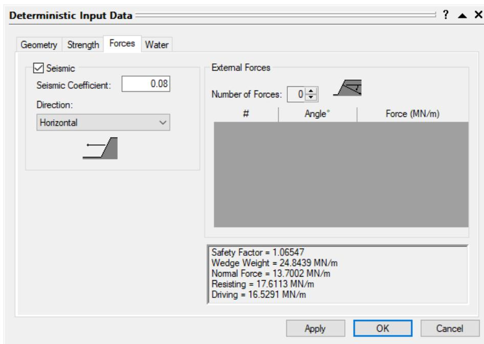
Figure 1.1.12: RocPlane Forces Input Data for Slope with Tension Crack
