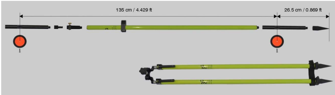
Figure 35: Parts of a Range Pole as they have to be joined together for tunnelling application. Good for tunnel faces up to 15 m.
