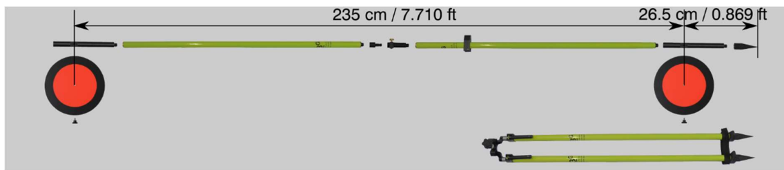
Figure 33: Standard configuration of the Range Pole with a target distance of 235 cm (7.710 ft)
