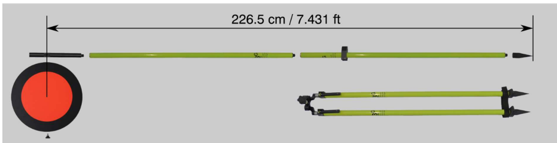
Figure 56: Components of a Highwall Delimiter as they have to be assembled. The target disc is at 226.5 cm (4.15 ft) height.
