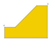
Slope, homogeneous (c-phi material), strength (m-c), probabilistic analysis (overall slope), ru pore pressure, reliability index, circular (grid search)
