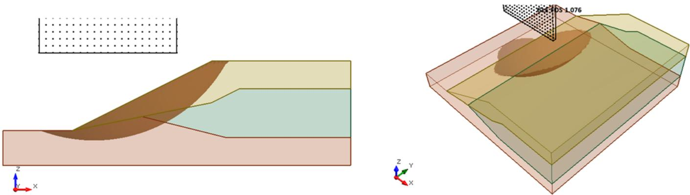
**Figure 5.4.5 – Slide3 Solution Using the GLE Method**
