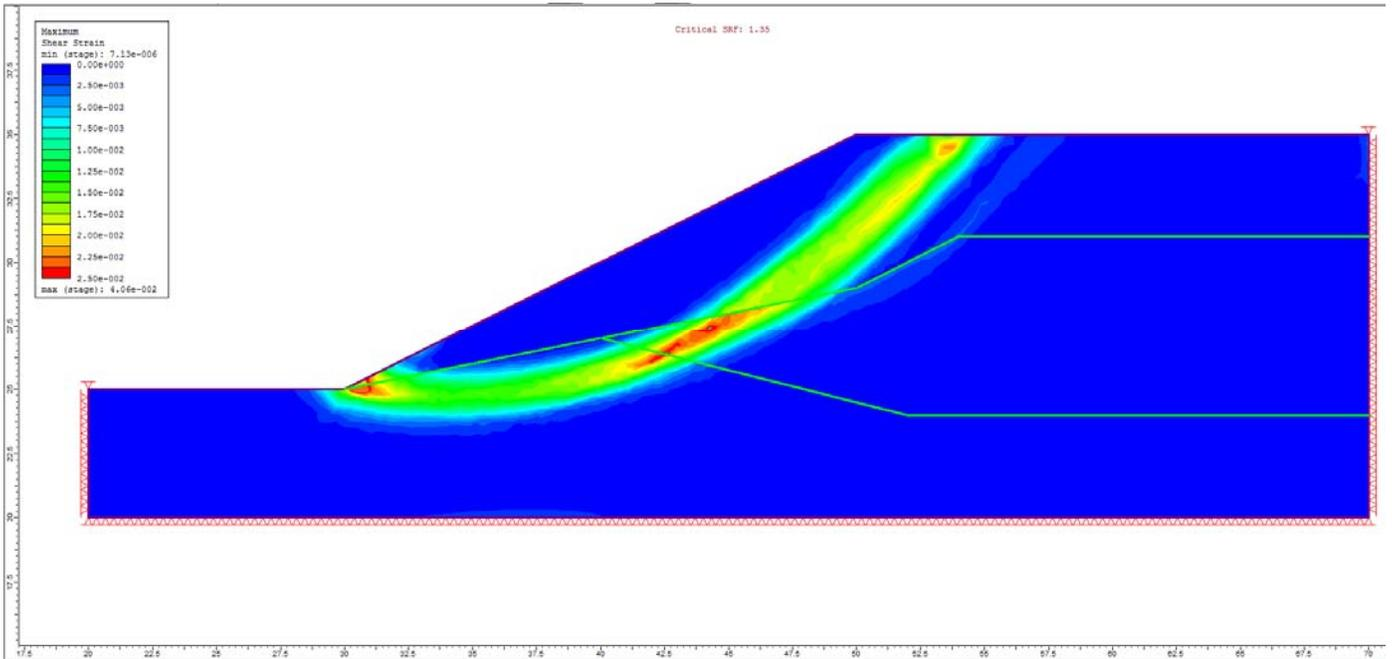
Figure 4.4.7 – RS2 Maximum Shear Strain
