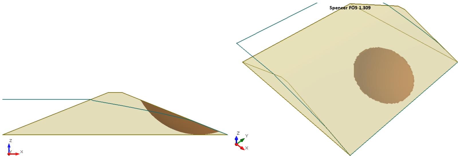
**Figure 30.4.5 – Slide3 Solution Using the Spencer Method**
