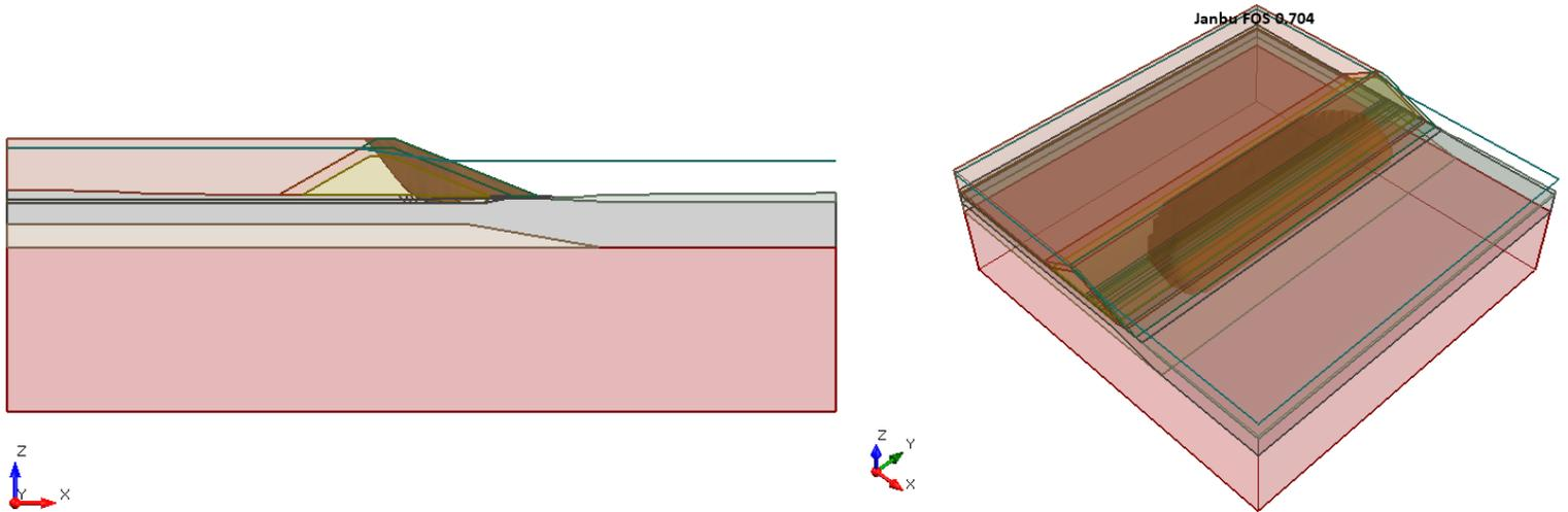
**Figure 45.4.5 – Slide3 Solution Using the Janbu Method**
