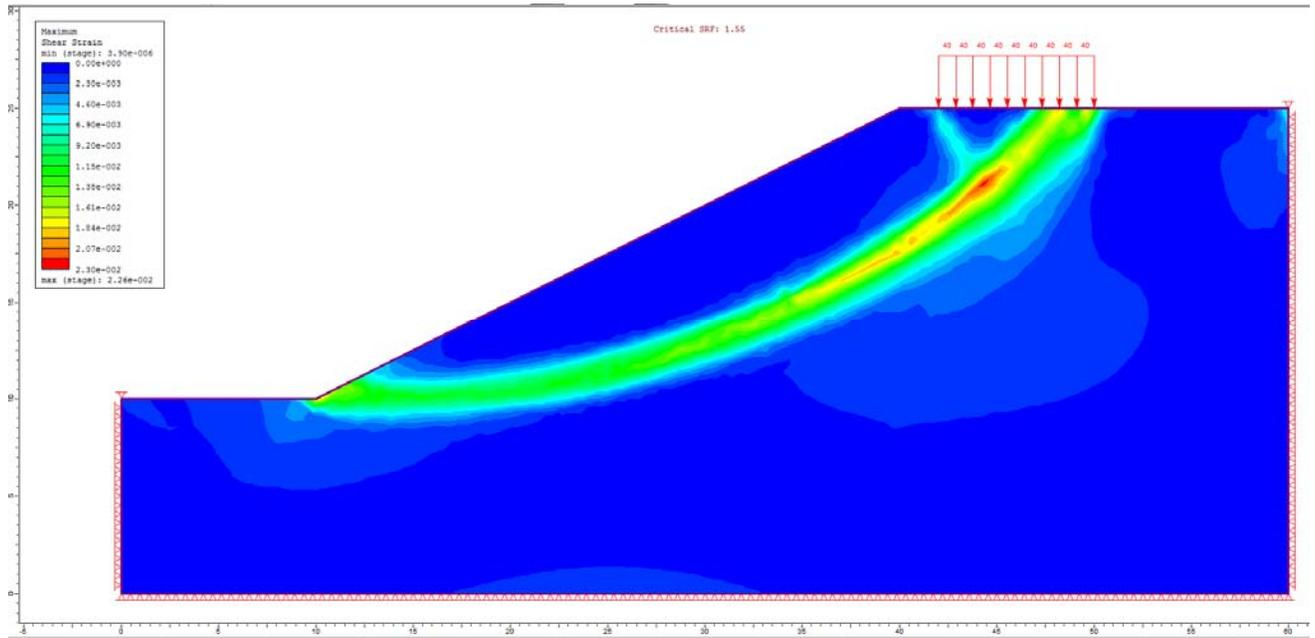
Figure 21.4.9 – RS2 Maximum Shear Strain
