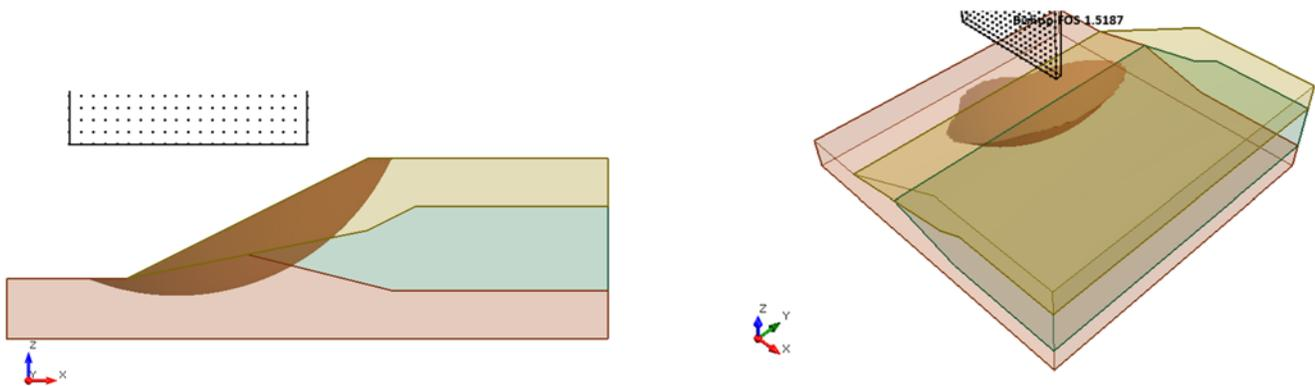
**Figure 3.4.1 – Slide3 Solution Using the Bishop Method**
