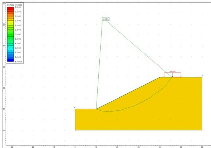
**Figure 21.4.2 – Slide Solution Using the Bishop Method**
