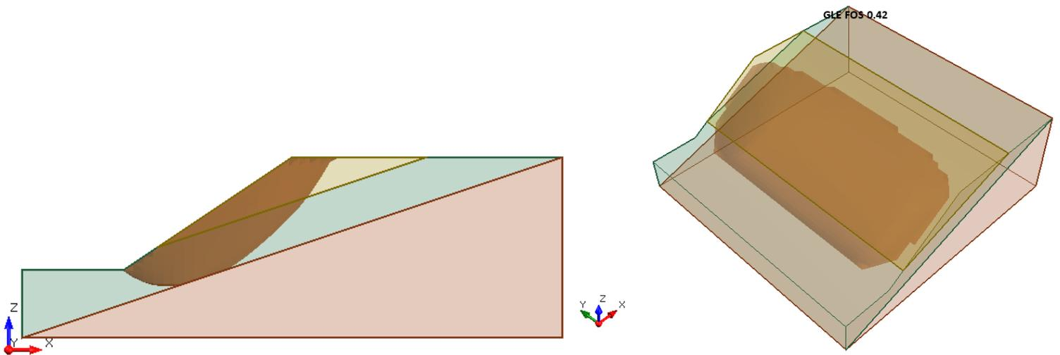
**Figure 11.4.5 – Slide3 Solution Using the GLE Method**
