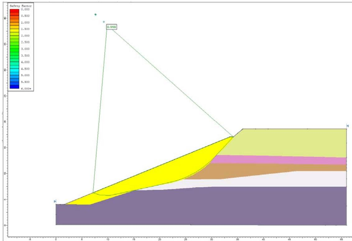
**Figure 44.4.6 – Slide Solution Using the Janbu Method**
