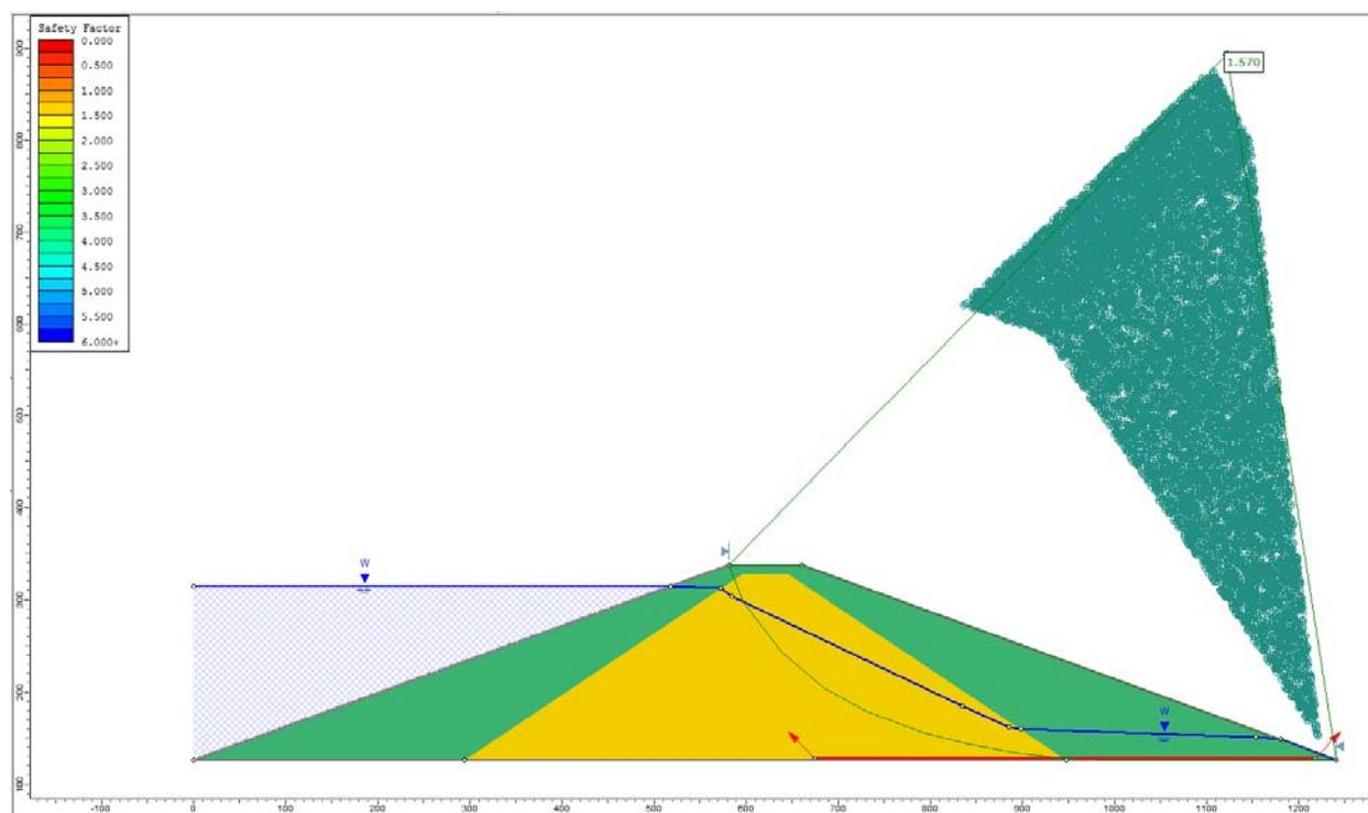
**Figure 33.4.6 – Slide Solution Using the Spencer Method**
