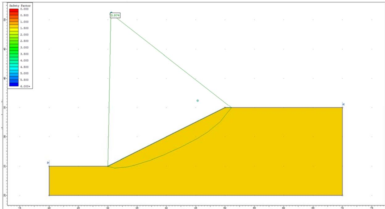
**Figure 2.4.6 – Slide Solution Using the GLE Method**
