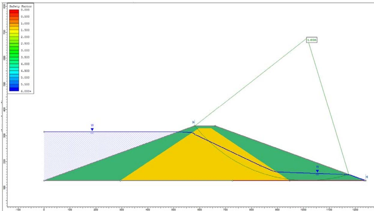
Figure 32.4.4 – Slide Solution Using the GLE Method
