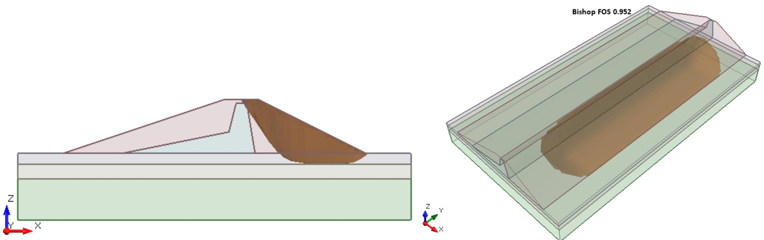
**Figure 40.4.1 – Slide3 Solution Using the Bishop Method**
