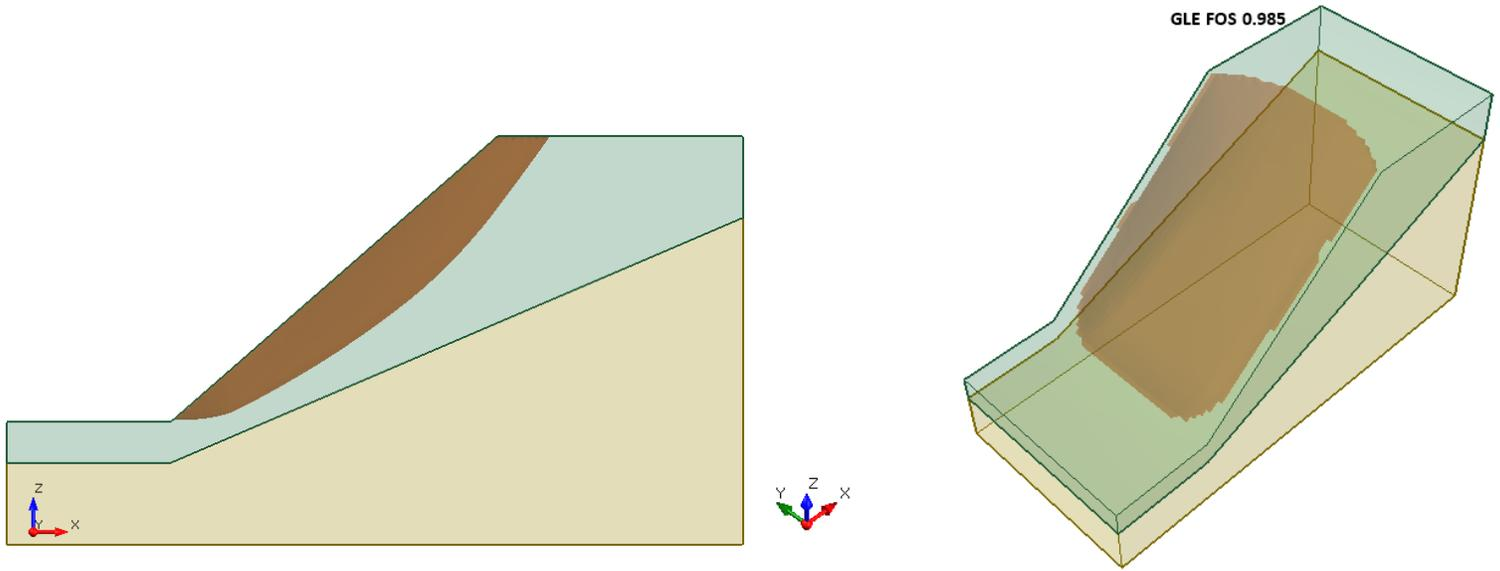
**Figure 17.4.3 – Slide3 Solution Using the GLE Method**
