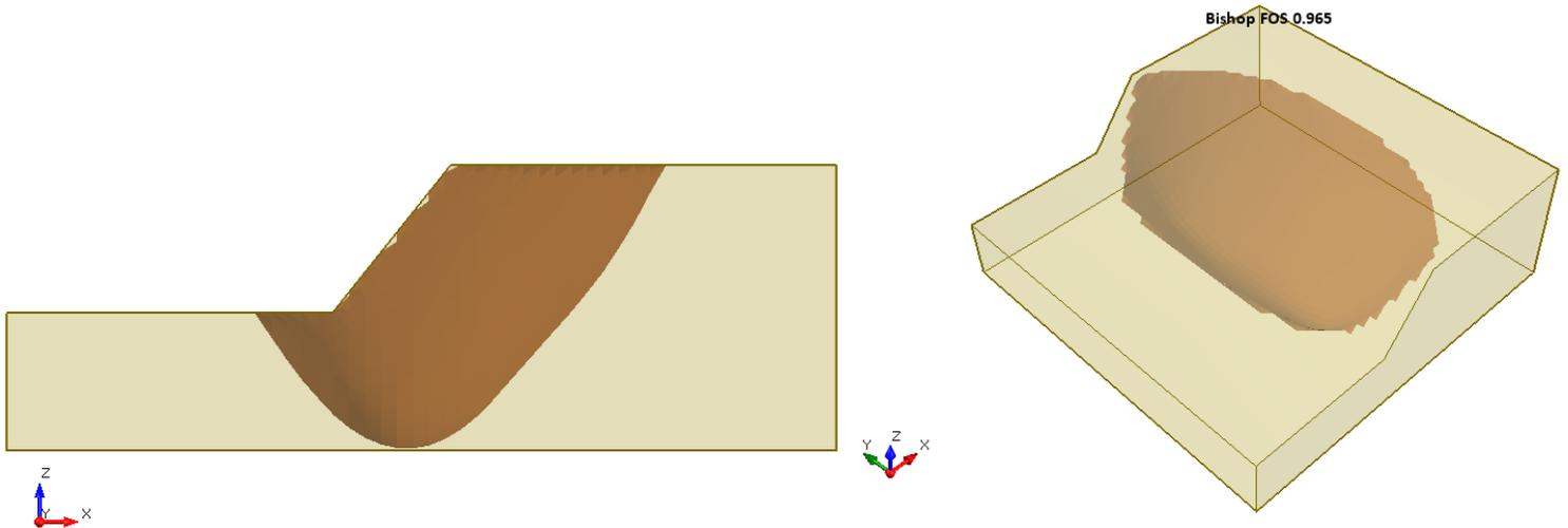
**Figure 37.4.1 – Slide3 Solution Using the Bishop Method**
