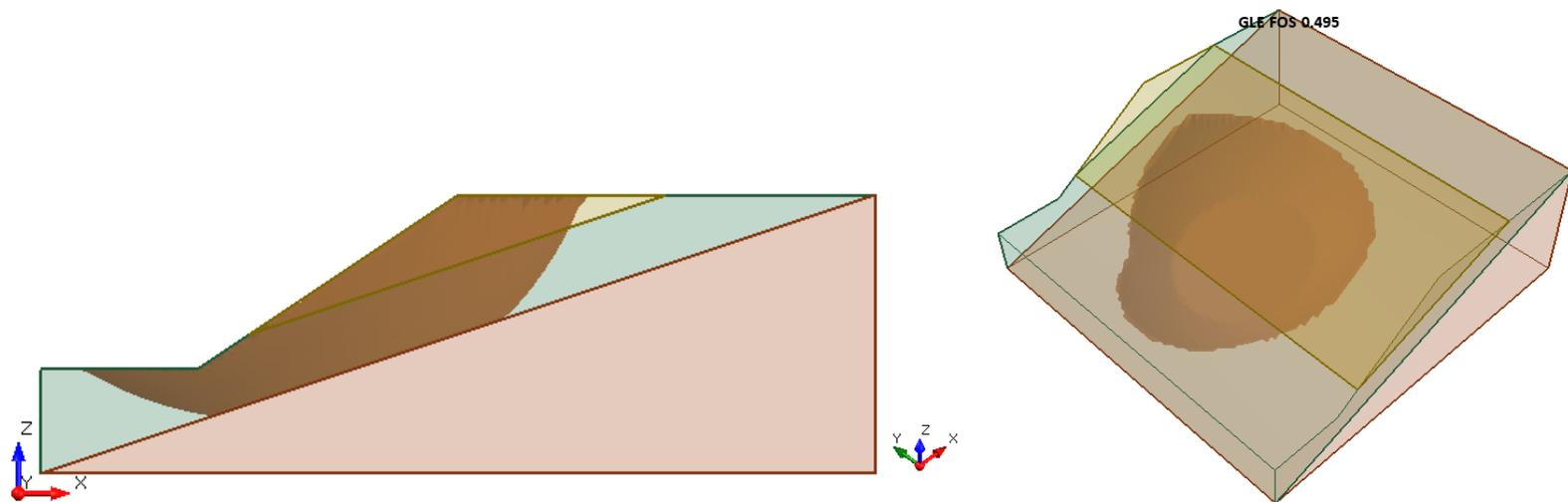
**Figure 10.4.5 – Slide3 Solution Using the GLE Method**
