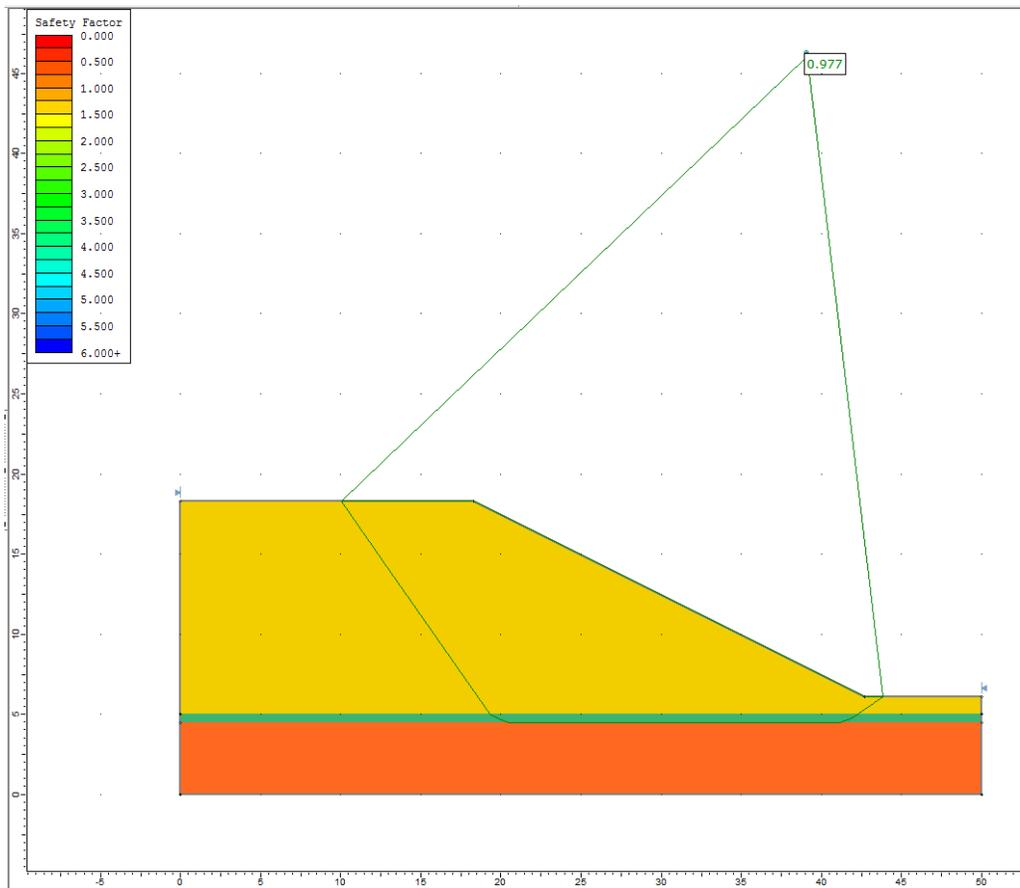
**Figure 15.4.8 – Slide Solution Using the Spencer Method**
