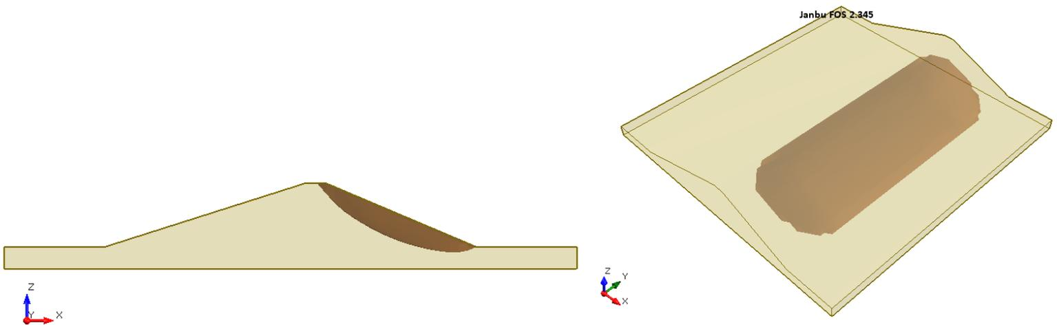
**Figure 12.4.5 – Slide3 Solution Using the Janbu Method**
