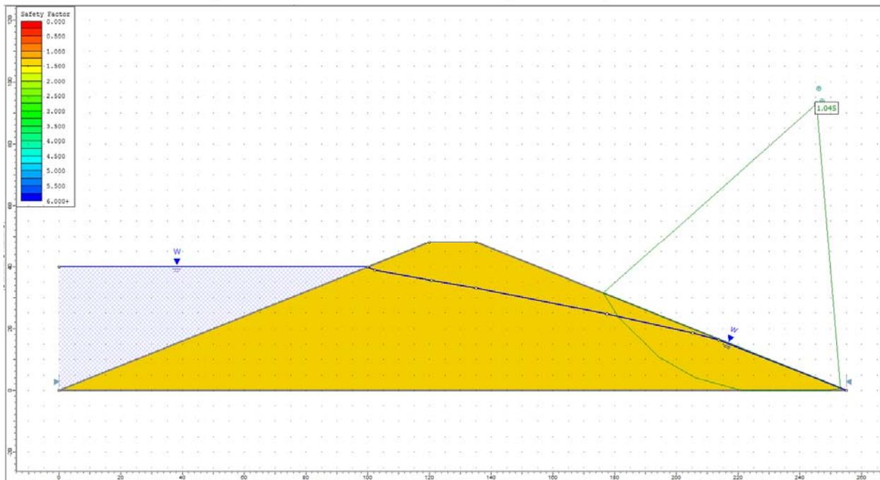
**Figure 31.4.2 – Slide Solution Using the Bishop Method**
