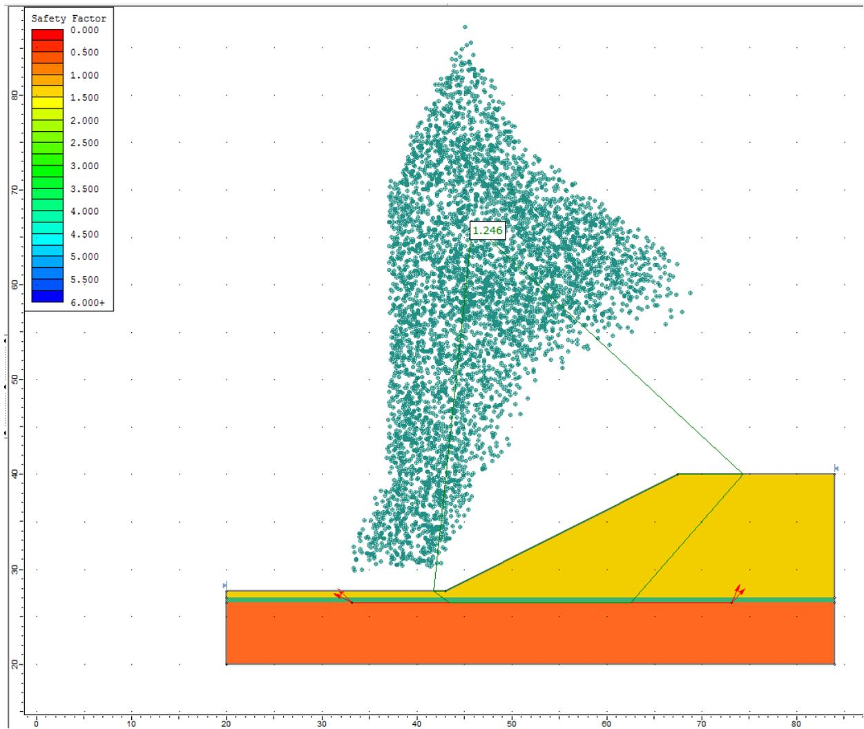
Figure 7.4.6 – Slide Solution Using the GLE Method
