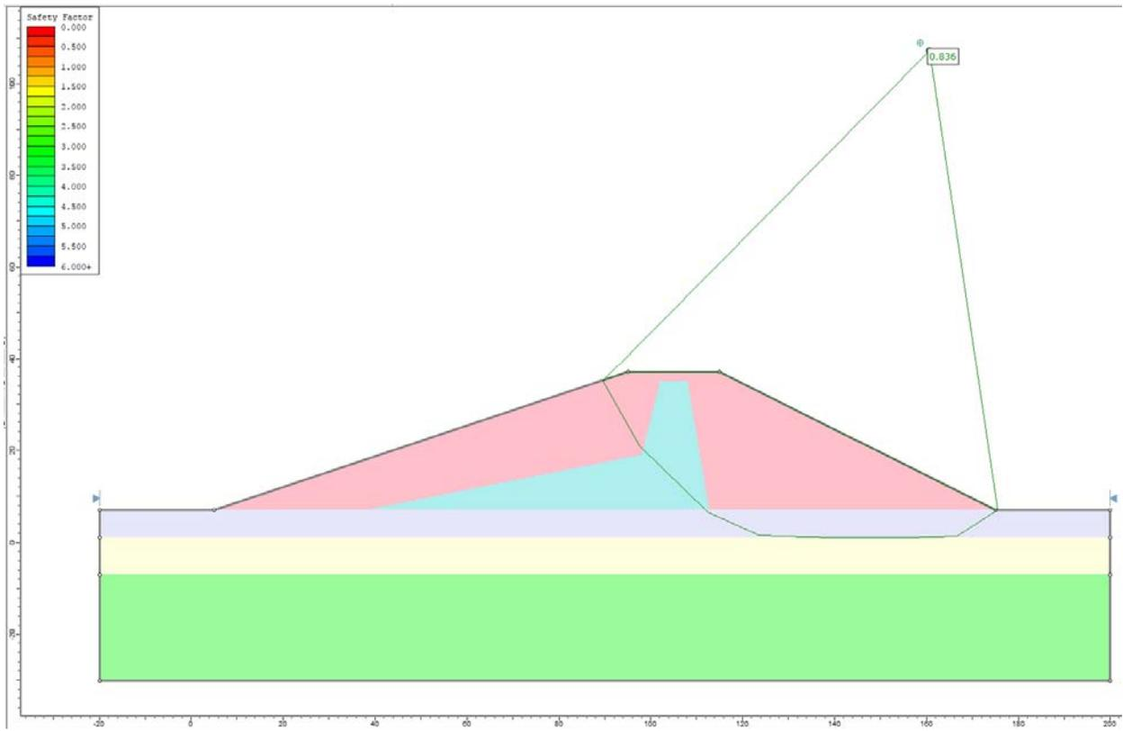
**Figure 40.4.4 – Slide Solution Using the GLE Method**
