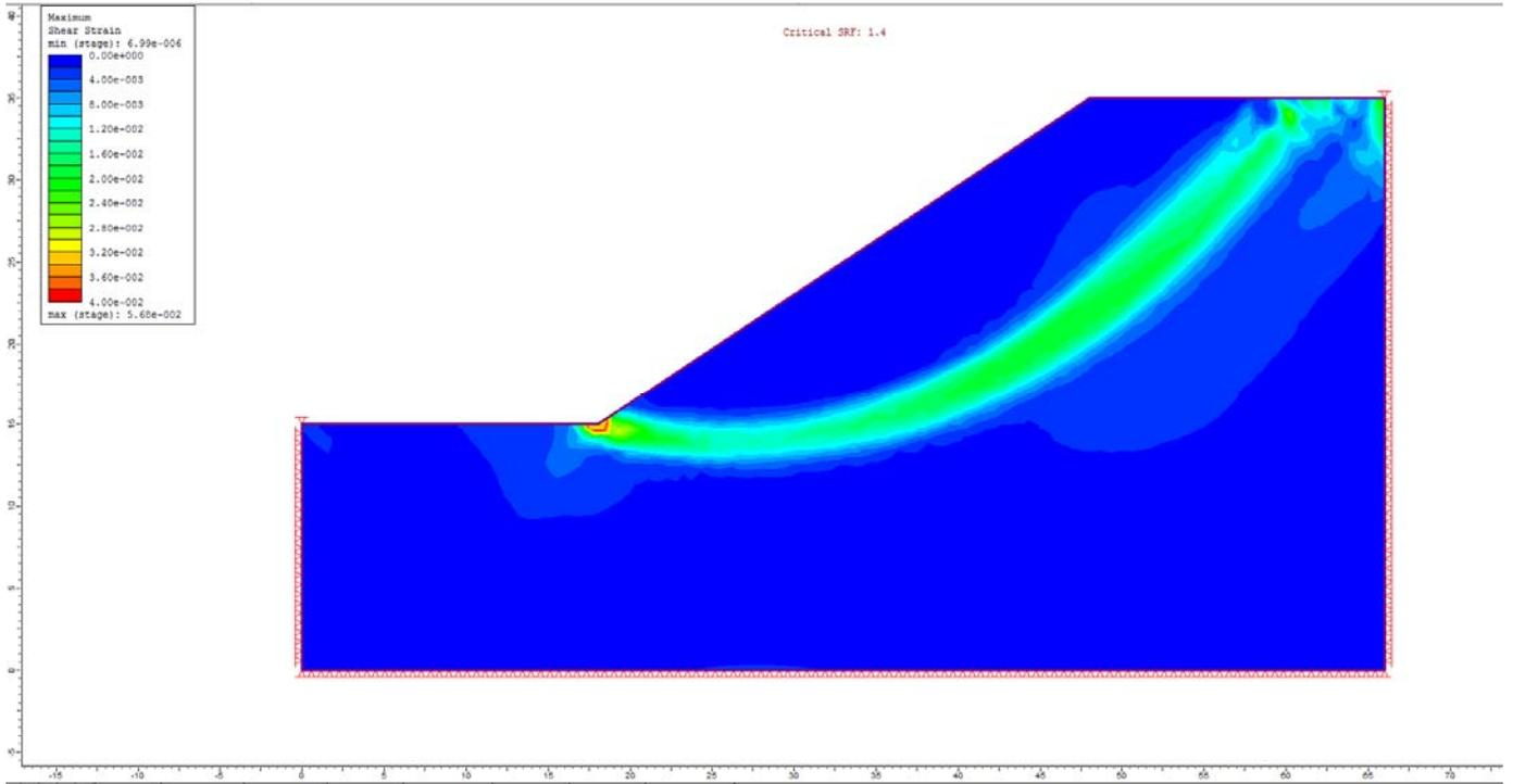
Figure 8.4.7 – RS2 Maximum Shear Strain
