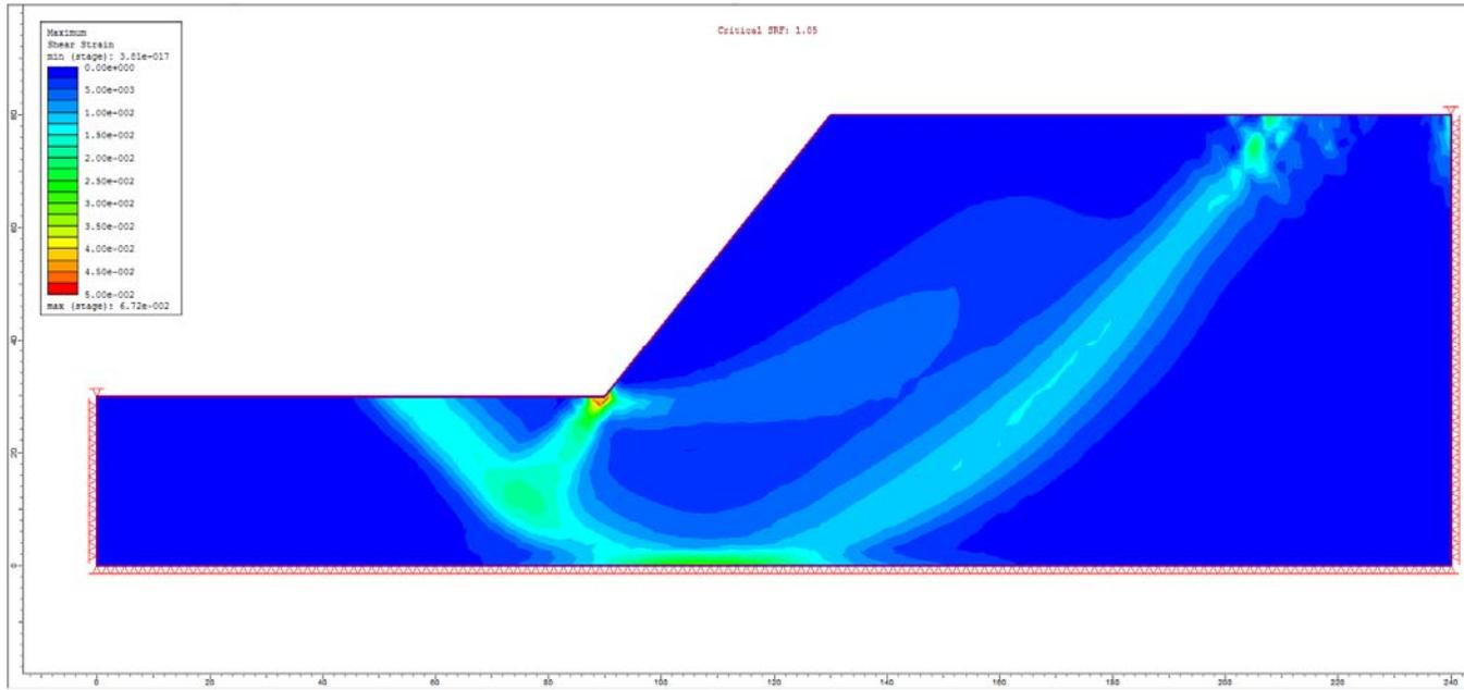
Figure 35.4.7 – RS2 Maximum Shear Strain
