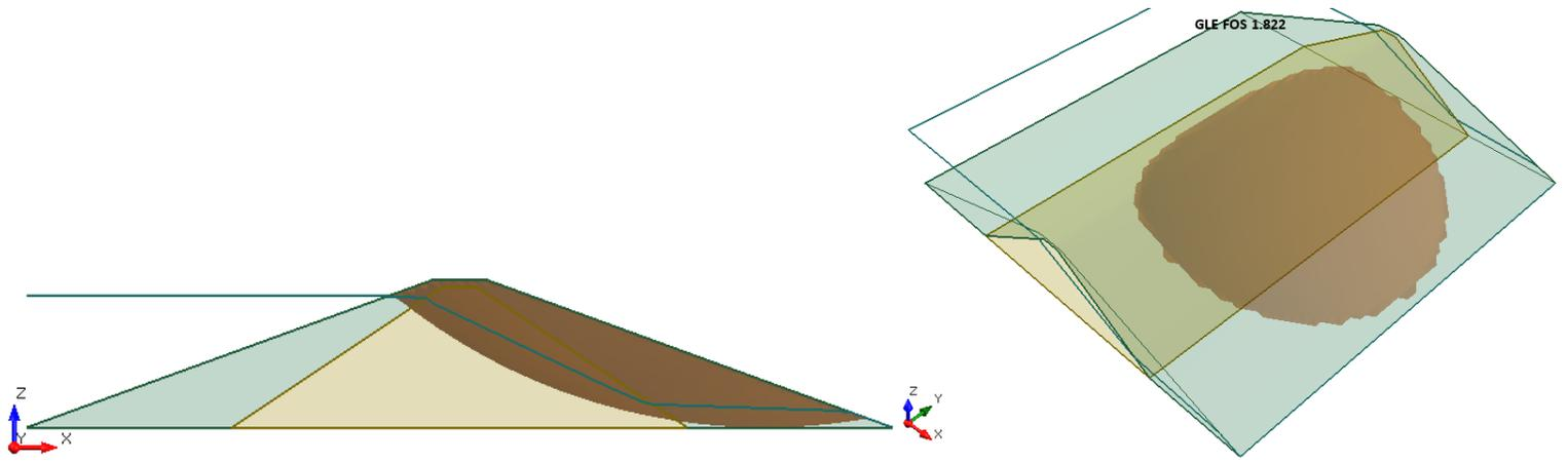
Figure 32.4.3 – Slide3 Solution Using the GLE Method
