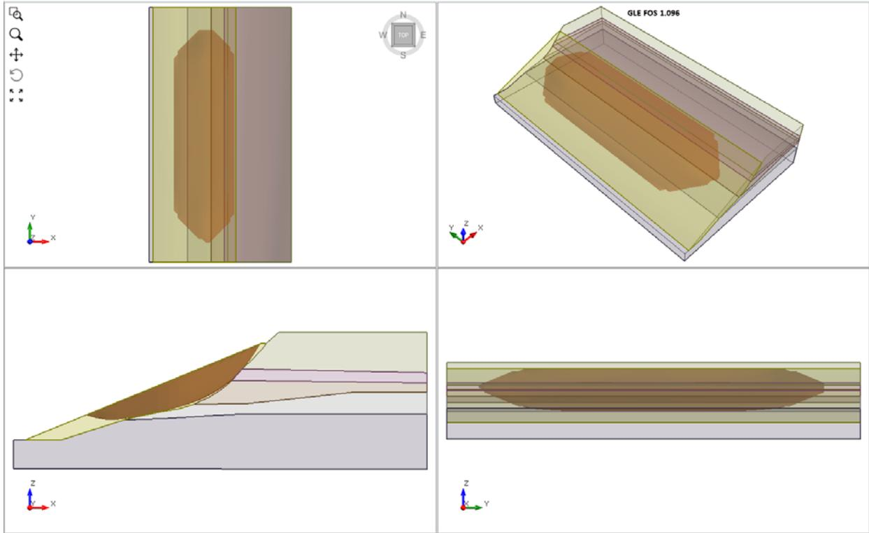
Figure 44.4.3 – Slide3 Solution Using the GLE Method
