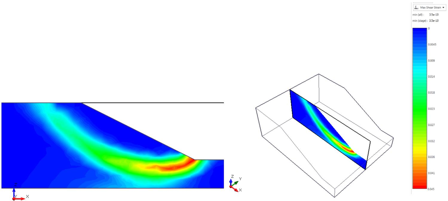
Figure 14.4.10 – RS3 Maximum Shear Strain
