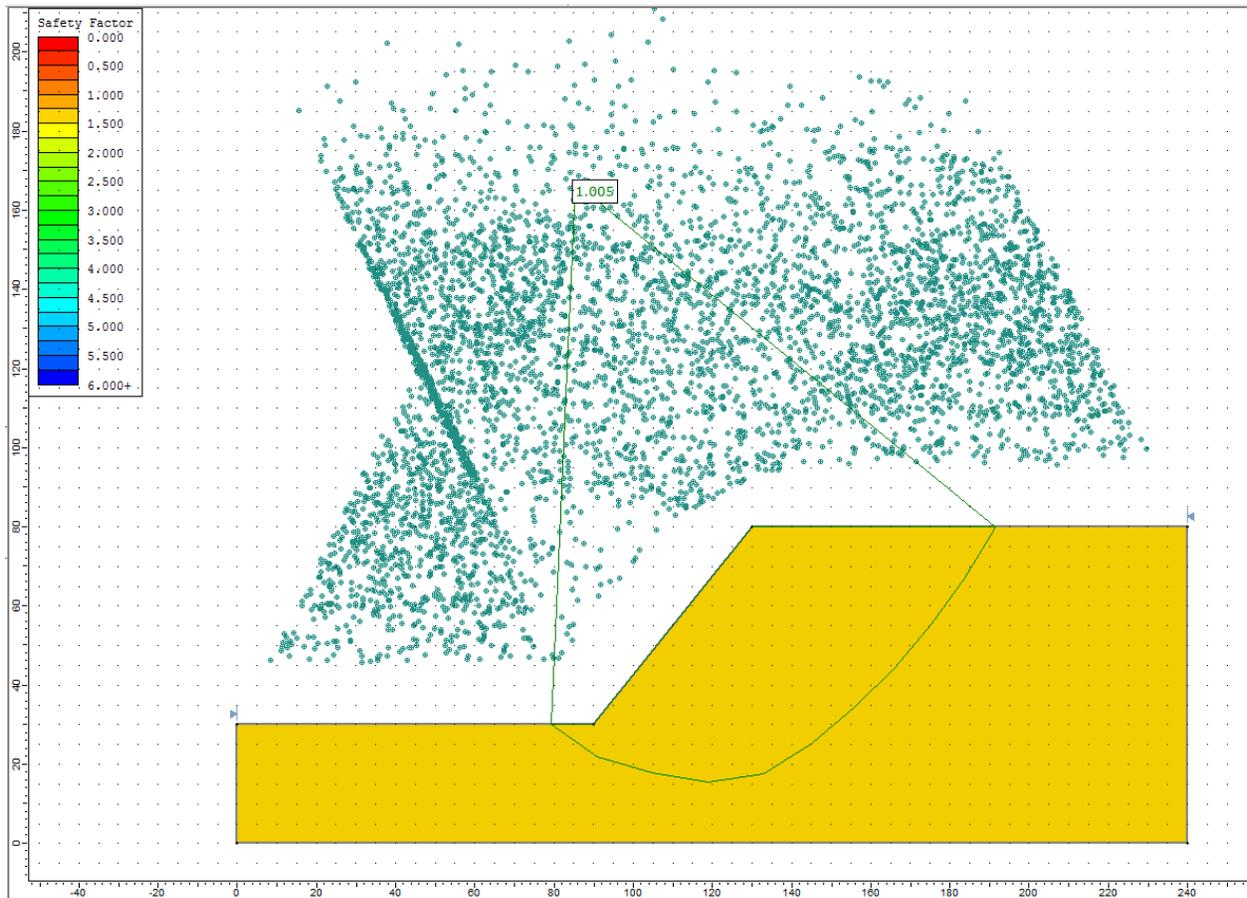
**Figure 35.4.6 – Slide Solution Using the Spencer Method**
