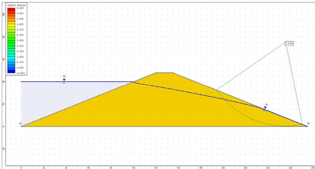
**Figure 30.4.2 – Slide Solution Using the Bishop Method**
