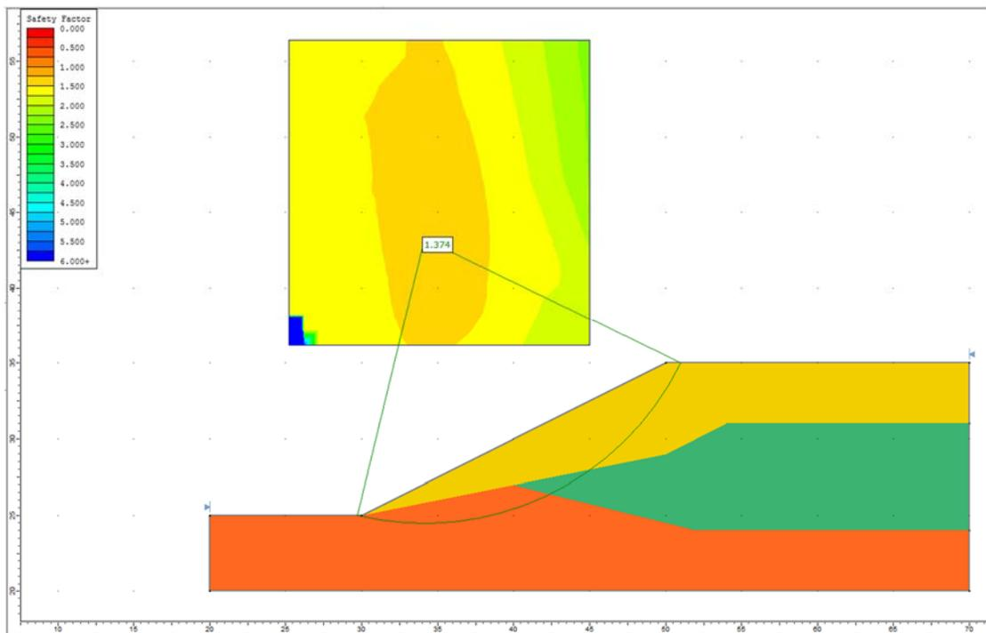
Figure 3.4.6 – Slide Solution Using the GLE Method
