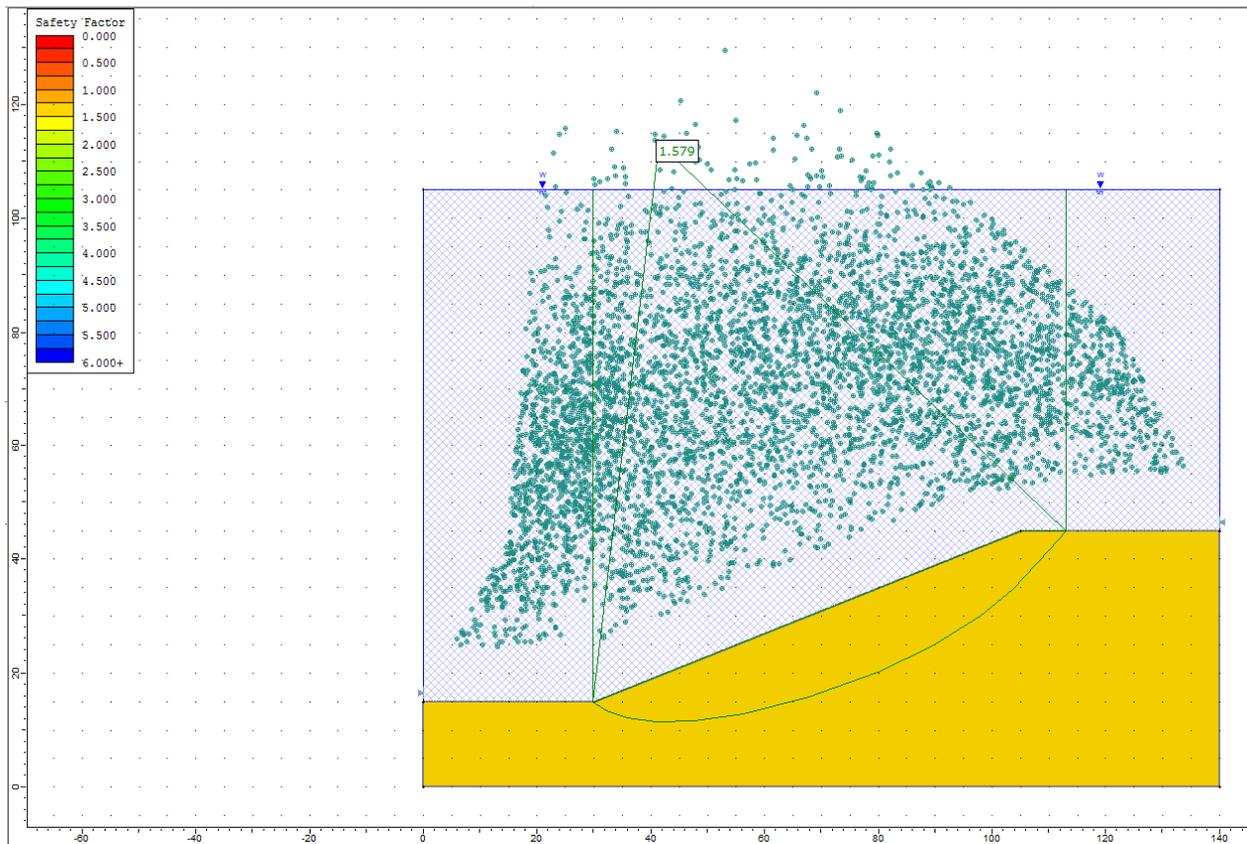
**Figure 28.4.4 – Slide Solution Using the GLE Method**
