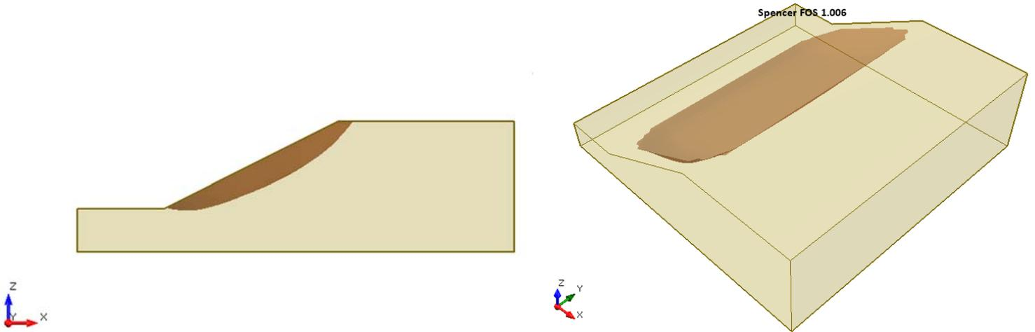
**Figure 2.4.3 – Slide3 Solution Using the Spencer Method**
