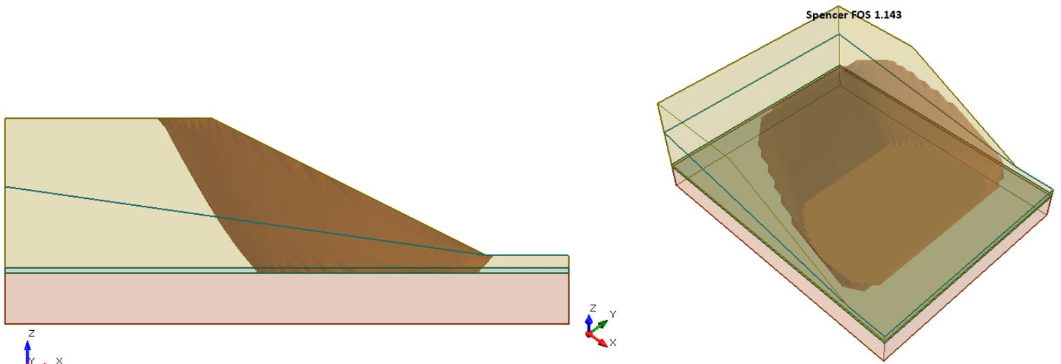
**Figure 16.4.7 – Slide3 Solution Using the Spencer Method**
