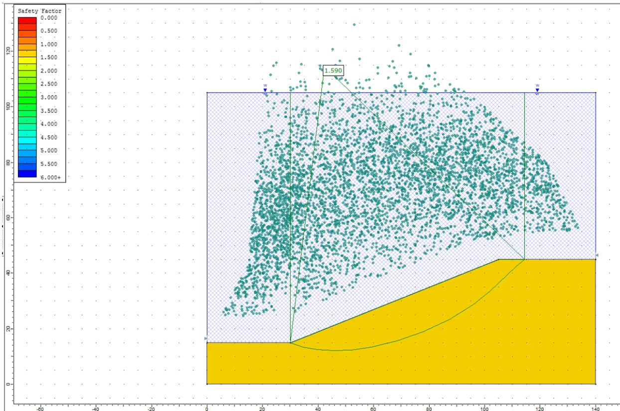
**Figure 28.4.6 – Slide Solution Using the Spencer Method**
