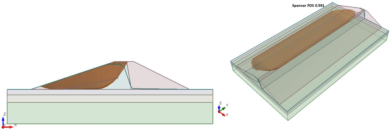
Figure 42.4.7 – Slide3 Solution using the Spencer Method
