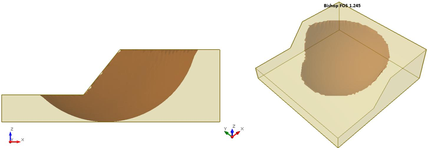
**Figure 34.4.1 – Slide3 Solution Using the Bishop Method**
