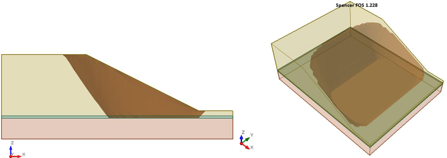
**Figure 15.4.7 – Slide 3 Solution Using the Spencer Method**
