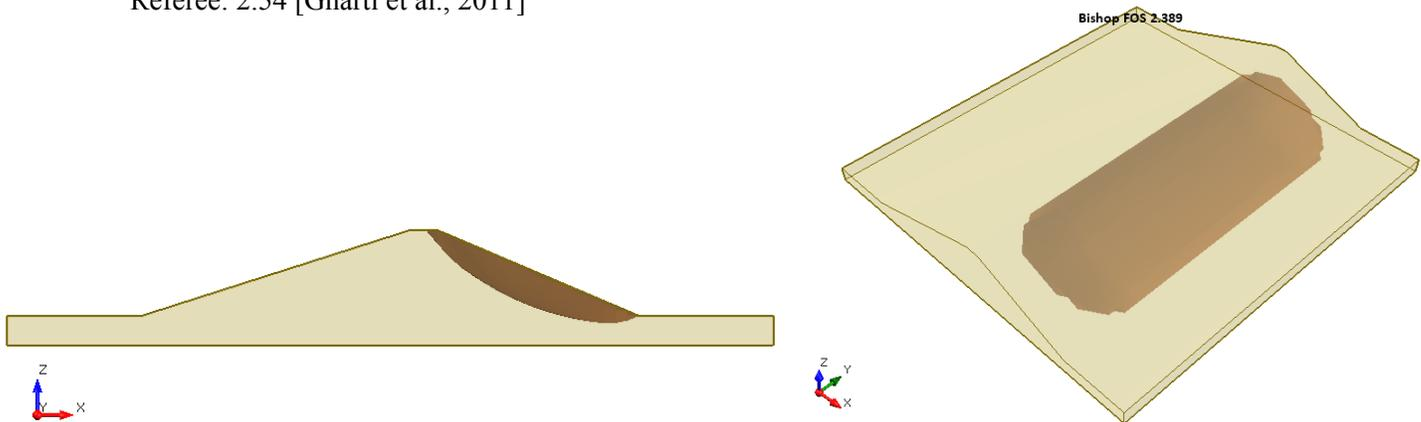
**Figure 12.4.1 – Slide3 Solution Using the Bishop Method**
