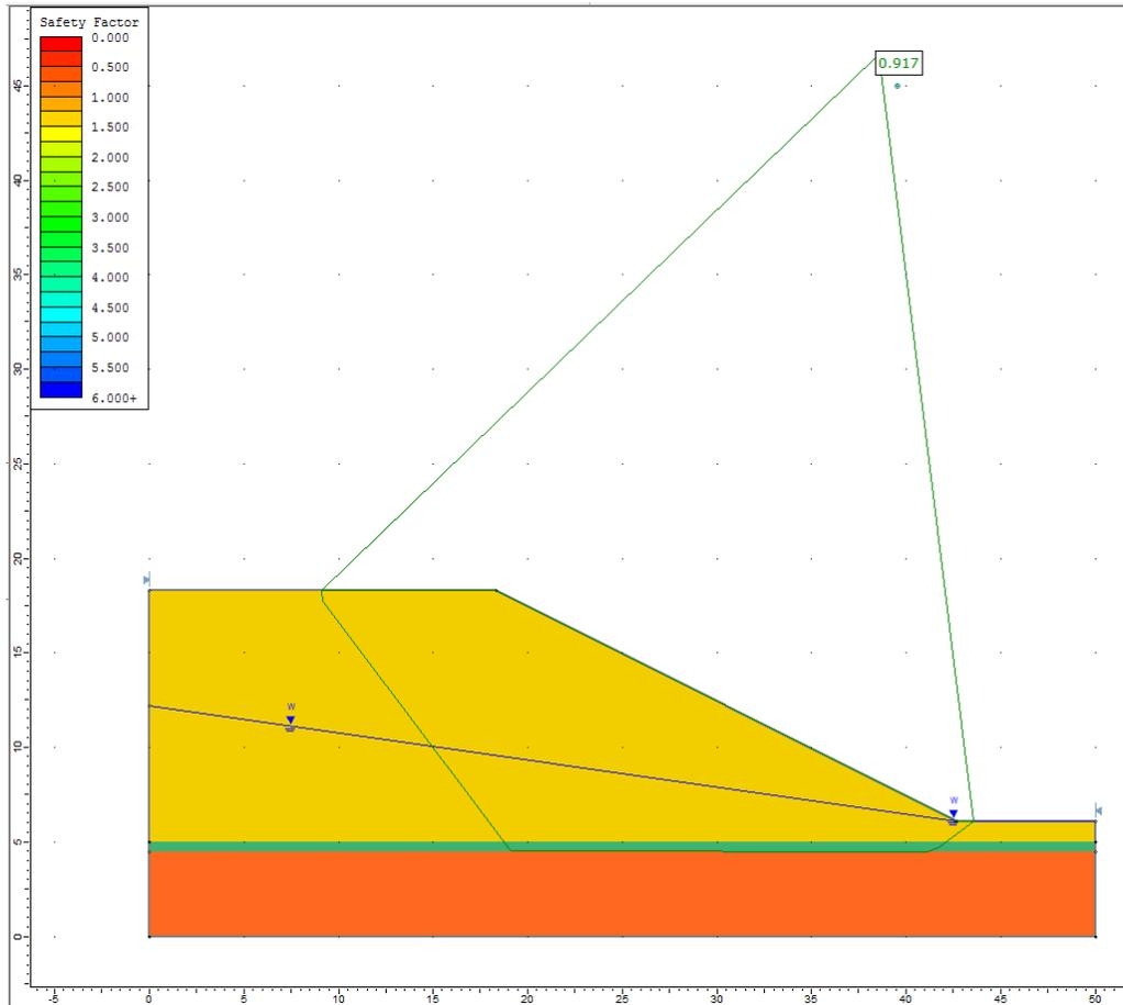
**Figure 16.4.8 – Slide Solution Using the Spencer Method**
