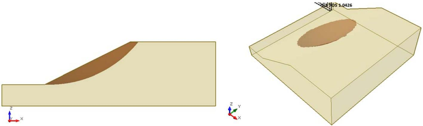
Figure 1.4.5 – Slide3 Solution Using the GLE Method
