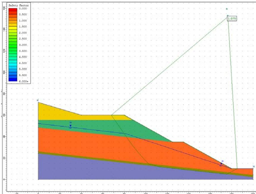
**Figure 20.4.2 – Slide Solution Using the Bishop Method**
