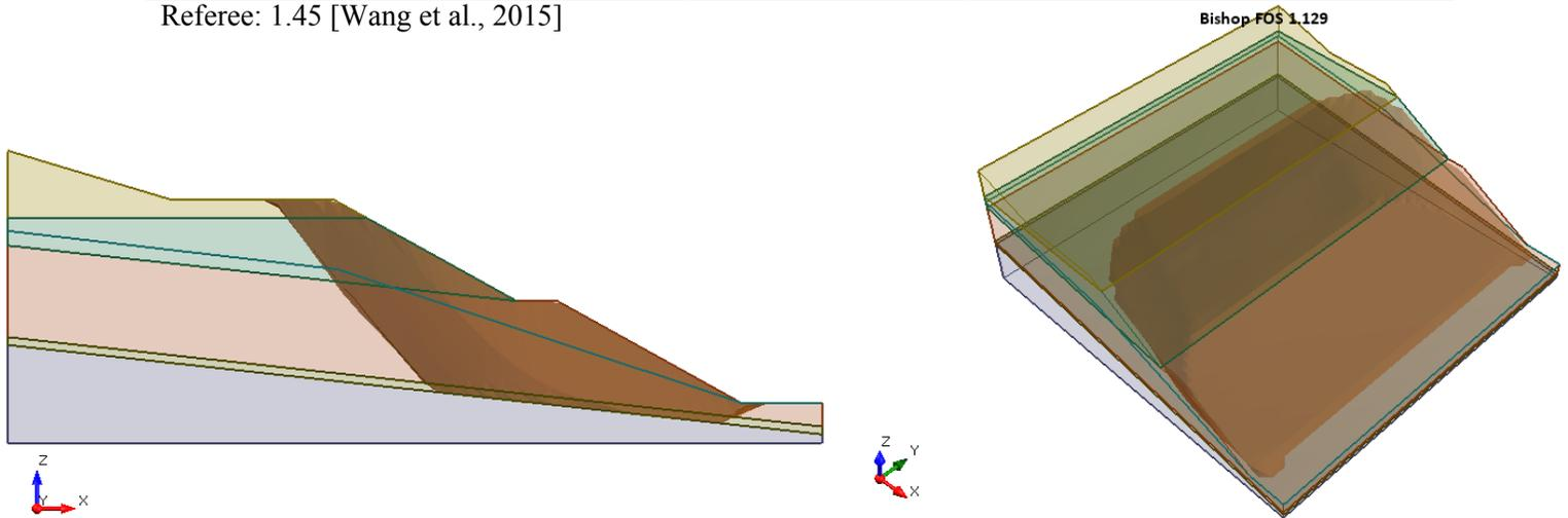
**Figure 20.2.1 – Slide3 Solution Using the Bishop Method**
