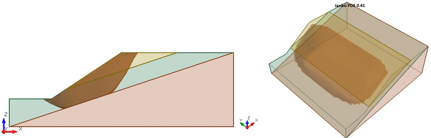
**Figure 11.4.1 – Slide3 Solution Using the Janbu Method**
