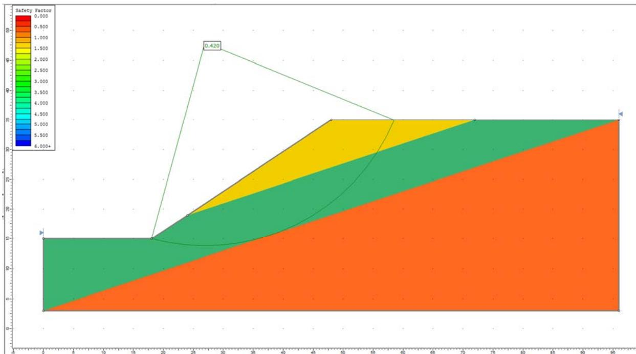
**Figure 10.4.2 – Slide Solution Using the Bishop Method**
