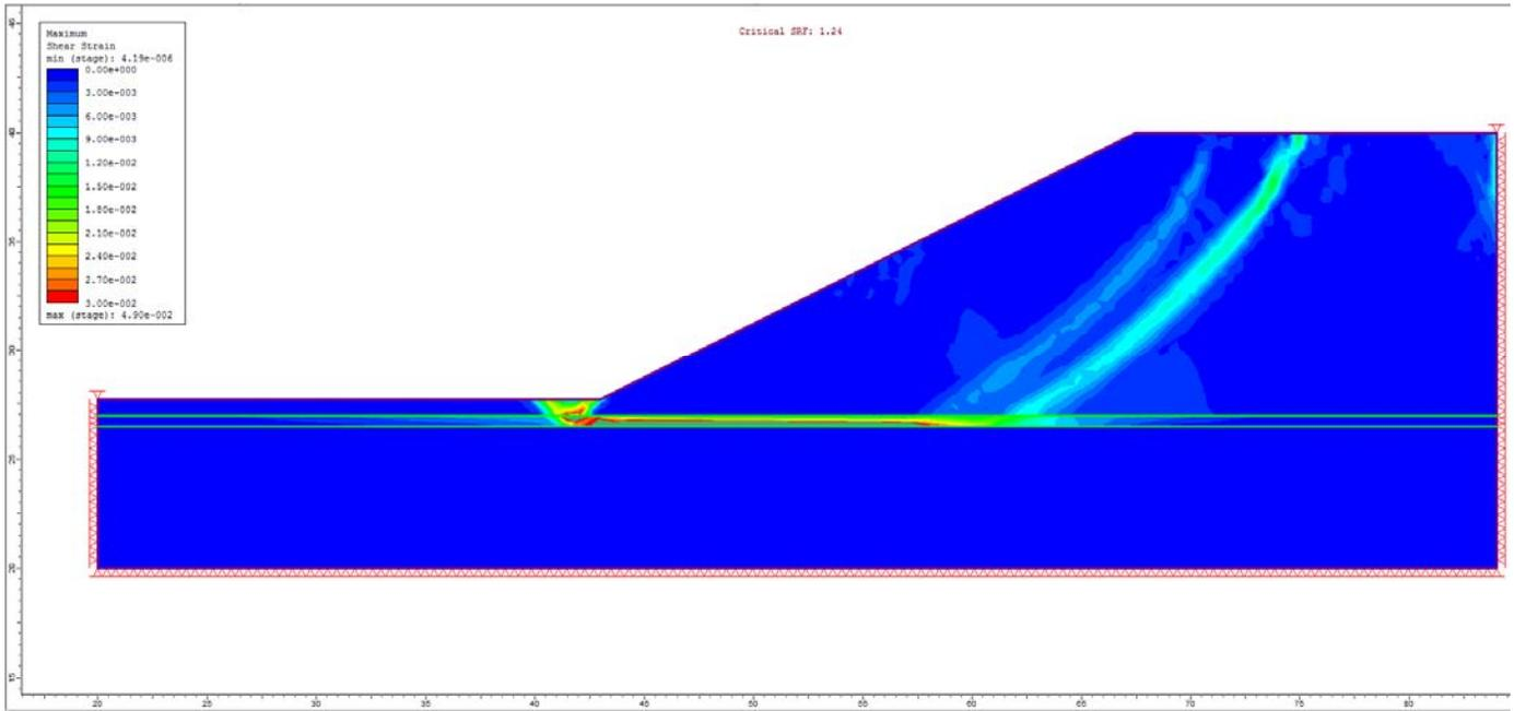
Figure 7.4.7 – RS2 Maximum Shear Strain
