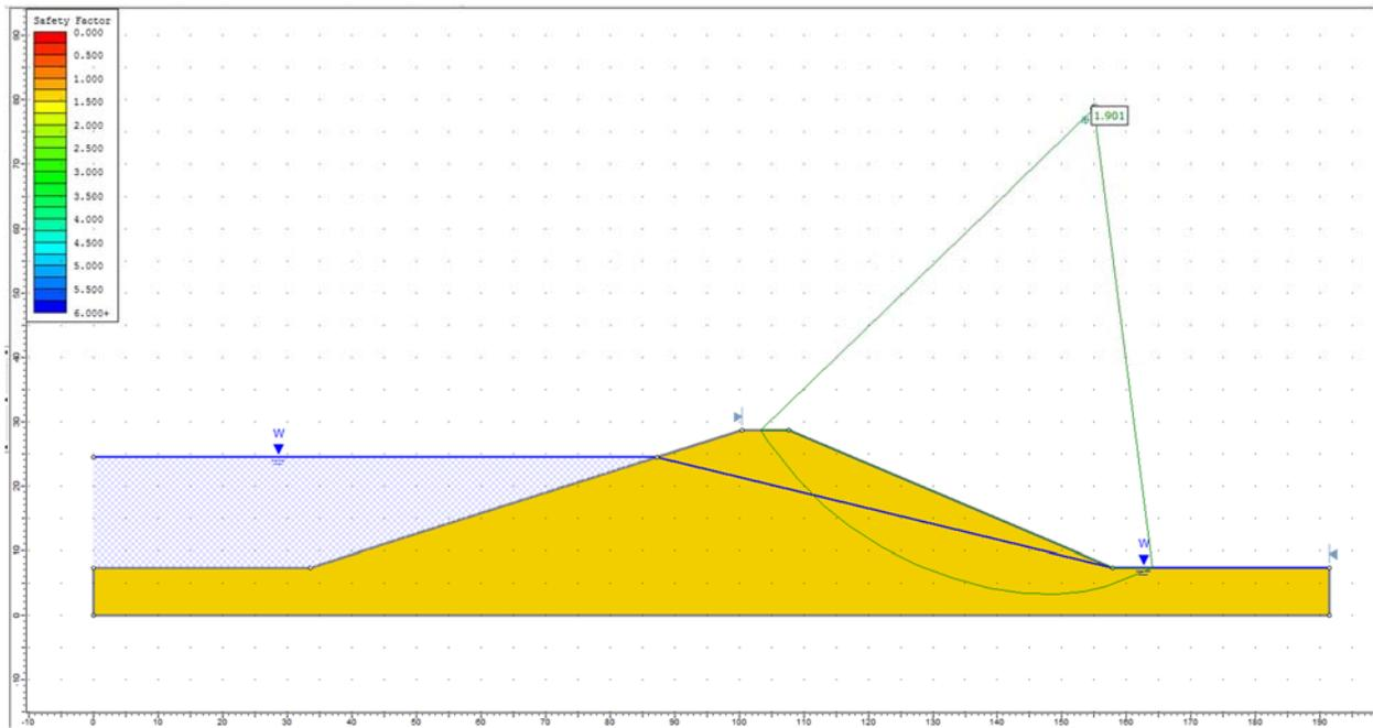
**Figure 13.4.8 – Slide Solution Using the Spencer Method**
