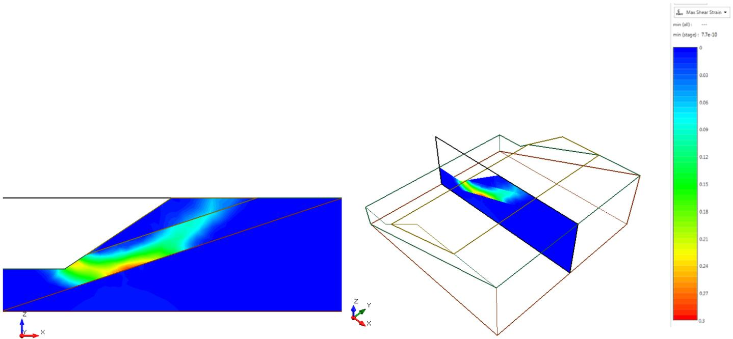
Figure 10.4.8 – RS3 Maximum Shear Strain
