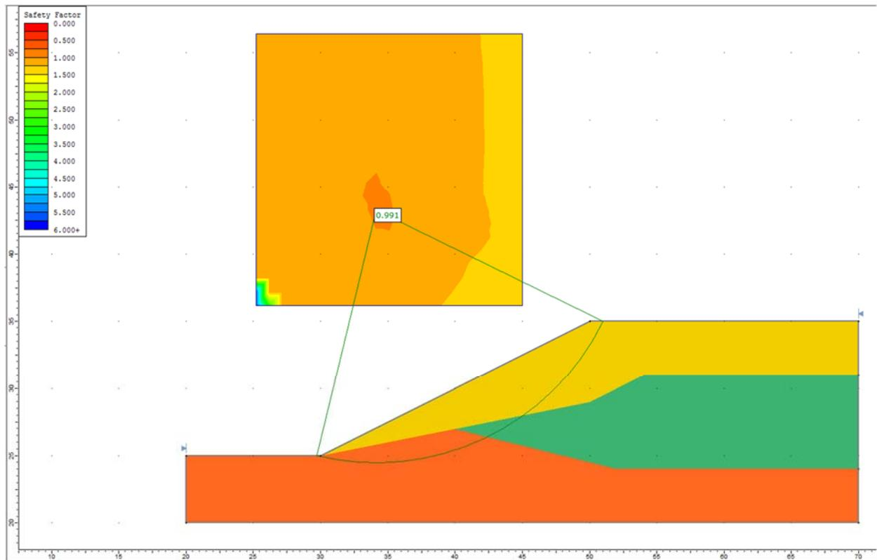
**Figure 5.4.4 – Slide Solution Using the Spencer Method**
