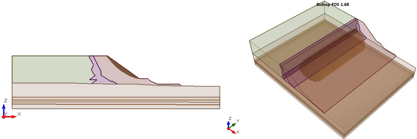
**Figure 46.4.1 – Slide3 Solution Using the Bishop Method**
