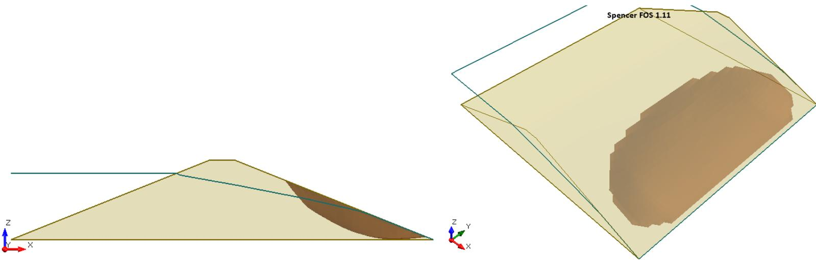
**Figure 31.4.5 – Slide3 Solution Using the Spencer Method**
