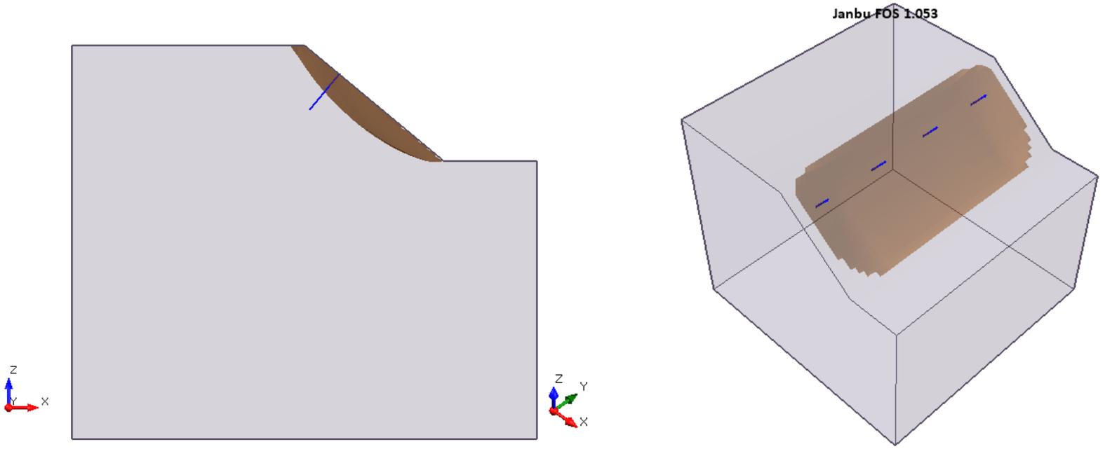
**Figure 22.4.5 – Slide3 Solution Using the Janbu Method**
