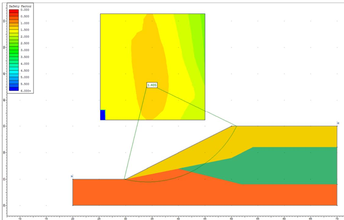
**Figure 3.4.2 – Slide Solution Using the Bishop Method**
