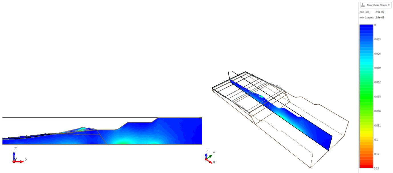
Figure 39.4.10 – RS3 Maximum Shear Strain
