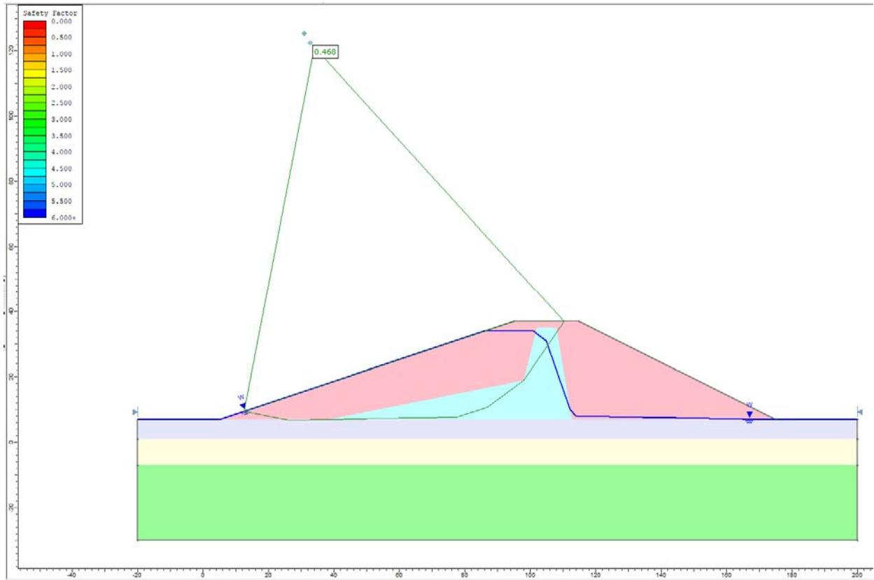
Figure 42.4.6 – Slide Solution using the Janbu Method
