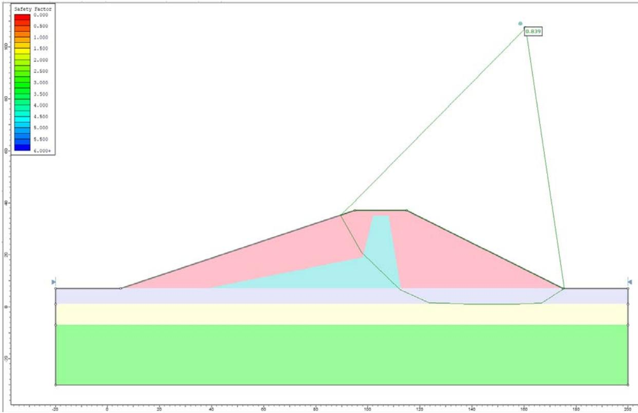
Figure 40.4.8 – Slide Solution Using the Spencer Method
