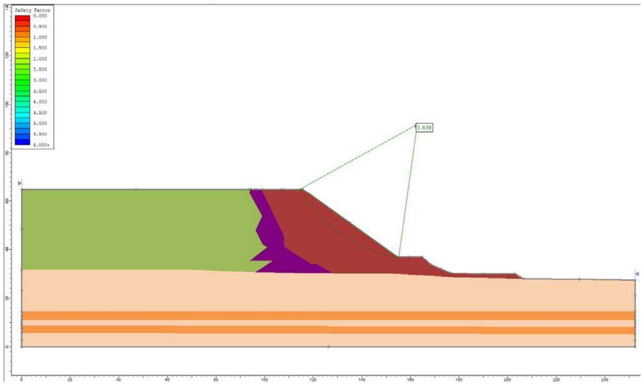
**Figure 46.4.6 – Slide Solution Using the Janbu Method**
