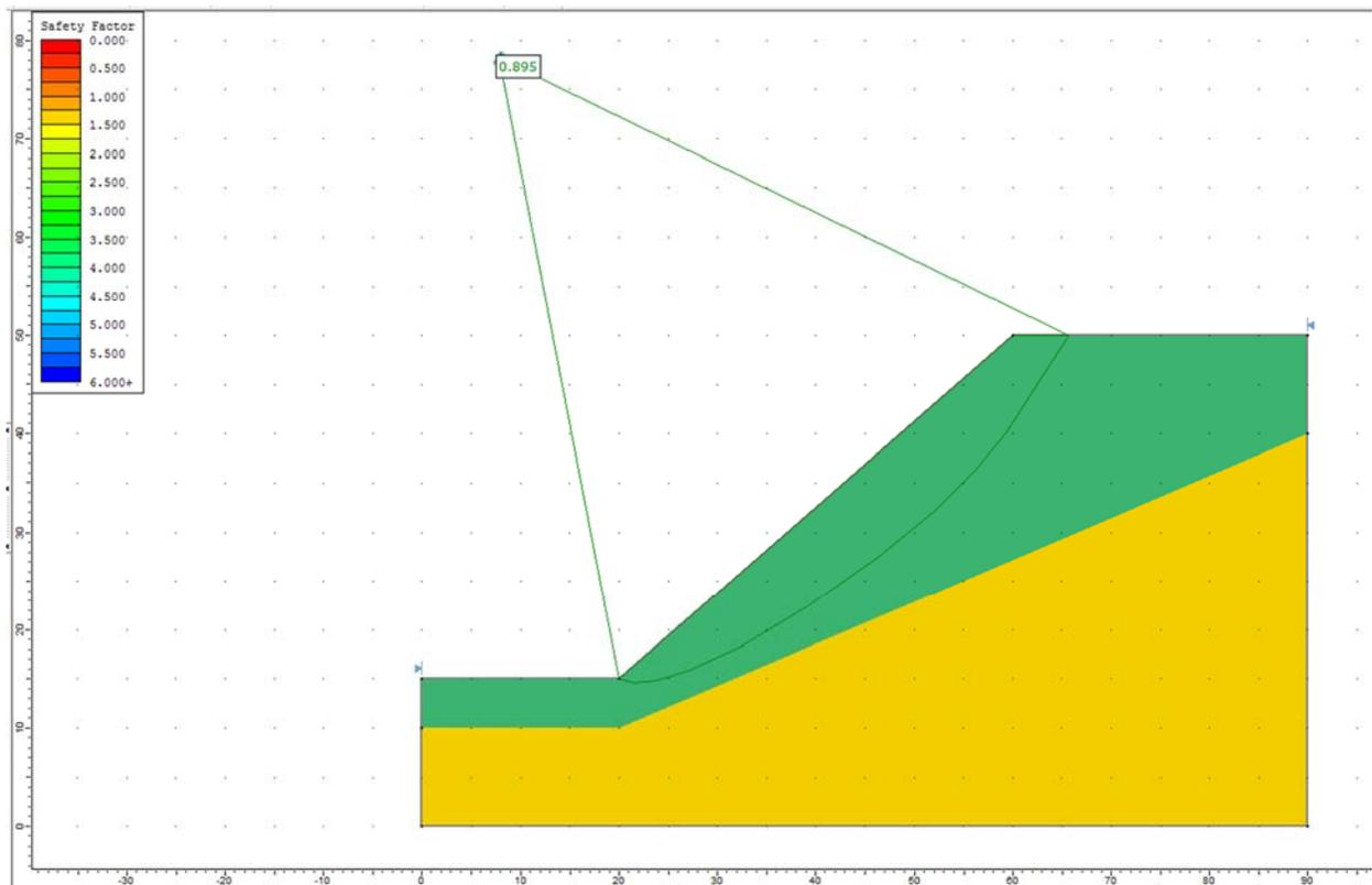
**Figure 17.4.4 – Slide Solution Using the GLE Method**
