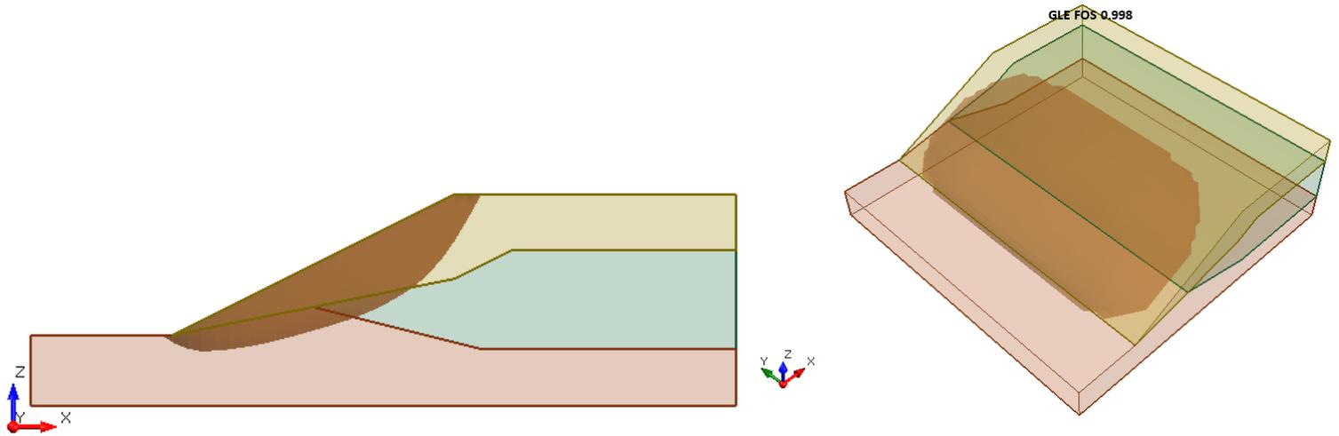
Figure 6.4.5 – Slide3 Solution Using the GLE Method
