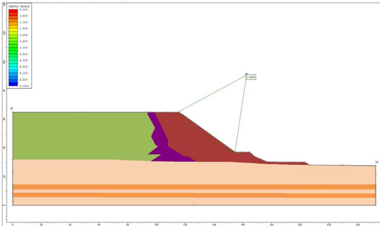
**Figure 46.4.4 – Slide Solution Using the GLE Method**
