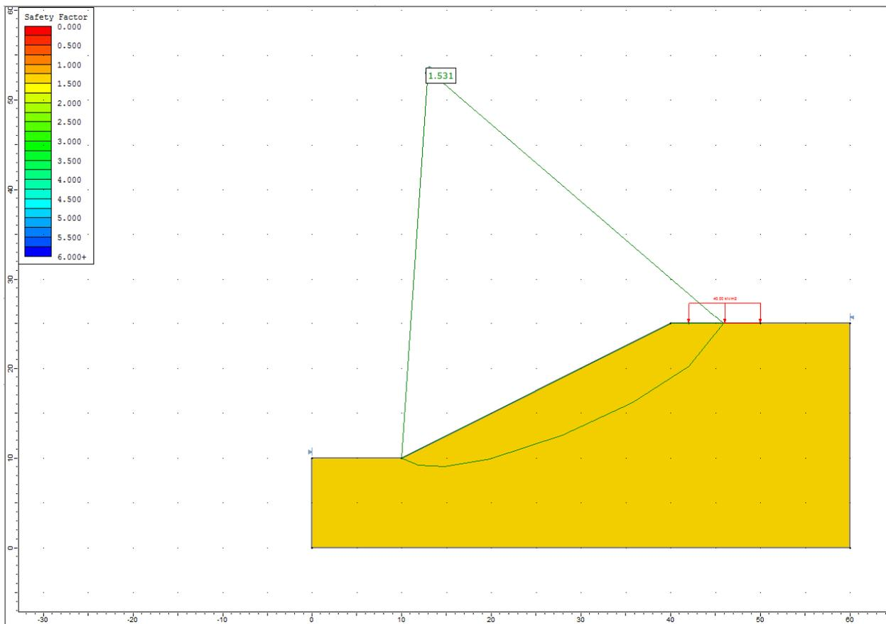
**Figure 21.4.4 – Slide Solution Using the GLE Method**
