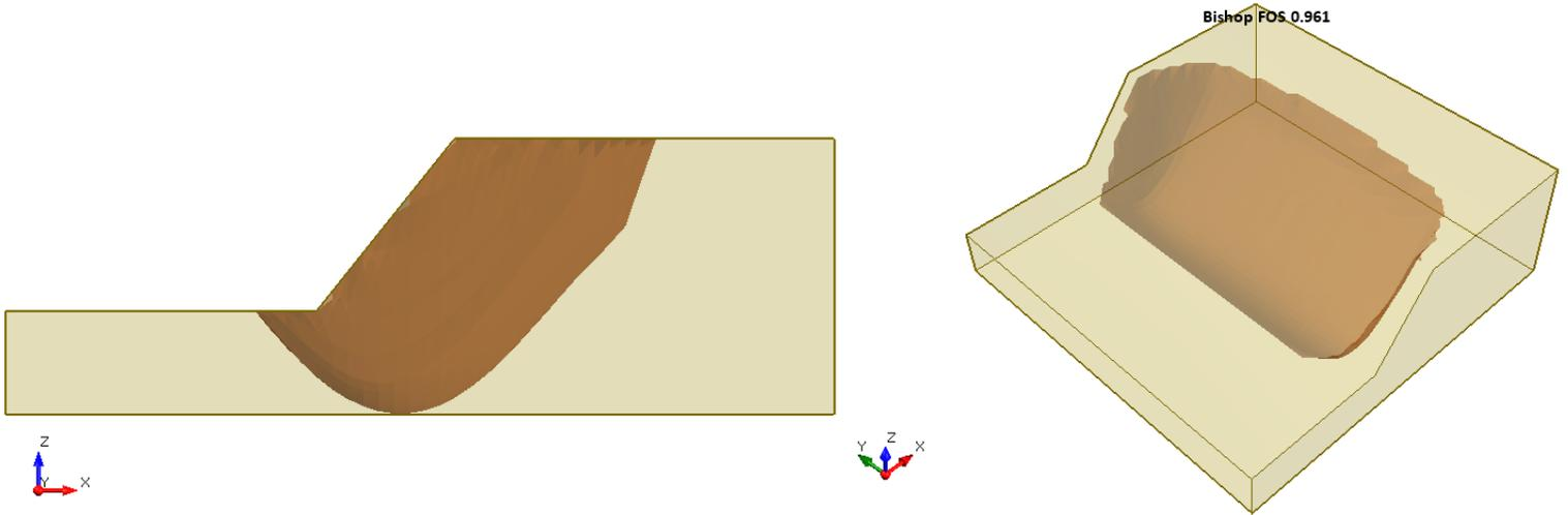
**Figure 35.4.1 – Slide3 Solution Using the Bishop Method**
