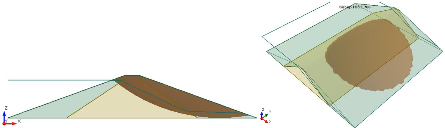
**Figure 32.4.1 – Slide3 Solution Using the Bishop Method**
