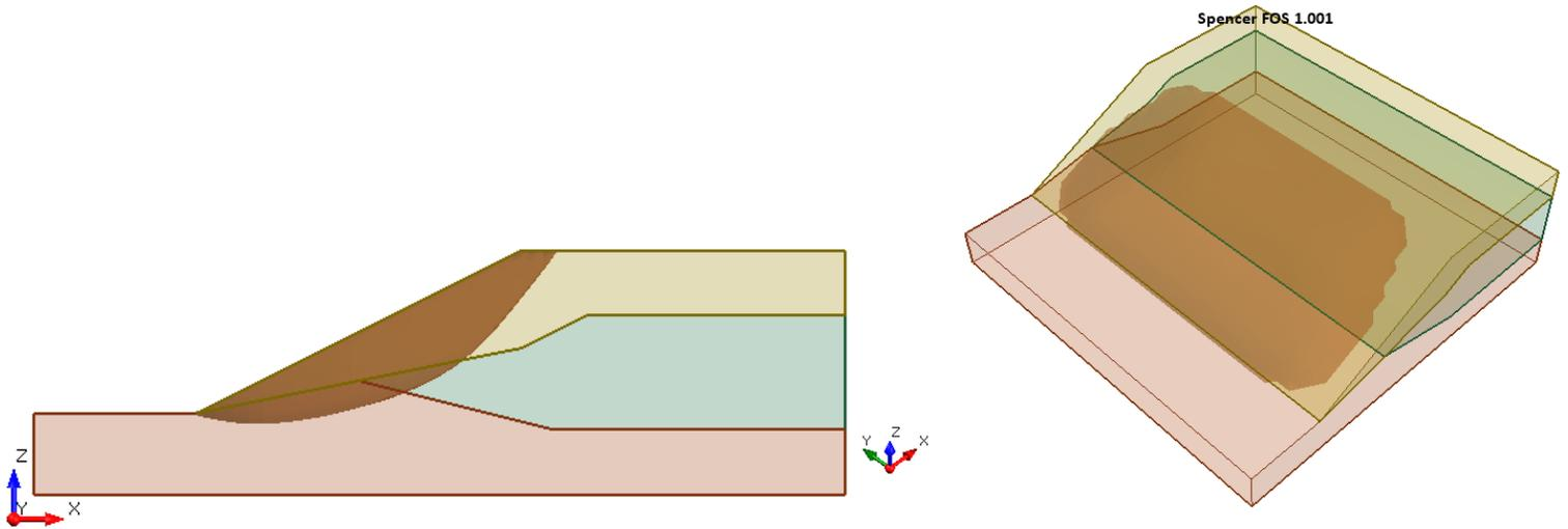
**Figure 6.4.3 – Slide3 Solution Using the Spencer Method**
