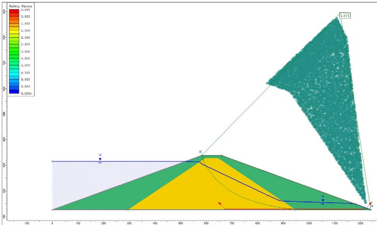
**Figure 33.4.4 – Slide Solution Using the GLE Method**
