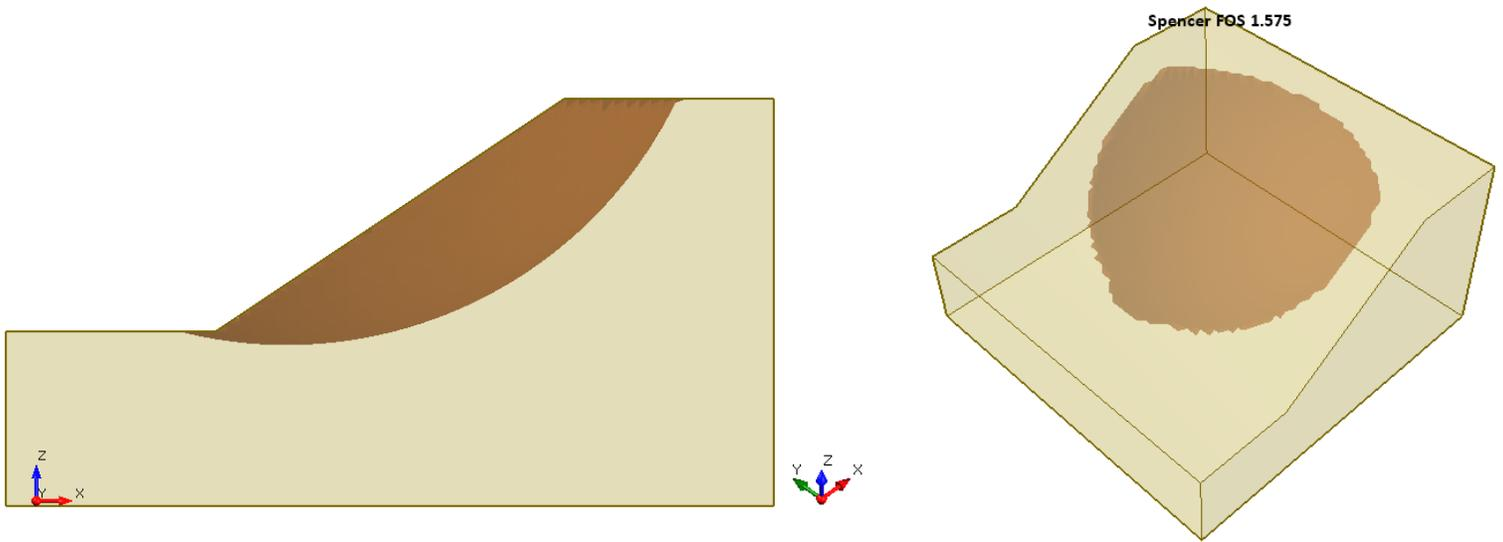
**Figure 8.4.3 – Slide3 Solution Using the Spencer Method**
