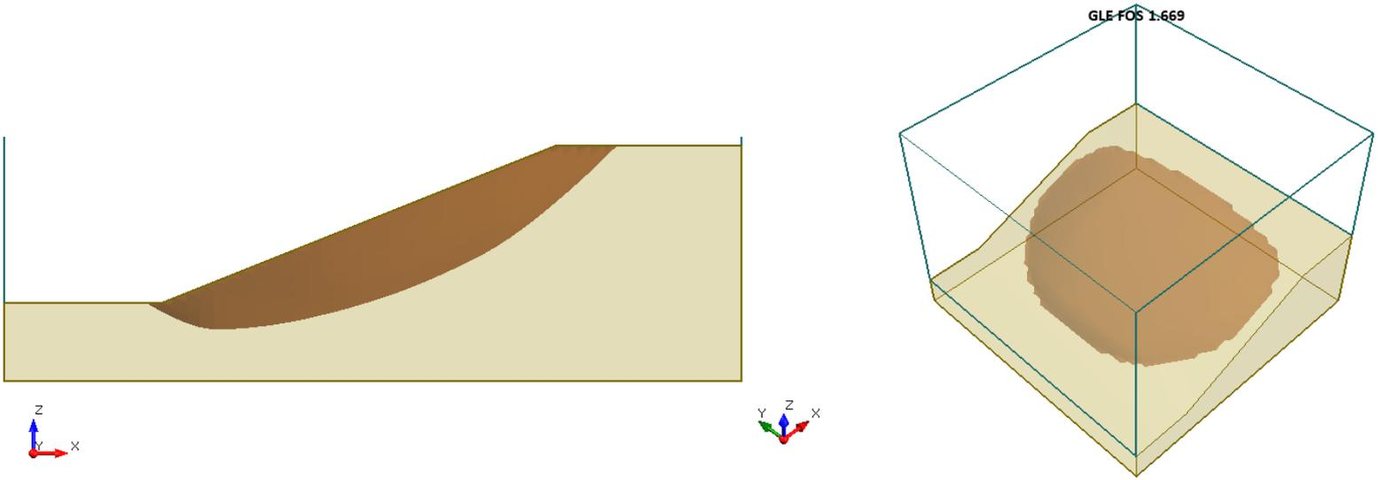
**Figure 28.4.3 – Slide3 Solution Using the GLE Method**
