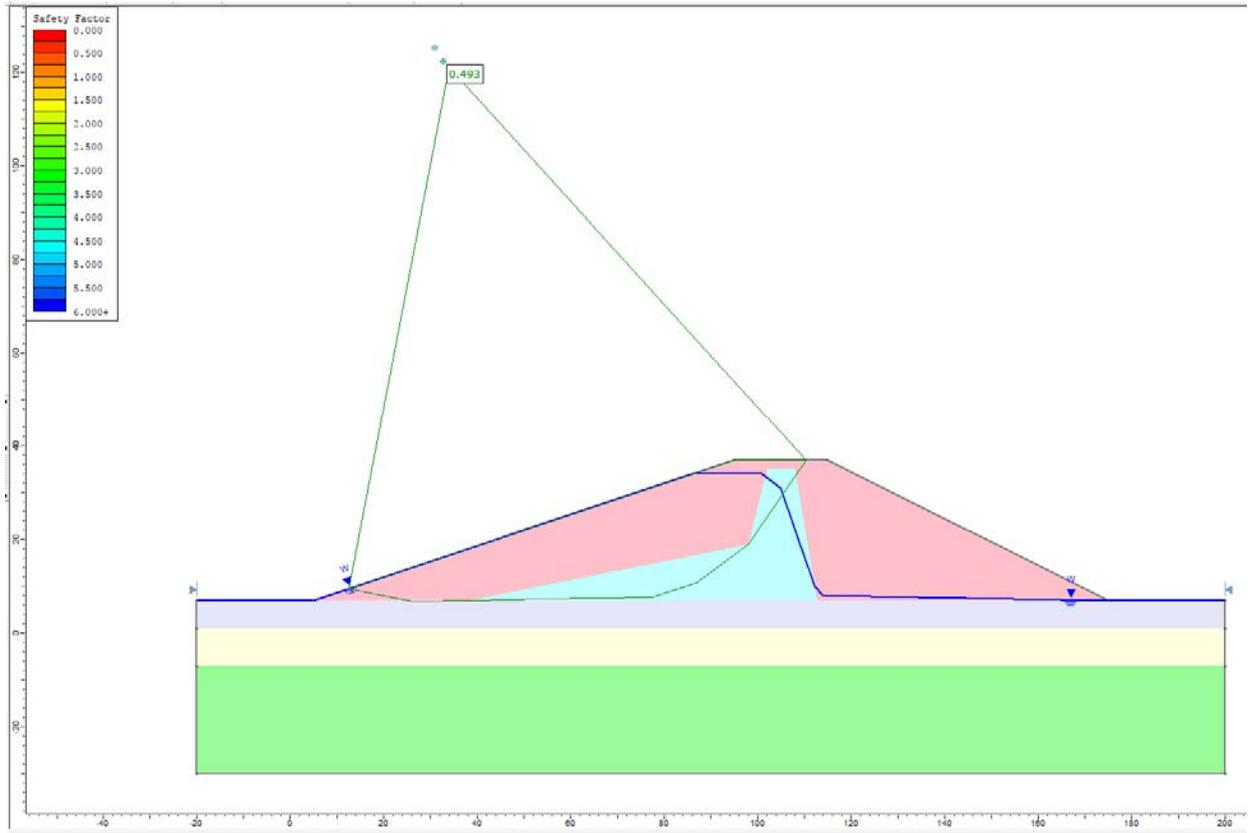
Figure 42.4.2 – Slide Solution Using the Bishop Method
