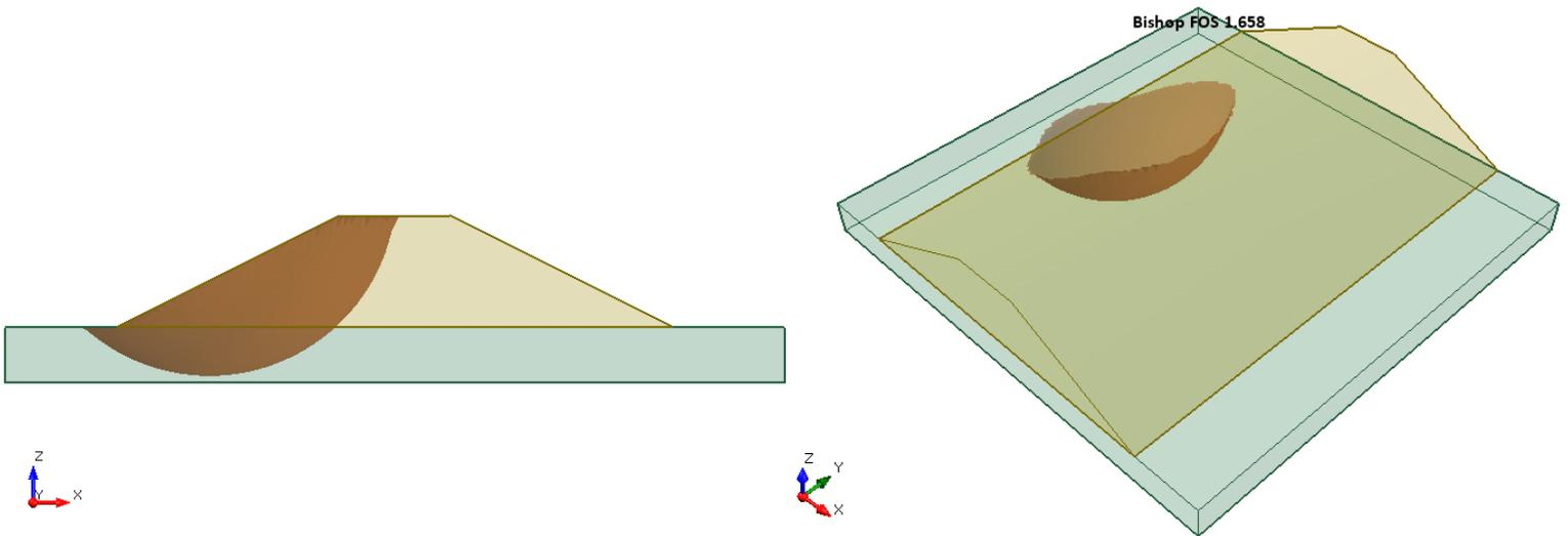
**Figure 29.4.1 – Slide3 Solution Using the Bishop Method**
