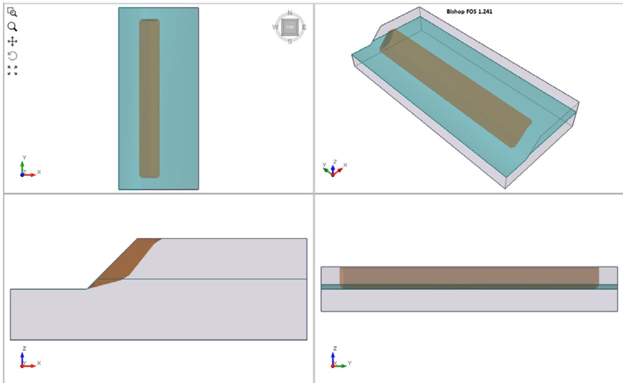
**Figure 24.4.1 – Slide3 User Defined Slip Surface Using Weak Planes**
