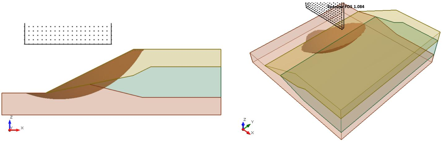
**Figure 5.4.3 – Slide3 Solution Using the Spencer Method**
