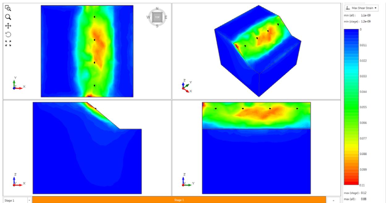
Figure 22.4.10 – RS3 Maximum Shear Strain
