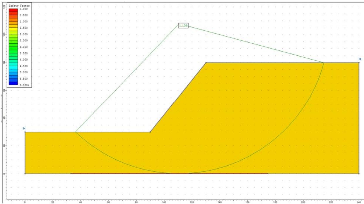
**Figure 34.4.6 – Slide Solution Using the Spencer Method**
