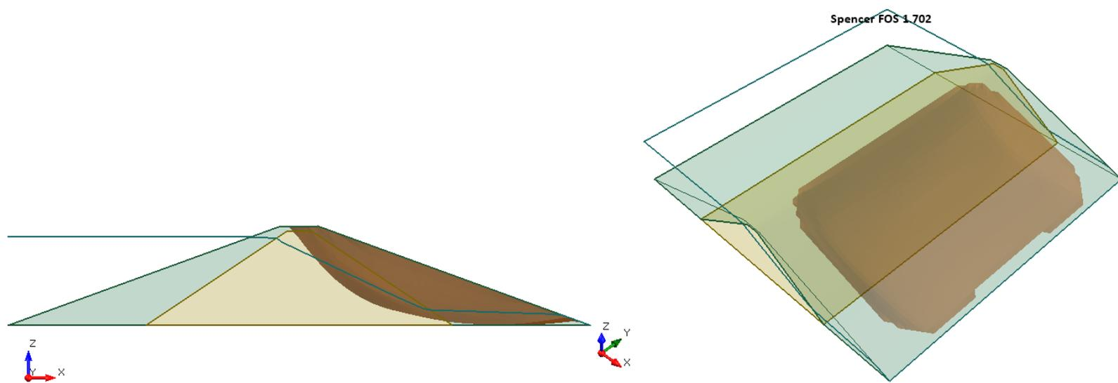
**Figure 33.4.5 – Slide3 Solution Using the Spencer Method**
