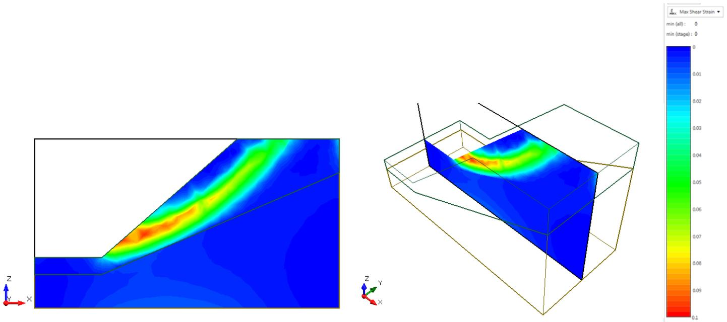
Figure 17.4.10 – RS3 Maximum Shear Strain
