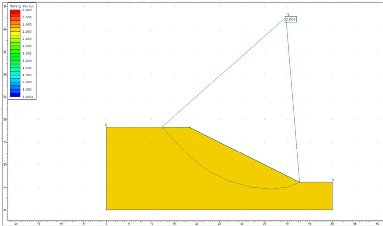
**Figure 14.4.8 – Slide Solution Using the Spencer Method**
