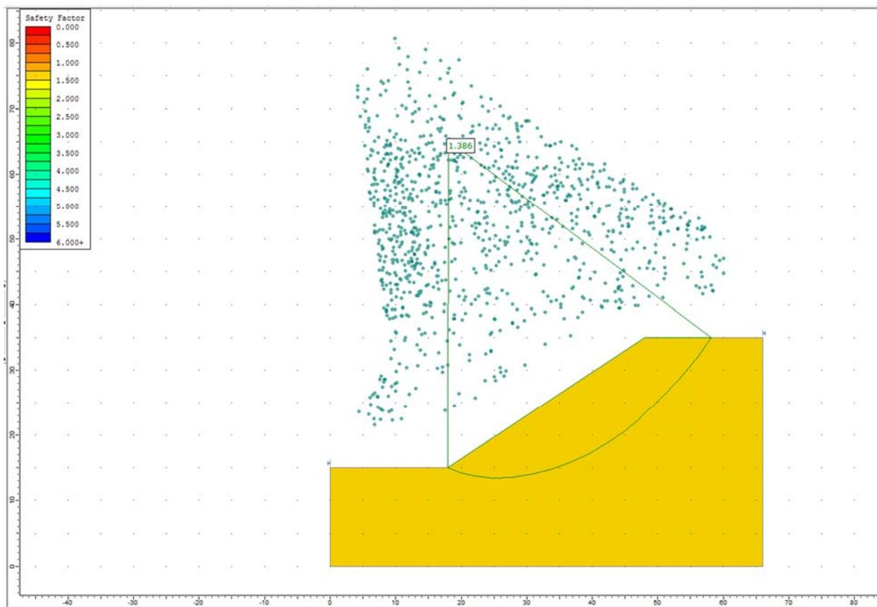
Figure 9.4.4 – Slide Solution Using the Spencer Method
