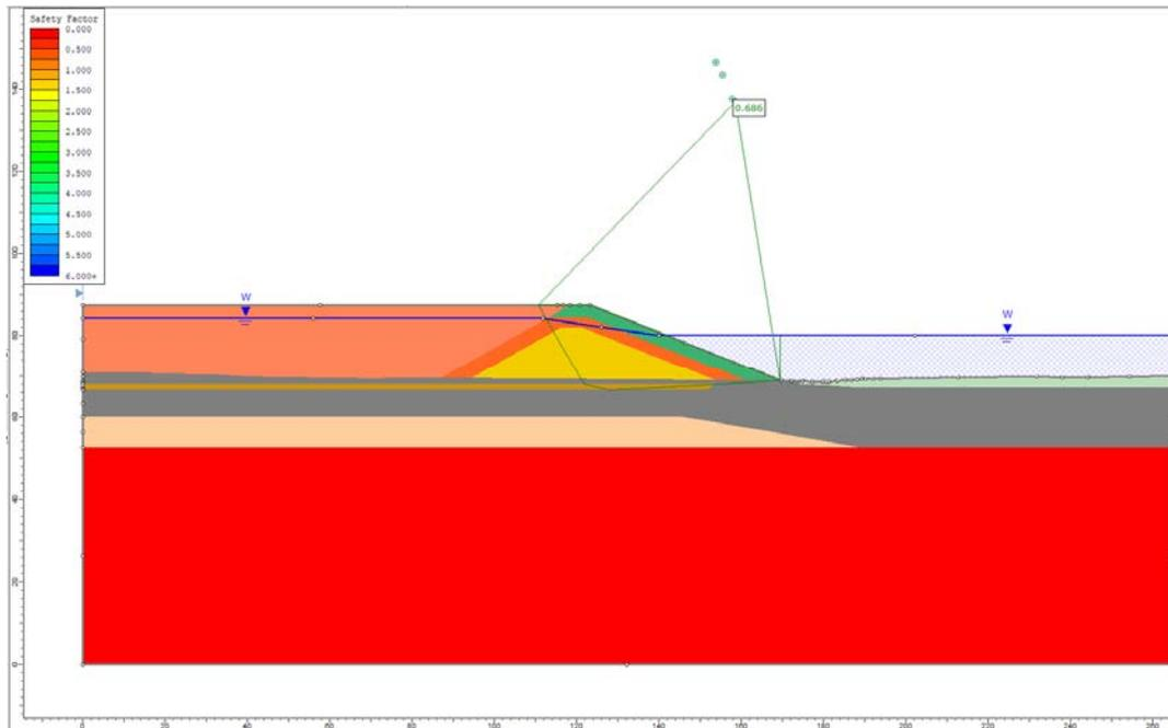
**Figure 45.4.2 – Slide Solution Using the Bishop Method**
