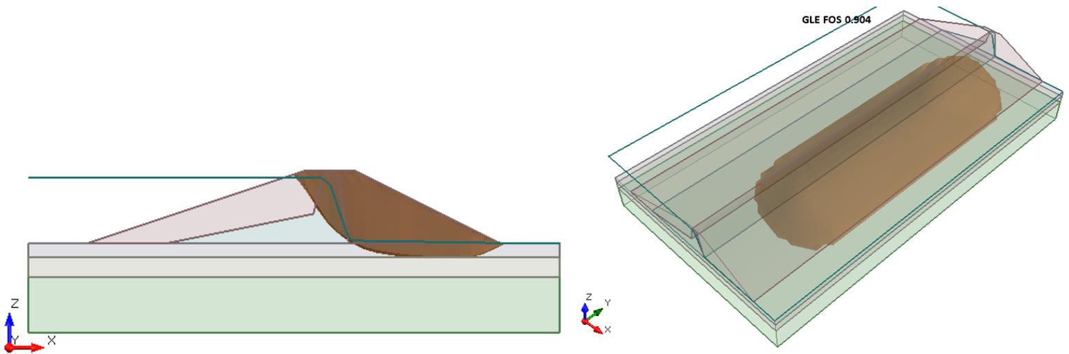
Figure 41.4.3 – Slide3 Solution using the GLE Method
