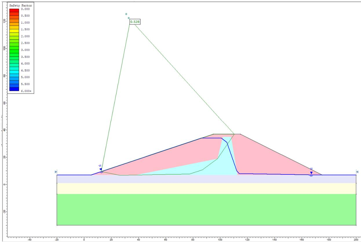
Figure 42.4.8 – Slide Solution Using the Spencer Method
