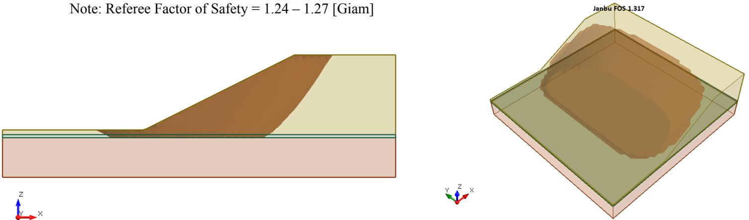
**Figure 7.4.1 – Solution Using the Janbu Simplified Method**
