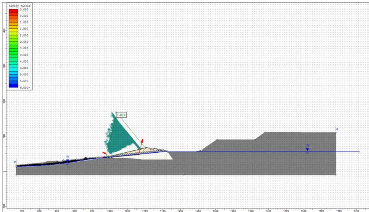
Figure 39.4.2 – Slide Solution Using the Bishop Method
