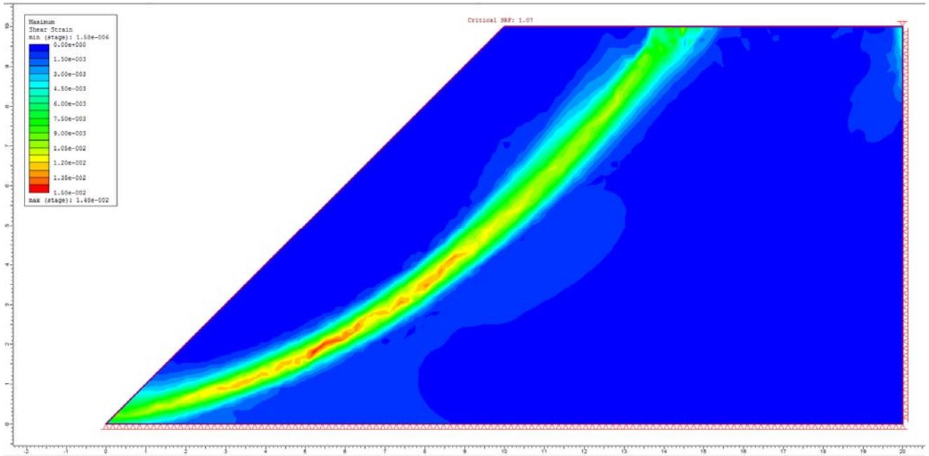
Figure 18.4.9 – RS2 Maximum Shear Strain
