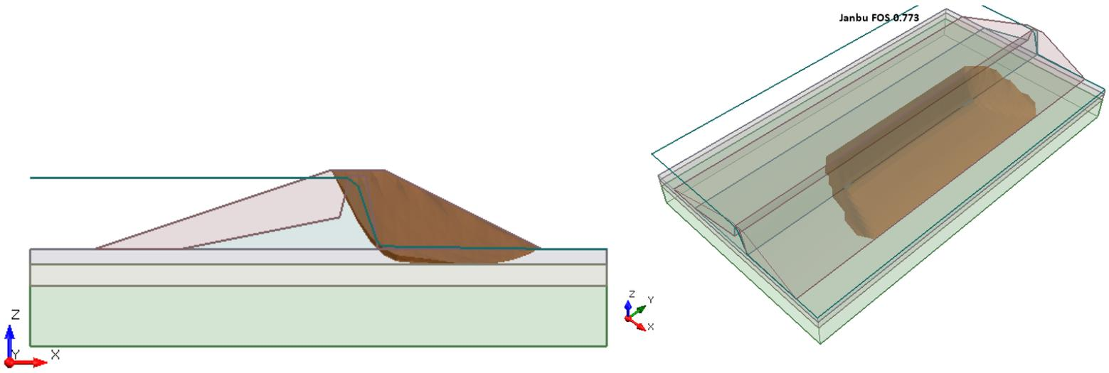
Figure 41.4.5 – Slide3 Solution Using the Janbu Method
