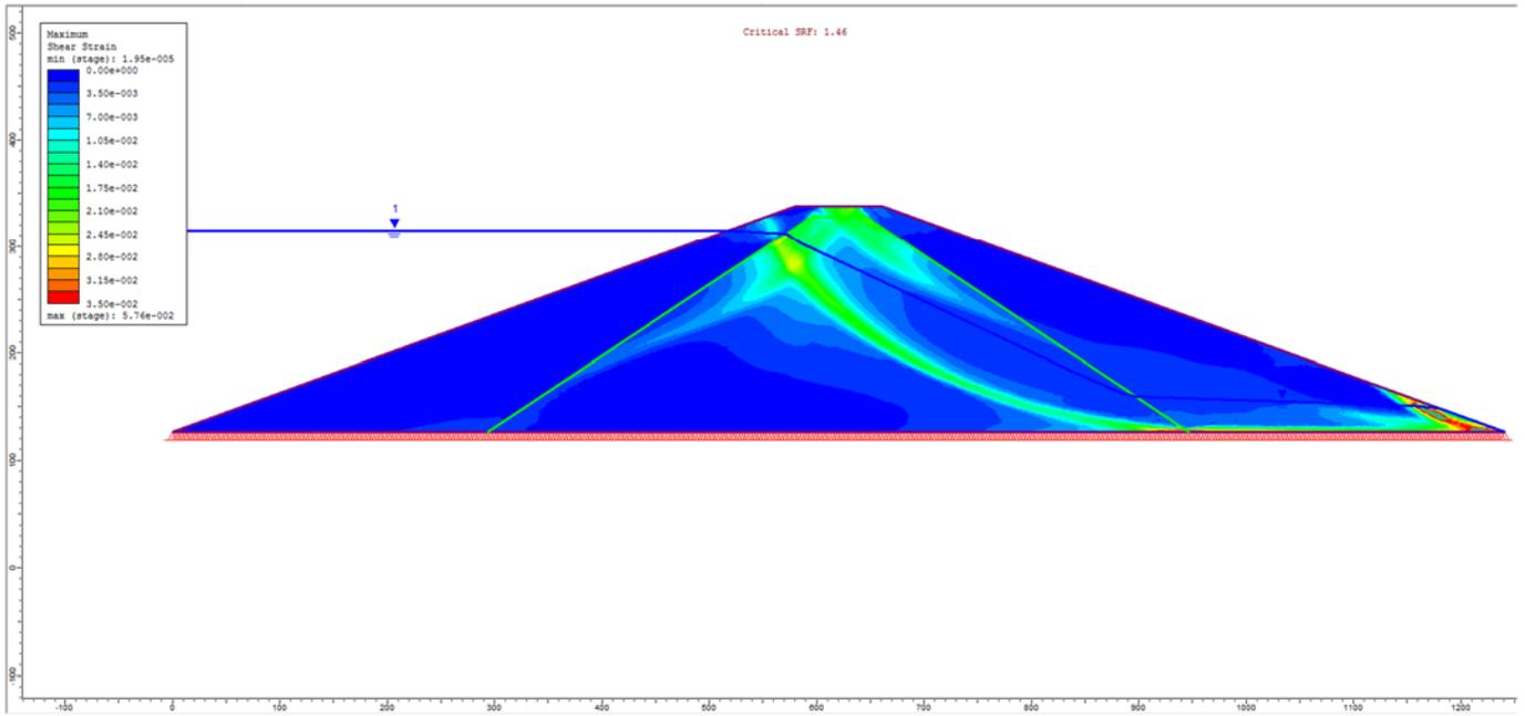
Figure 33.4.7 – RS2 Maximum Shear Strain
