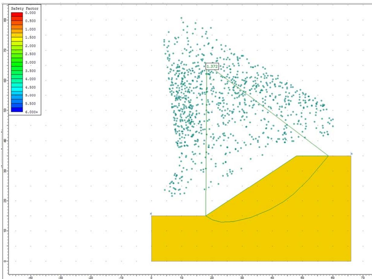
**Figure 9.4.6 – Slide Solution Using the GLE Method**
