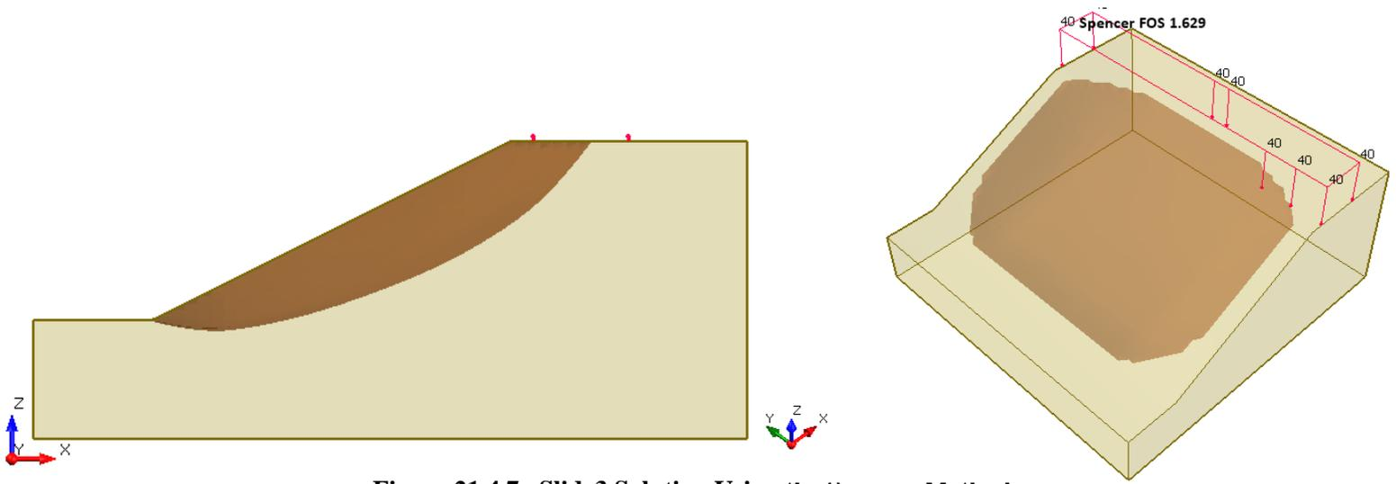
Figure 21.4.7 –Slide3 Solution Using the Spencer Method
