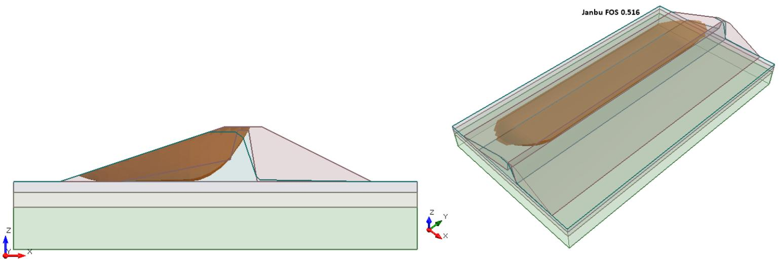
Figure 42.4.5 – Slide3 Solution Using the Janbu Method
