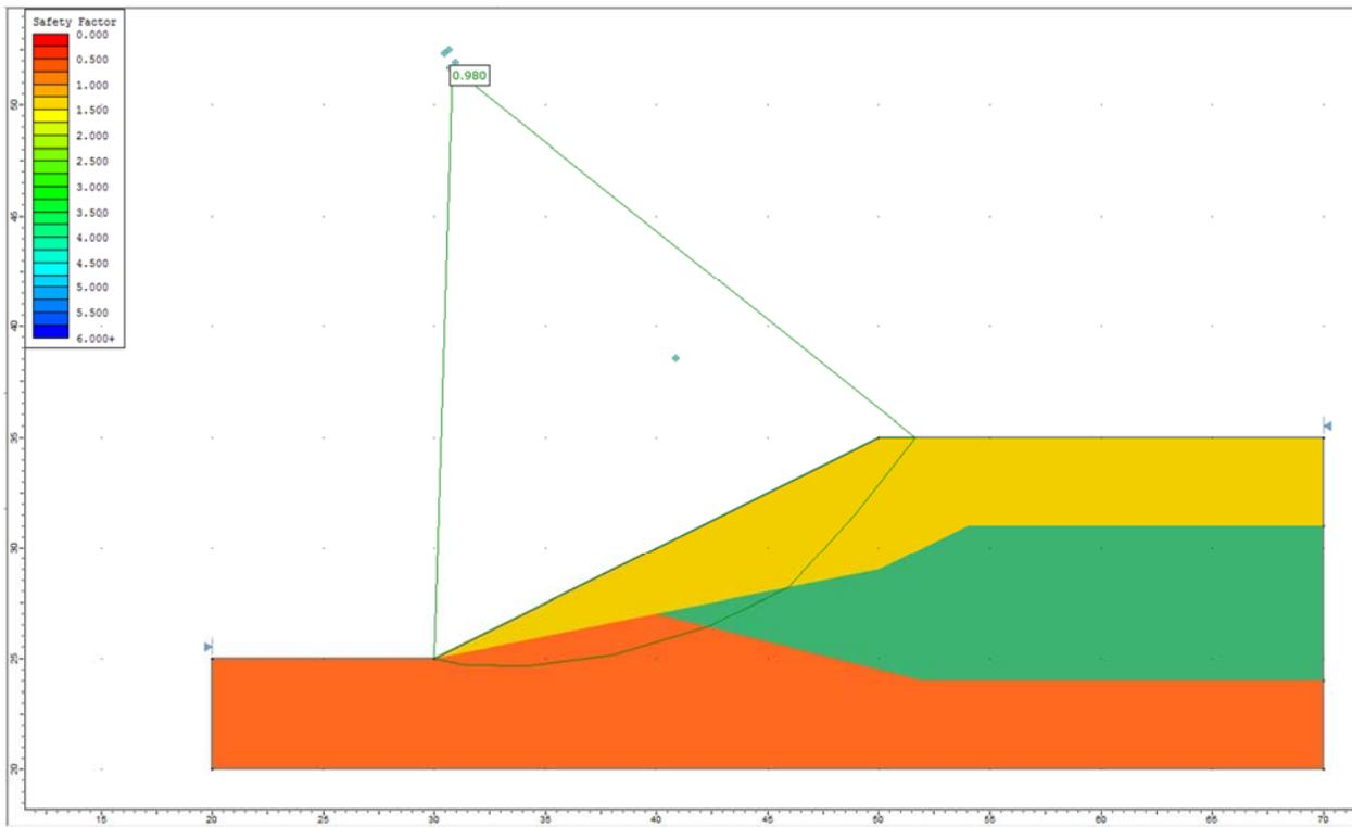
**Figure 6.4.4 – Slide Solution Using the Spencer Method**
