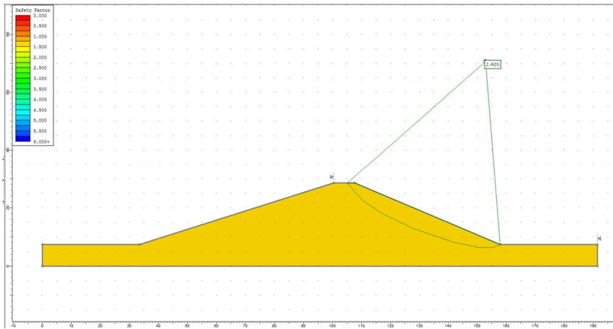
**Figure 12.4.4 – Slide Solution Using the GLE Method**
