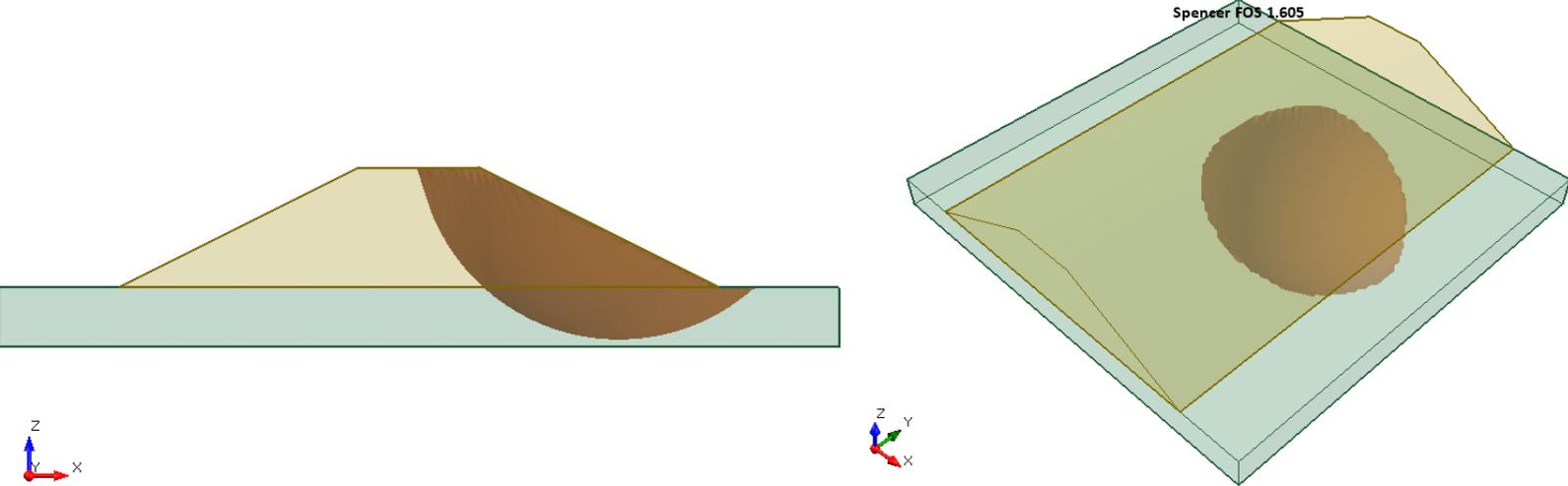
**Figure 29.4.5 – Slide3 Solution Using the Spencer Method**
