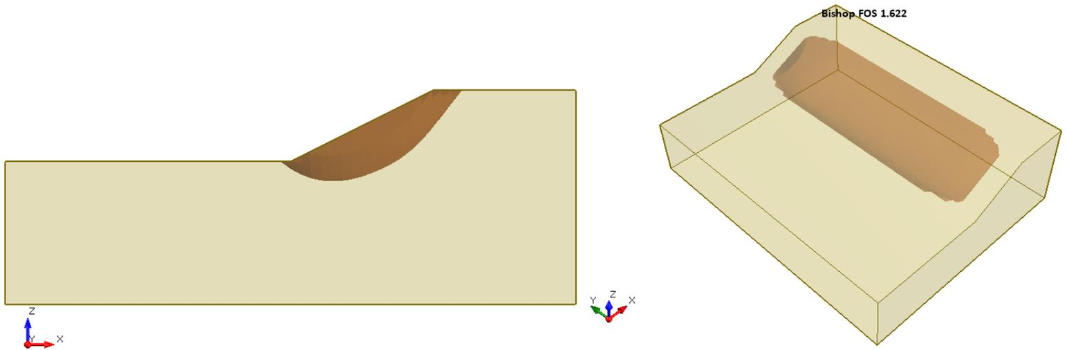
**Figure 19.4.1 – Slide3 Solution Using the Bishop Method**
