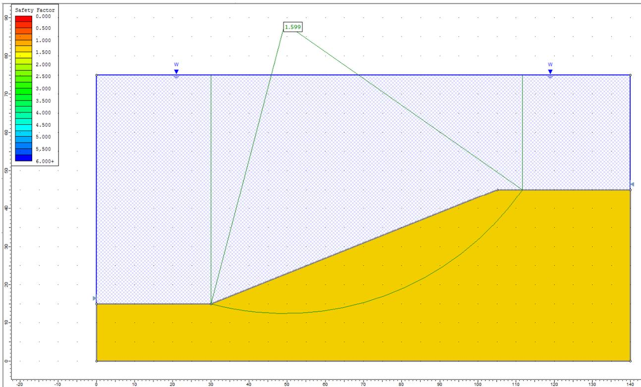
**Figure 27.4.4 – Slide Solution Using the GLE Method**
