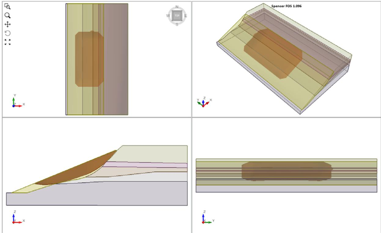
Figure 44.4.7 – Slide3 Solution Using the Spencer Method
