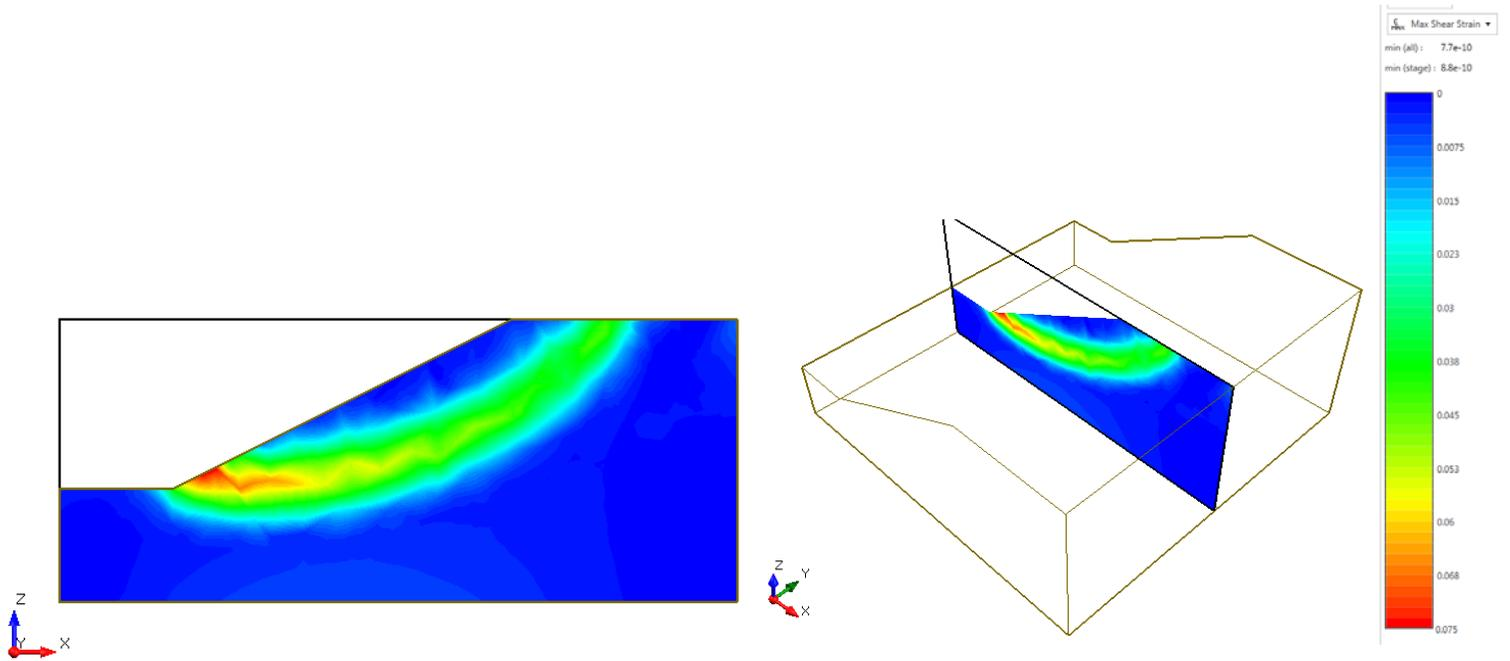
Figure 21.4.10 – RS3 Maximum Shear Strain
