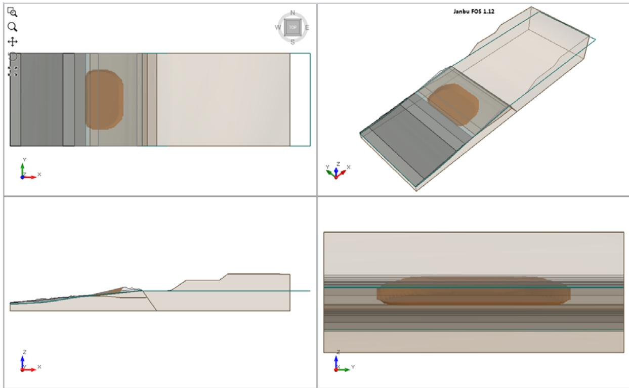
Figure 39.4.5 – Slide3 Solution Using the Janbu Method
