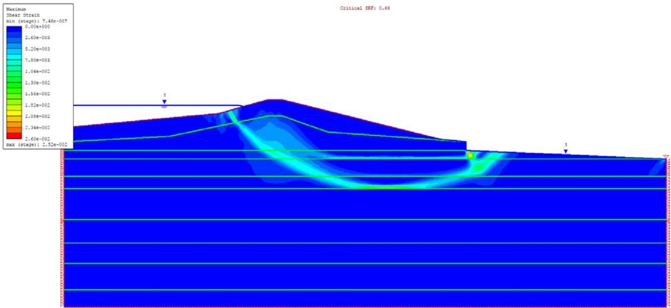
Figure 43.4.9 – RS2 Maximum Shear Strain
