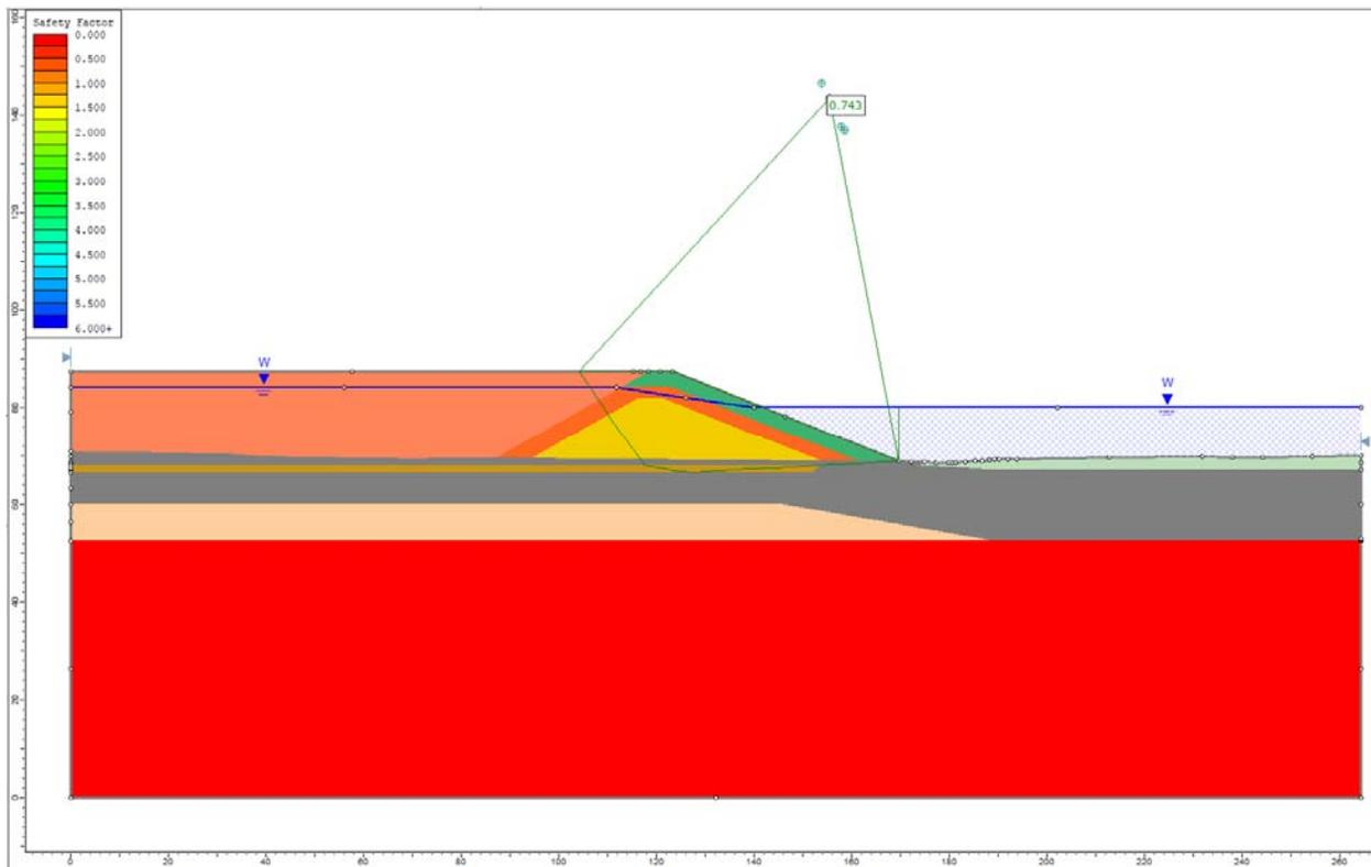
Figure 45.4.8 – Slide Solution Using the Spencer Method
