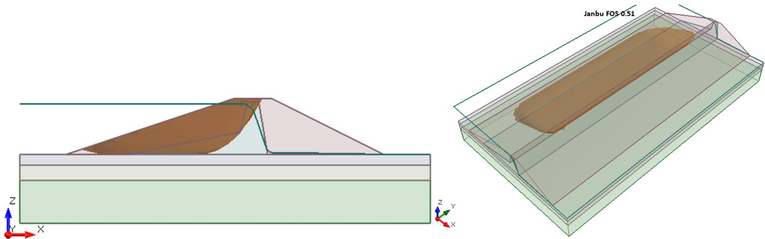
**Figure 42.5.3 – Slide3 Rapid Drawdown Using the Janbu Method**
