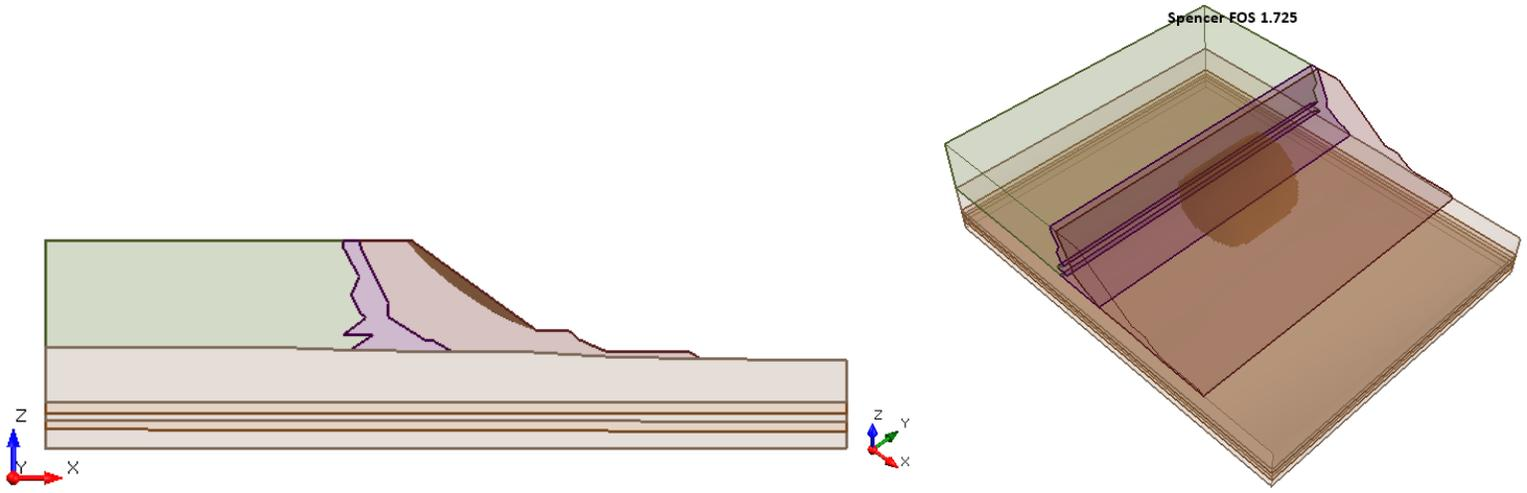
**Figure 46.4.7 – Slide3 Solution Using the Spencer Method**
