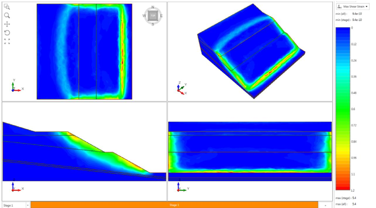
Figure 20.4.10 – RS3 Maximum Shear Strain
