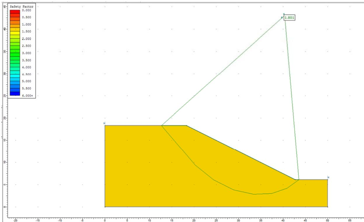
**Figure 14.4.6 – Slide Solution Using the Janbu Method**
