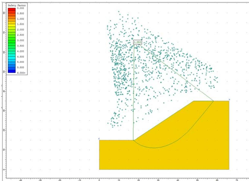
**Figure 9.4.2 – Slide Solution Using the Janbu Method**
