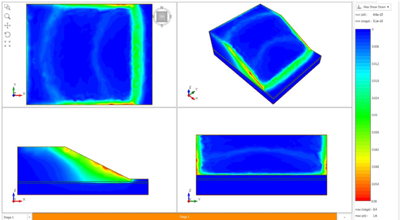
Figure 15.4.10 – RS3 Maximum Shear Strain
