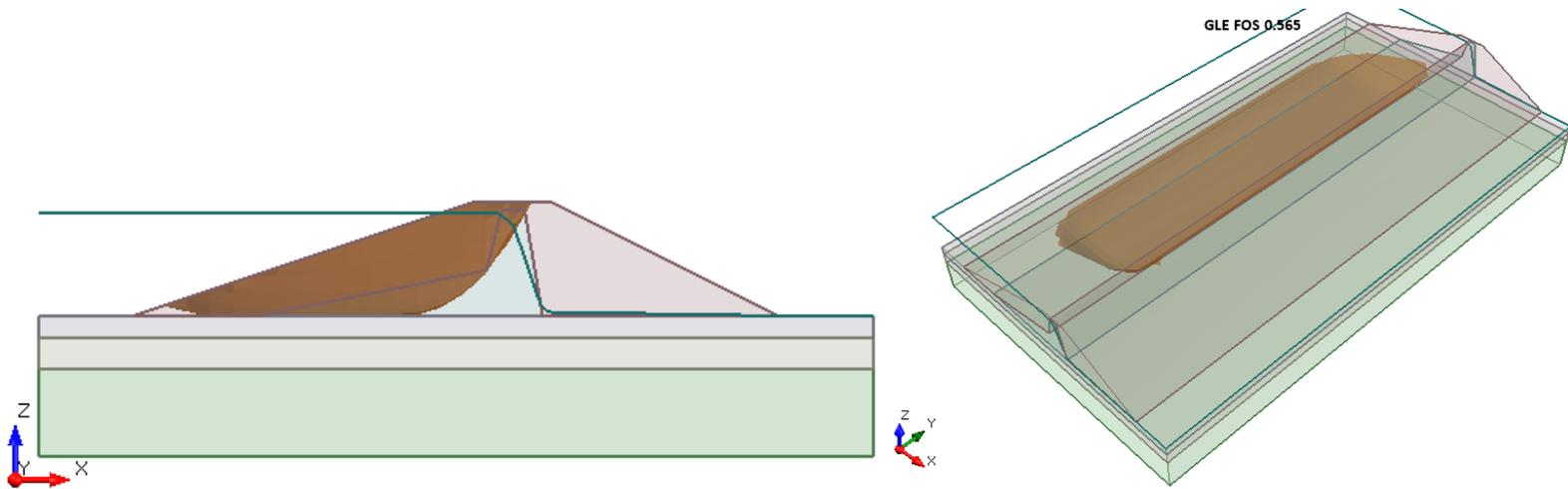
**Figure 42.5.2 – Slide3 Rapid Drawdown Using the GLE Method**
