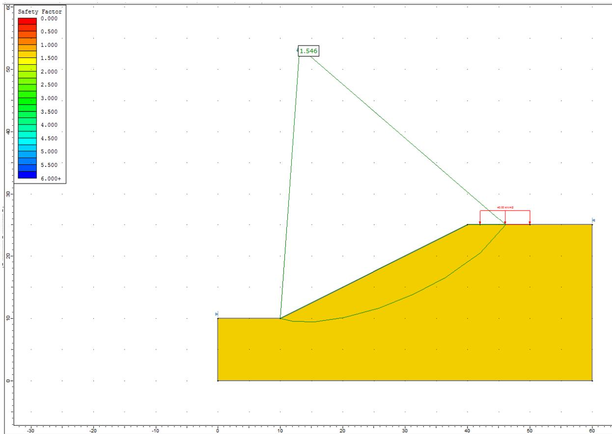
Figure 21.4.8 – Slide Solution Using the Spencer Method
