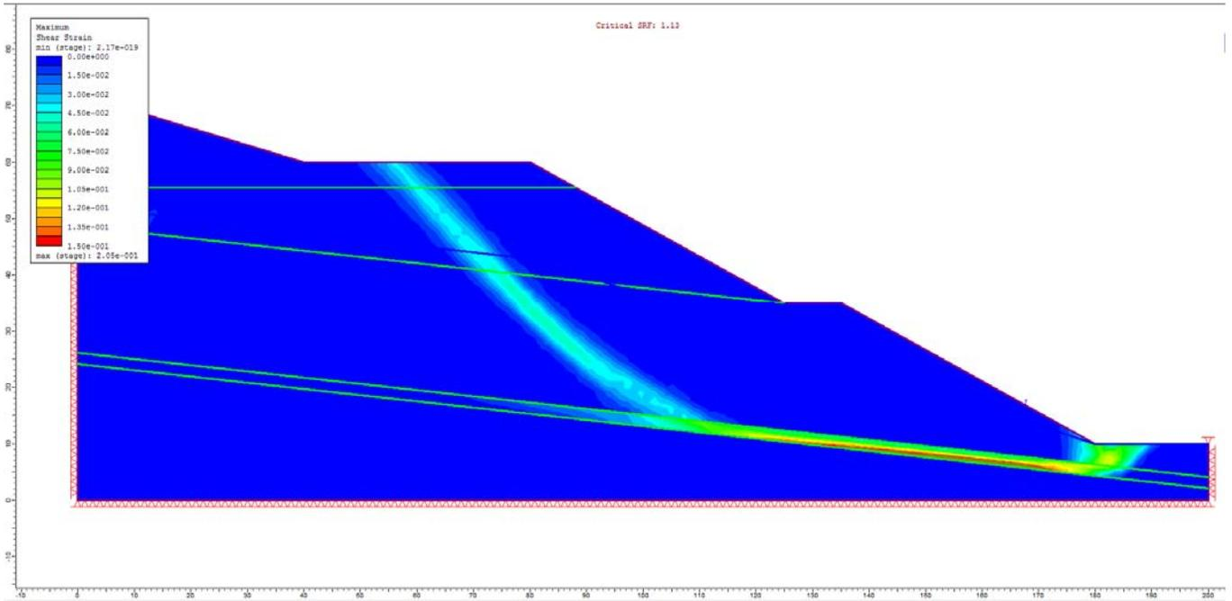
Figure 20.4.9 – RS2 Maximum Shear Strain
