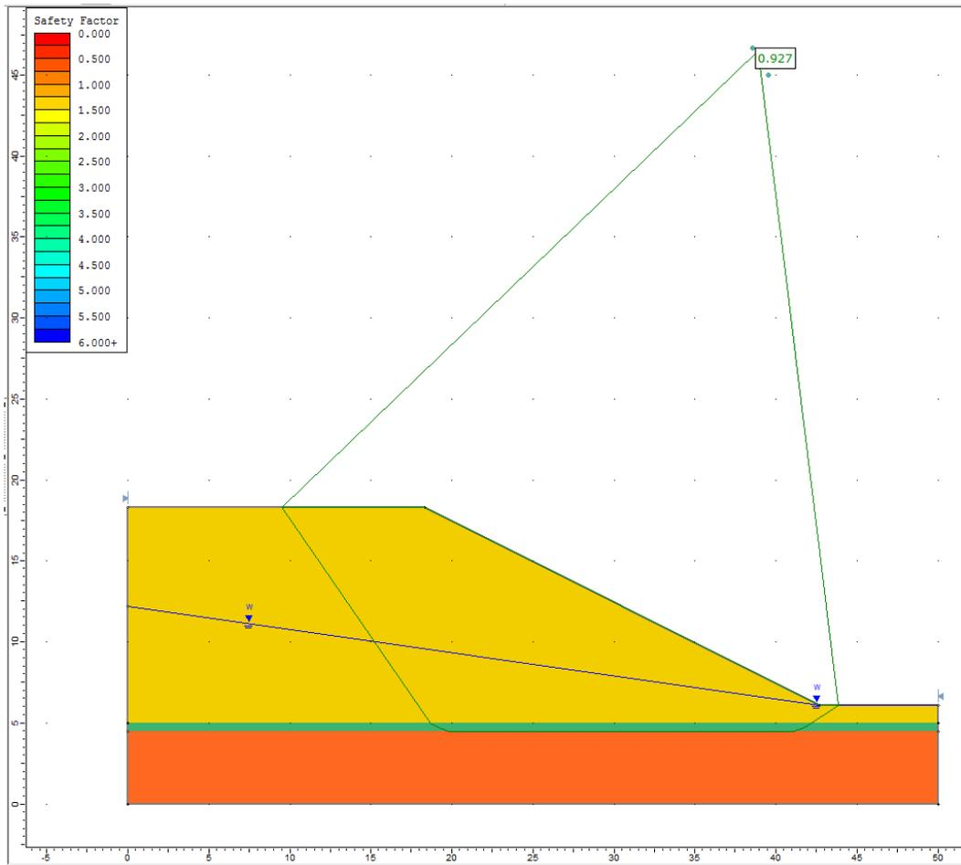
**Figure 16.4.4 – Slide Solution Using the GLE Method**
