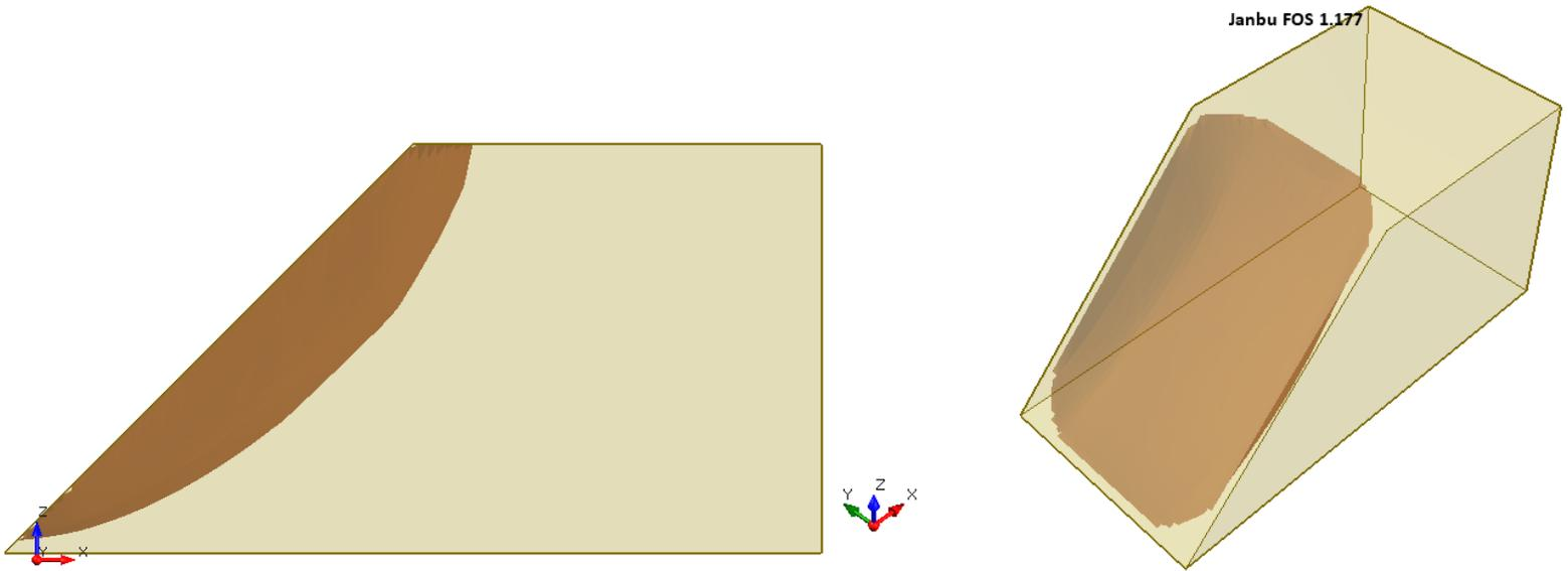
**Figure 18.4.5 – Slide3 Solution Using the Janbu Method**
