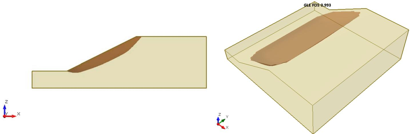
**Figure 2.4.5 – Slide3 Solution Using the GLE Method**
