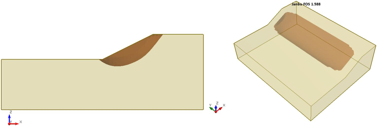
**Figure 19.4.5 – Slide3 Solution Using the Janbu Method**
