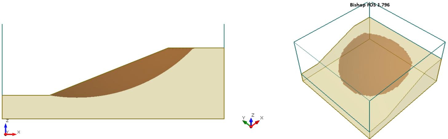
**Figure 27.4.1 – Slide3 Solution Using the Bishop Method**
