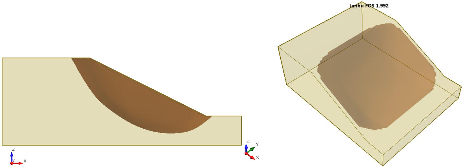
**Figure 14.4.5 – Slide3 Solution Using the Janbu Method**
