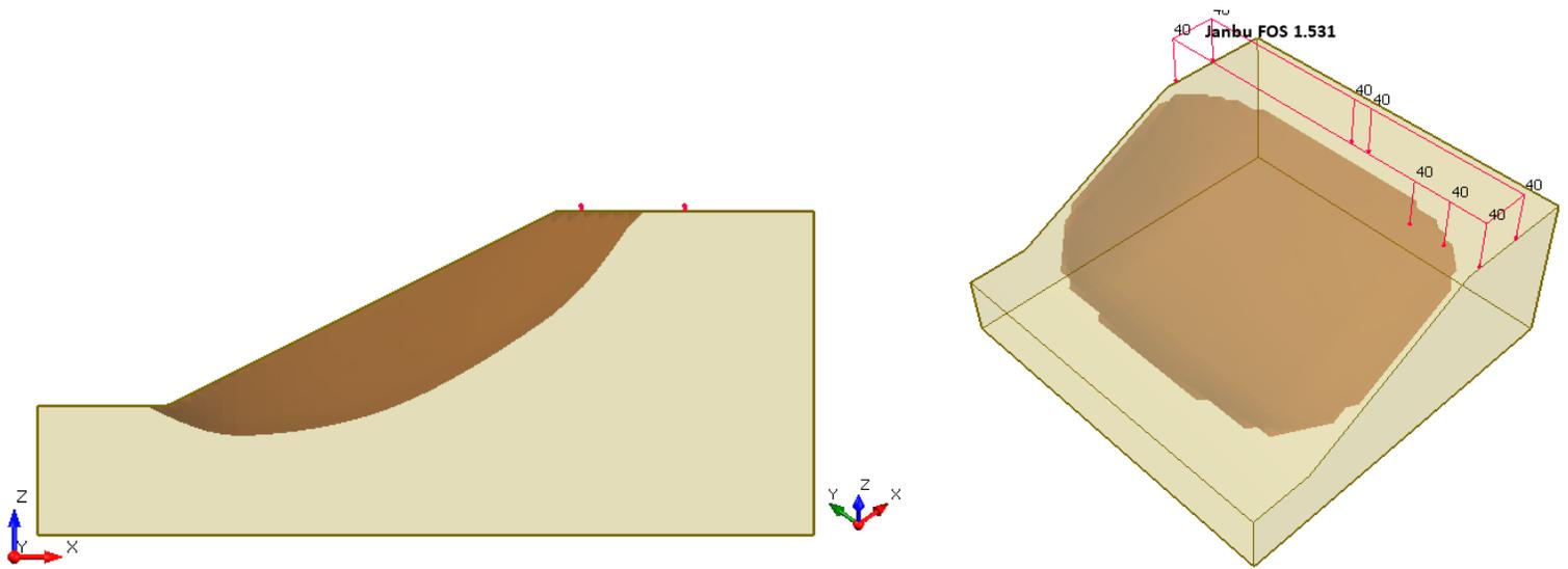
Figure 21.4.5 – Slide3 Solution Using the Janbu Method
