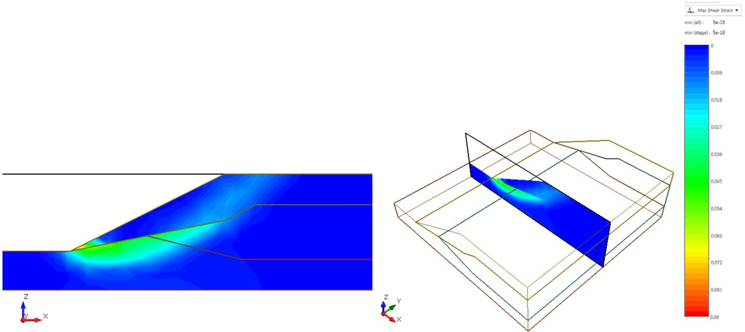
Figure 4.4.8 – RS3 Maximum Shear Strain
