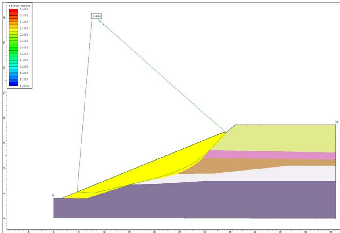
Figure 44.4.8 – Slide Solution Using the Spencer Method
