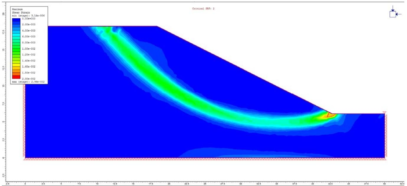
Figure 14.4.9 – RS2 Maximum Shear Strain
