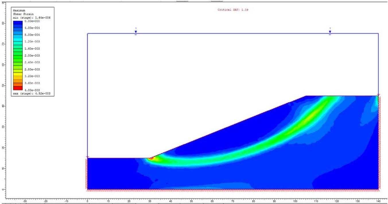
Figure 27.4.7 – RS2 Maximum Shear Strain
