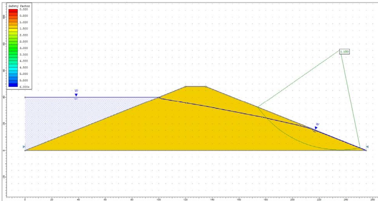
**Figure 30.4.6 – Slide Solution Using the Spencer Method**
