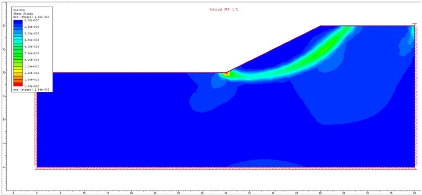
Figure 19.4.9 – RS2 Maximum Shear Strain
