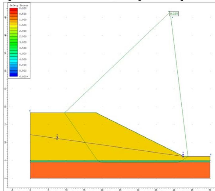
**Figure 16.4.2 – Slide Solution Using the Bishop Method**
