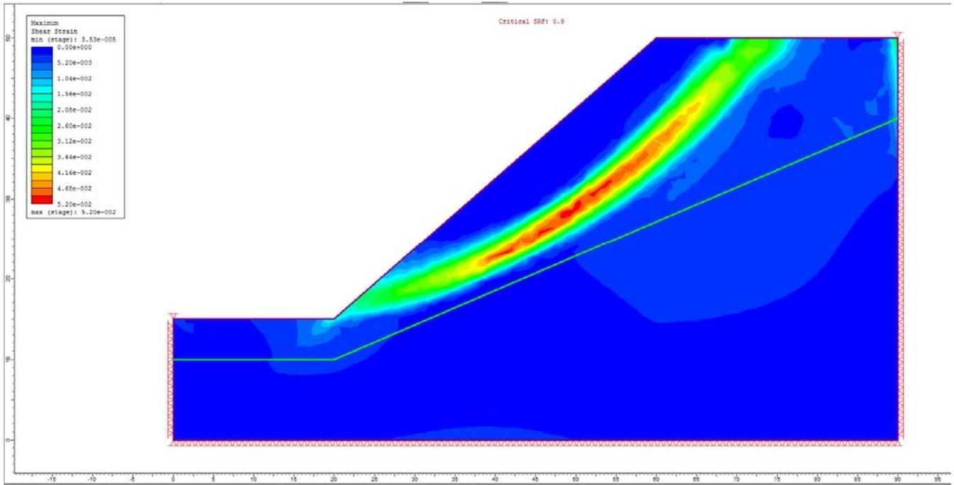
Figure 17.4.9 – RS2 Maximum Shear Strain
