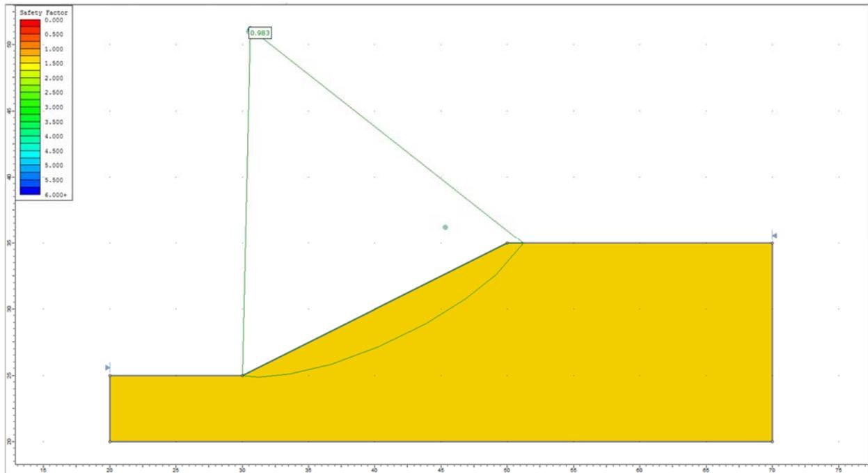
**Figure 2.4.4 – Slide Solution Using the Spencer Method**
