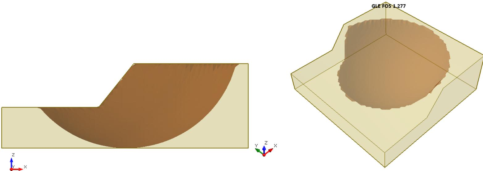
**Figure 36.4.3 – Slide3 Solution Using the GLE Method**
