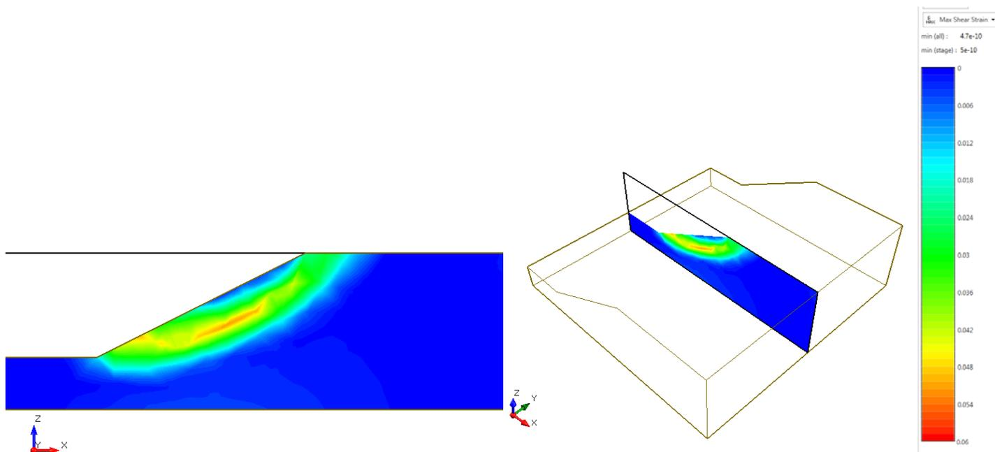
Figure 1.4.8 – RS3 Maximum Shear Strain
