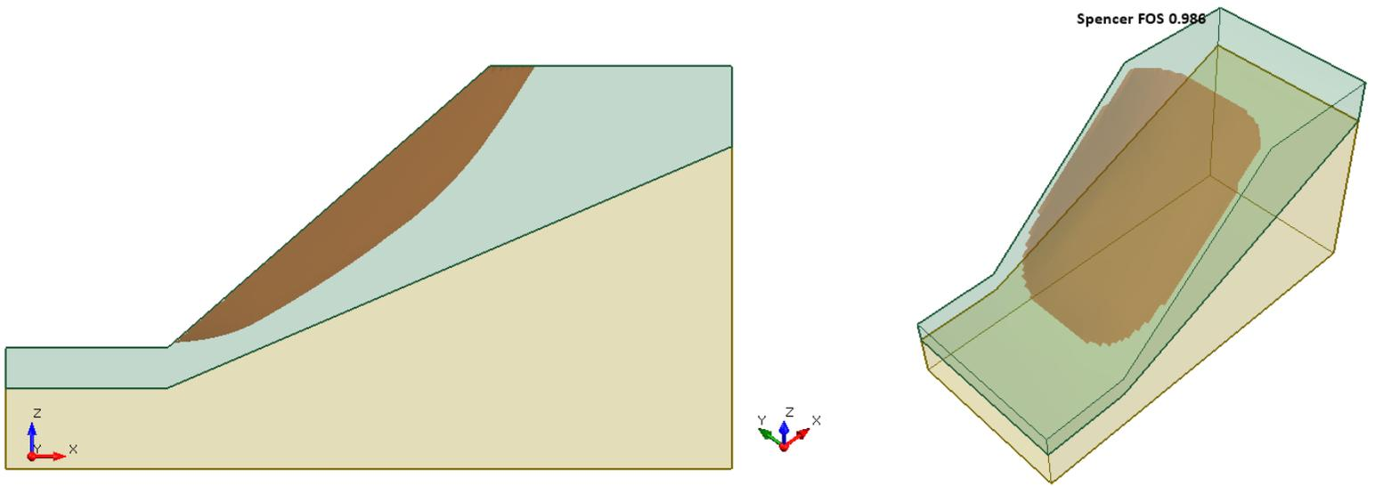
**Figure 17.4.7 – Slide3 Solution Using the Spencer Method**
