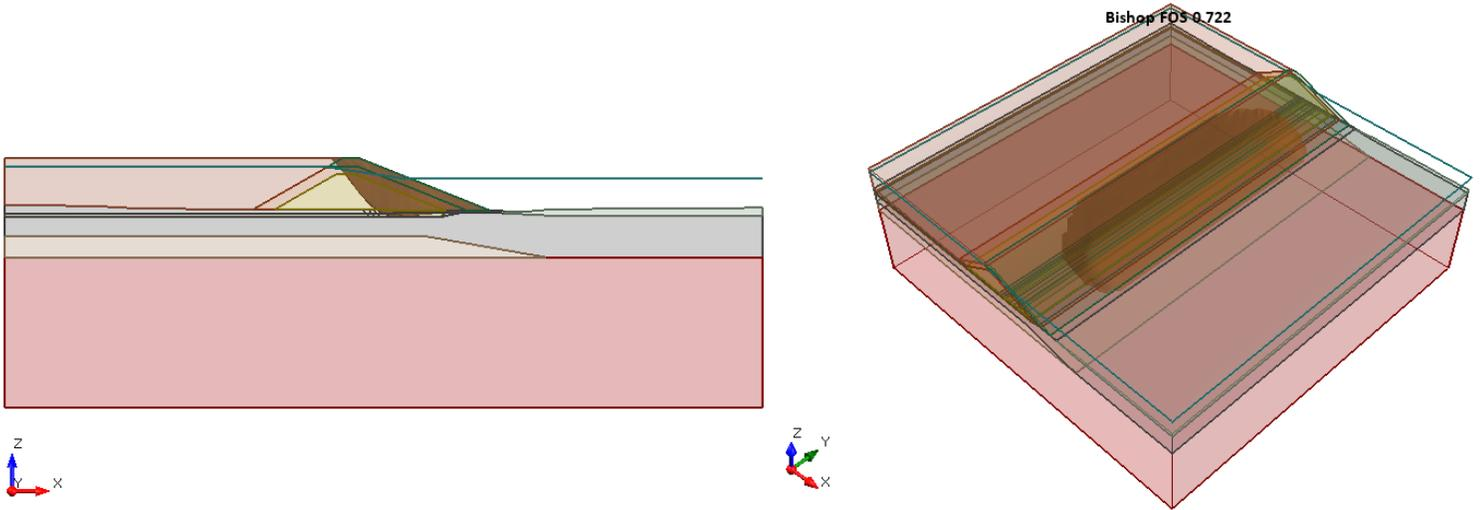
**Figure 45.4.1 – Slide3 Solution Using the Bishop Method**
