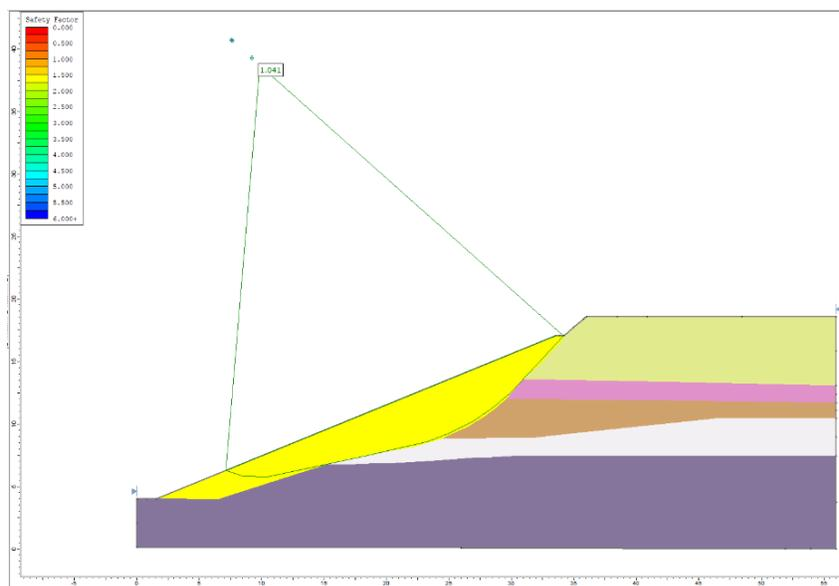
**Figure 44.4.2 – Slide Solution Using the Bishop Method**
