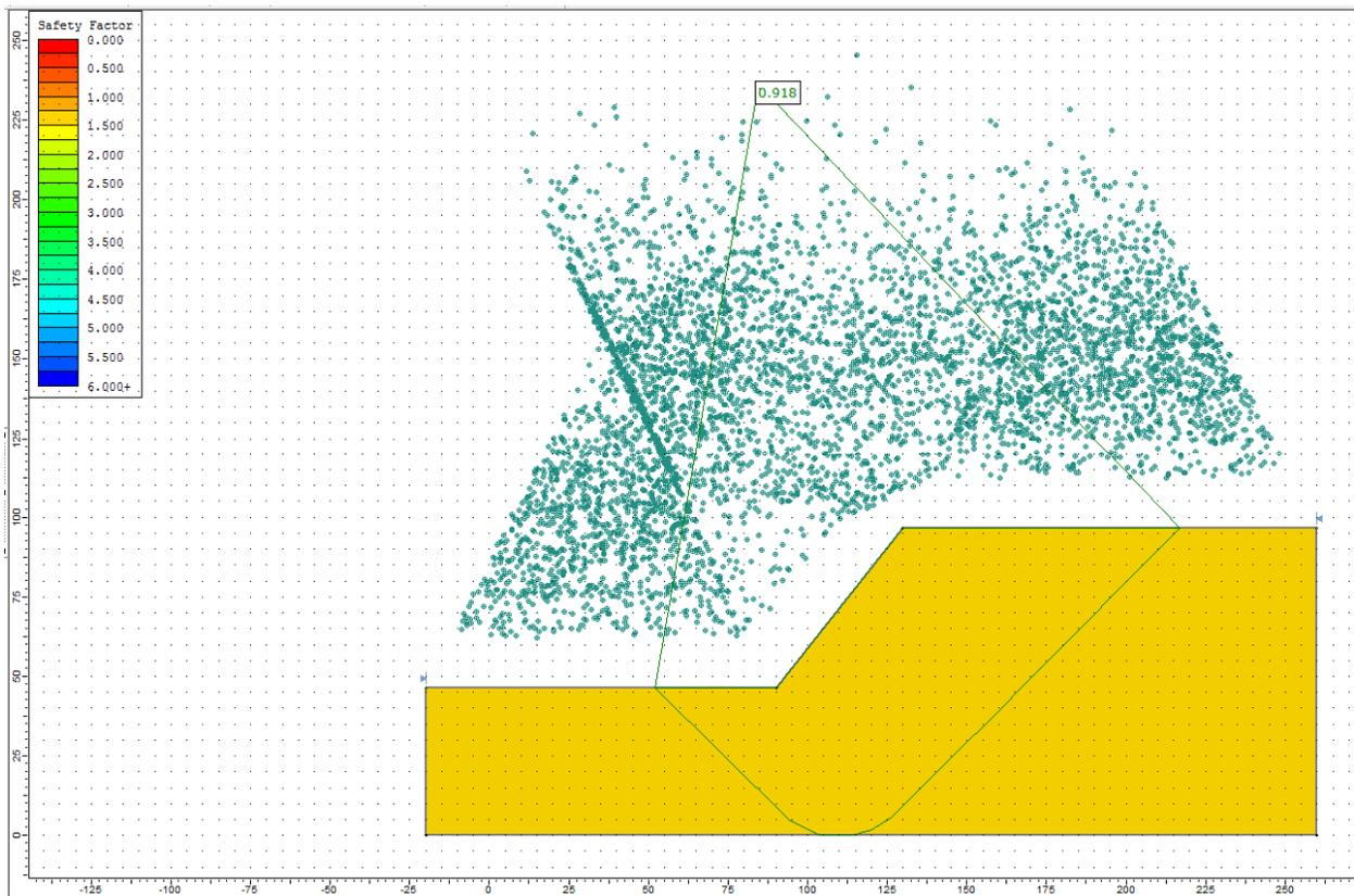
**Figure 37.4.4 – Slide Solution Using the GLE Method**
