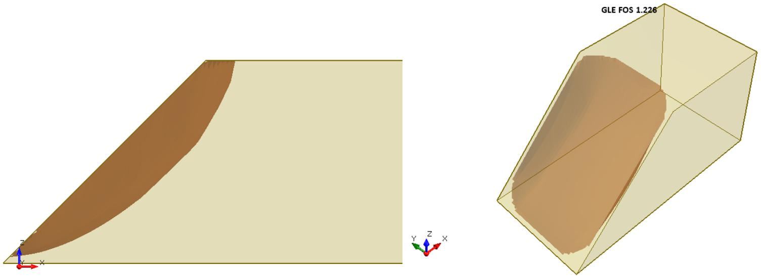
**Figure 18.4.3 – Slide3 Solution Using the GLE Method**
