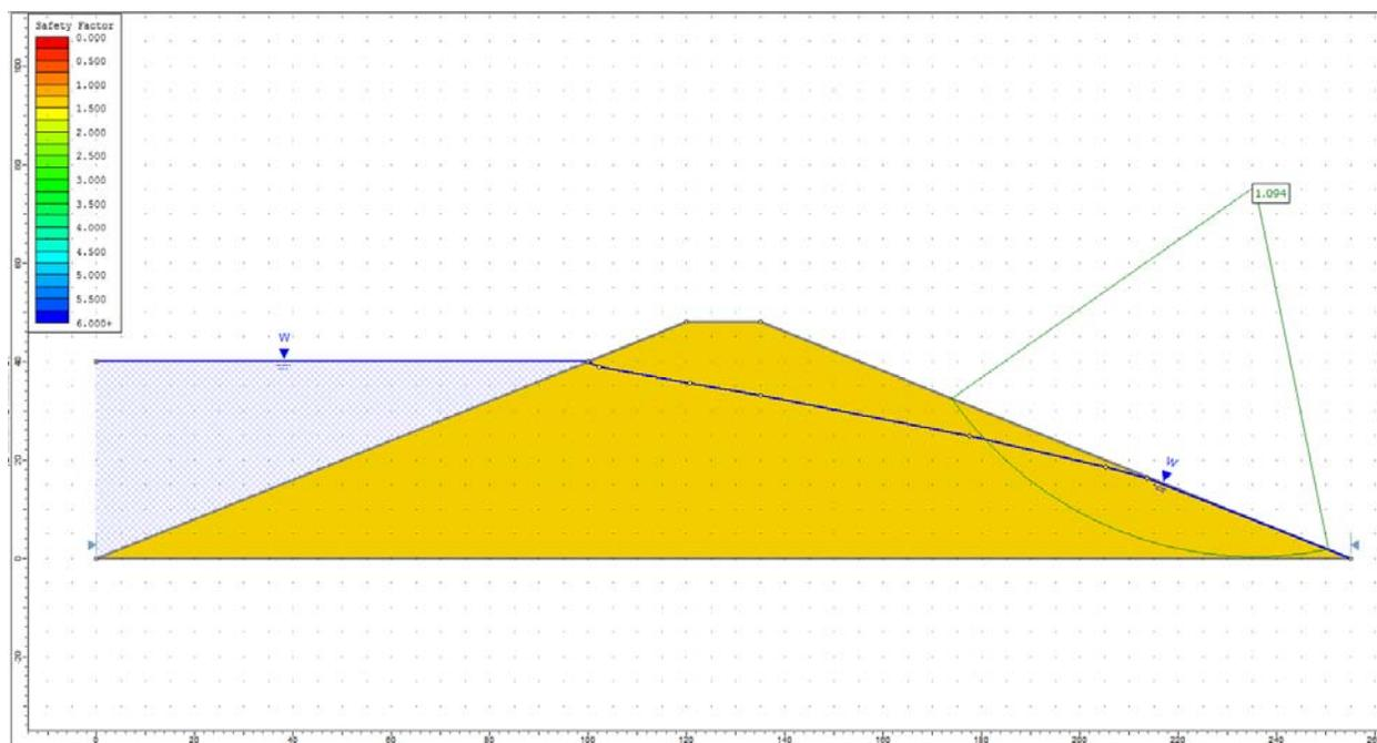
**Figure 30.4.4 – Slide Solution Using the GLE Method**
