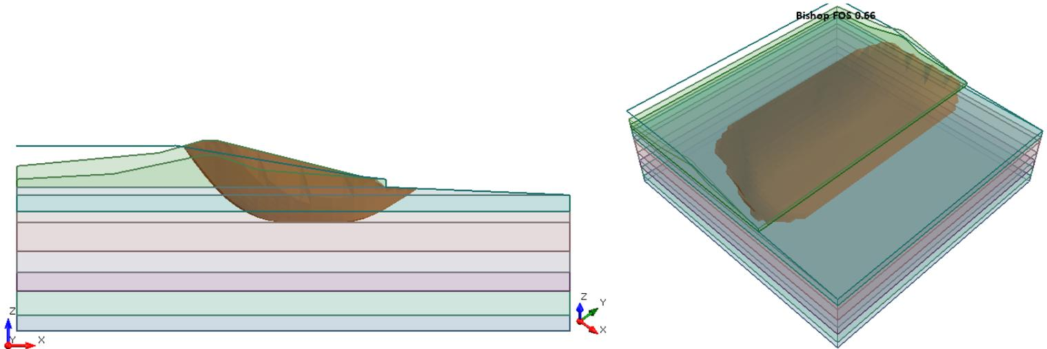
Figure 43.4.1 – Slide3 Solution Using the Bishop Method
