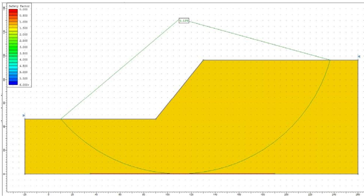
**Figure 36.4.6 – Slide Solution Using the Spencer Method**
