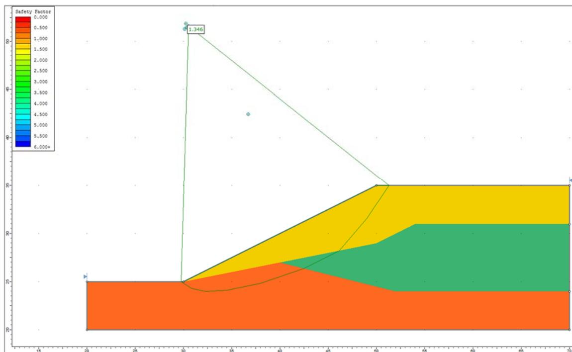
Figure 4.4.6 – Slide Solution Using the GLE Method
