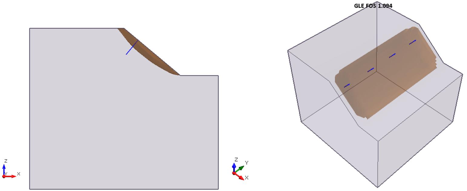
**Figure 22.4.3 – Slide3 Solution Using the GLE Method**
