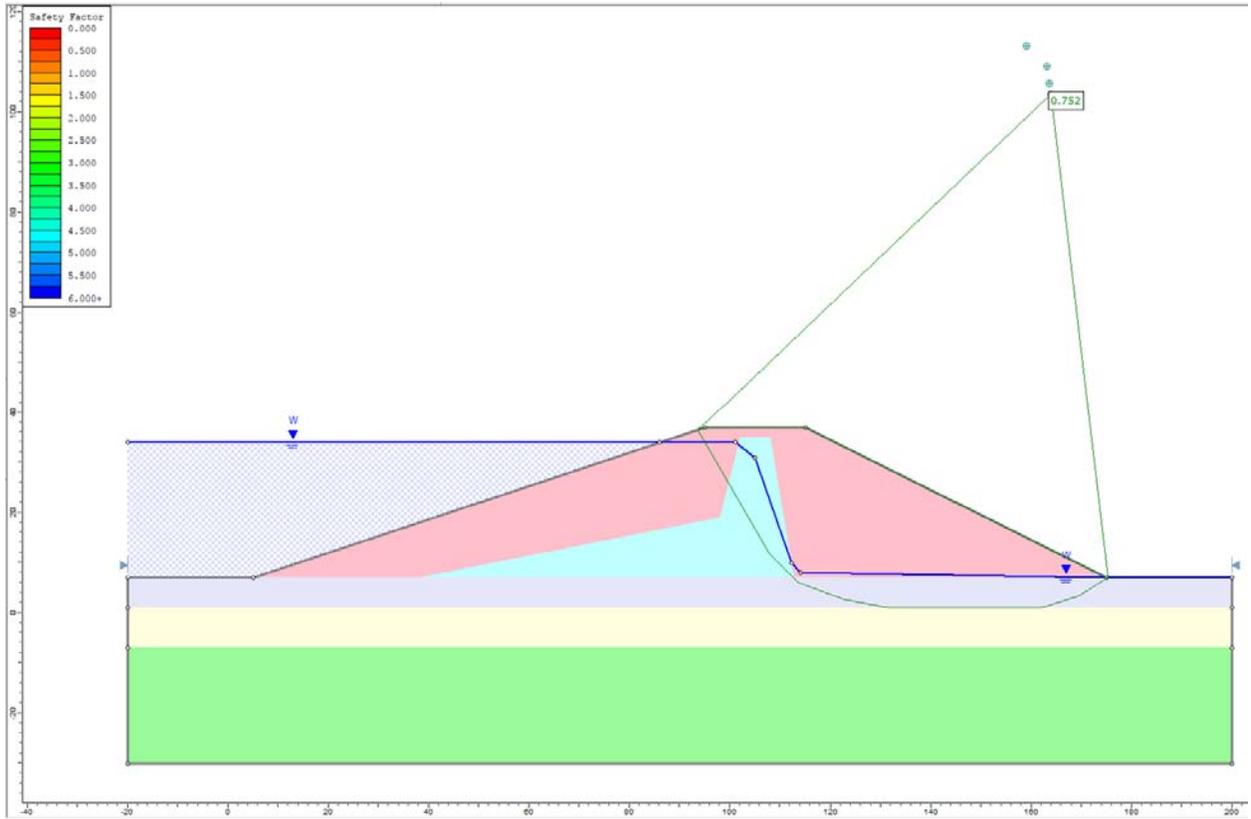
Figure 41.4.2 – Slide Solution Using the Bishop Method
