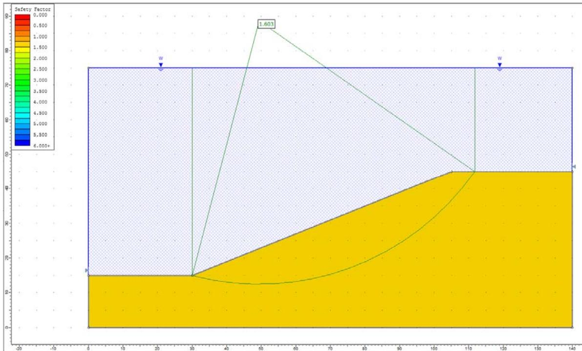
**Figure 27.4.2 – Slide Solution Using the Bishop Method**
