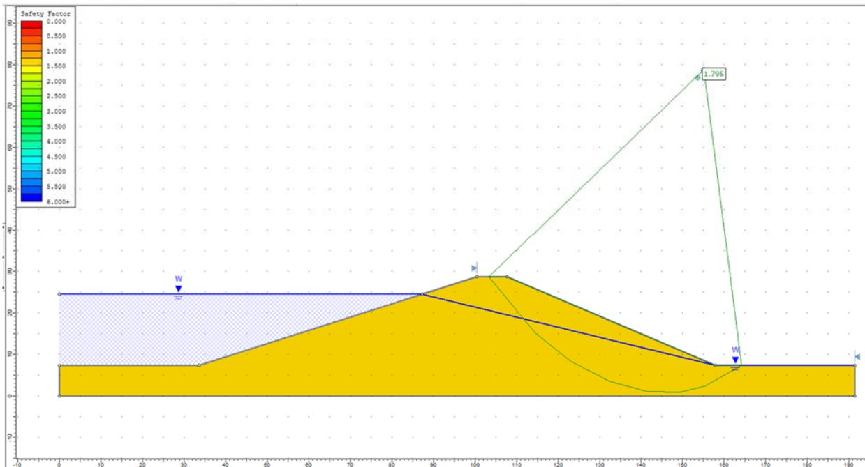
**Figure 13.4.2 – Slide Solution Using the Bishop method**
