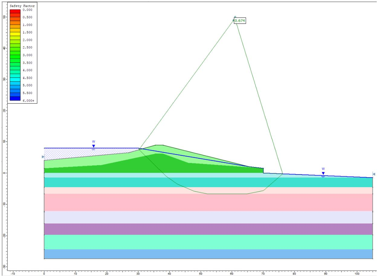
Figure 43.4.4 – Slide Solution Using the GLE Method
