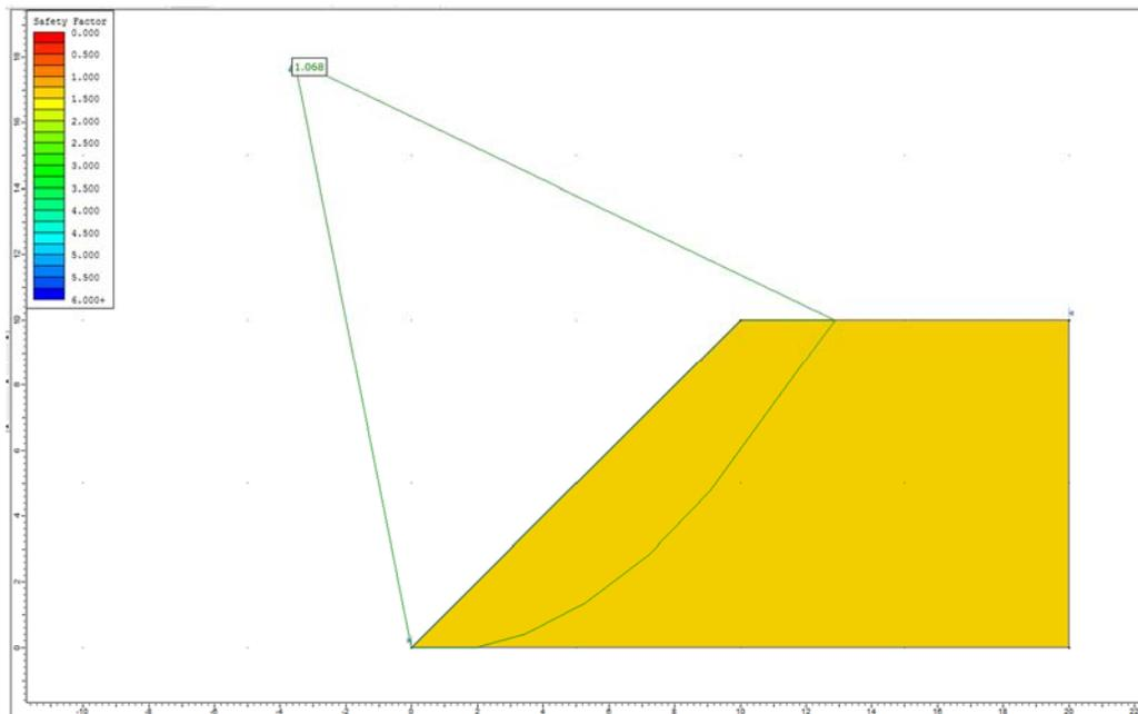
**Figure 18.4.2 – Slide Solution Using the Bishop Method**
