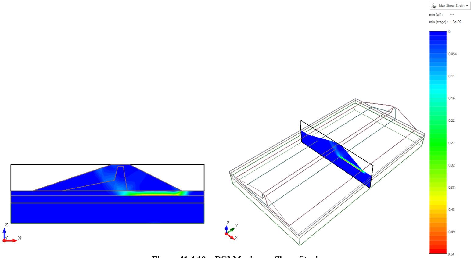
**Figure 41.4.10 – RS3 Maximum Shear Strain**
