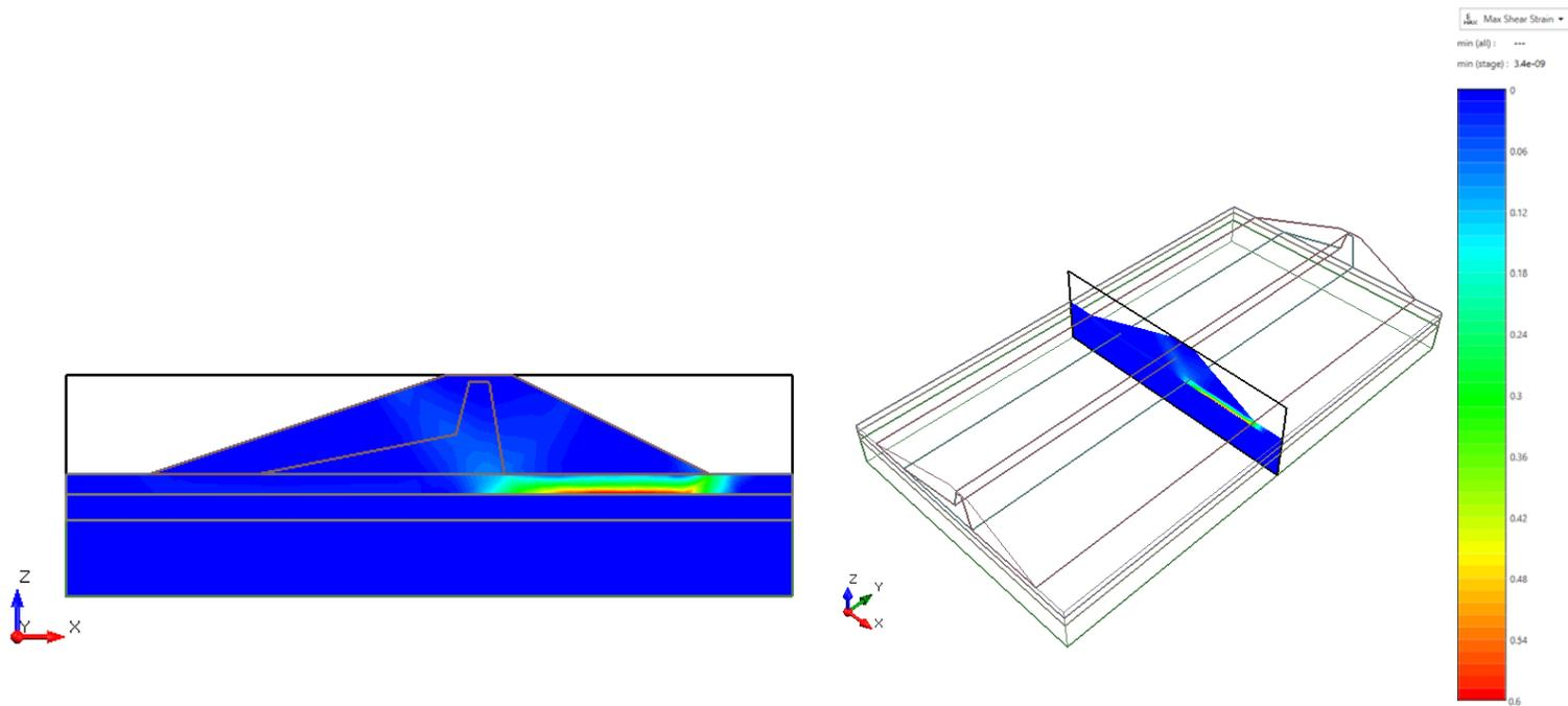
**Figure 40.4.10 – RS3 Maximum Shear Strain**
