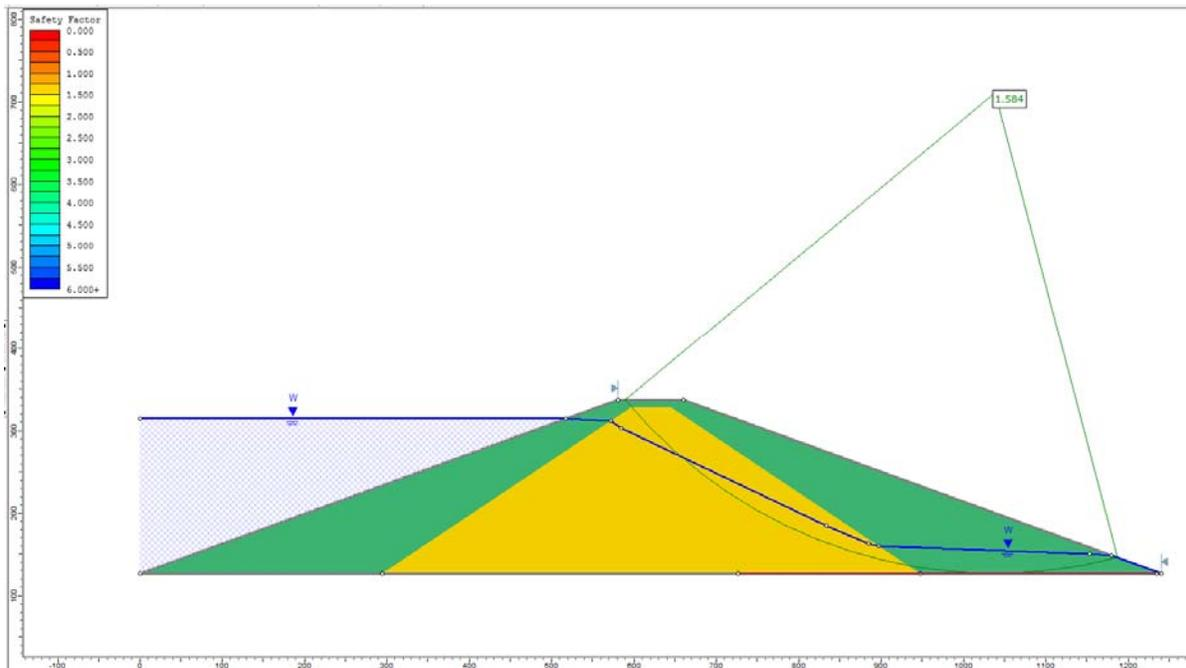
**Figure 32.4.2 – Slide Solution Using the Bishop Method**
