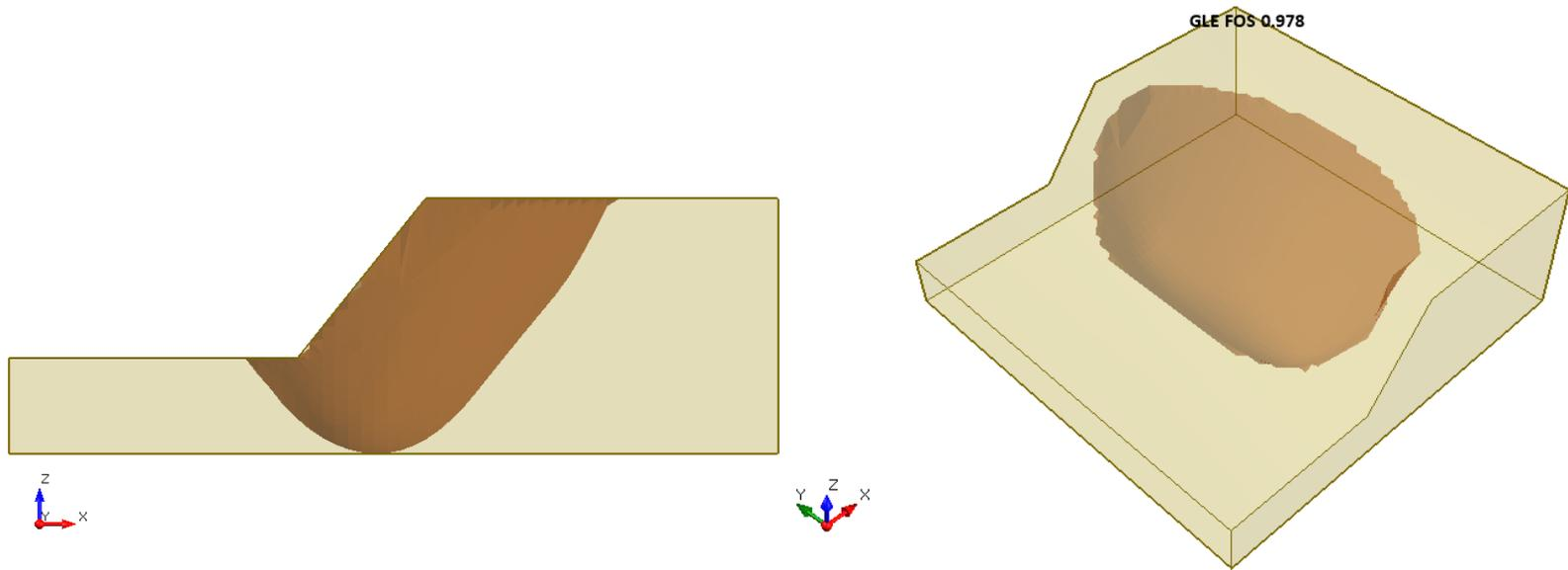
**Figure 35.4.3 – Slide3 Solution Using the GLE Method**
