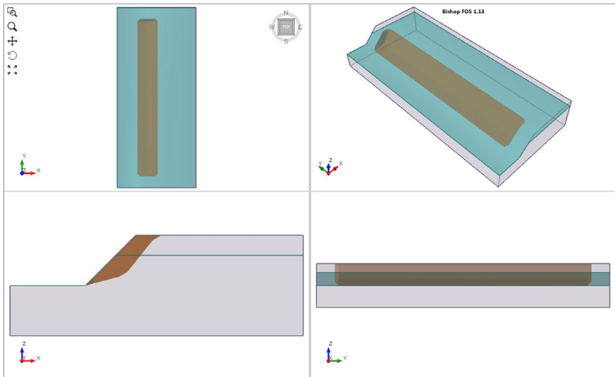
**Figure 26.4.1 – Slide3 User Defined Slip Surface Using Weak Planes**
