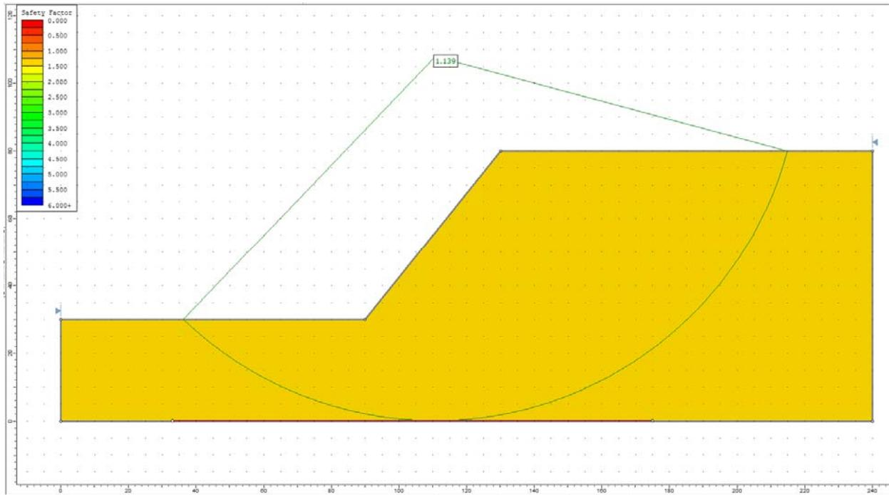
**Figure 34.4.4 – Slide Solution Using the GLE Method**
