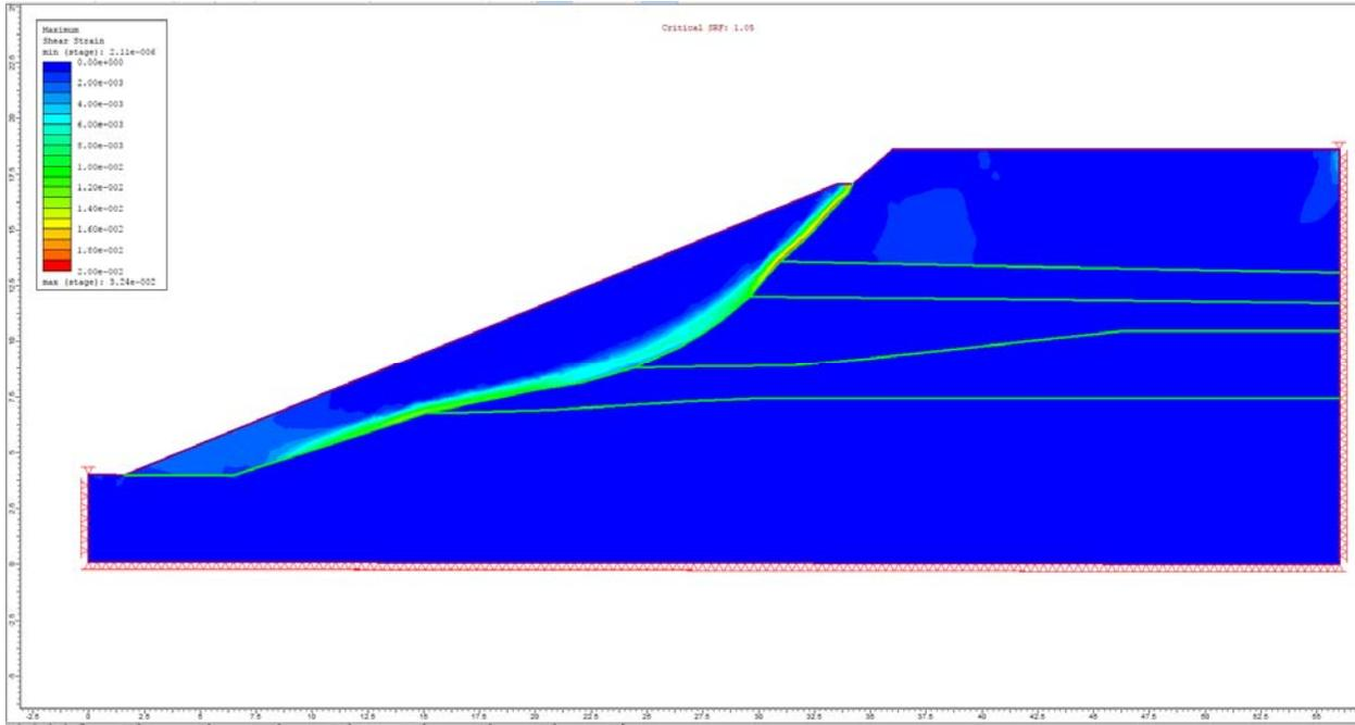
Figure 44.4.9 – RS2 Maximum Shear Strain
