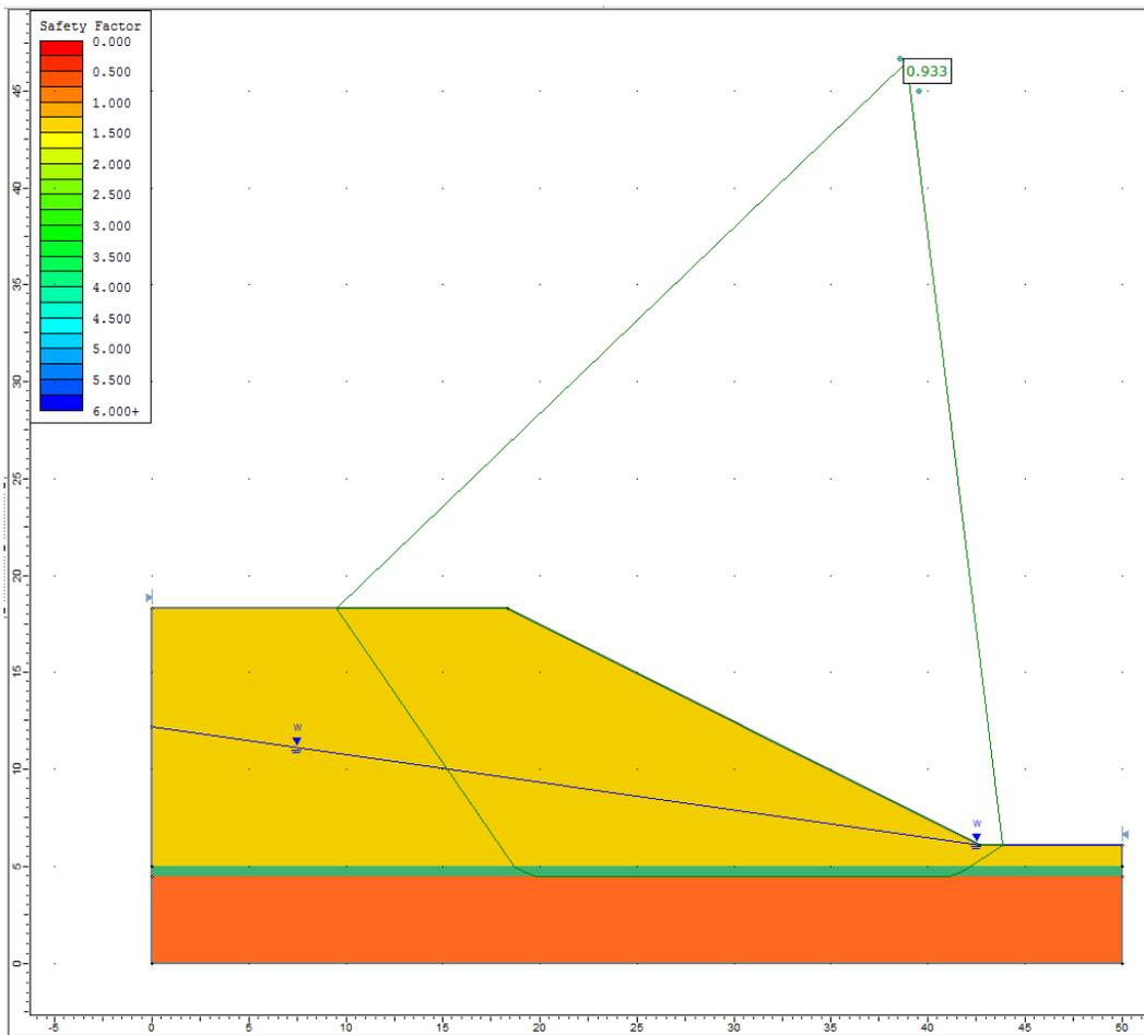
Figure 16.4.6 – Slide Solution Using the Janbu Method
