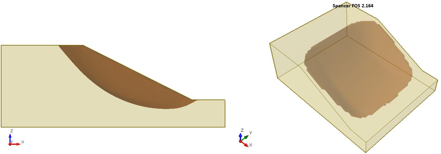
**Figure 14.4.7 – Slide3 Solution Using the Spencer Method**
