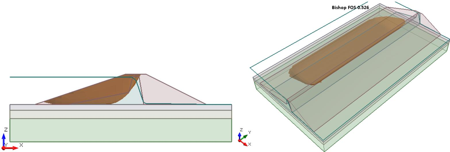
**Figure 42.5.1 – Slide3 Rapid Drawdown Using the Bishop Method**
