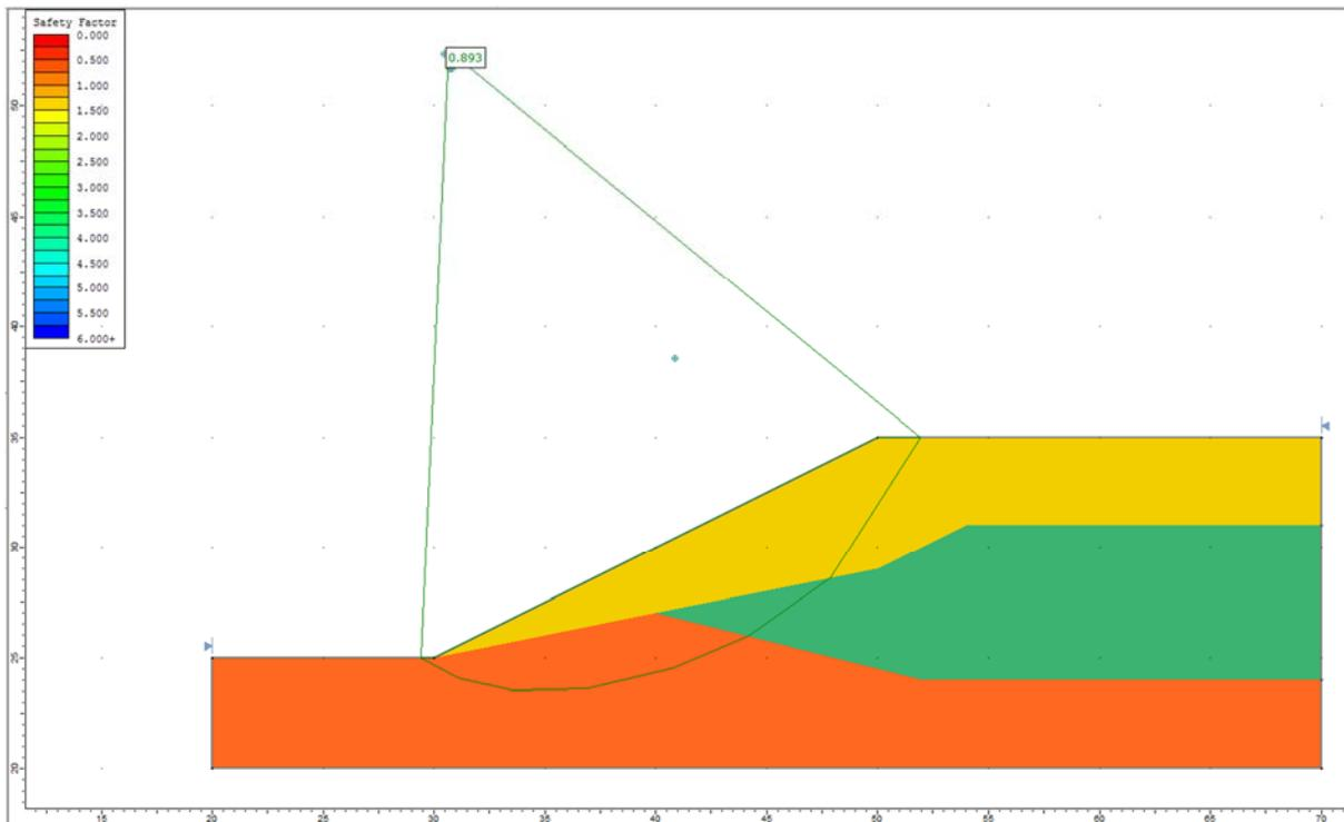
**Figure 6.4.2 – Slide Solution Using the Janbu Method**
