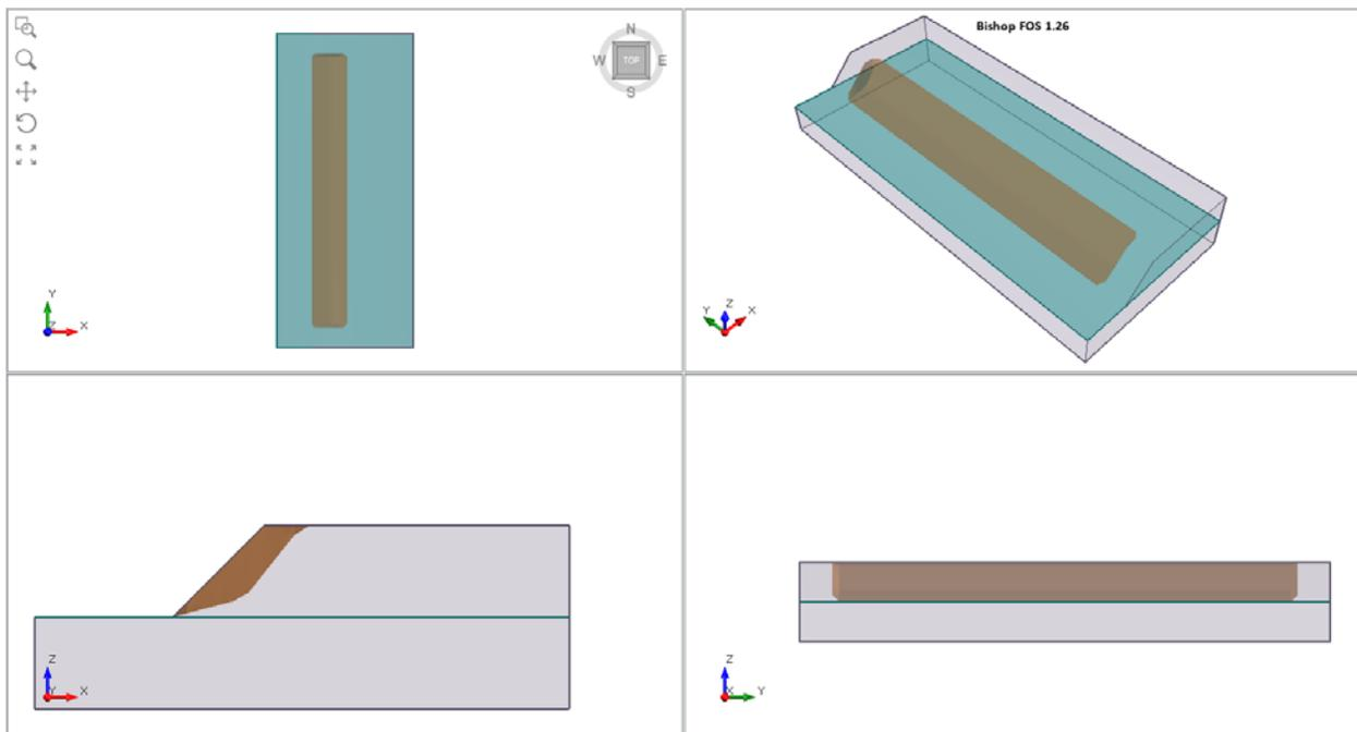
**Figure 23.4.1 – Slide3 User Defined Slip Surface Using Weak Planes**
