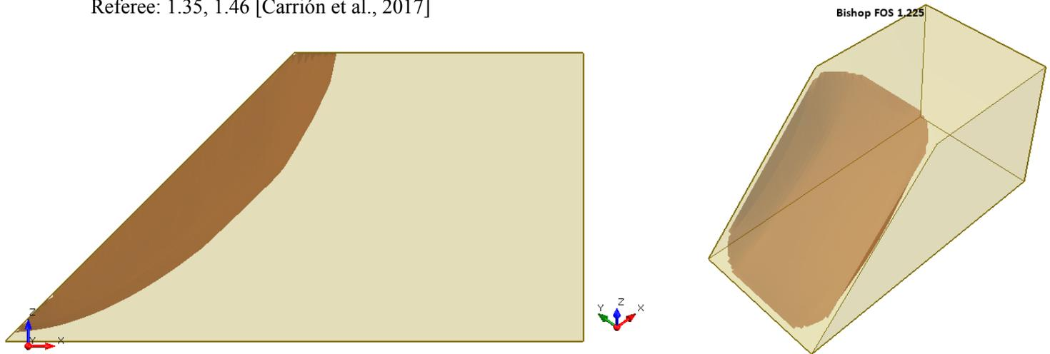
**Figure 18.4.1 – Slide3 Solution Using the Bishop Method**
