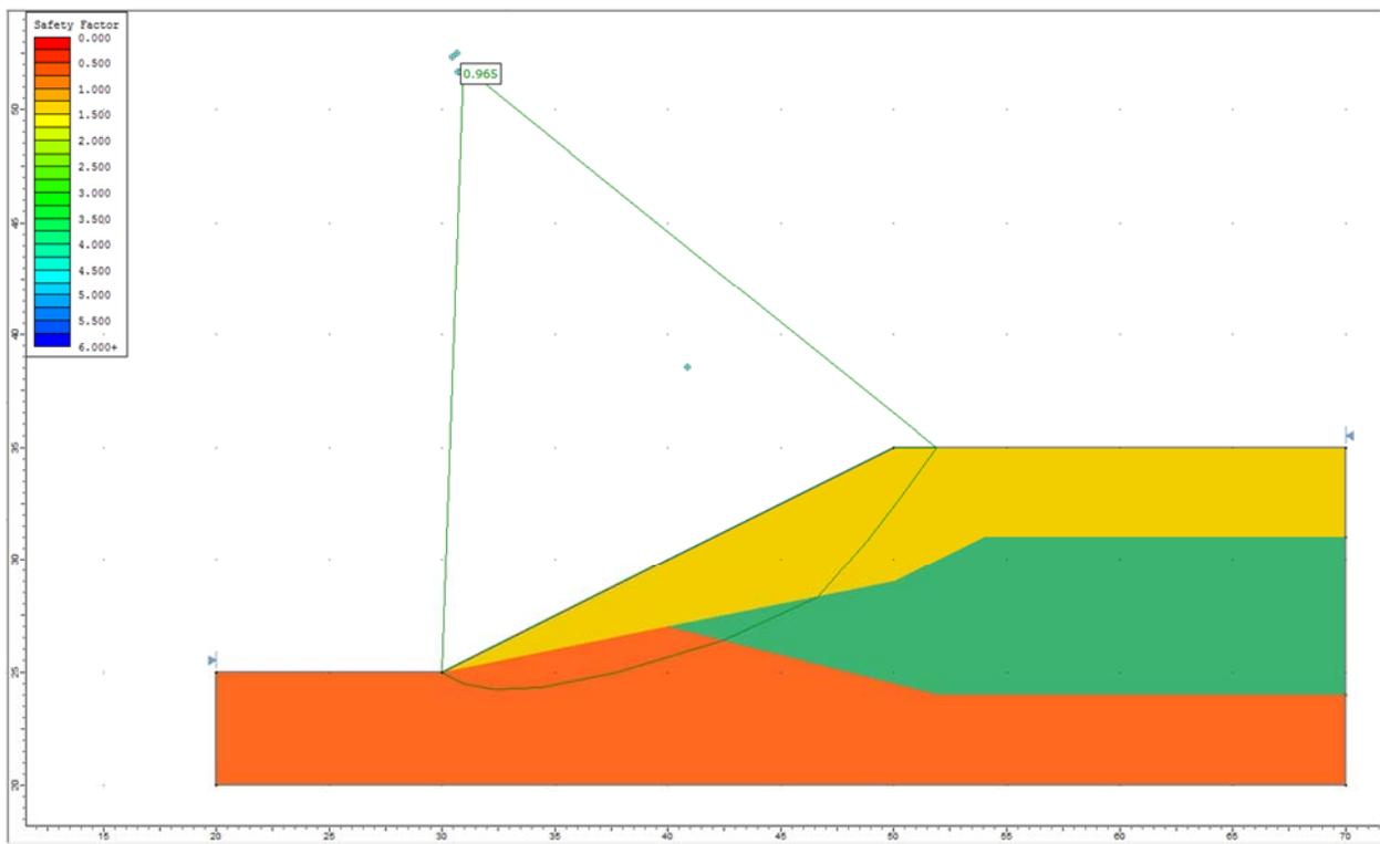
Figure 6.4.6 – Slide Solution Using the GLE Method
