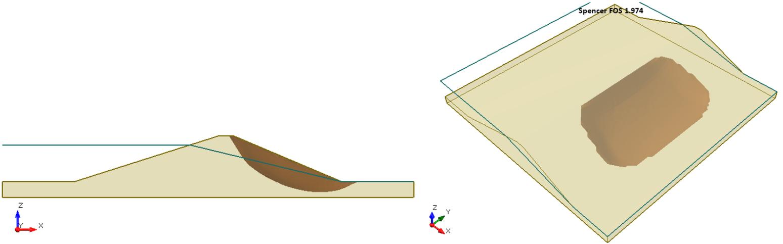
**Figure 13.4.7 – Slide3 Solution Using the Spencer Method**
