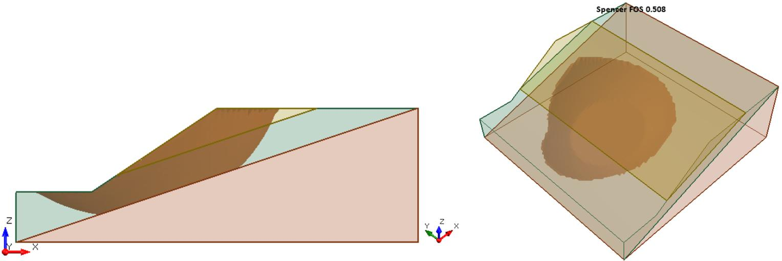
Figure 10.4.3 – Slide3 Solution Using the Spencer Method
