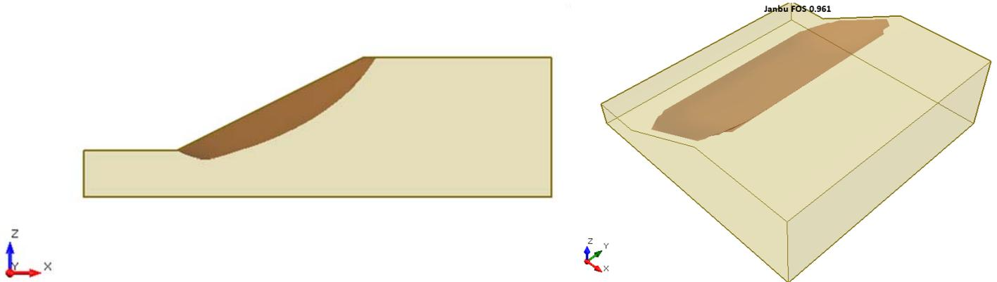
**Figure 2.4.1 – Slide3 Solution Using the Janbu Method**
