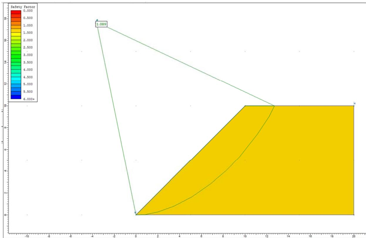
**Figure 18.4.8 – Slide Solution Using the Spencer Method**
