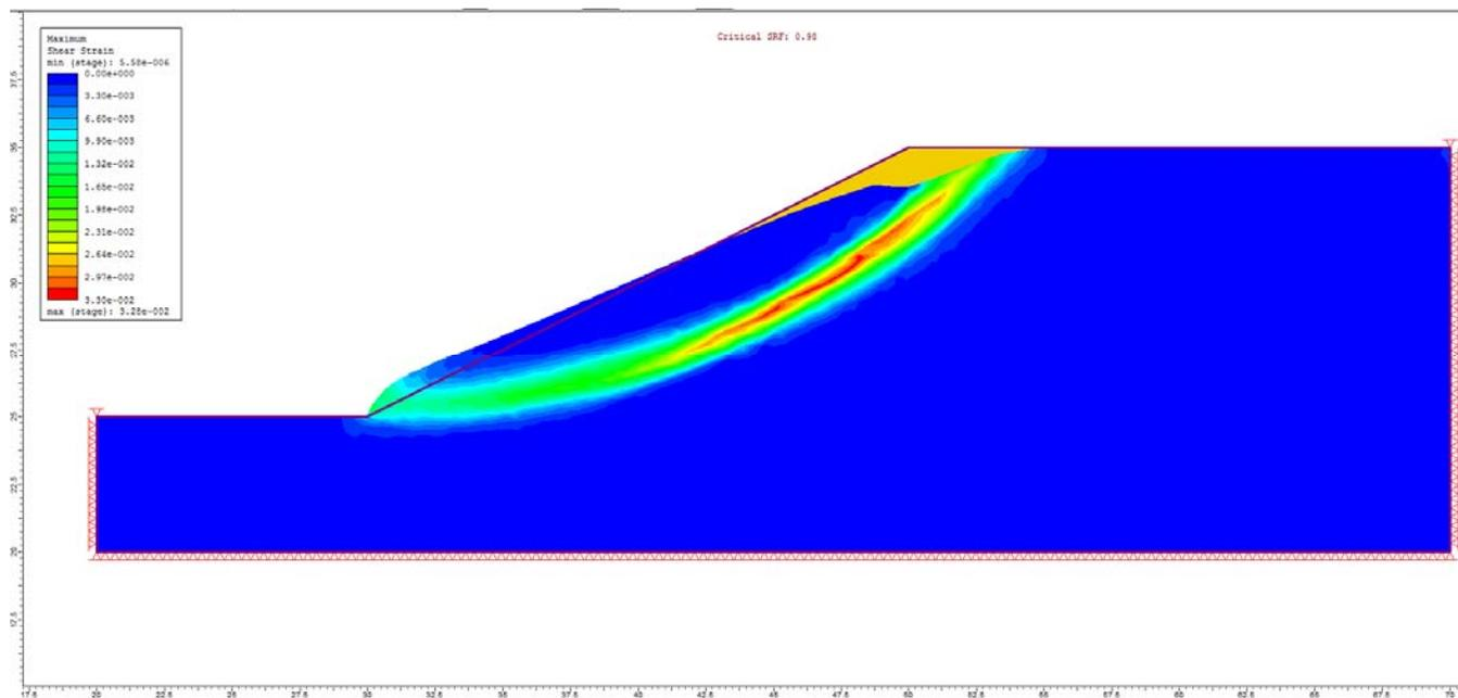
Figure 1.4.7 – RS2 Maximum Shear Strain with Deformation Contours
