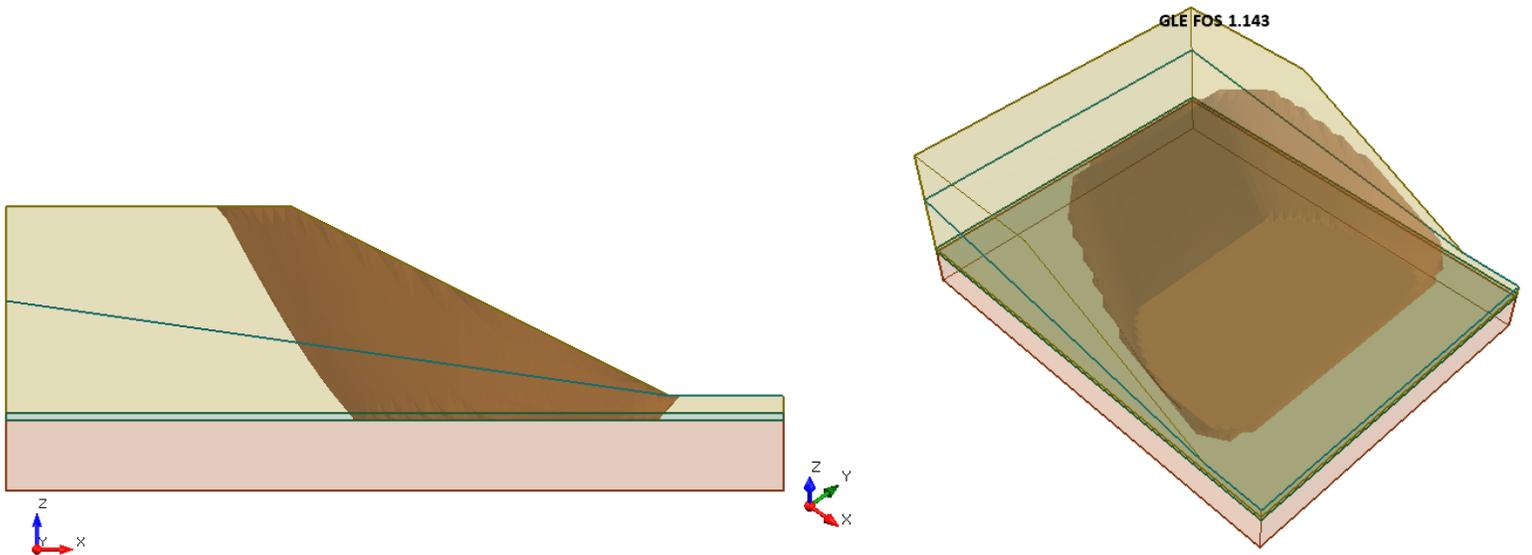
**Figure 16.4.3 – Slide3 Solution Using the GLE Method**
