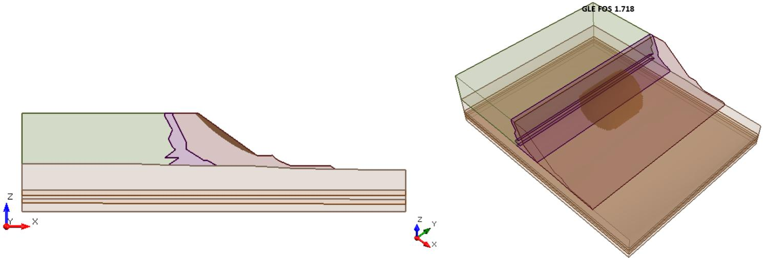
**Figure 46.4.3 – Slide3 Solution Using the GLE Method**
