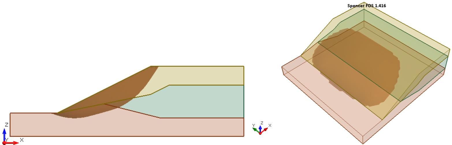
**Figure 4.4.3 – Slide3 Solution Using the Spencer Method**
