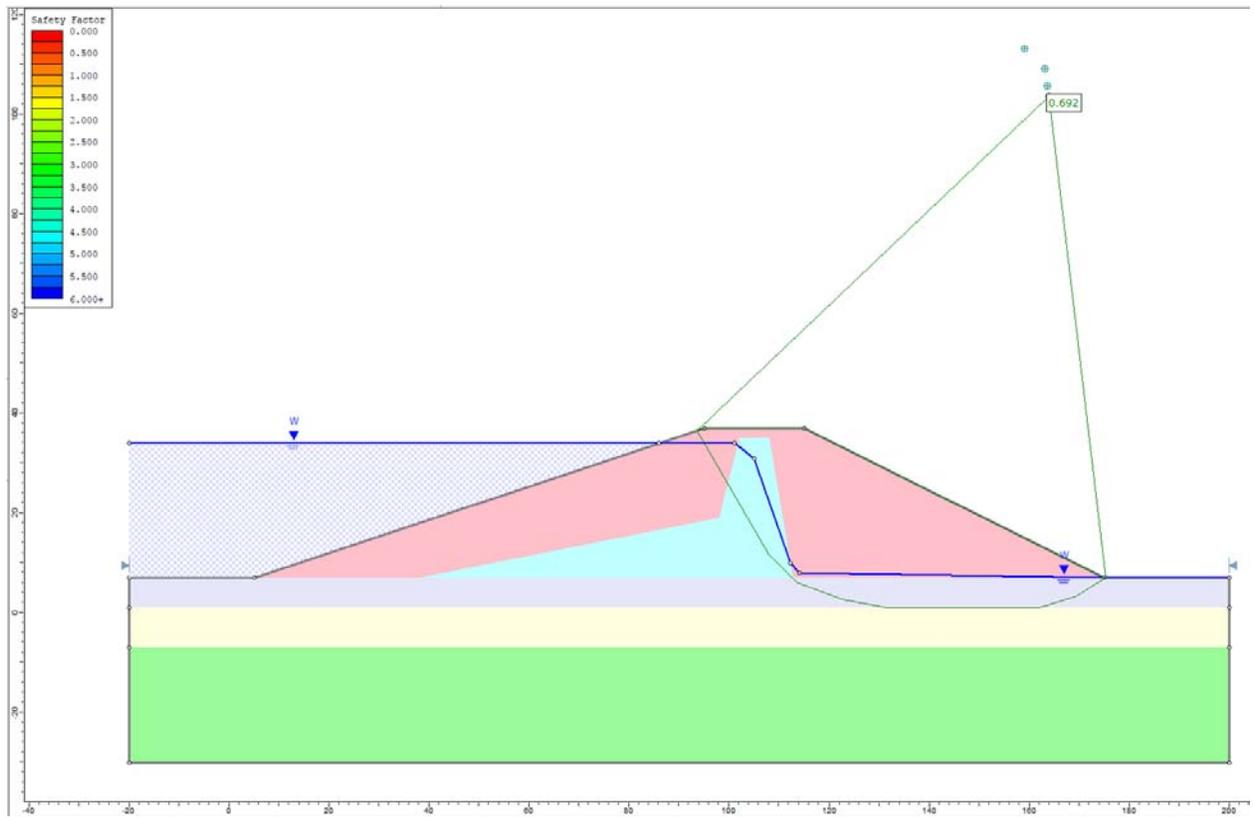
Figure 41.4.6 – Slide Solution using the Janbu Method
