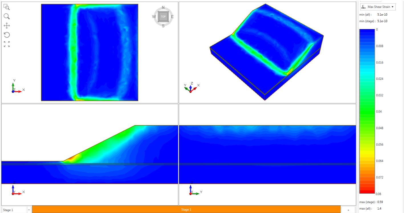
Figure 7.4.8 – RS3 Maximum Shear Strain
