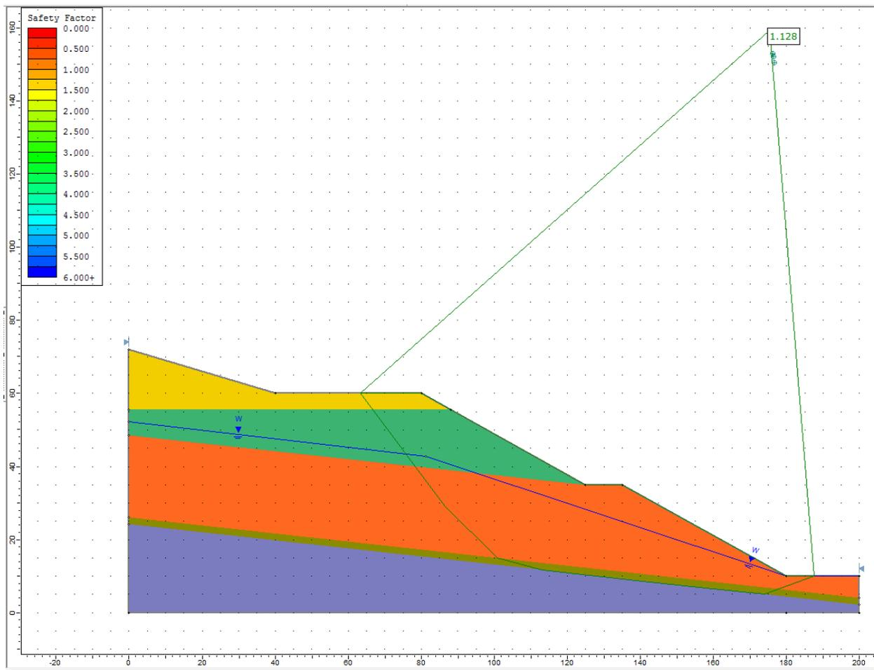
Figure 20.4.8 – Slide Solution Using the Spencer Method
