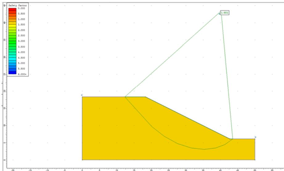
**Figure 14.4.2 – Slide Solution Using the Bishop Method**
