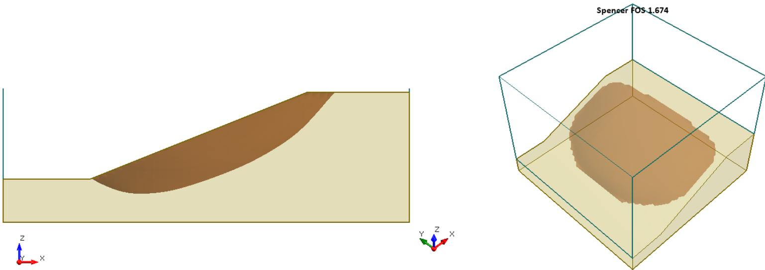
**Figure 28.4.5 – Slide3 Solution Using the Spencer Method**
