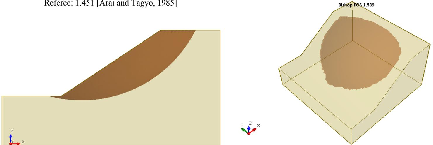
**Figure 8.4.1 – Slide3 Solution Using the Bishop Method**
