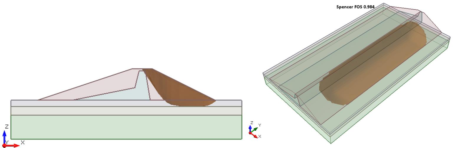
**Figure 40.4.7 – Slide3 Solution using the Spencer Method**
