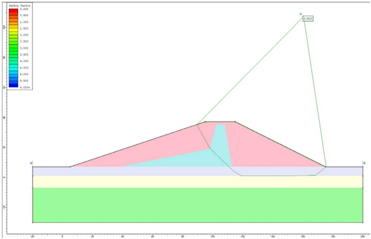
**Figure 40.4.6 – Slide Solution using the Janbu Method**
