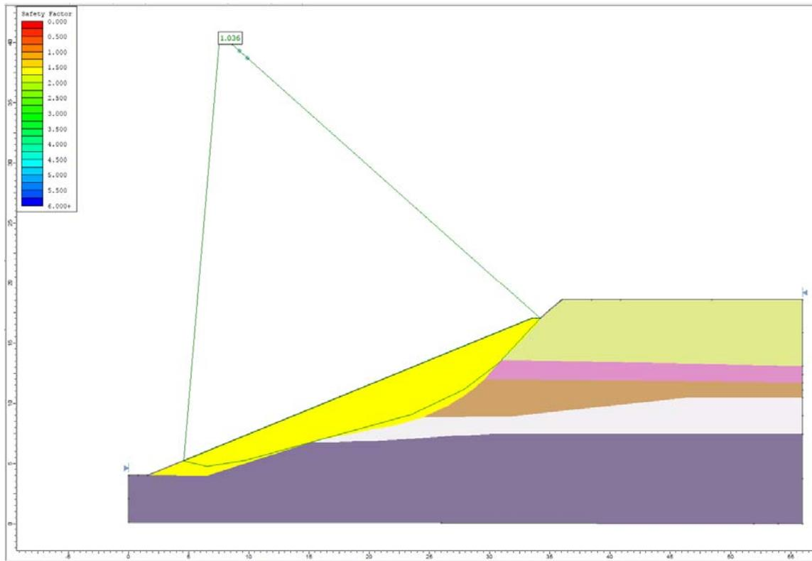
Figure 44.4.4 – Slide Solution Using the GLE Method
