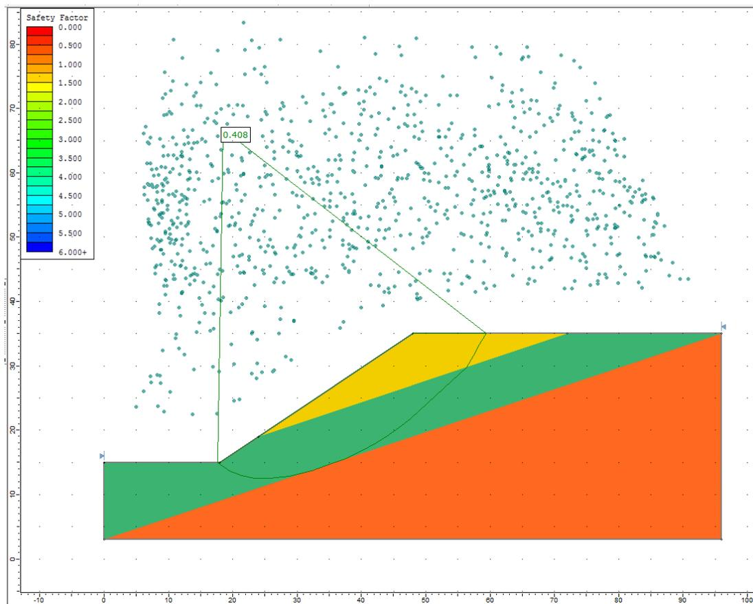
**Figure 11.4.6 – Slide Solution Using the GLE Method**
