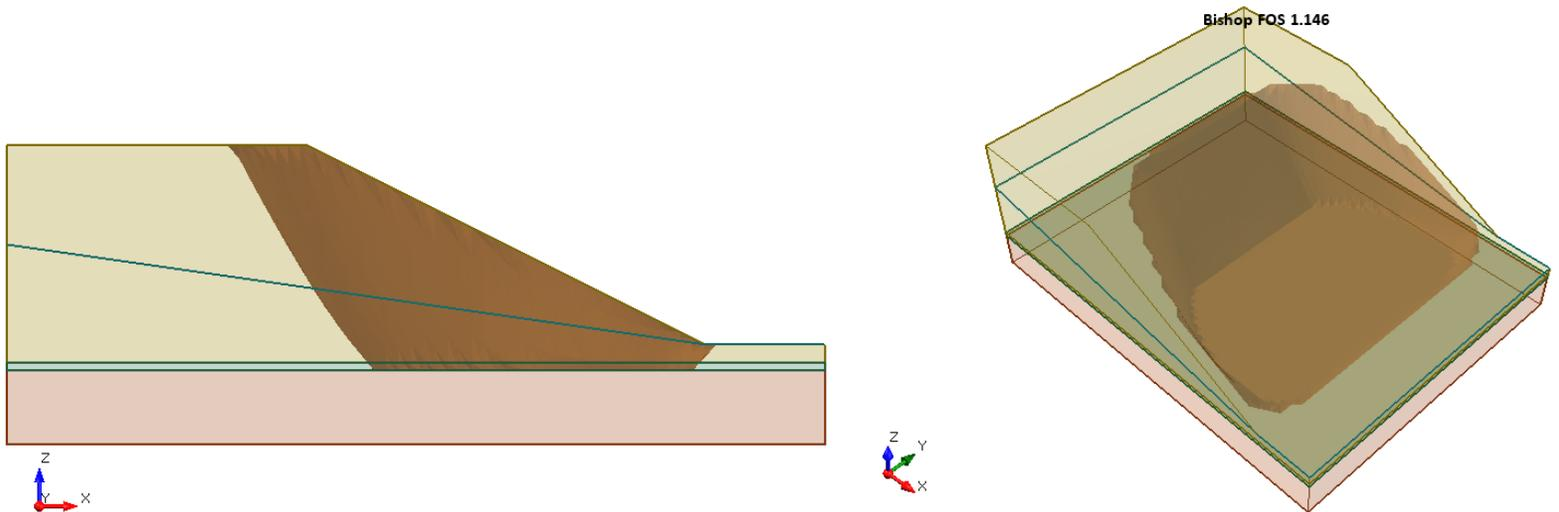
**Figure 16.4.1 – Slide3 Solution Using the Bishop Method**
