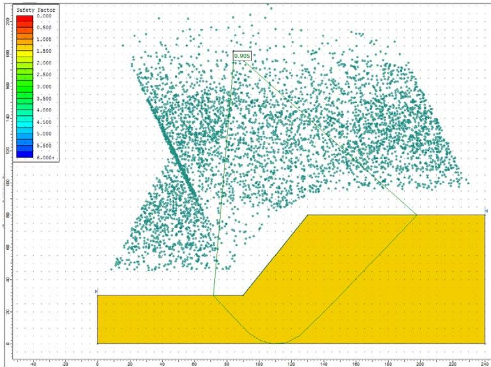
**Figure 35.4.2 – Slide Solution Using the Bishop Method**
