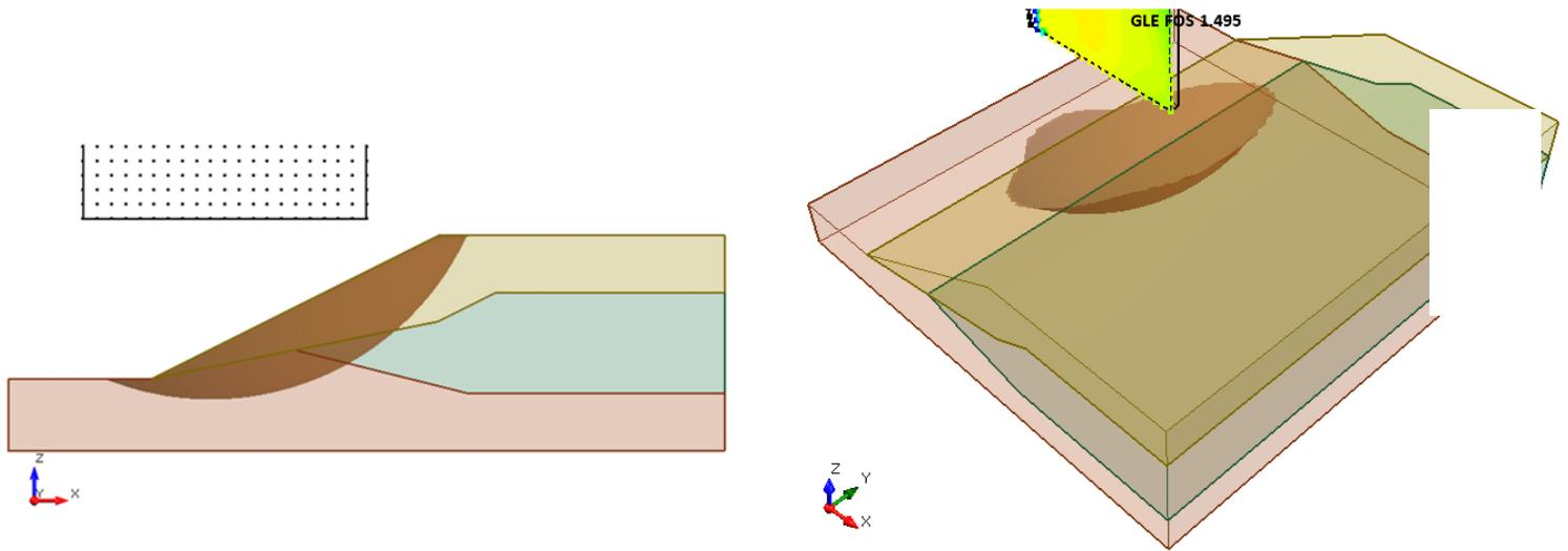
Figure 3.4.5 – Slide3 Solution Using the GLE Method
