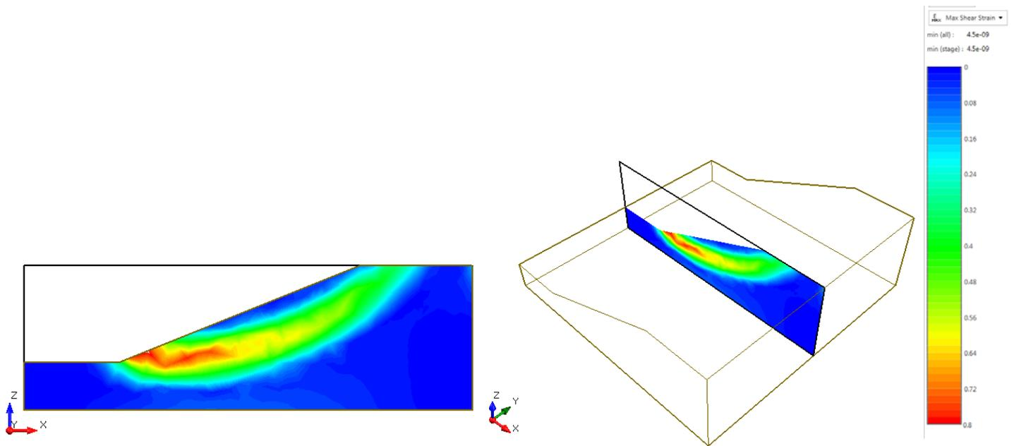
Figure 27.4.8 – RS3 Maximum Shear Strain
