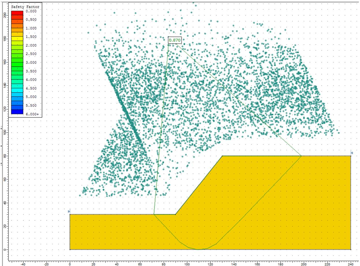
**Figure 35.4.4 – Slide Solution Using the GLE Method**
