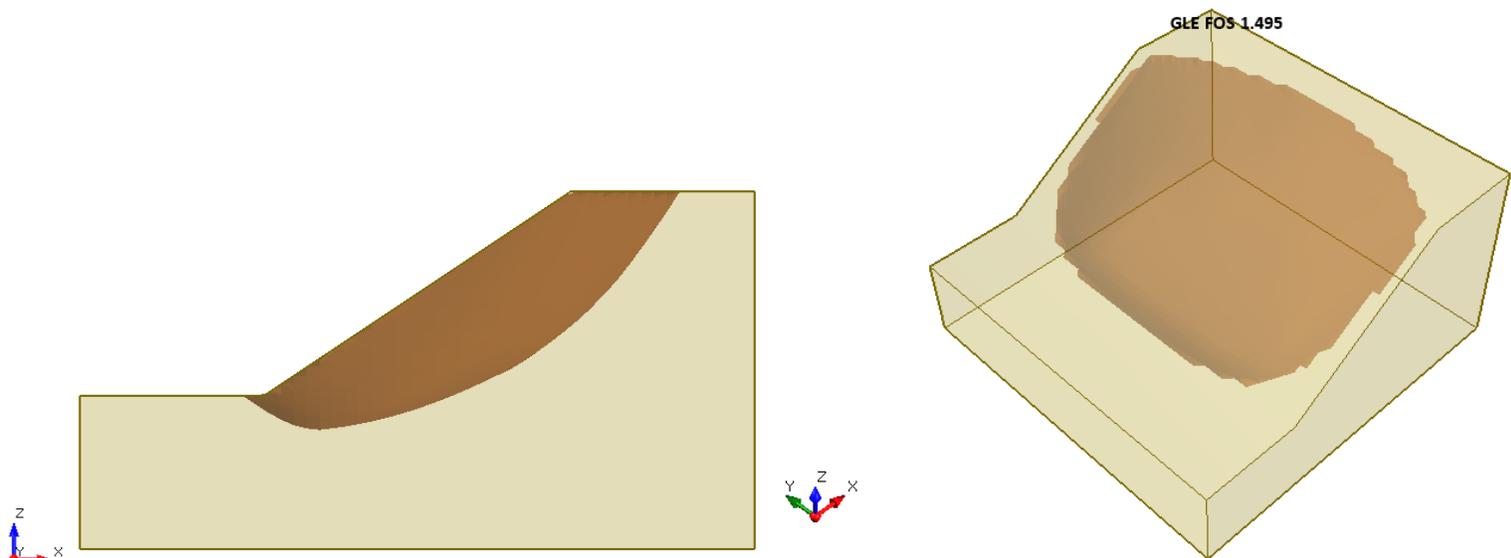
**Figure 9.4.5 – Slide3 Solution Using the GLE Method**
