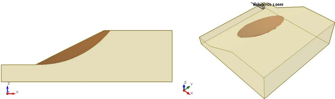
**Figure 1.4.1 – Slide3 Solution Using the Bishop Method**
