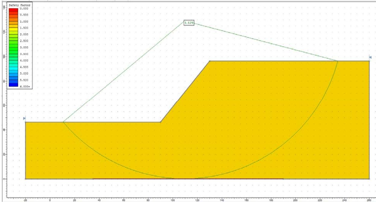
**Figure 36.4.4 – Slide Solution Using the GLE Method**
