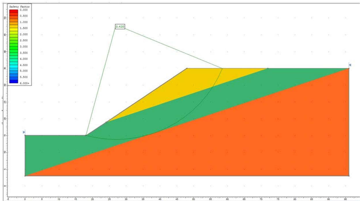
**Figure 10.4.6 – Slide Solution Using the GLE Method**
