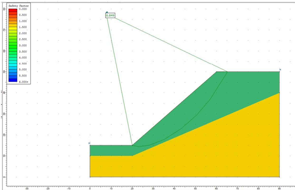
Figure 17.4.6 – Slide Solution Using the Janbu Method
