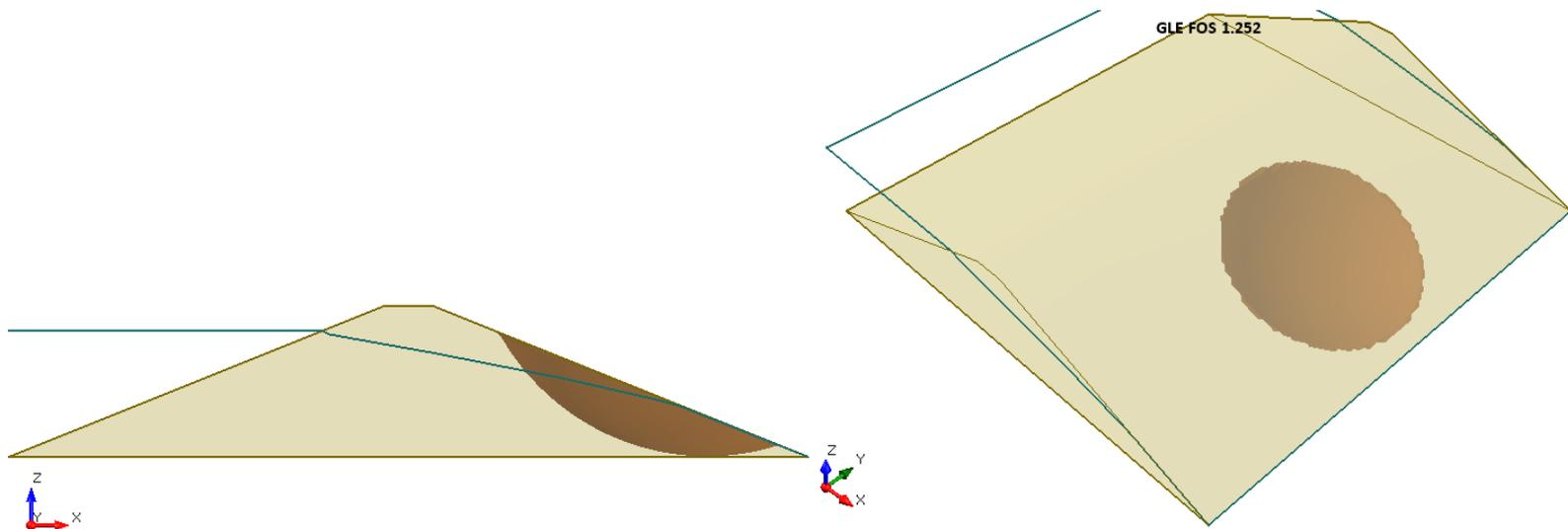
**Figure 30.4.3 – Slide3 Solution Using the GLE Method**
