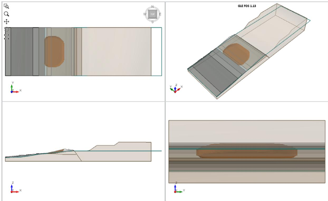
Figure 39.4.3 – Slide3 Solution Using the GLE Method
