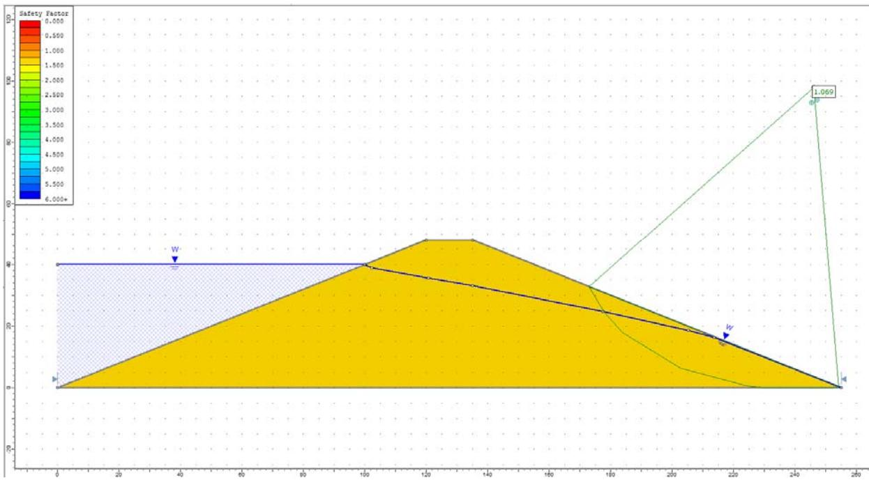
**Figure 31.4.4 – Slide Solution Using the GLE Method**
