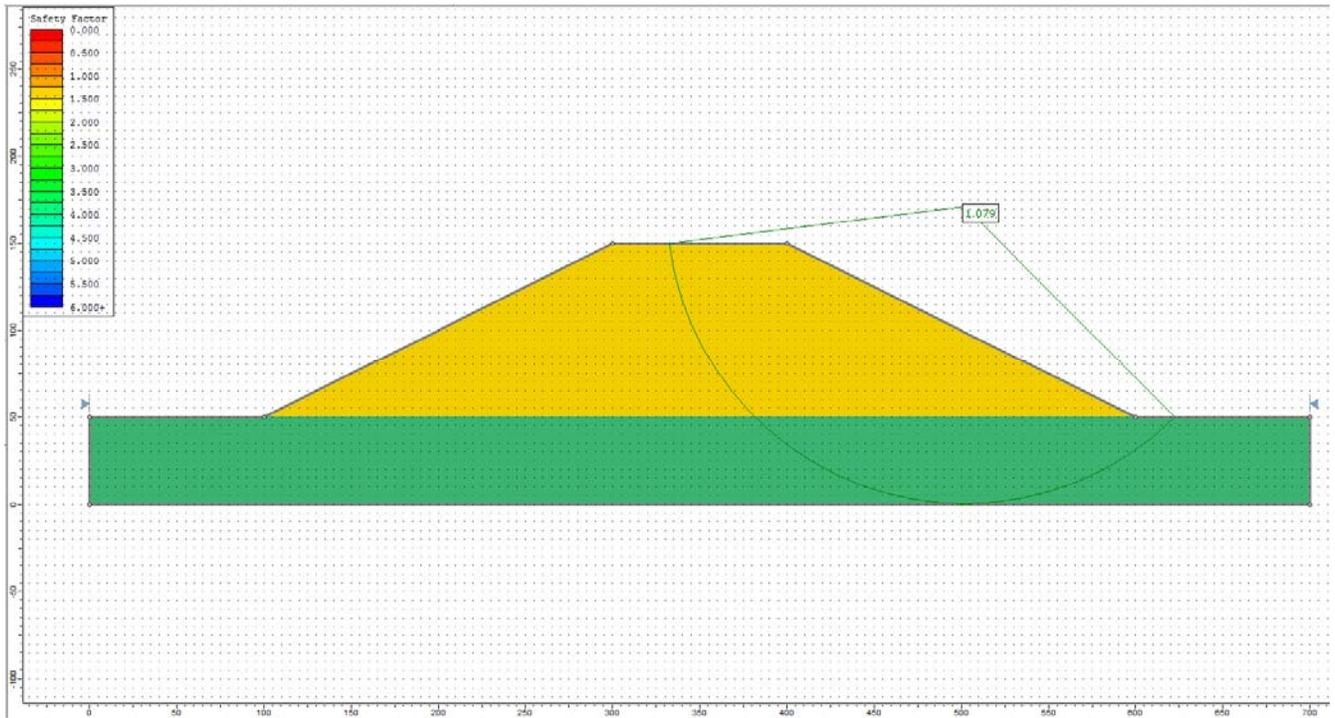
**Figure 29.4.4 – Slide Solution Using the Janbu Method**
