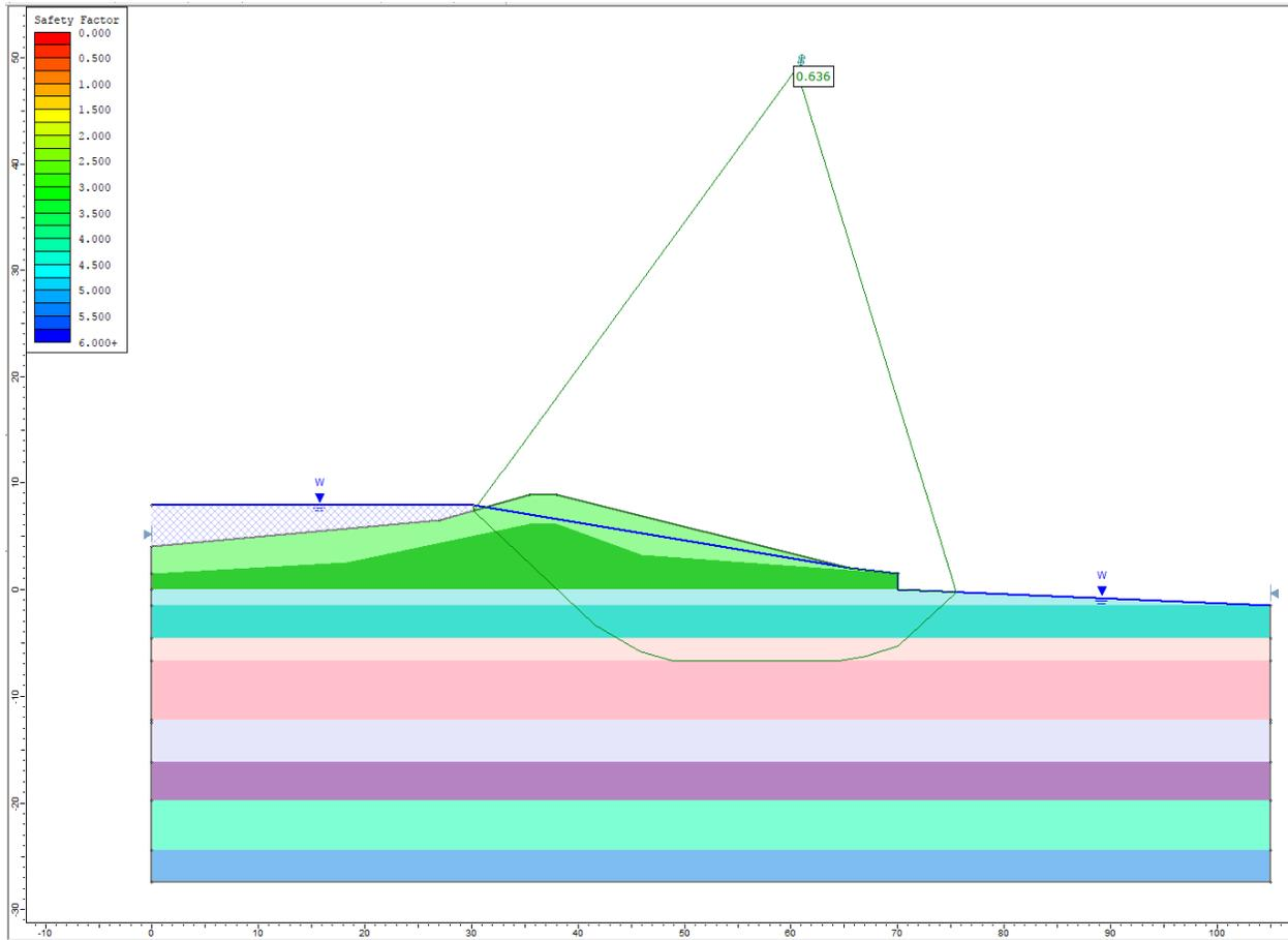
Figure 43.4.6 – Slide Solution Using the Janbu Method
