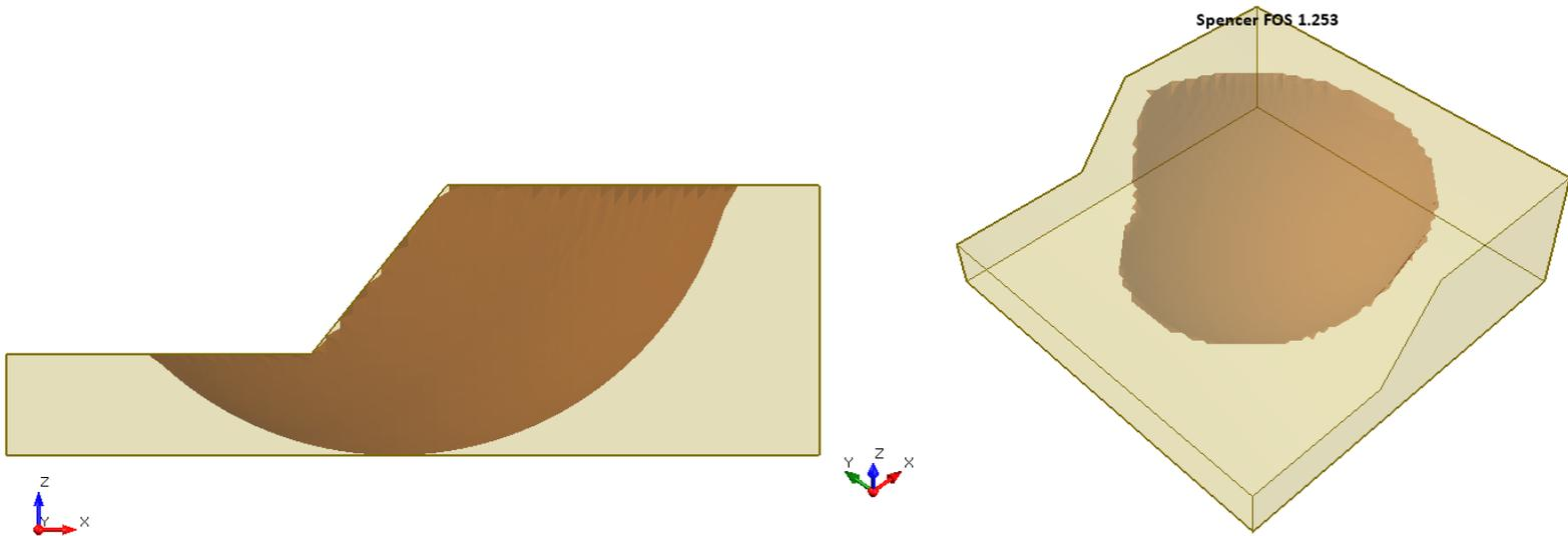
**Figure 34.4.5 – Slide3 Solution Using the Spencer Method**
