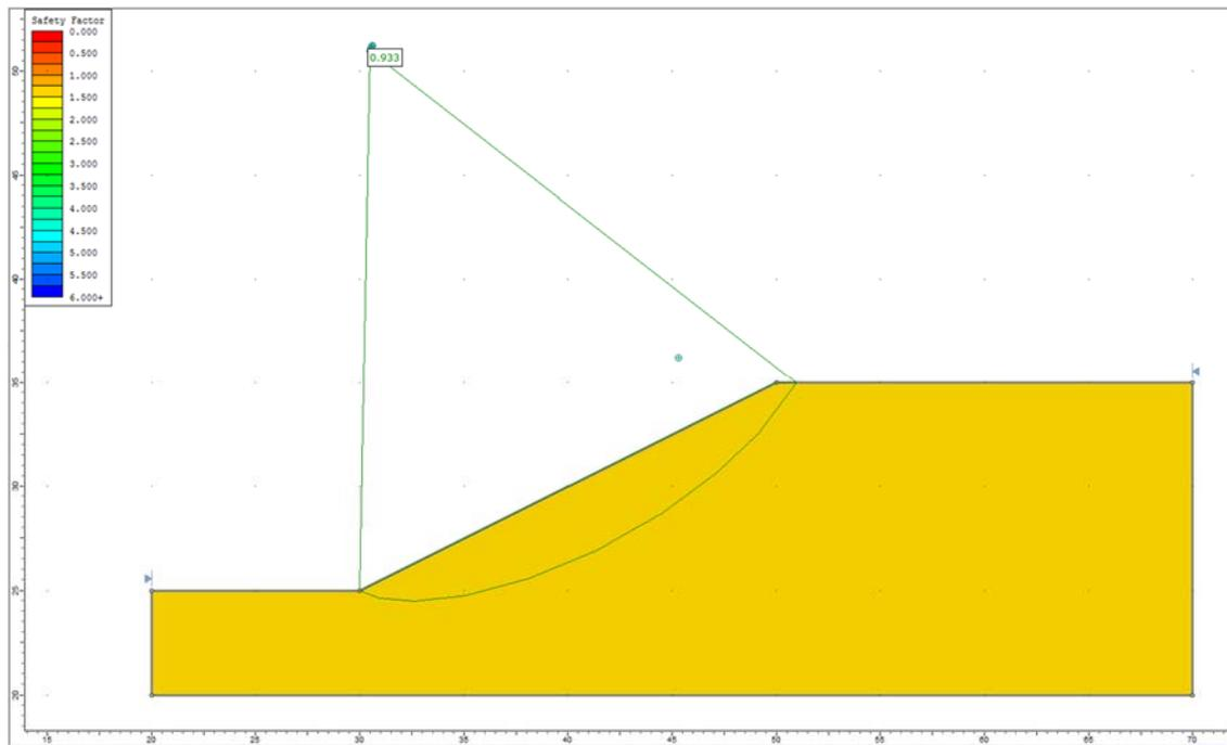
**Figure 2.4.2 – Slide Solution Using the Janbu Method**
