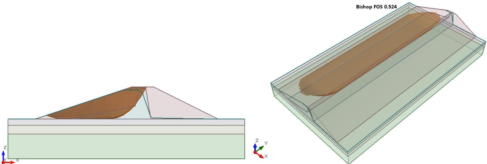
Figure 42.4.1 – Slide3 Solution Using the Bishop Method
