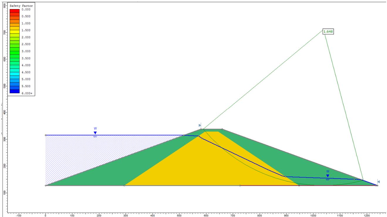
**Figure 32.4.6 – Slide Solution Using the Spencer Method**
