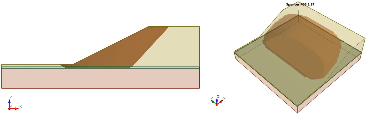
Figure 7.4.3 – Solution Using the Spencer Method
