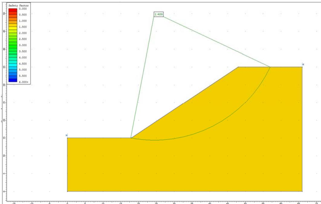
**Figure 8.4.2 – Slide Solution Using the Bishop Method**
