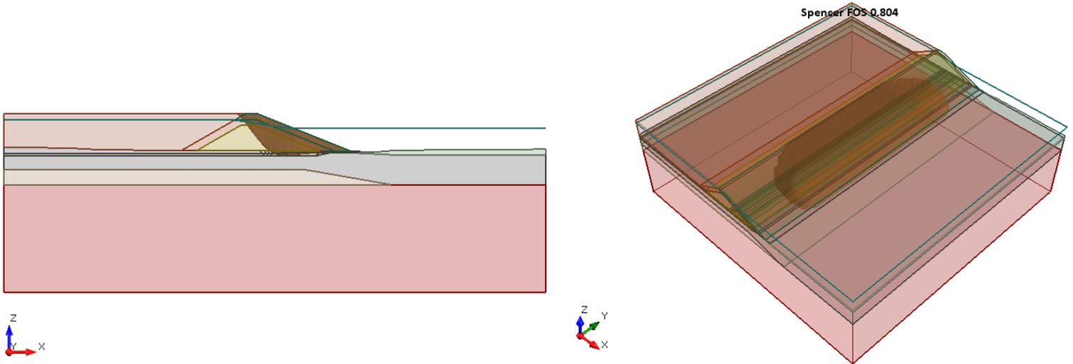
Figure 45.4.7 – Slide3 Solution Using the Spencer Method
