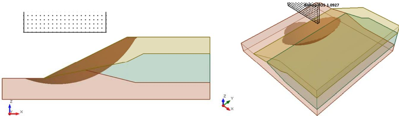
**Figure 5.4.1 – Slide3 Solution Using the Bishop Method**
