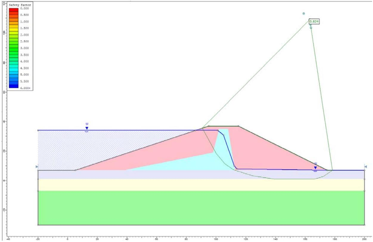
Figure 41.4.4 – Slide Solution Using the GLE Method
