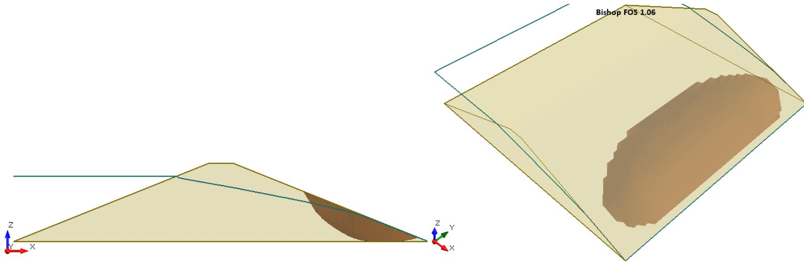
**Figure 31.4.1 – Slide3 Solution Using the Bishop Method**
