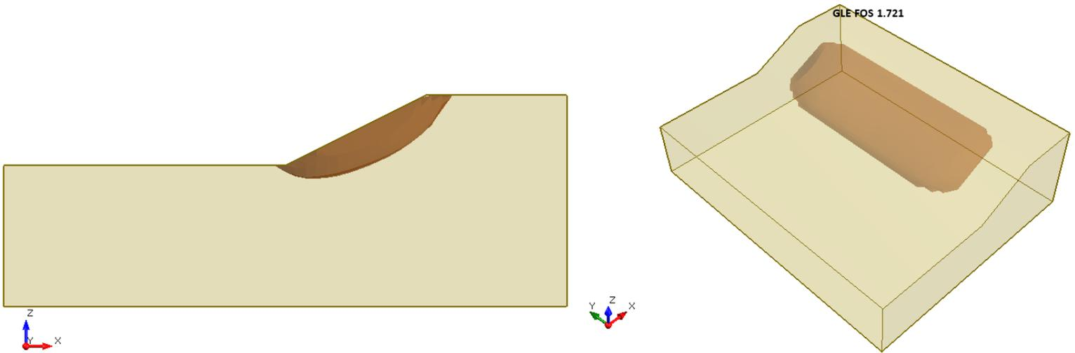
**Figure 19.4.3 – Slide3 Solution Using the GLE Method**
