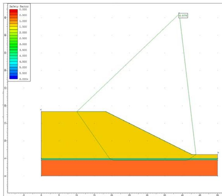
**Figure 15.4.2 – Slide Solution Using the Bishop Method**
