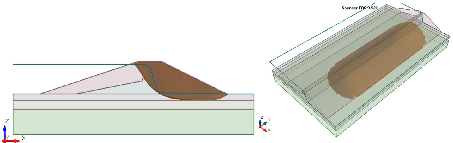
Figure 41.4.7 – Slide3 Solution using the Spencer Method
