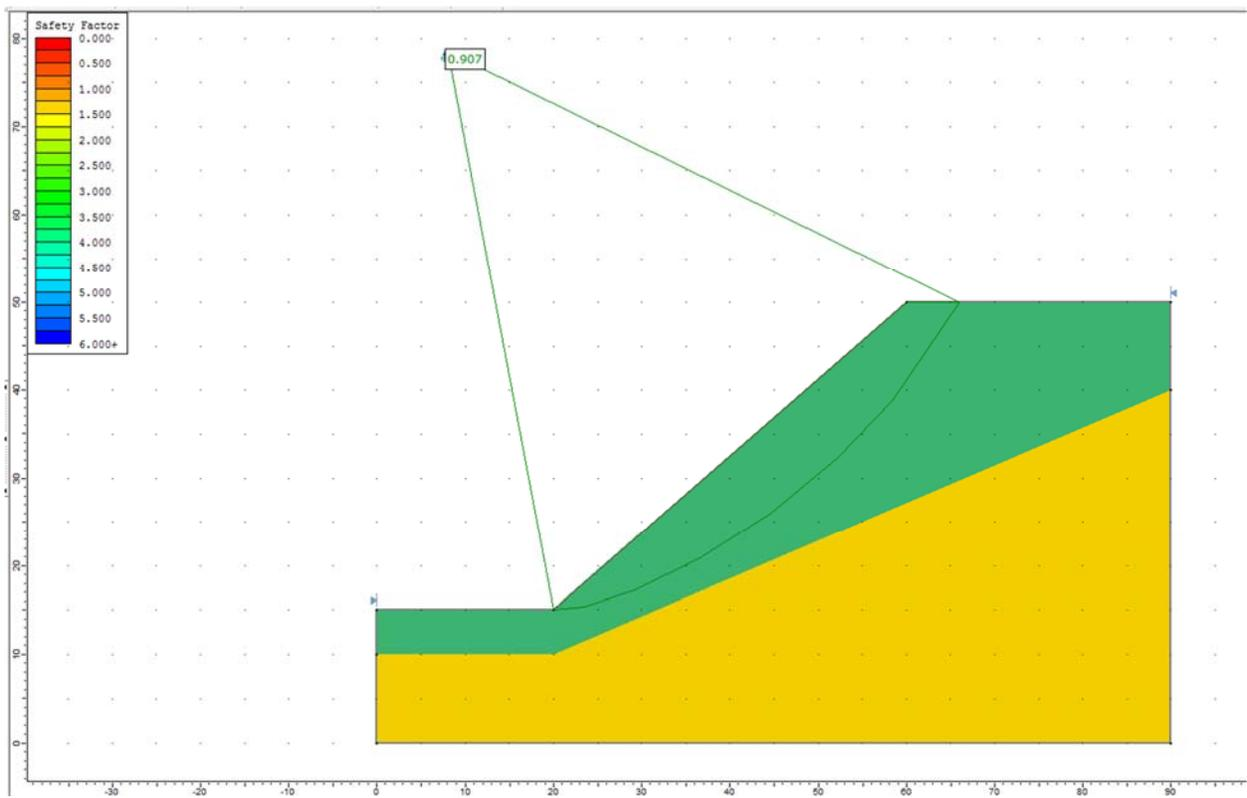
**Figure 17.4.8 – Slide Solution Using the Spencer Method**
