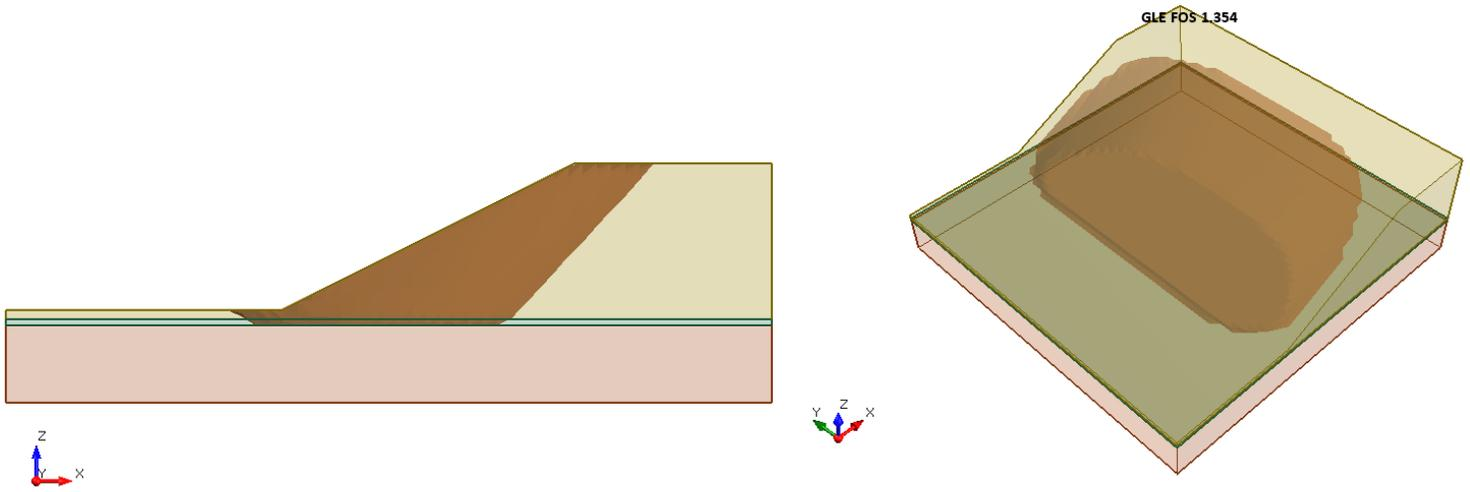
Figure 7.4.5 – Solution Using the GLE Method
