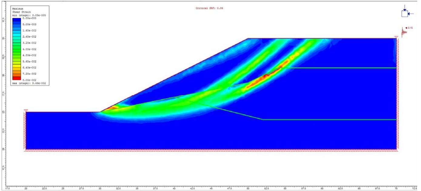
Figure 5.4.7 – RS2 Maximum Shear Strain
