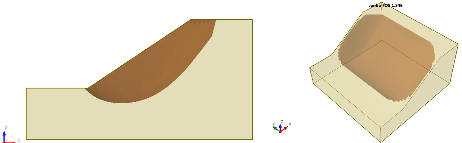
**Figure 9.4.1 – Slide3 Solution Using the Janbu Method**
