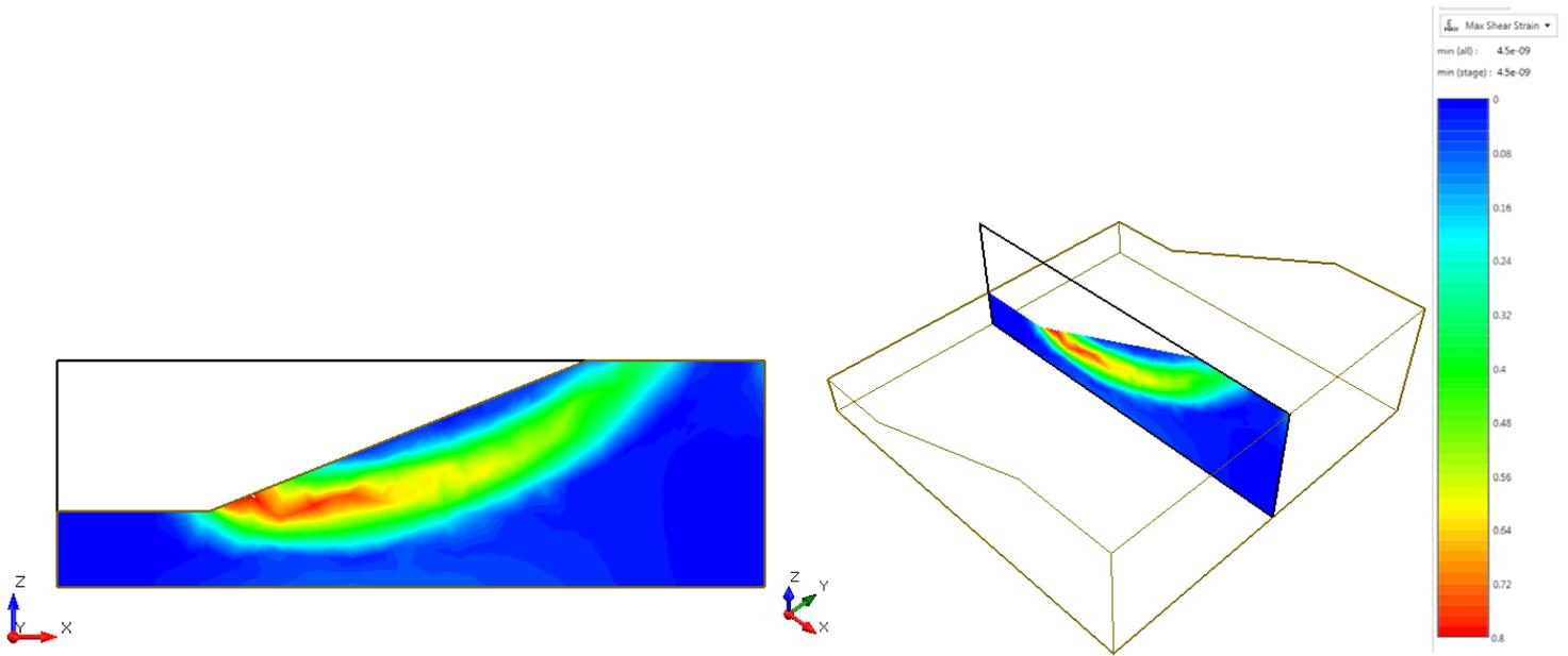
Figure 28.4.8 – RS3 Maximum Shear Strain
