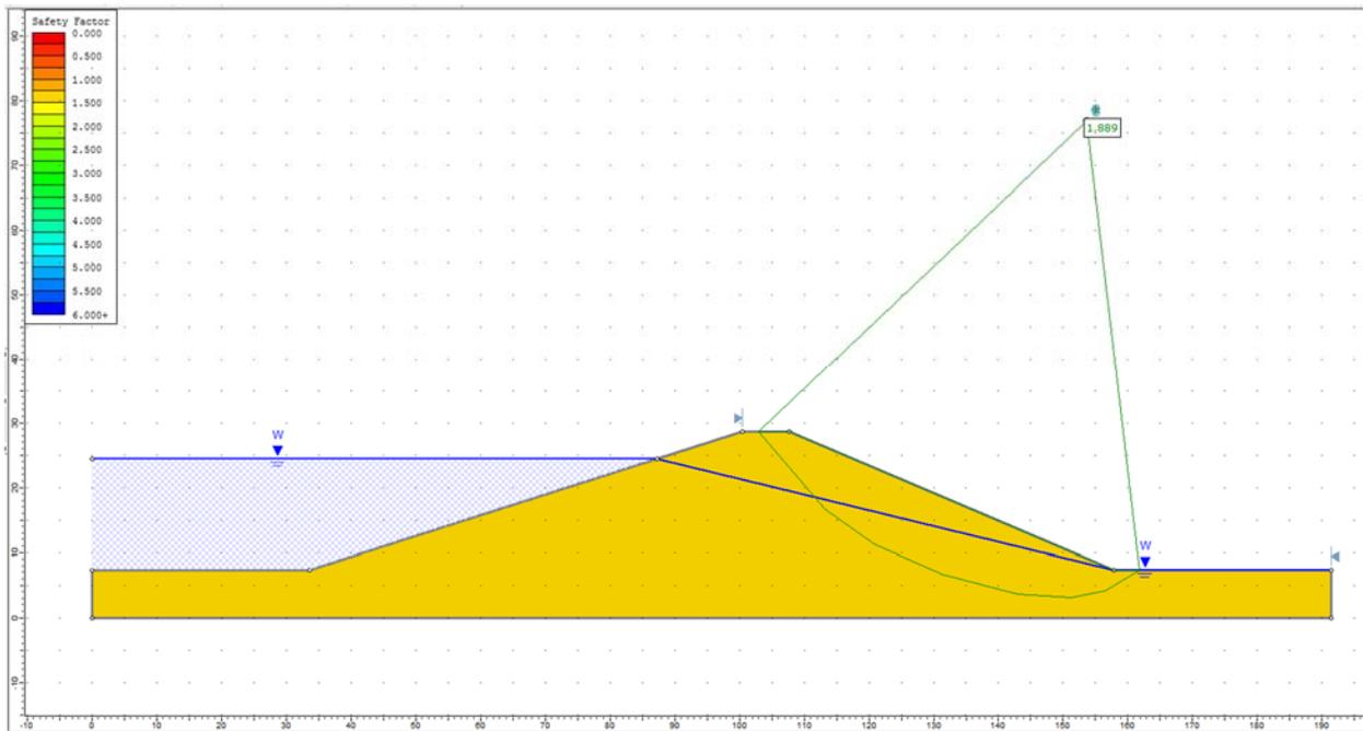
**Figure 13.4.4 – Slide Solution Using the GLE Method**
