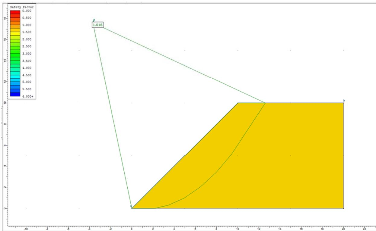
**Figure 18.4.6 – Slide Solution Using the Janbu Method**
