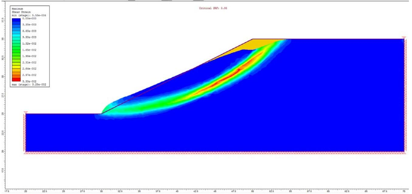
Figure 2.4.7 – RS2 Maximum Shear Strain with Deformation Contours
