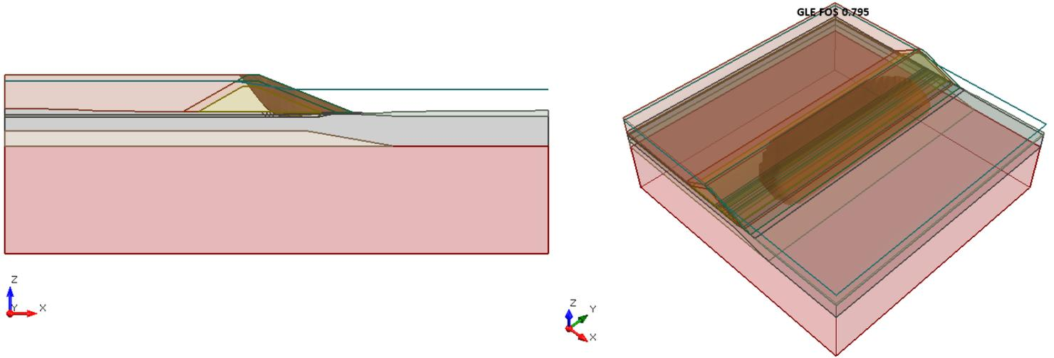
**Figure 45.4.3 – Slide3 Solution Using the GLE Method**
