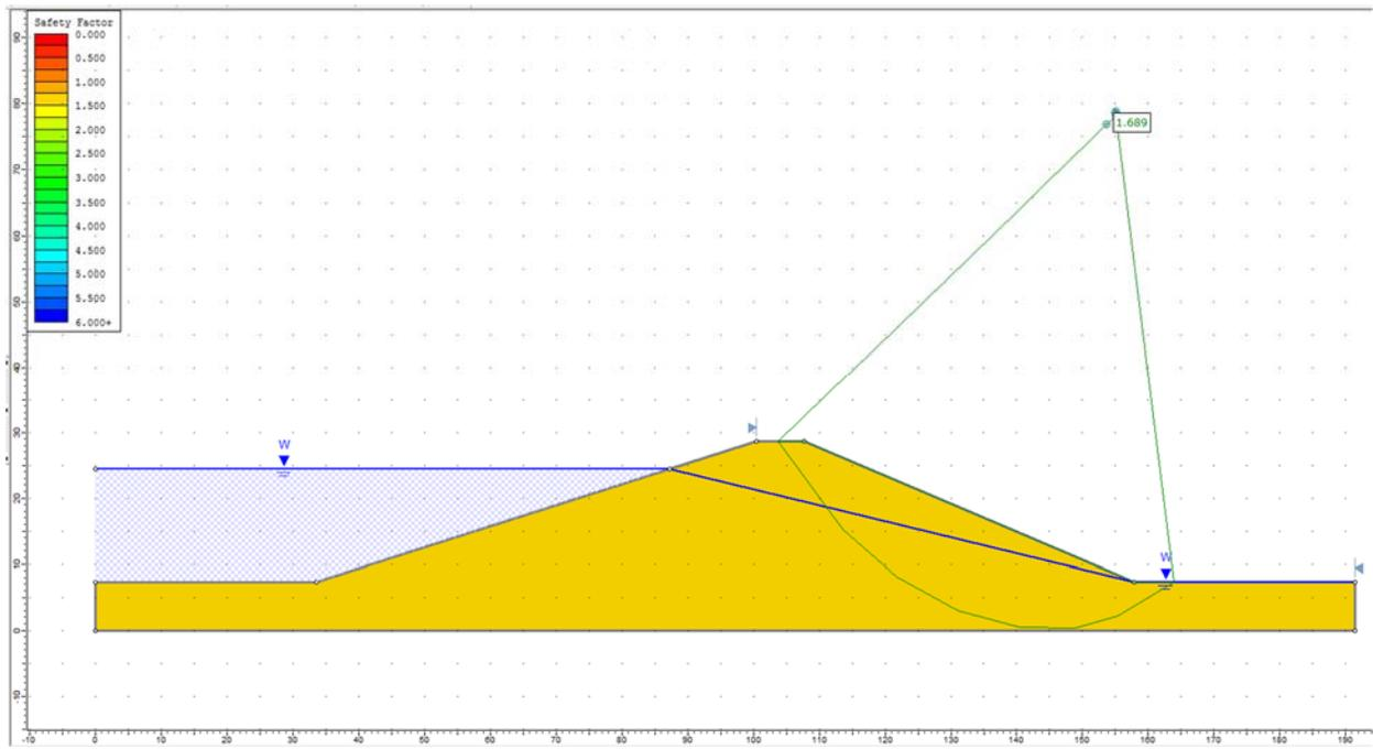
Figure 13.4.6 – Slide Solution Using the Janbu Method
