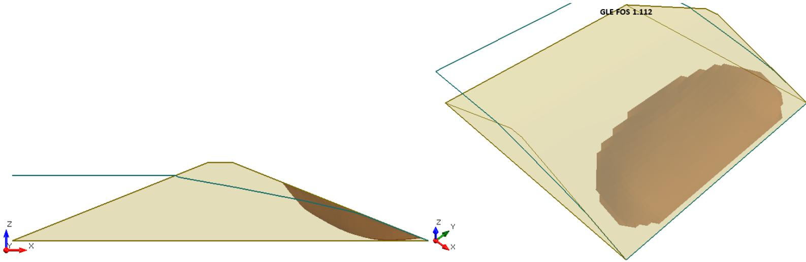
**Figure 31.4.3 – Slide3 Solution Using the GLE Method**
