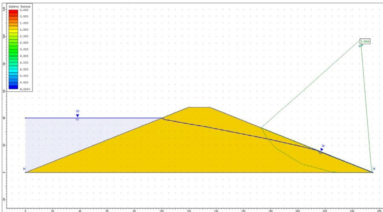
**Figure 31.4.6 – Slide Solution Using the Spencer Method**
