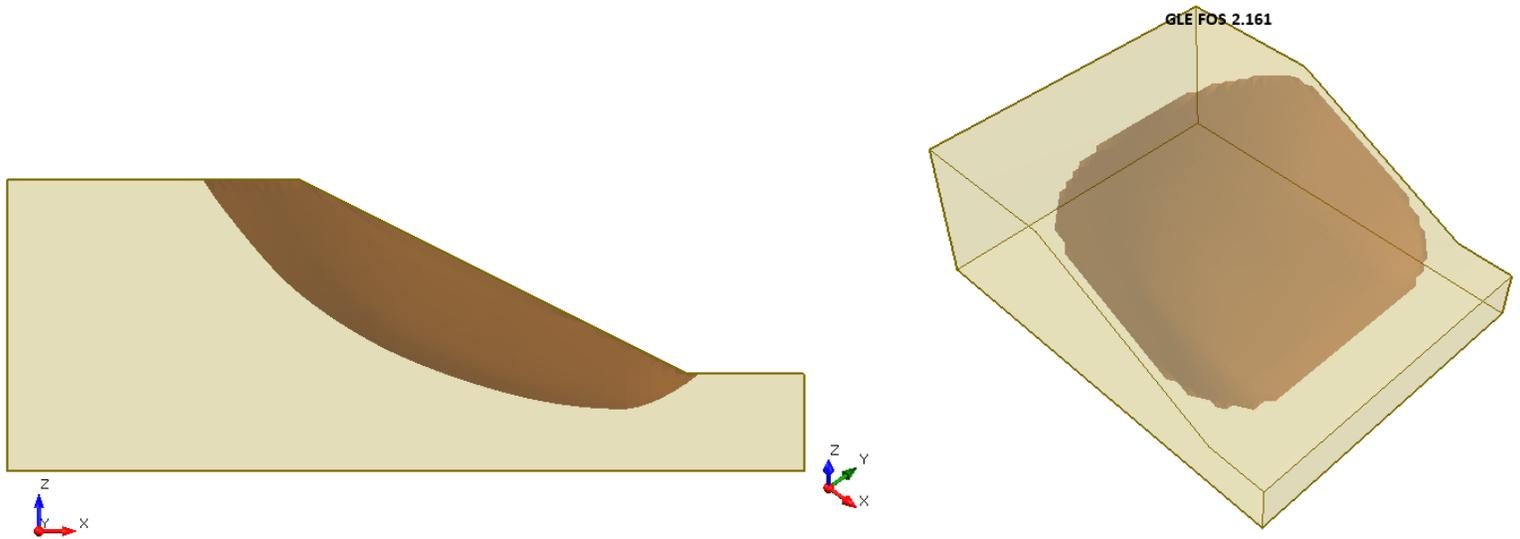
**Figure 14.4.3 – Slide3 Solution Using the GLE Method**
