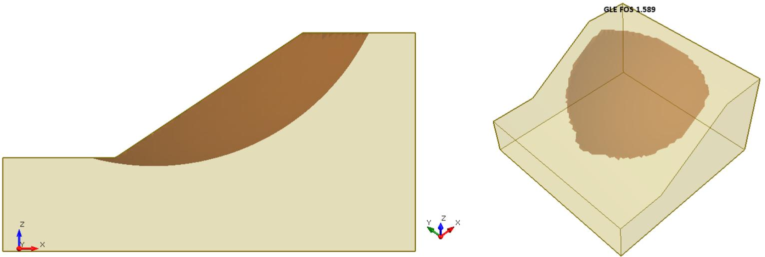
Figure 8.4.5 – Slide3 Solution Using the GLE Method
