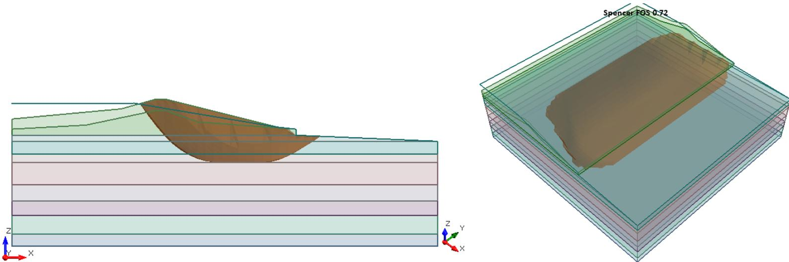
Figure 43.4.7 – Slide3 Solution Using the Spencer Method
