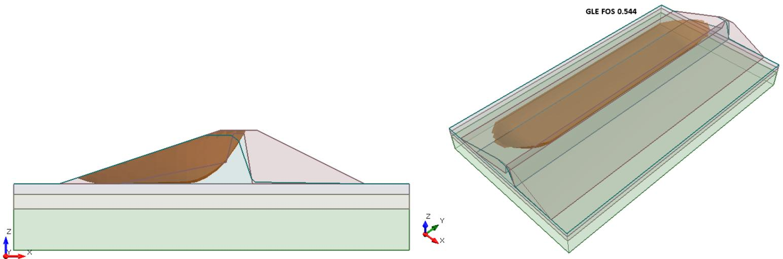
Figure 42.4.3 – Slide3 Solution using the GLE Method
