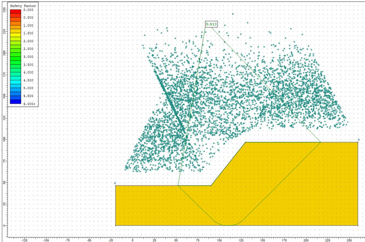
**Figure 37.4.6 – Slide Solution Using the Spencer Method**
