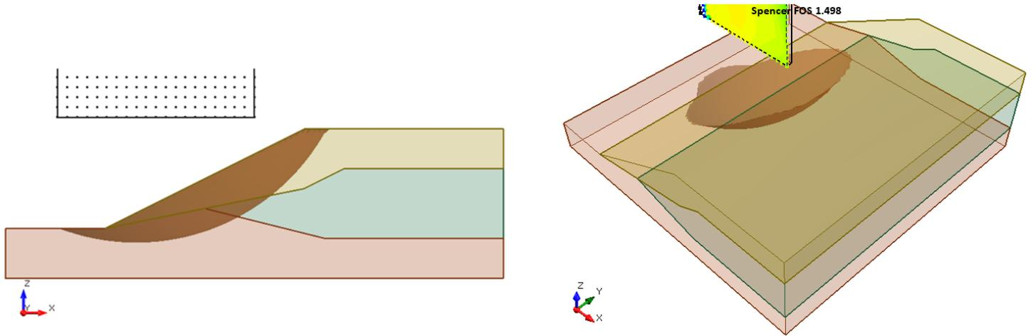
**Figure 3.4.3 – Slide3 Solution Using the Spencer Method**
