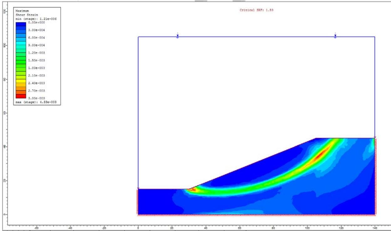
Figure 28.4.7 – RS2 Maximum Shear Strain
