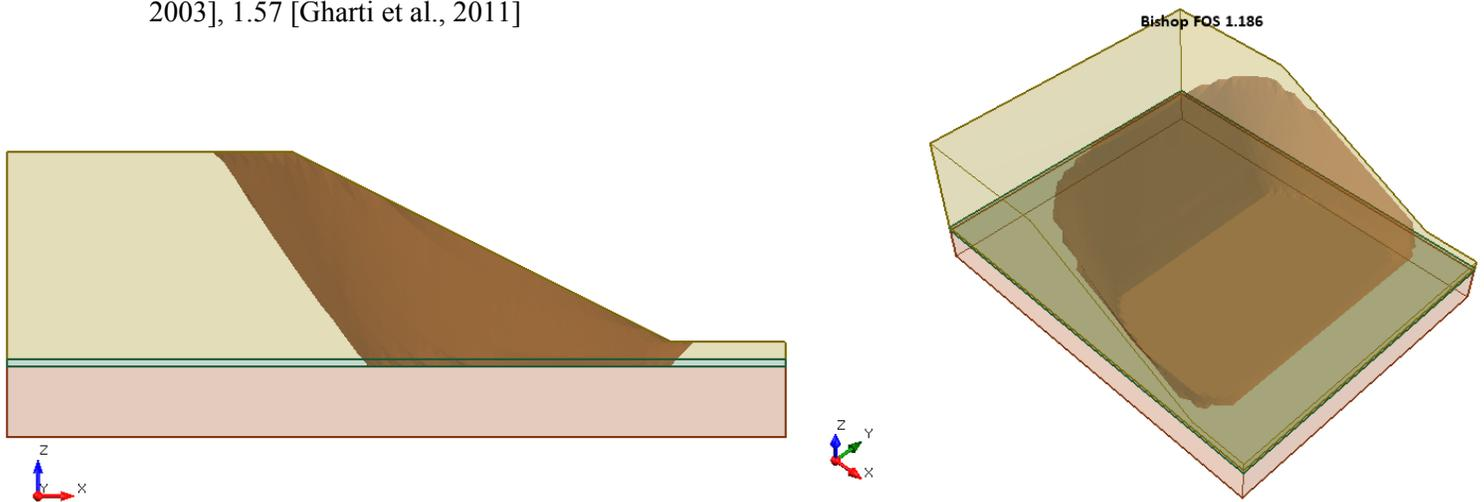
**Figure 15.4.1 – Slide3 Solution Using the Bishop Method**
