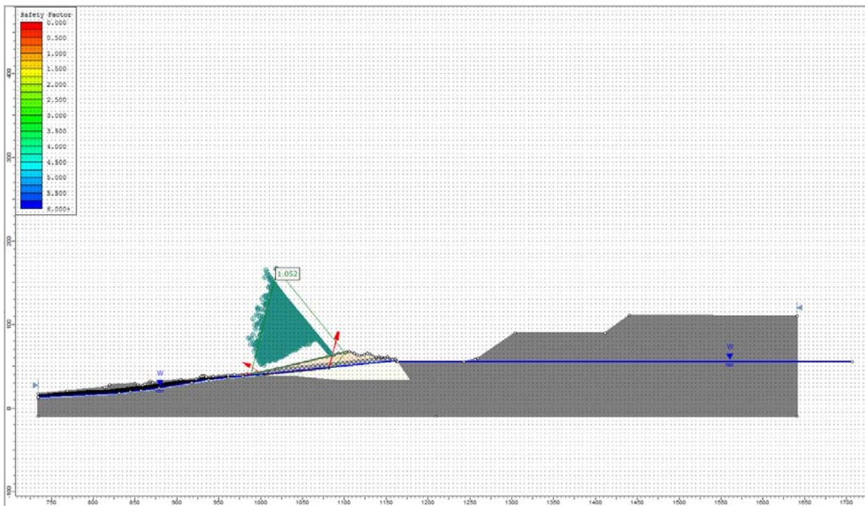
Figure 39.4.6 – Slide3 Solution Using the Janbu Method
