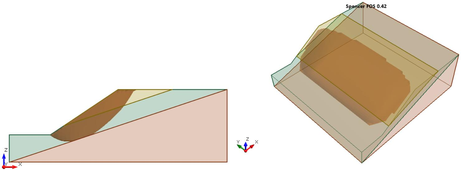
**Figure 11.4.3 – Slide3 Solution Using the Spencer Method**
