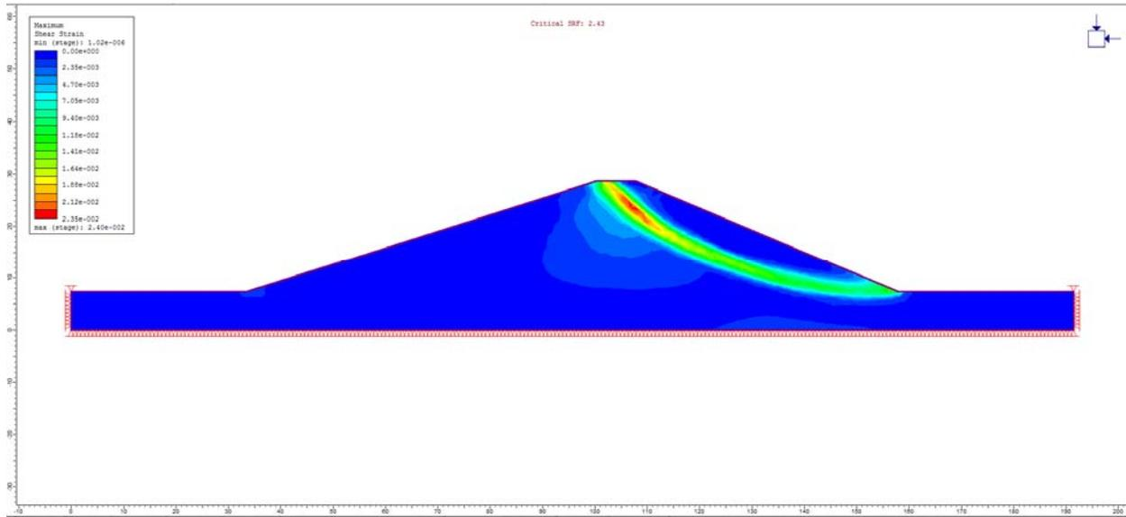
Figure 12.4.9 – RS2 Maximum Shear Strain
