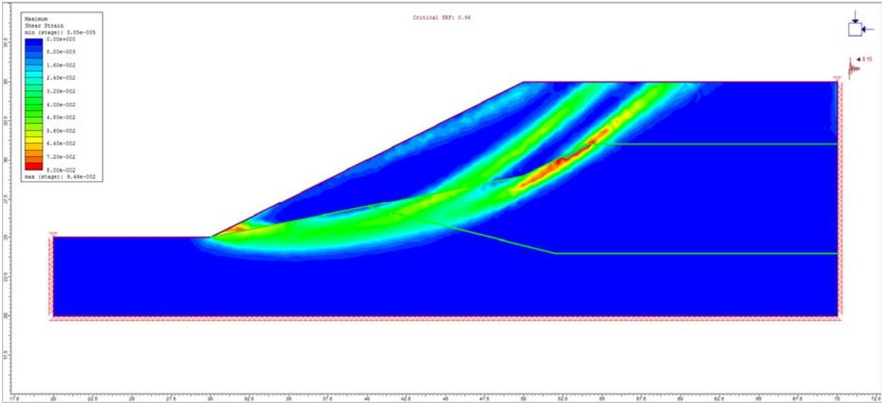
**Figure 6.4.7 – RS2 Maximum Shear Strain Contour with Displacement Contour**
