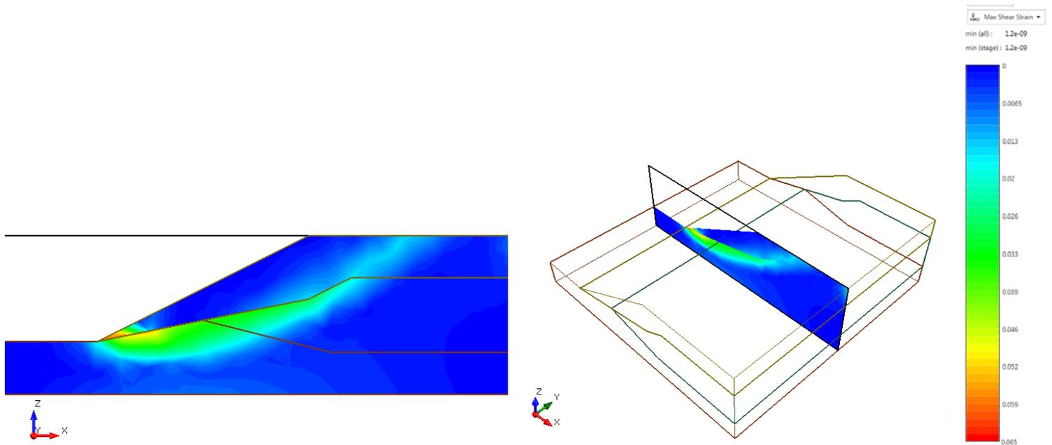
Figure 5.4.8 – RS3 Maximum Shear Strain Contour in the XZ Plane
