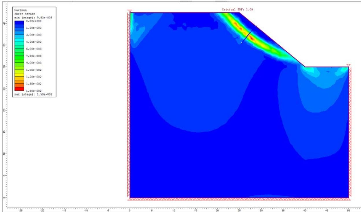
Figure 22.4.9 – RS2 Maximum Shear Strain
