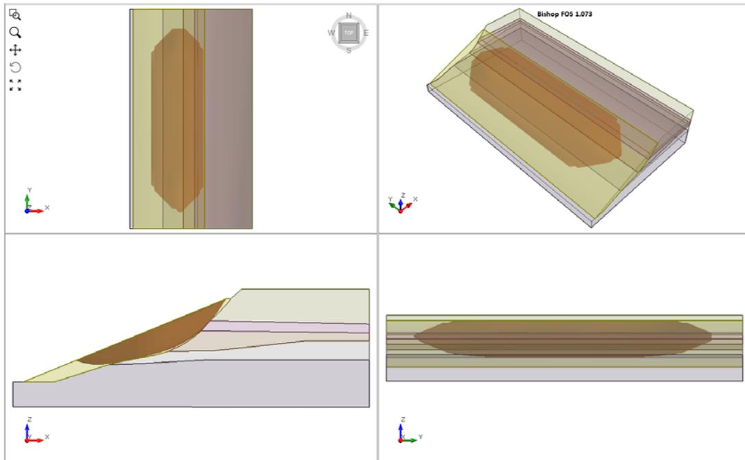
**Figure 44.4.1 – Slide3 Solution Using the Bishop Method**
