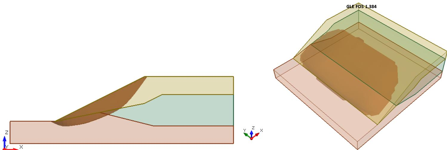
Figure 4.4.5 – Slide3 Solution Using the GLE Method
