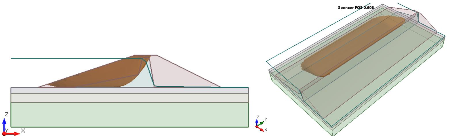
**Figure 42.5.4 – Slide3 Rapid Drawdown Using the Spencer Method**
