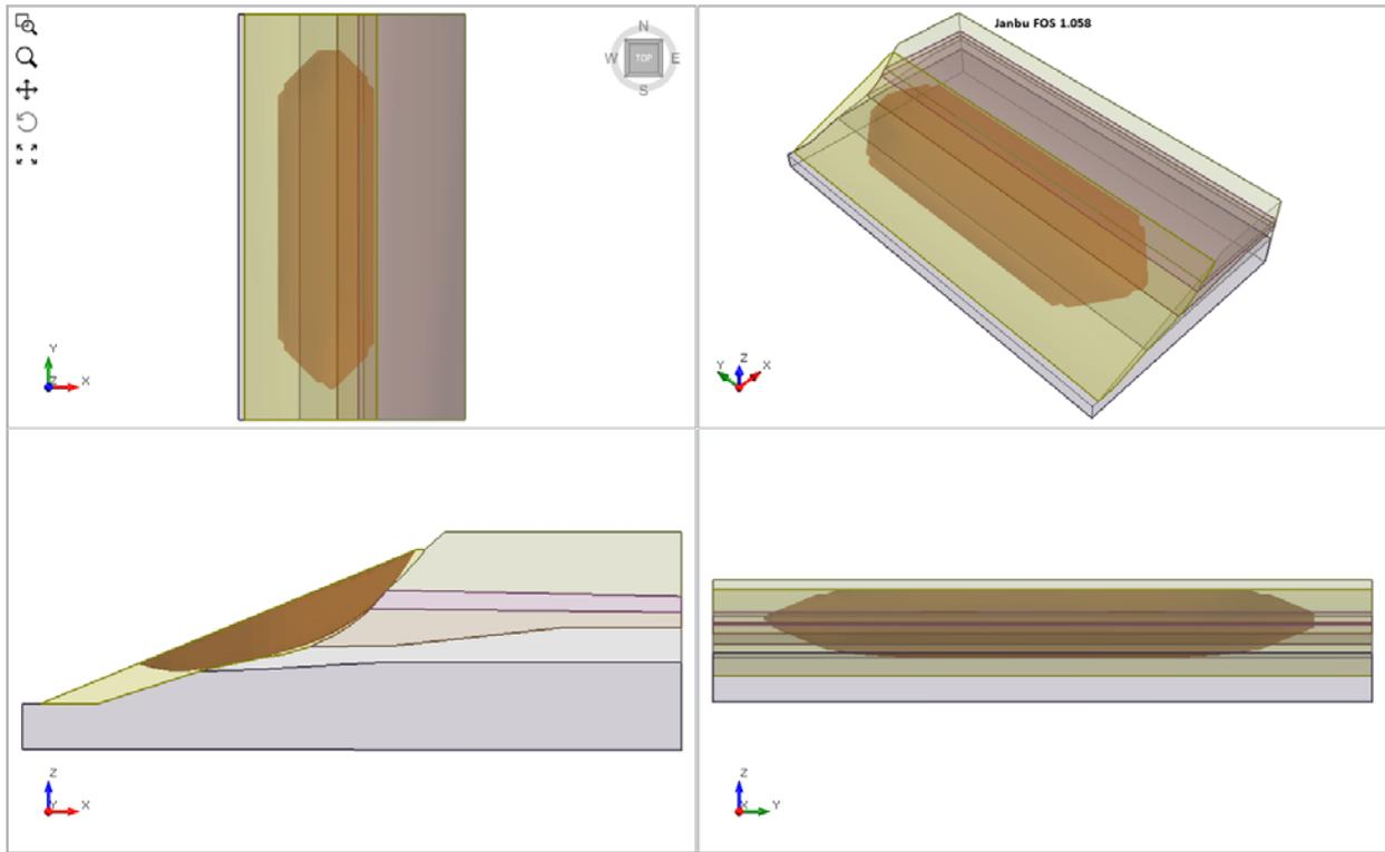
**Figure 44.4.5 – Slide3 Solution Using the Janbu Method**
