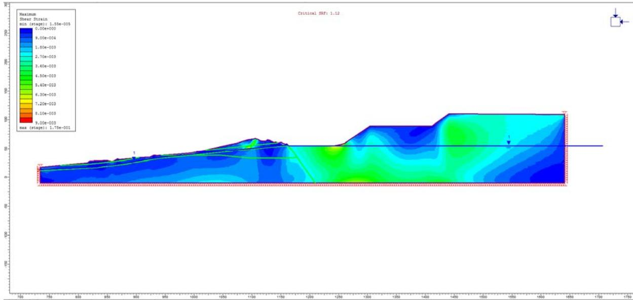
Figure 39.4.9 – RS2 Maximum Shear Strain
