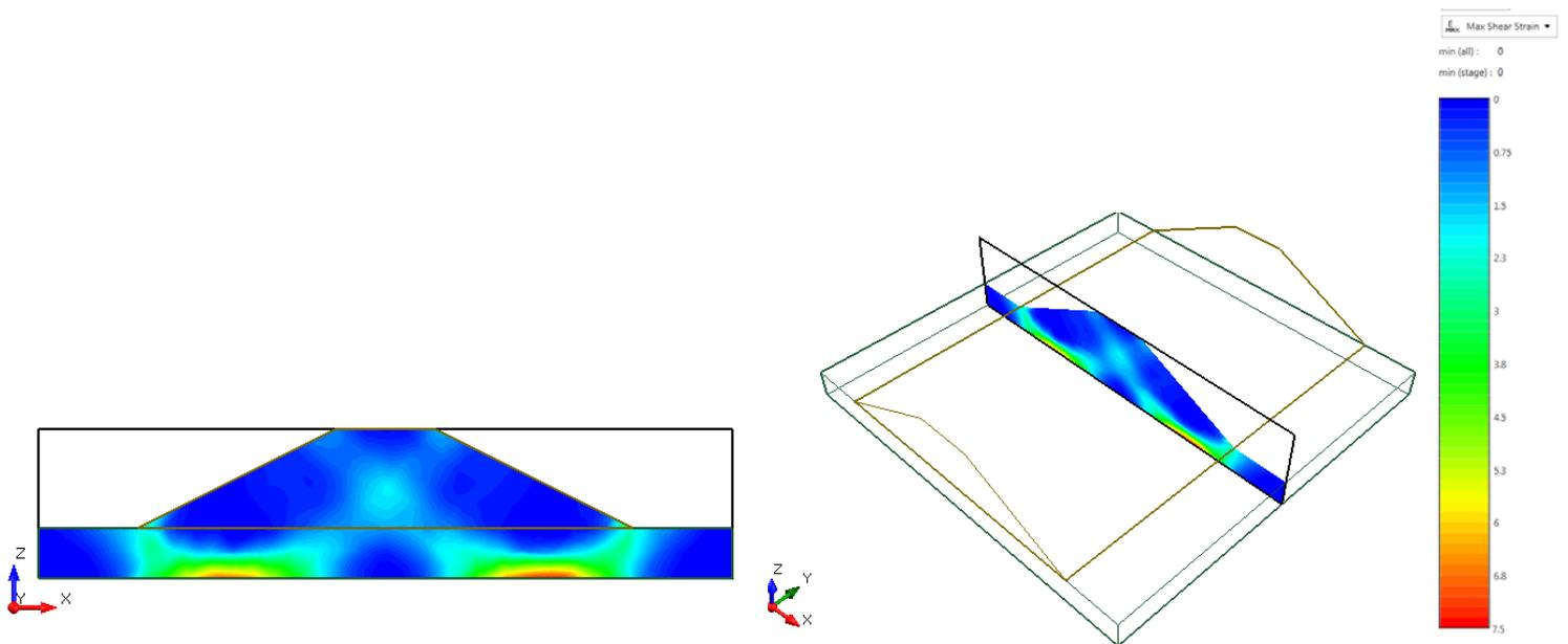
Figure 29.4.8 – RS3 Maximum Shear Strain
