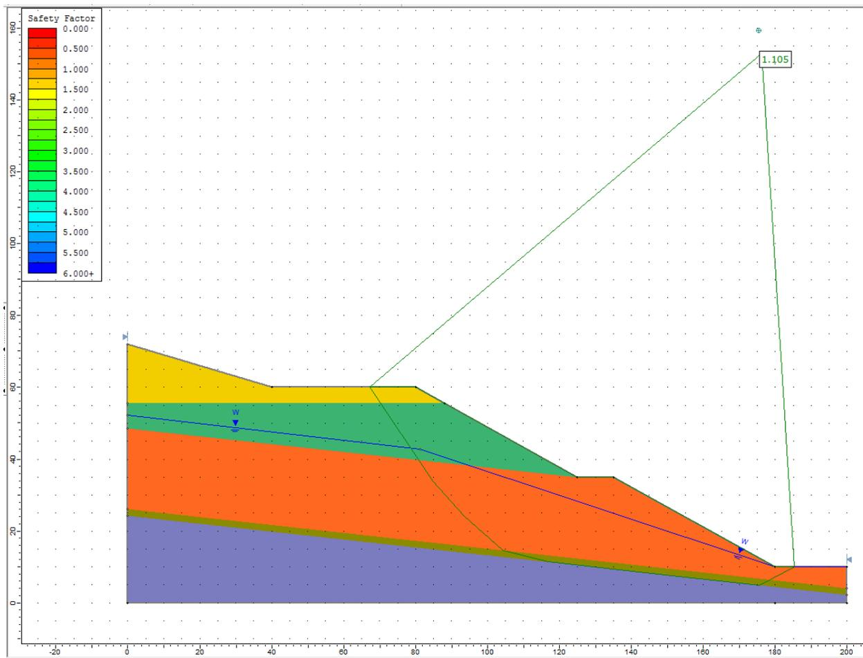
Figure 20.4.4 – Slide Solution Using the GLE Method
