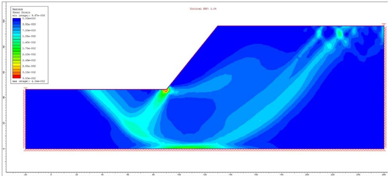
Figure 37.4.7 – RS2 Maximum Shear Strain
