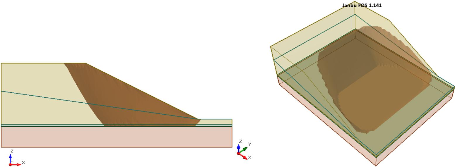
Figure 16.4.5 – Slide3 Solution Using the Janbu Method
