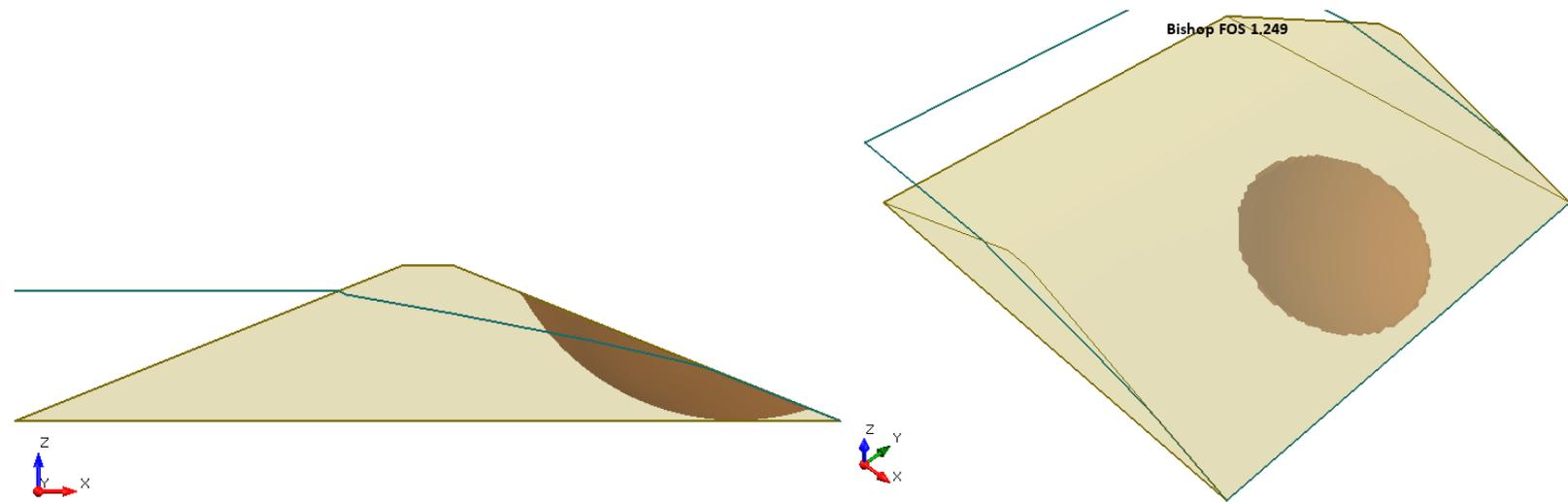
**Figure 30.4.1 – Slide3 Solution Using the Bishop Method**
