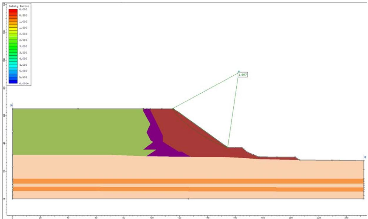
**Figure 46.4.8 – Slide Solution Using the Spencer Method**
