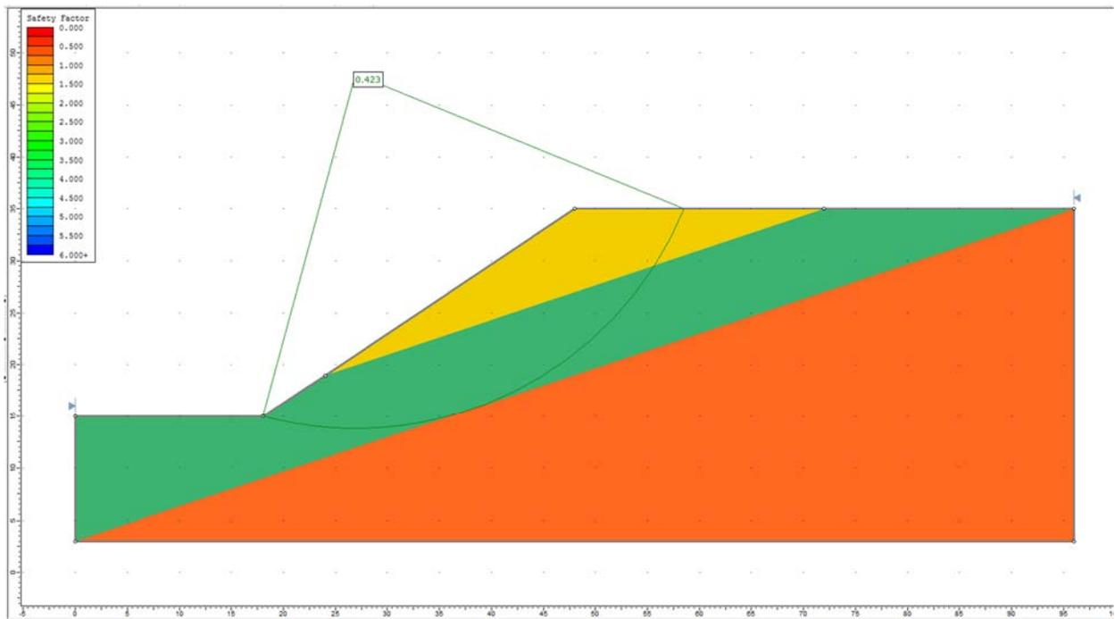
Figure 10.4.4 – Slide Solution Using the Spencer Method
