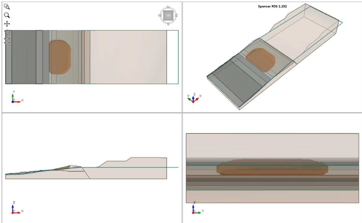
Figure 39.4.7 – Slide3 Solution Using the Spencer Method
