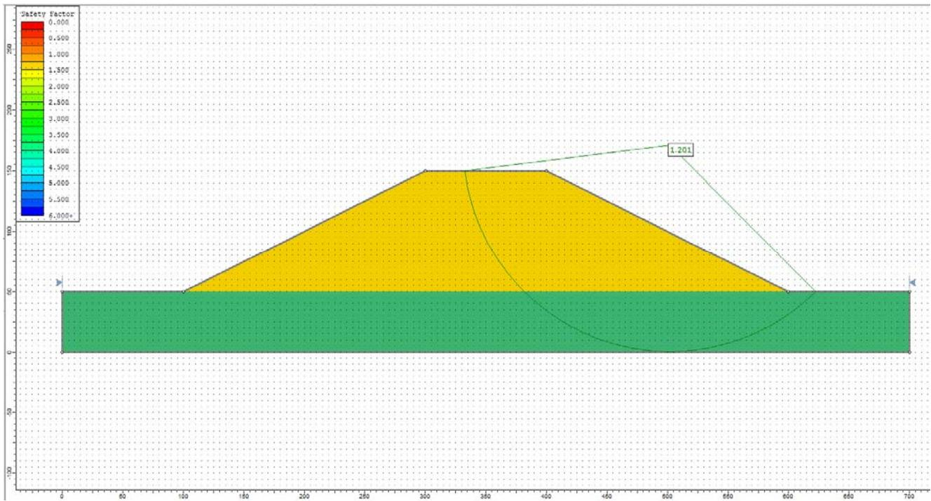
**Figure 29.4.6 – Slide Solution Using the Spencer Method**
