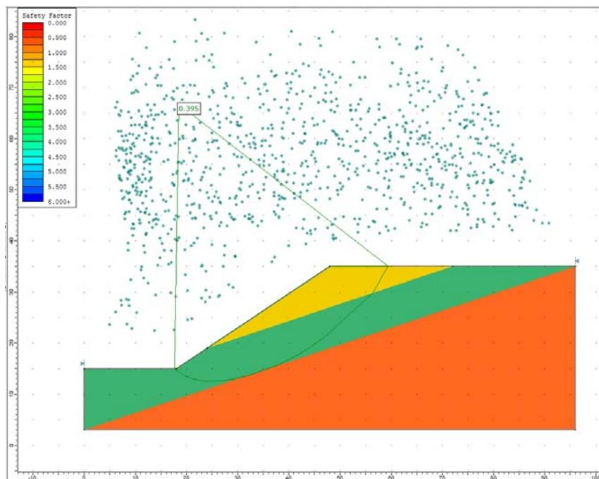
**Figure 11.4.2 – Slide Solution Using the Janbu Method**
