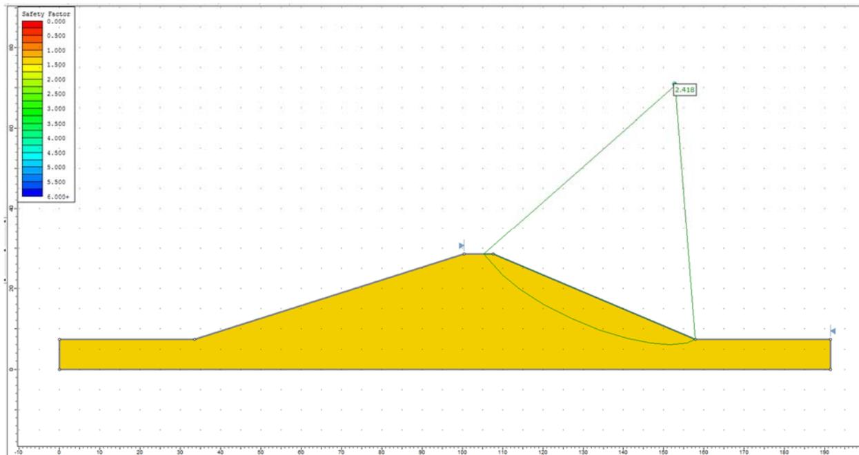
**Figure 12.4.2 – Slide Solution Using the Bishop Method**
