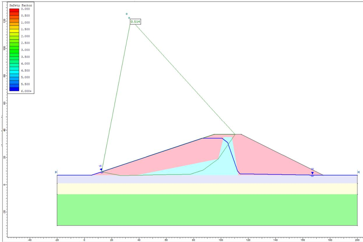
Figure 42.4.4 – Slide Solution Using the GLE Method
