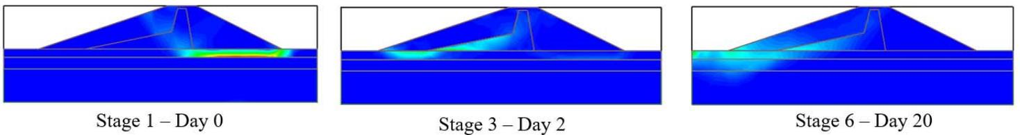
**Figure 42.6.1 – RS3 Maximum Shear Strain by Stage**
