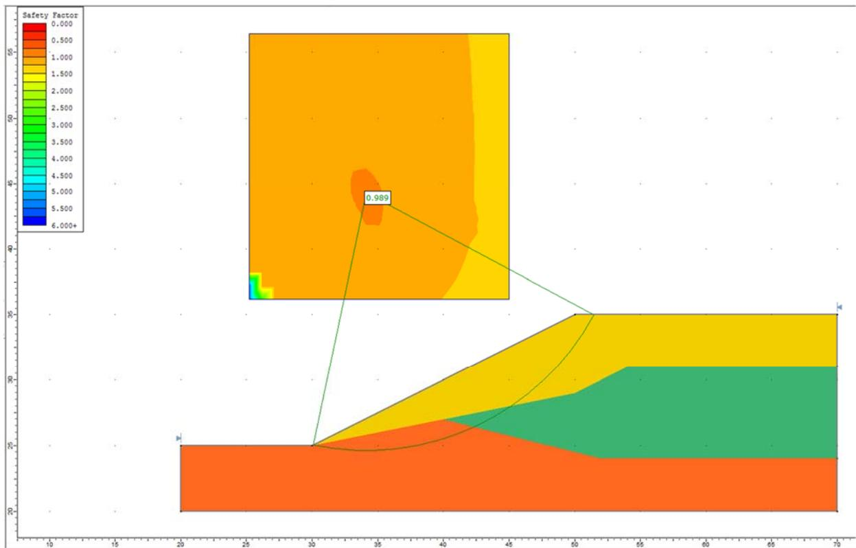
**Figure 5.4.6 – Slide Solution Using the GLE Method**
