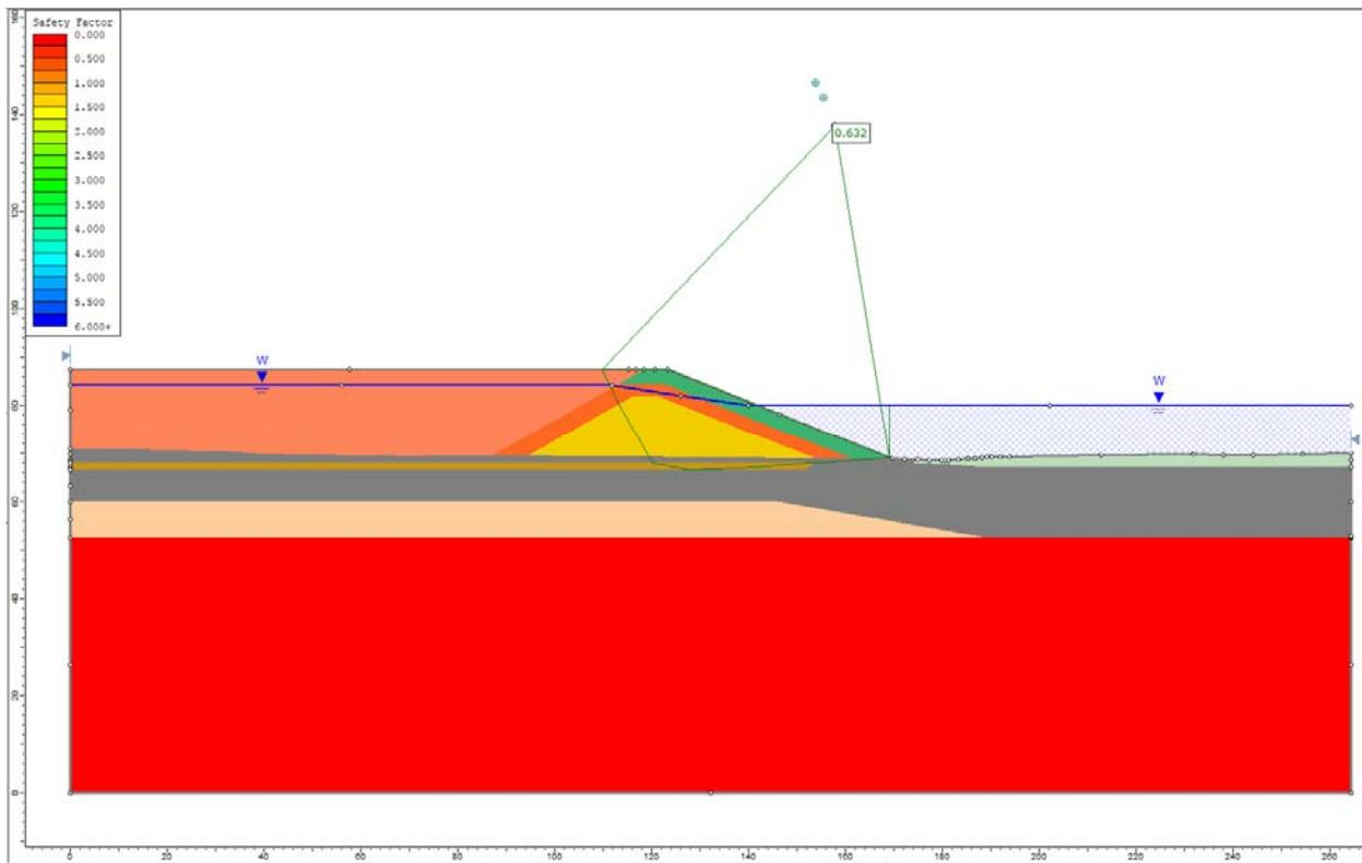
**Figure 45.4.6 – Slide Solution Using the Janbu Method**
