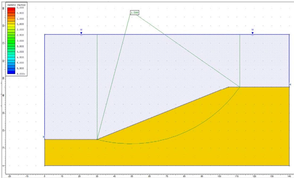
**Figure 27.4.6 – Slide Solution Using the Spencer Method**
