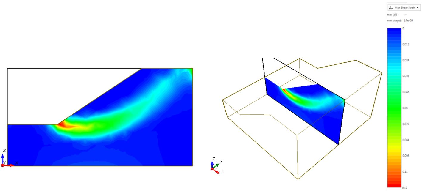
Figure 8.4.8 – RS3 Maximum Shear Strain
