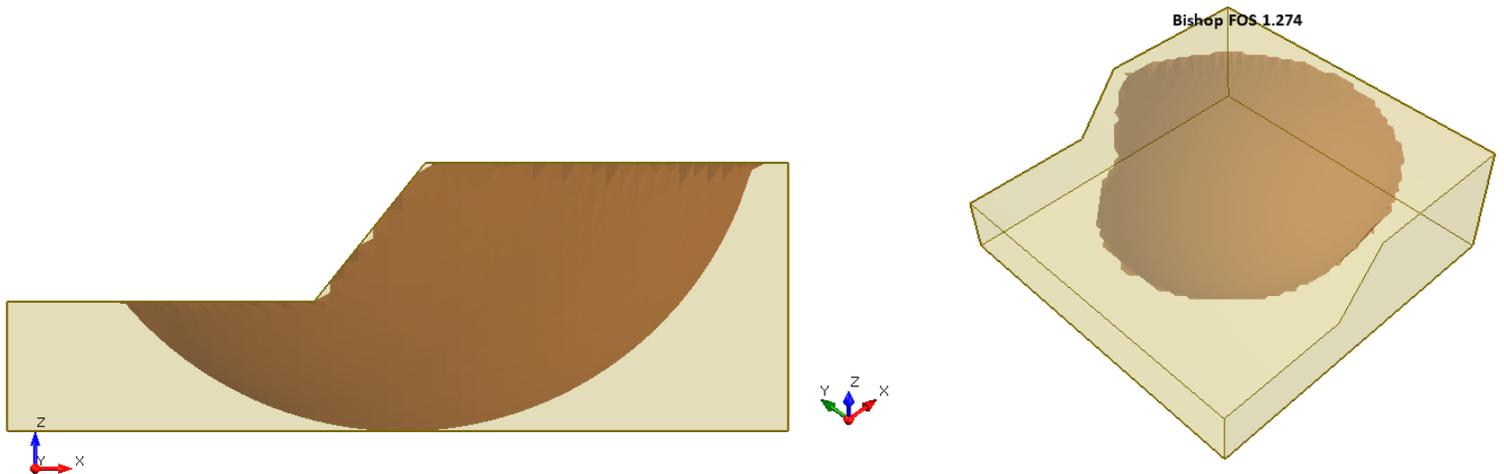
**Figure 36.4.1 – Slide3 Solution Using the Bishop Method**
