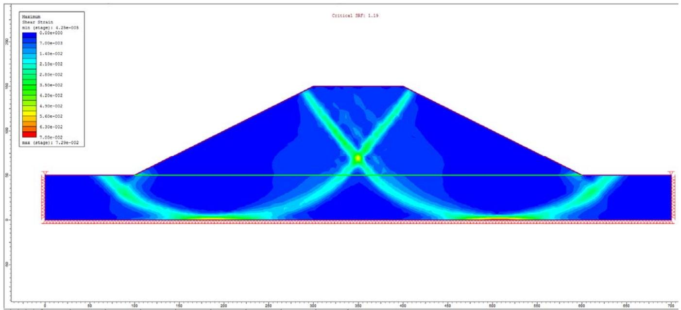
Figure 29.4.7 – RS2 Maximum Shear Strain
