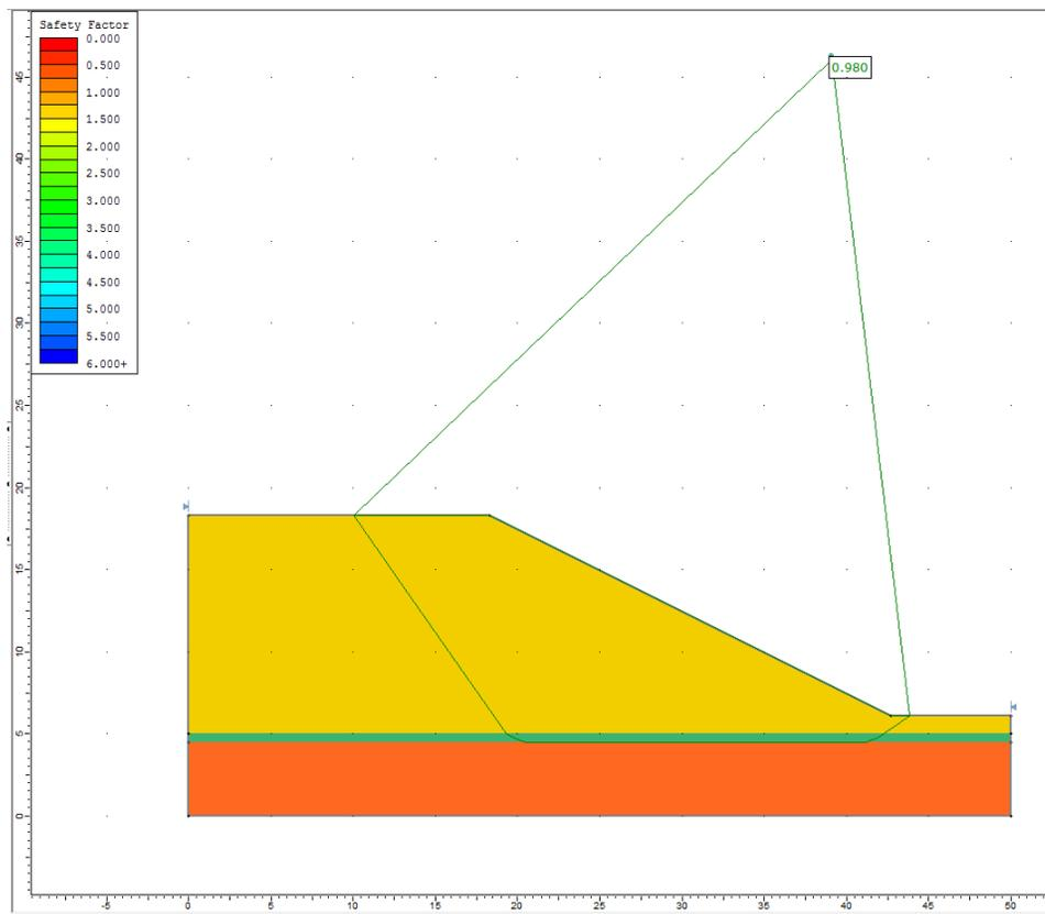
Figure 15.4.6 – Slide Solution Using the Janbu Method
