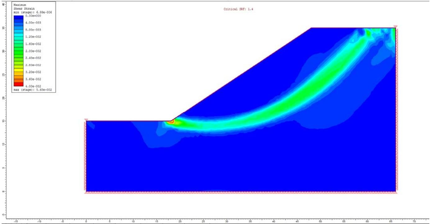
Figure 9.4.7 – RS2 Maximum Shear Strain
