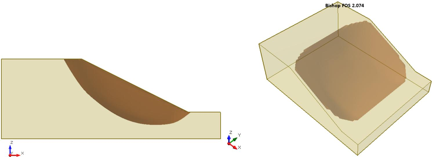
**Figure 14.4.1 – Slide3 Solution Using the Bishop Method**
