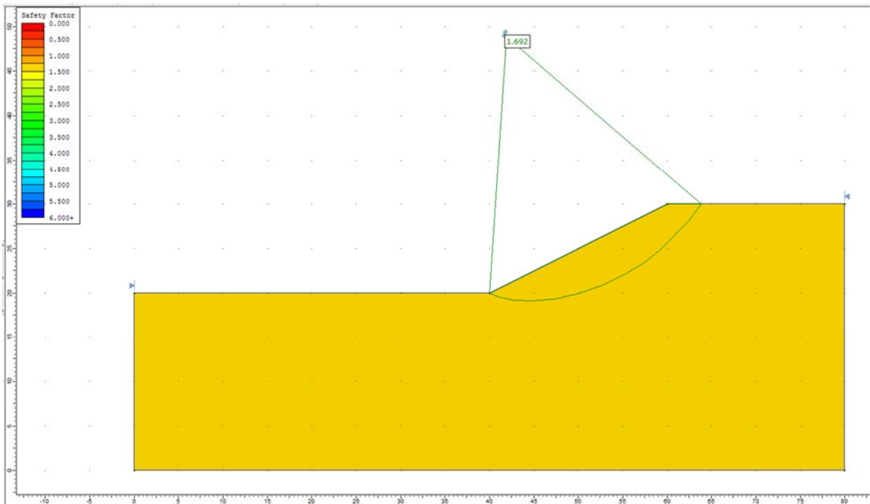
**Figure 19.4.8 – Slide Solution Using the Spencer Method**
