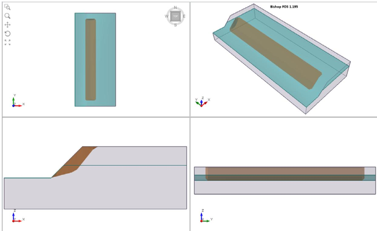
**Figure 25.4.1 – Slide3 User Defined Slip Surface Using Weak Planes**
