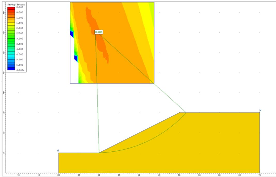
**Figure 1.4.4 – Slide Solution Using the Spencer Method**
