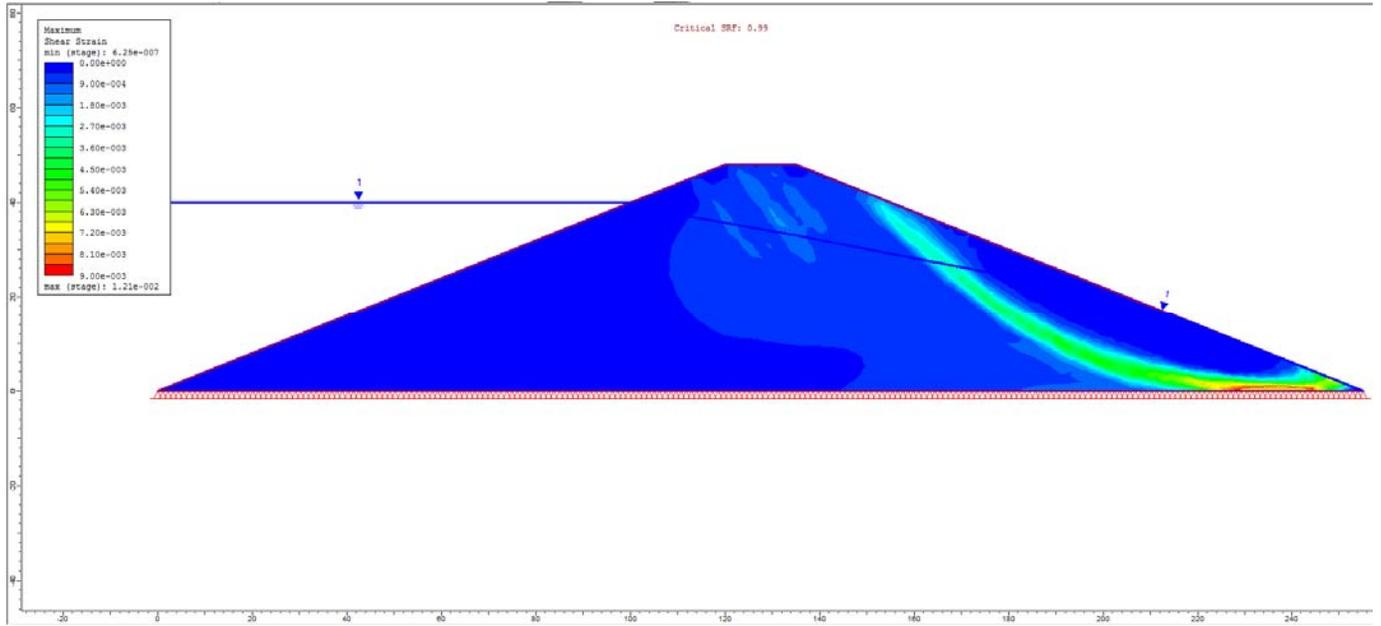
Figure 30.4.7 – RS2 Maximum Shear Strain
