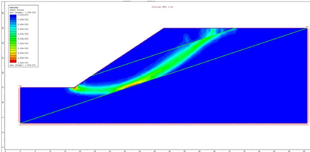
Figure 10.7 – RS2 Maximum Shear Strain
