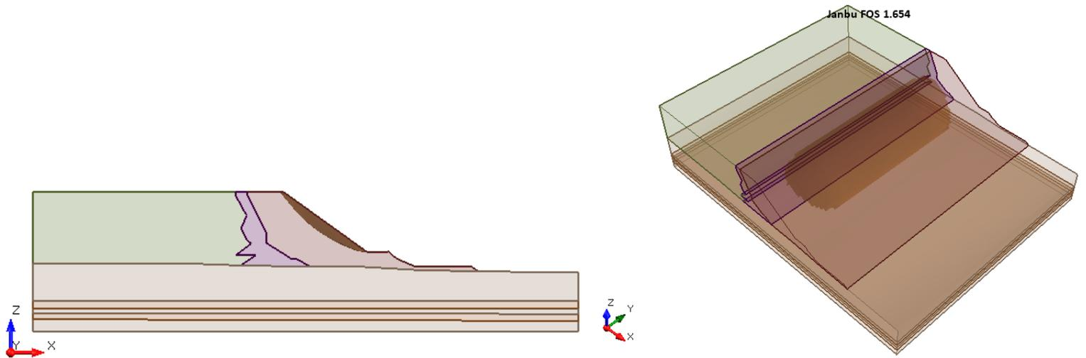
**Figure 46.4.5 – Slide3 Solution Using the Janbu Method**
