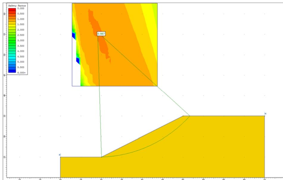
**Figure 1.4.2 – Slide Solution Using the Bishop Method**
