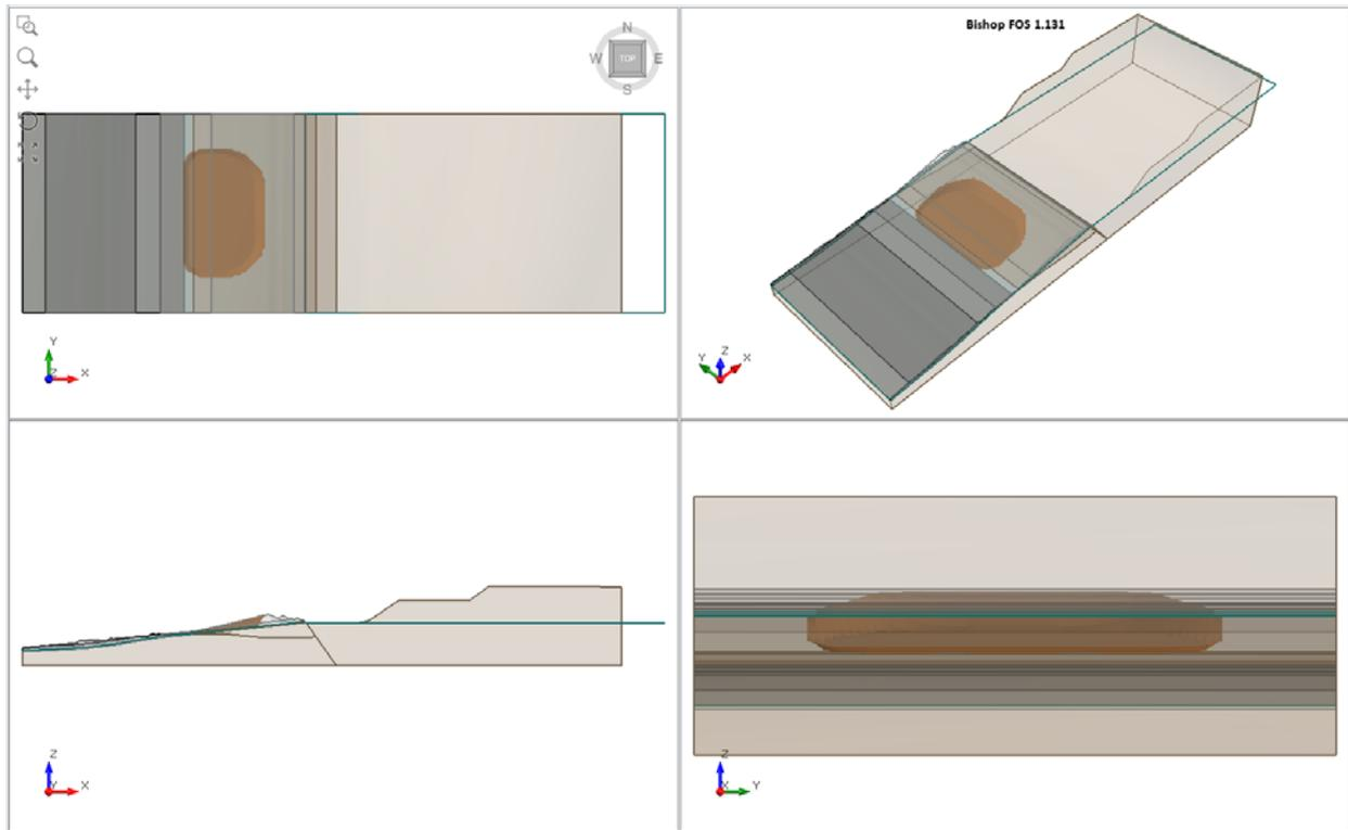
Figure 39.4.1 – Slide3 Solution Using the Bishop Method
