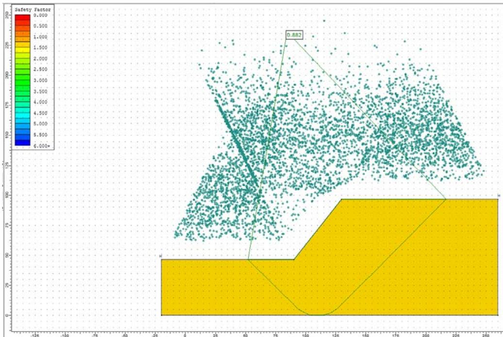
**Figure 37.4.2 – Slide Solution Using the Bishop Method**
