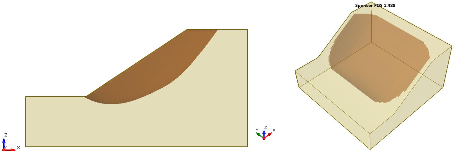
Figure 9.4.3 – Slide3 Solution Using the Spencer Method
