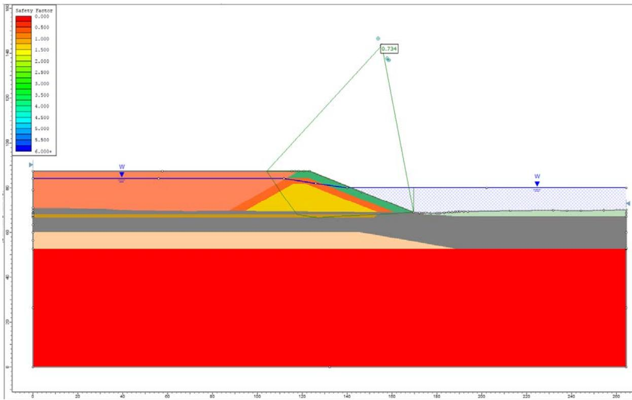
**Figure 45.4.4 – Slide Solution Using the GLE Method**
