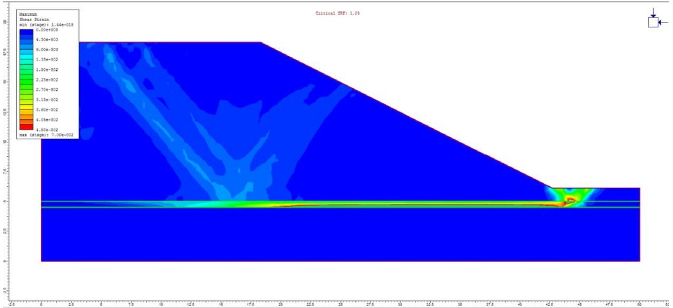
Figure 15.4.9 – RS2 Maximum Shear Strain
