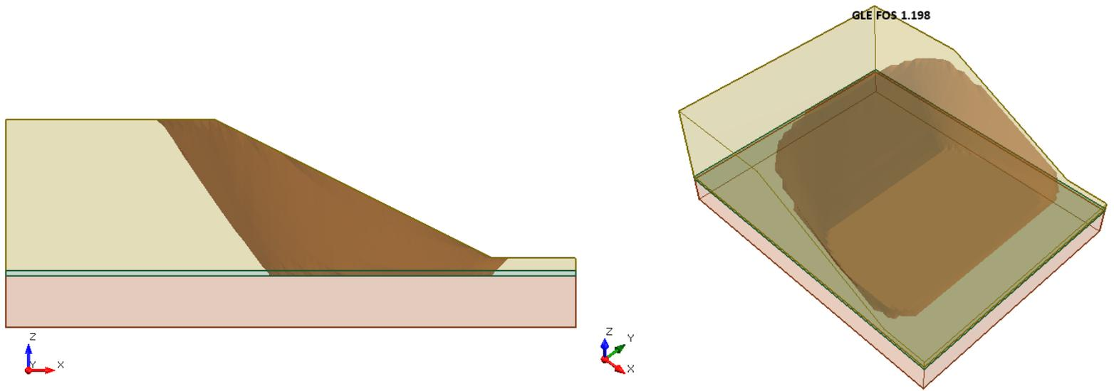
**Figure 15.4.3 – Slide3 Solution Using the GLE Method**
