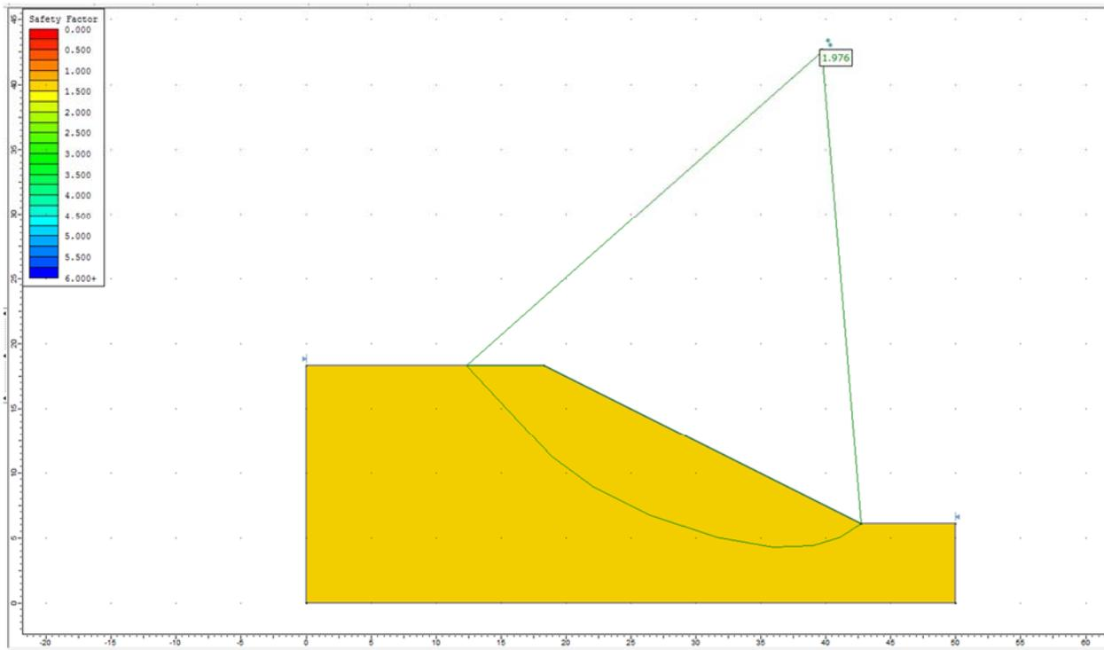
**Figure 14.4.4 – Slide Solution Using the GLE Method**
