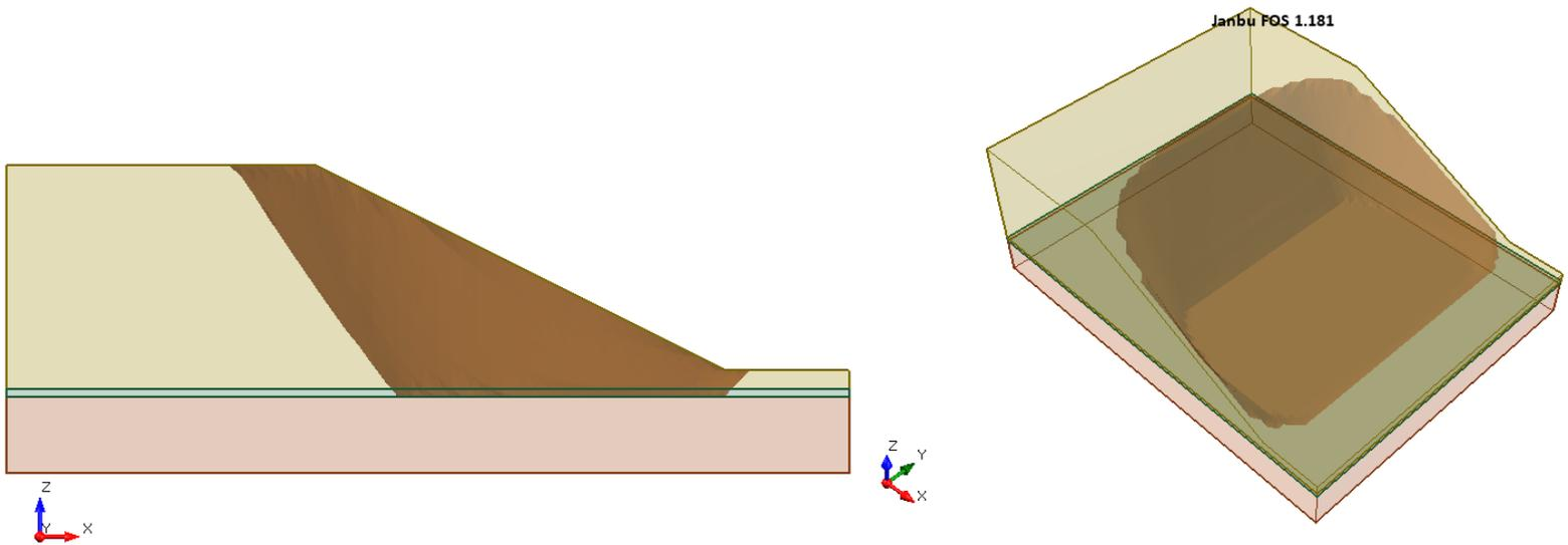
Figure 15.4.5 – Slide3 Solution Using the Janbu Method
