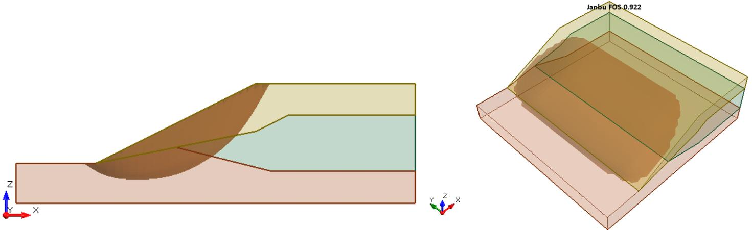
**Figure 6.4.1 – Slide3 Solution Using the Janbu Method**
