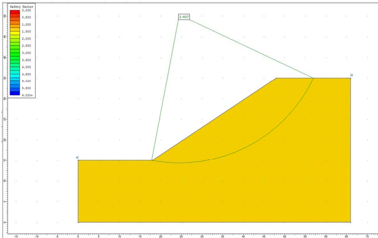
**Figure 8.4.4 – Slide Solution Using the Spencer Method**
