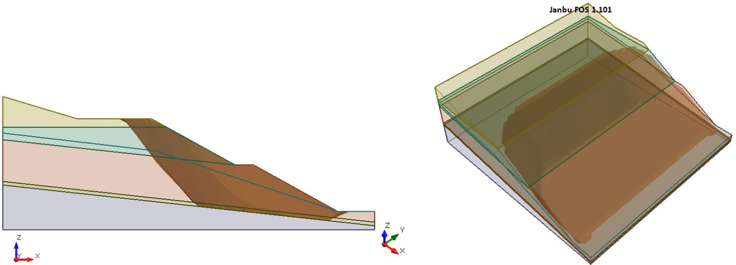
Figure 20.4.5 – Slide3 Solution Using the Janbu Method
