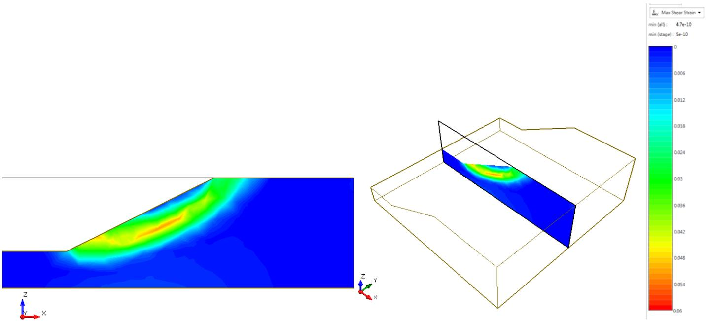
Figure 2.4.8 – RS3 Maximum Shear Strain
