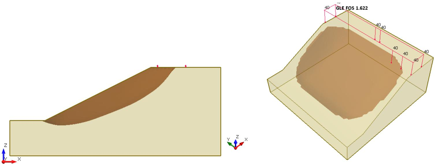
**Figure 21.4.3 – Slide3 Solution Using the GLE Method**
