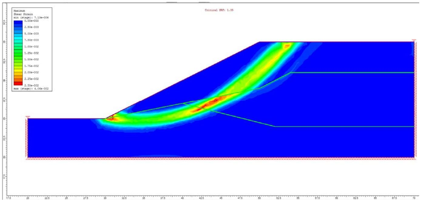
Figure 3.4.7 – RS2 Maximum Shear Strain
