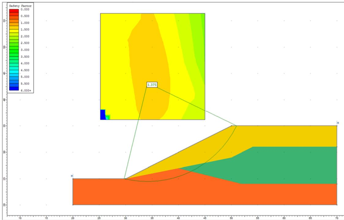
**Figure 3.4.4 – Slide Solution Using the Spencer Method**
