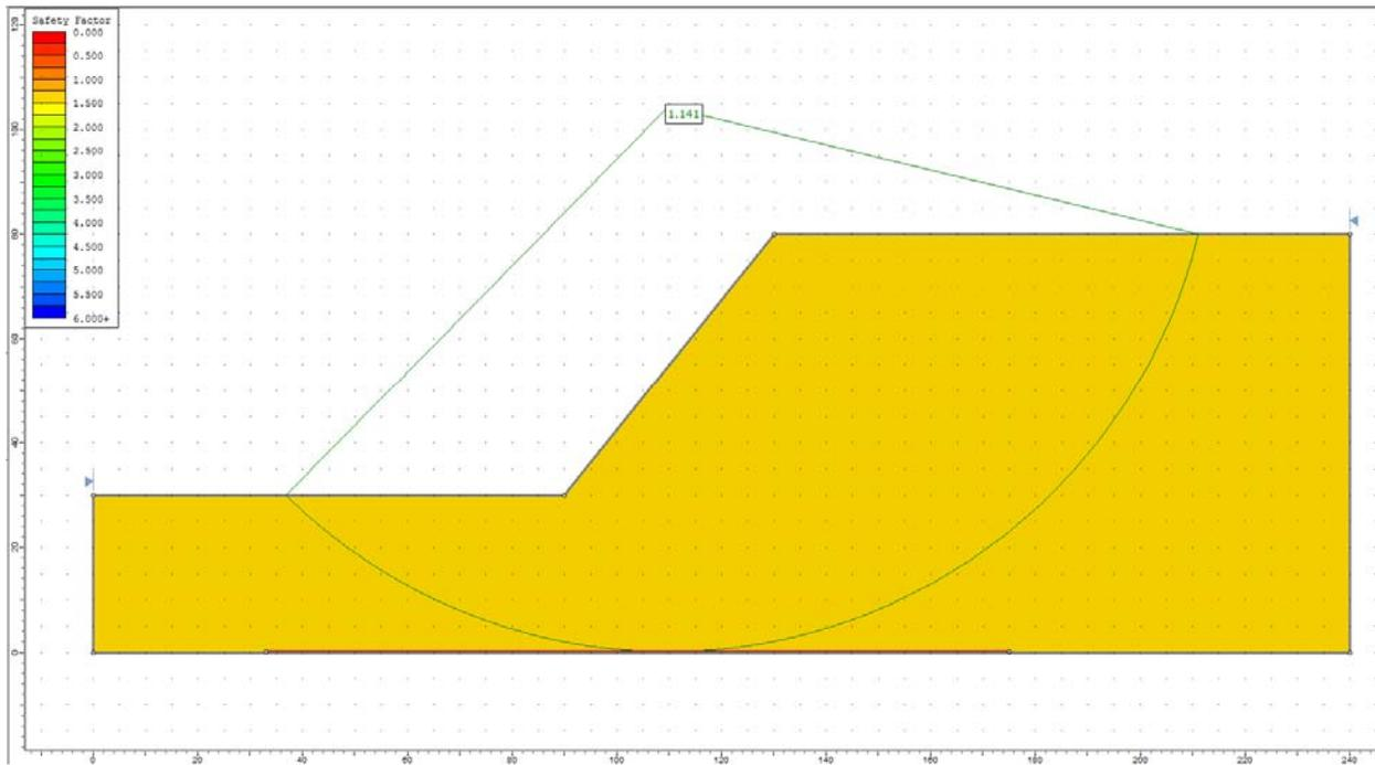
**Figure 34.4.2 – Slide Solution Using the Bishop Method**
