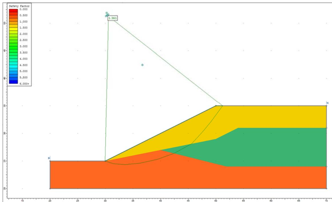
**Figure 4.4.4 – Slide Solution Using the Spencer Method**
