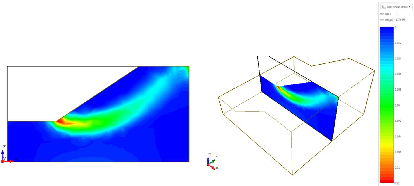
Figure 9.4.8 – RS3 Maximum Shear Strain
