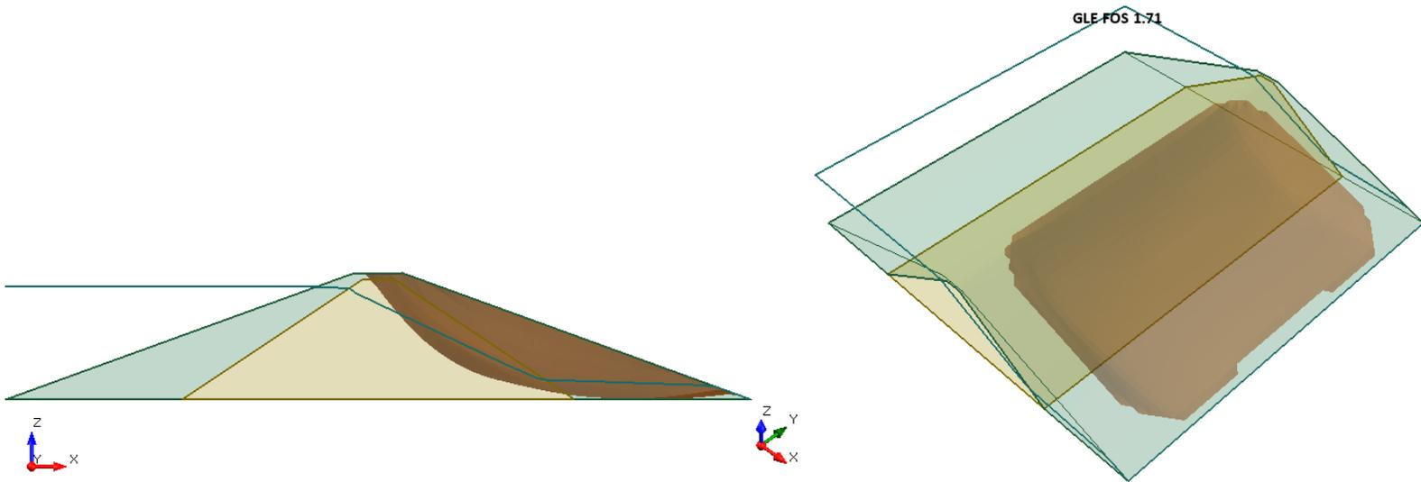
**Figure 33.4.3 – Slide3 Solution Using the GLE Method**
