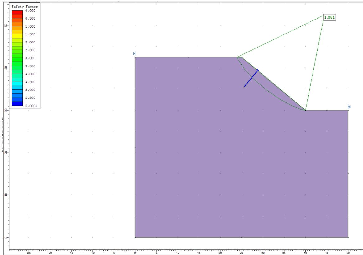
**Figure 22.4.8 – Slide Solution Using the Spencer Method**
