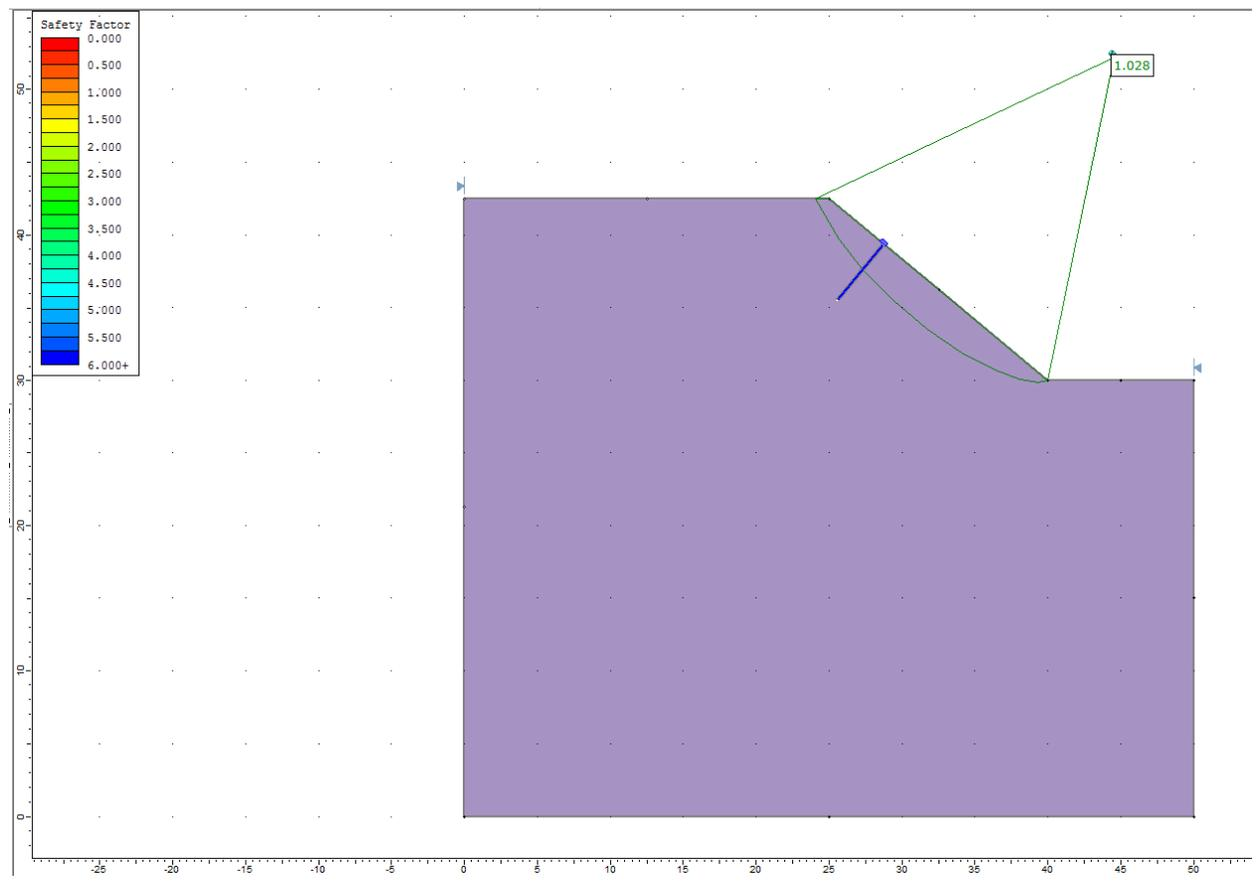
**Figure 22.4.6 – Slide Solution Using the Janbu Method**
