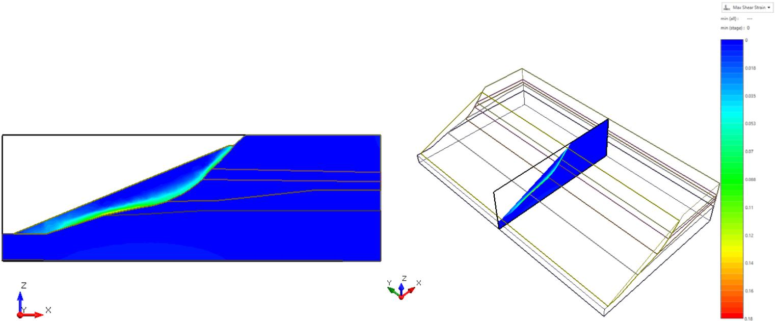
Figure 44.4.10 – RS3 Maximum Shear Strain
