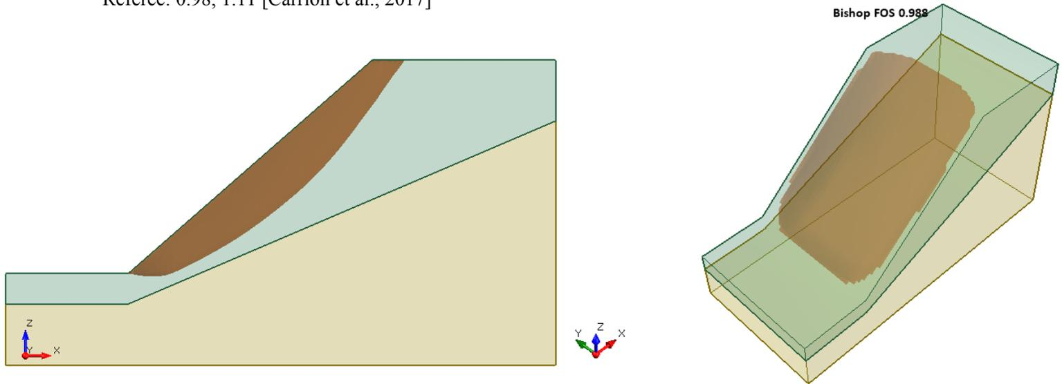
**Figure 17.4.1 – Slide3 Solution Using the Bishop Method**
