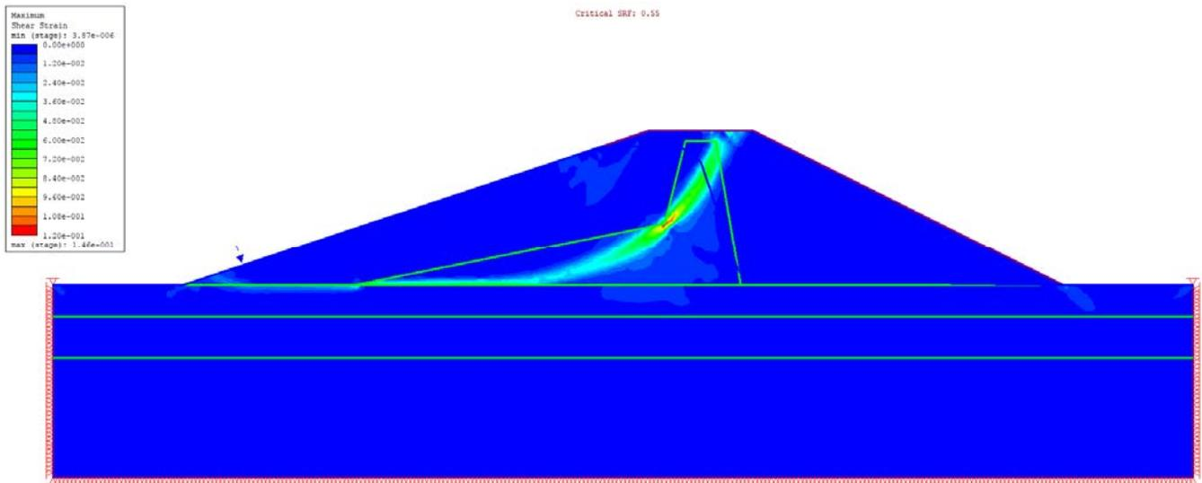
Figure 42.4.9 – RS2 Maximum Shear Strain
