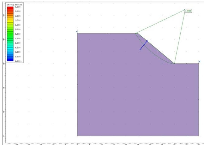
**Figure 22.4.2 – Slide Solution Using the Bishop Method**
