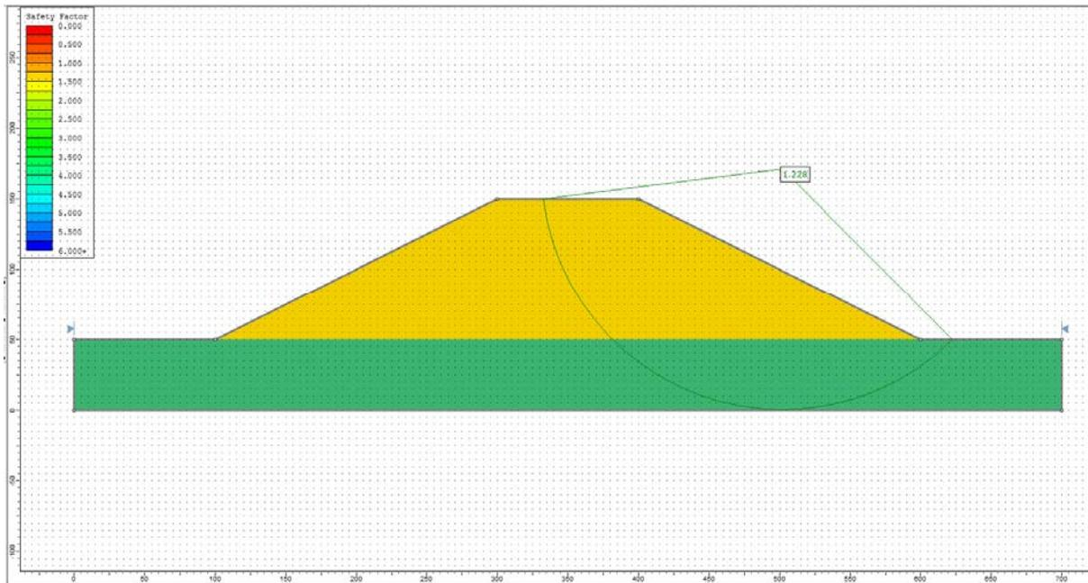
**Figure 29.4.2 – Slide Solution Using the Bishop Method**
