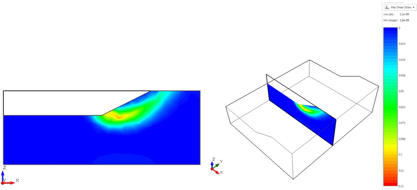
Figure 19.4.10 – RS3 Maximum Shear Strain
