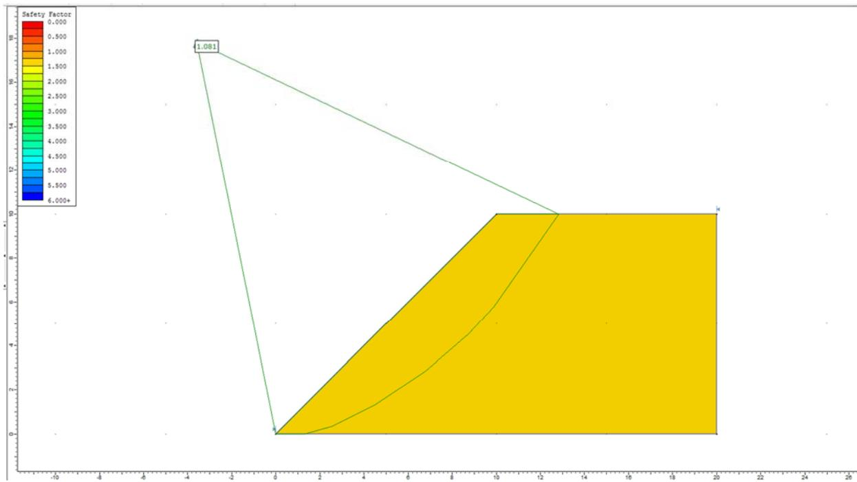
**Figure 18.4.4 – Slide Solution Using the GLE Method**
