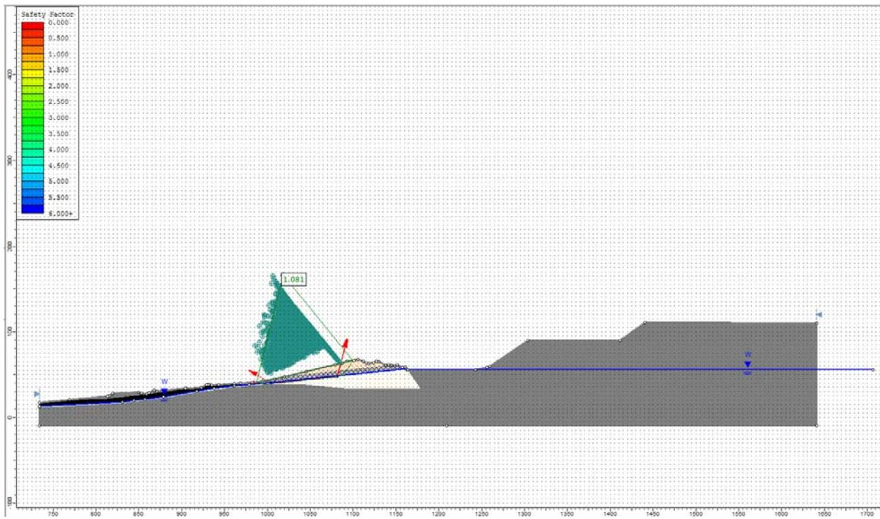
Figure 39.4.8 – Slide3 Solution Using the Spencer Method
