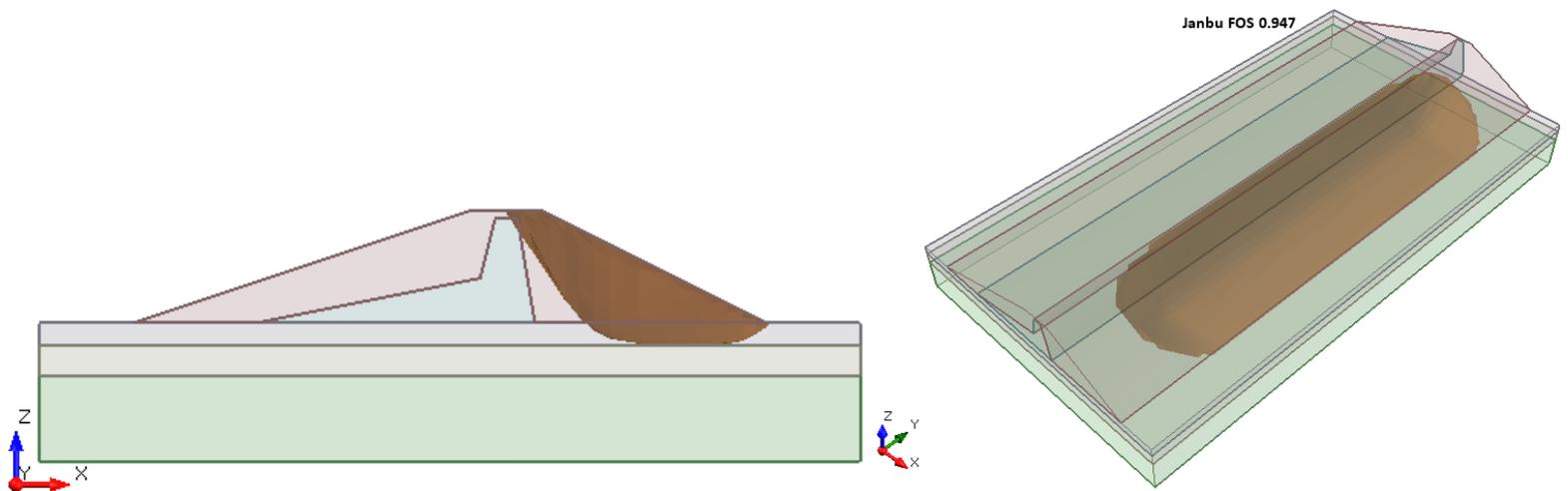
**Figure 40.4.5 – Slide3 Solution Using the Janbu Method**
