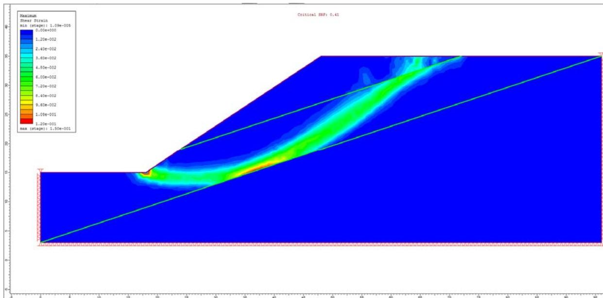
Figure 11.7 – RS2 Maximum Shear Strain
