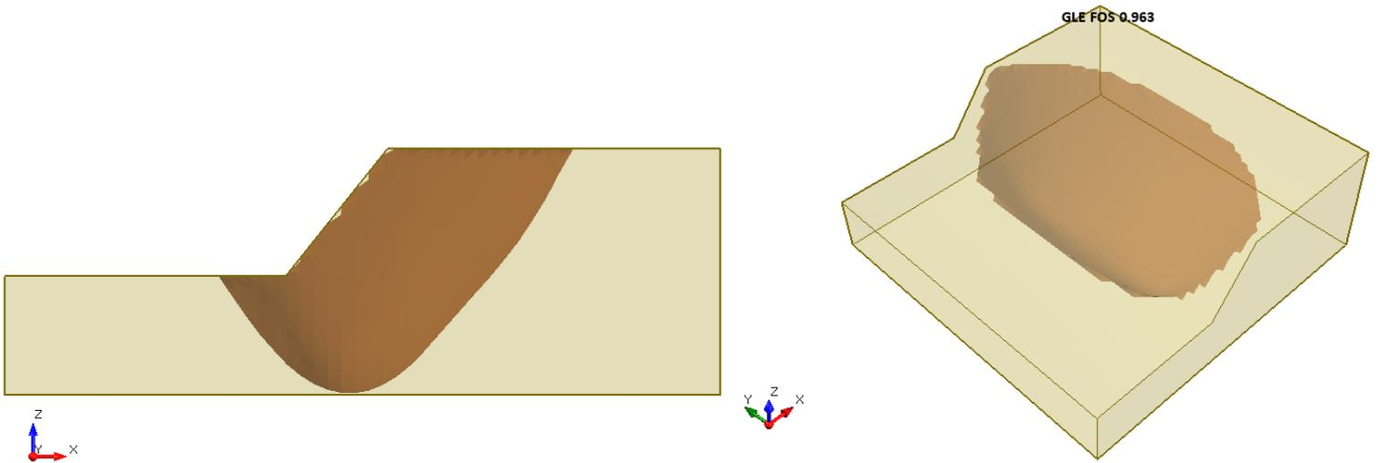
**Figure 37.4.3 – Slide3 Solution Using the GLE Method**
