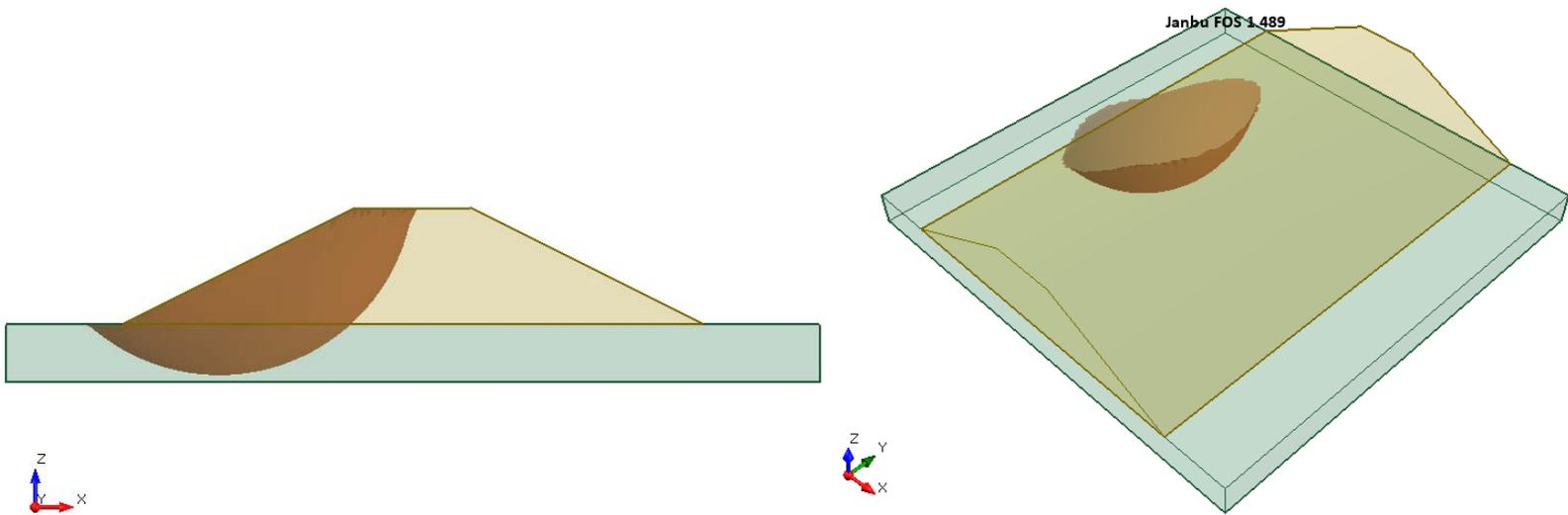
**Figure 29.4.3 – Slide3 Solution Using the Janbu Method**
