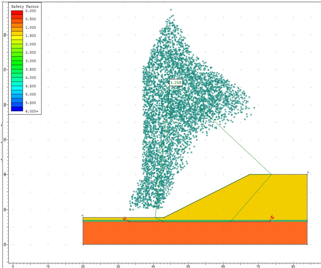
Figure 7.4.4 – Slide Solution Using the Spencer Method
