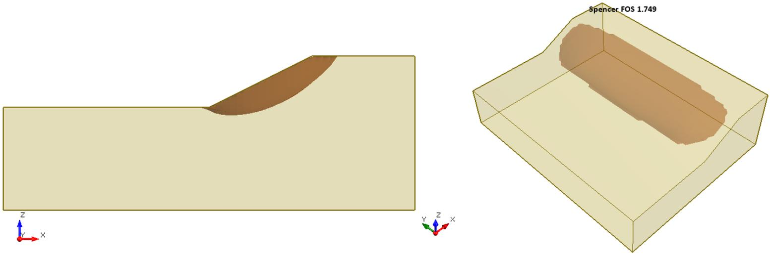
**Figure 19.4.7 – Slide3 Solution Using the Spencer Method**
