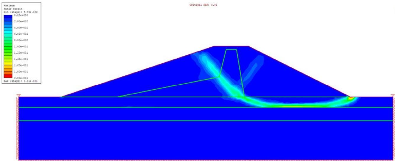
Figure 40.4.9 – RS2 Maximum Shear Strain
