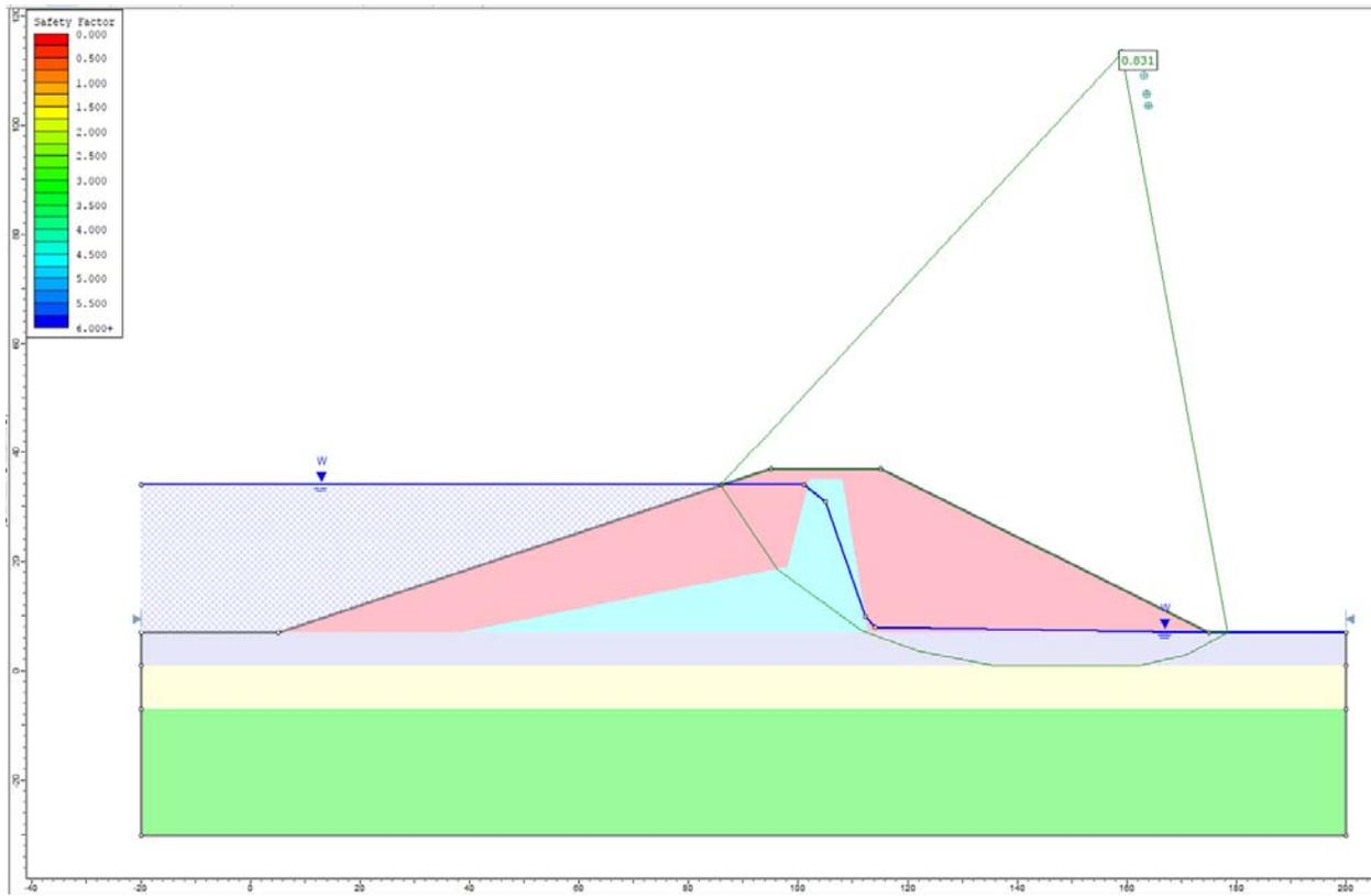
Figure 41.4.8 – Slide Solution Using the Spencer Method
