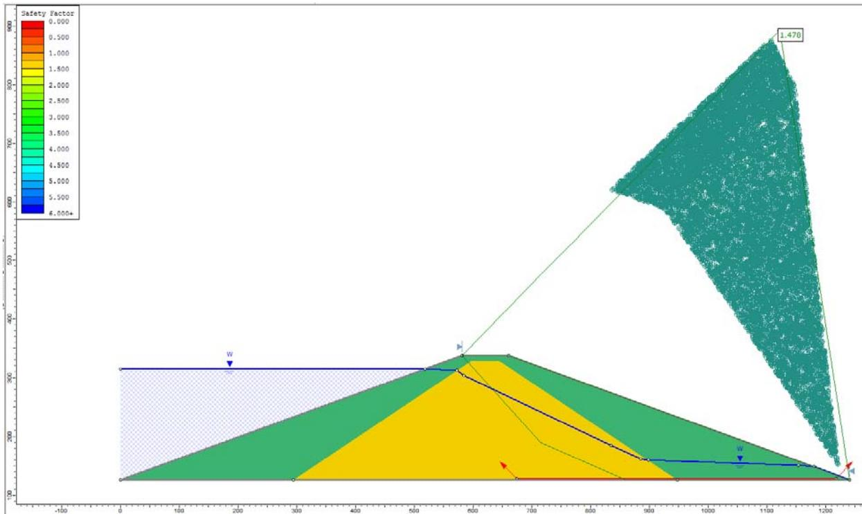
**Figure 33.4.2 – Slide Solution Using the Bishop Method**
