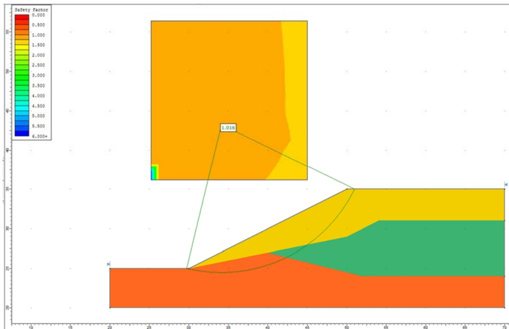
**Figure 5.4.2 – Slide Solution Using the Bishop Method**
