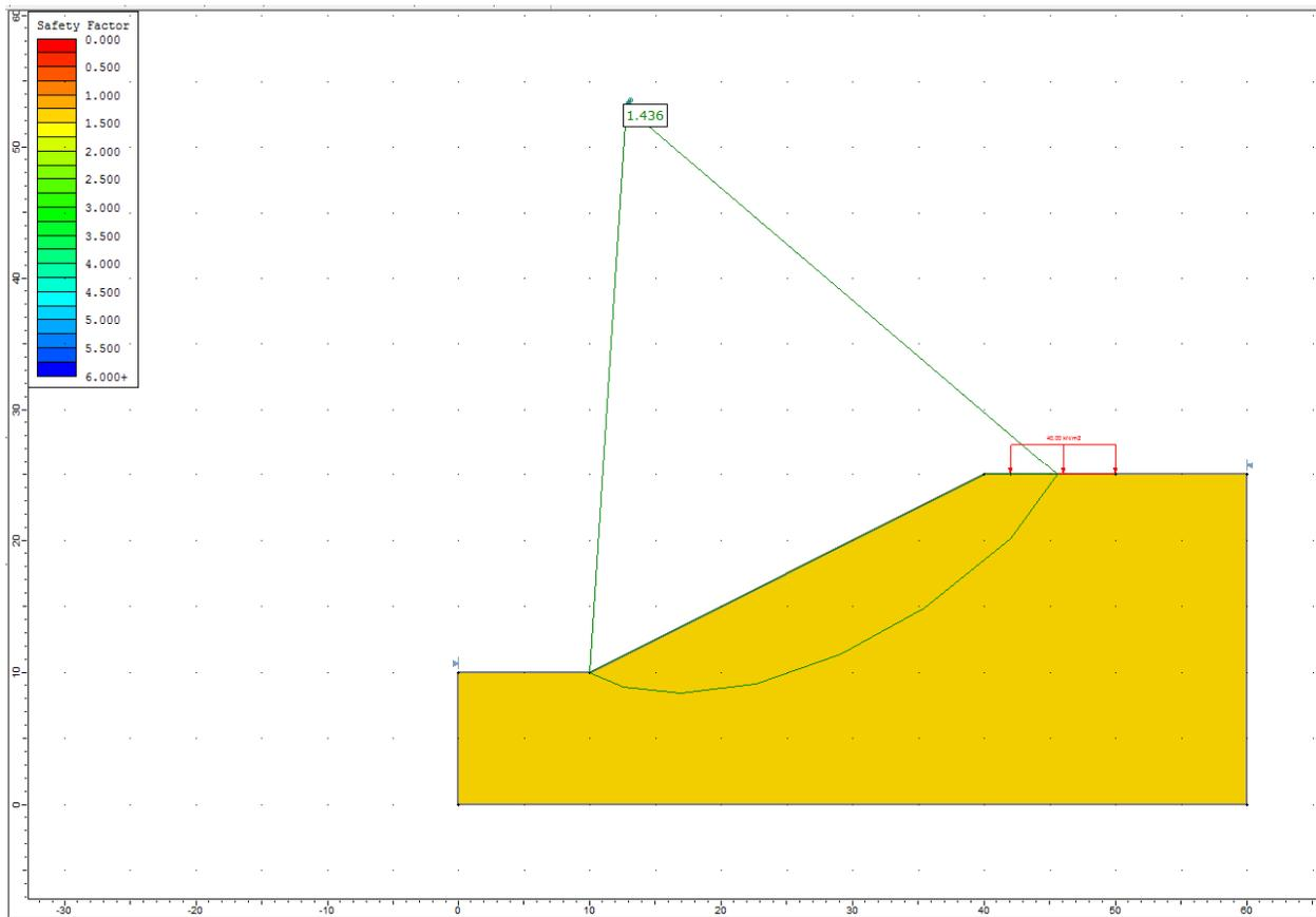
Figure 21.4.6 – Slide Solution Using the Janbu Method
