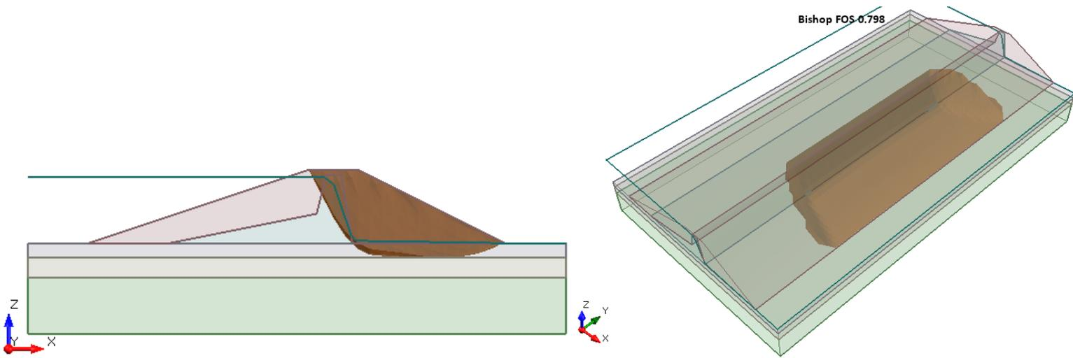
Figure 41.4.1 – Slide3 Solution Using the Bishop Method
