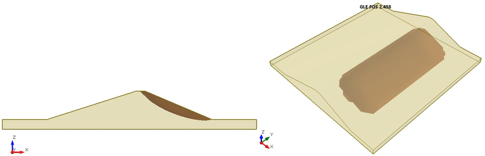
**Figure 12.4.3 – Slide3 Solution Using the GLE Method**
