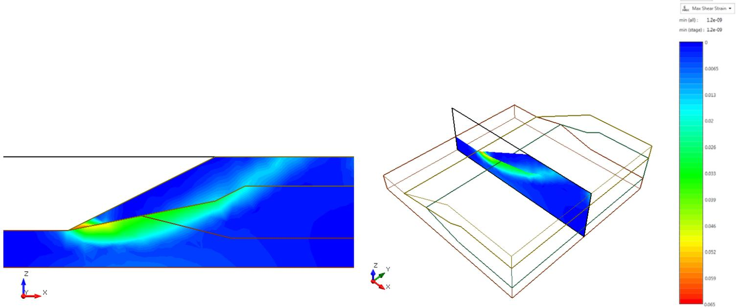
**Figure 6.4.8 – RS3 Maximum Shear Strain Contour in the XZ Plane**
