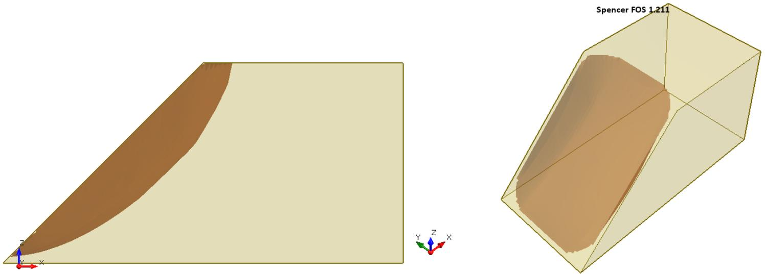
**Figure 18.4.4 – Slide3 Solution Using the Spencer Method**
