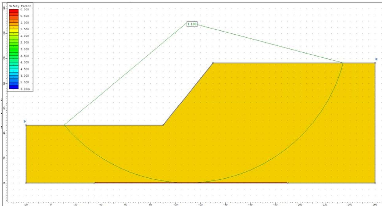
**Figure 36.4.2 – Slide Solution Using the Bishop Method**
