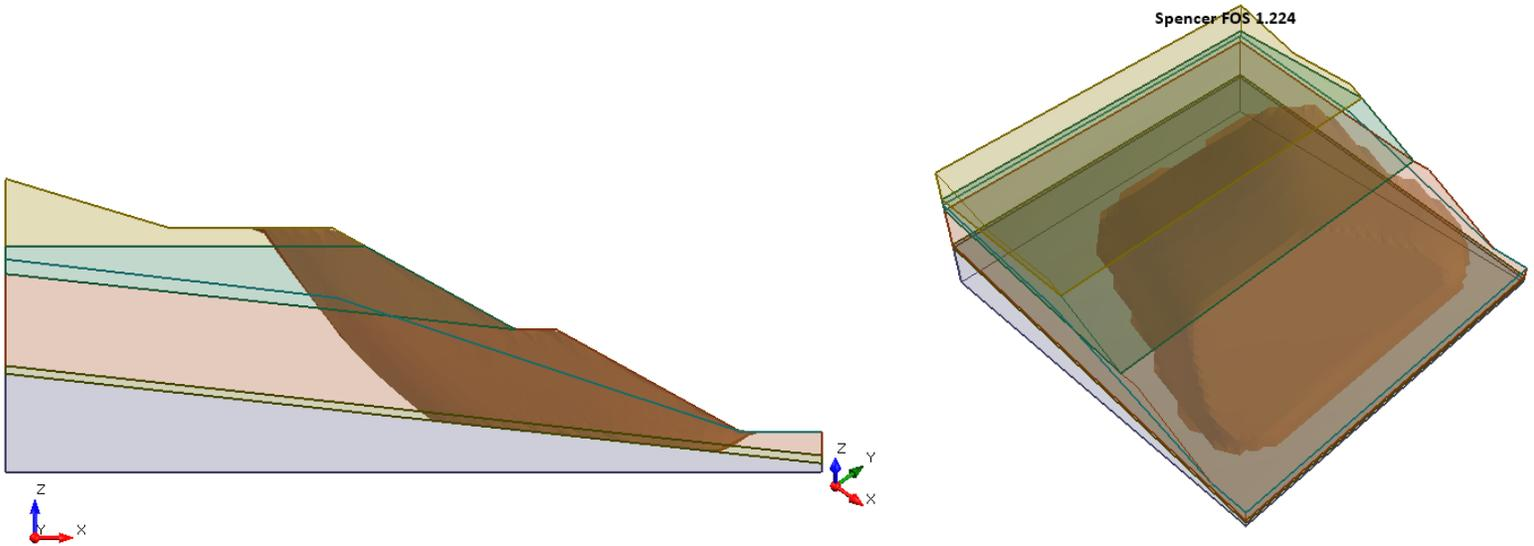
Figure 20.4.7 – Slide3 Solution Using the Spencer Method
