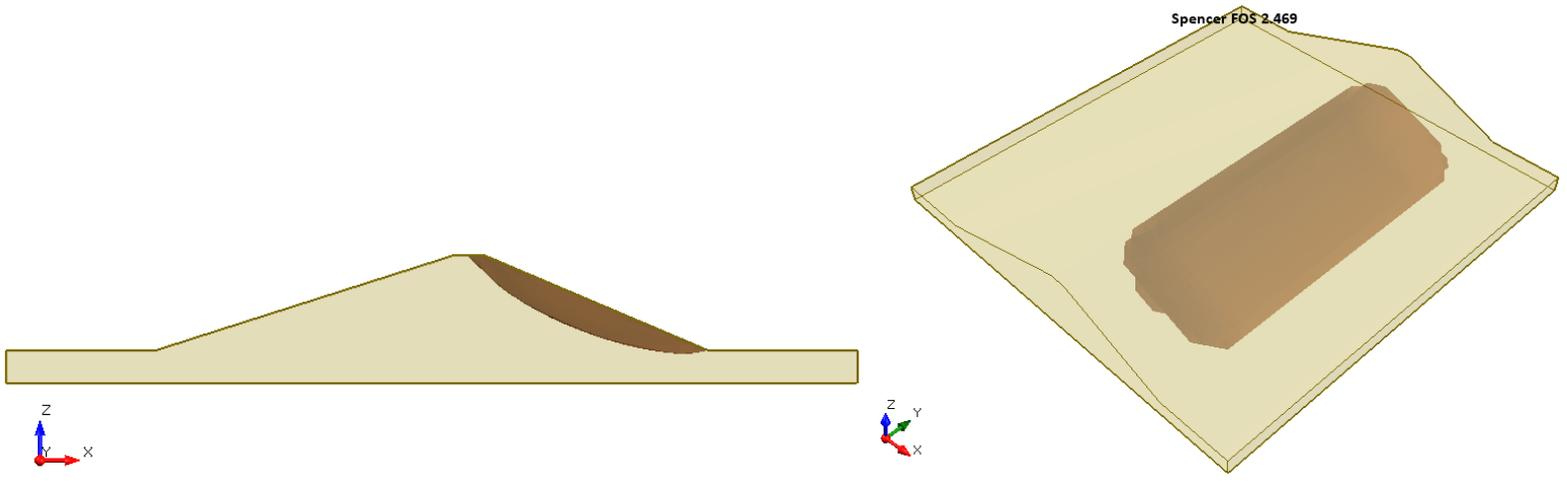
**Figure 12.4.7 – Slide3 Solution Using the Spencer Method**
