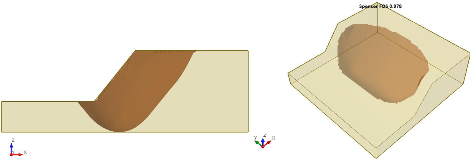
**Figure 35.4.5 – Slide3 Solution Using the Spencer Method**
