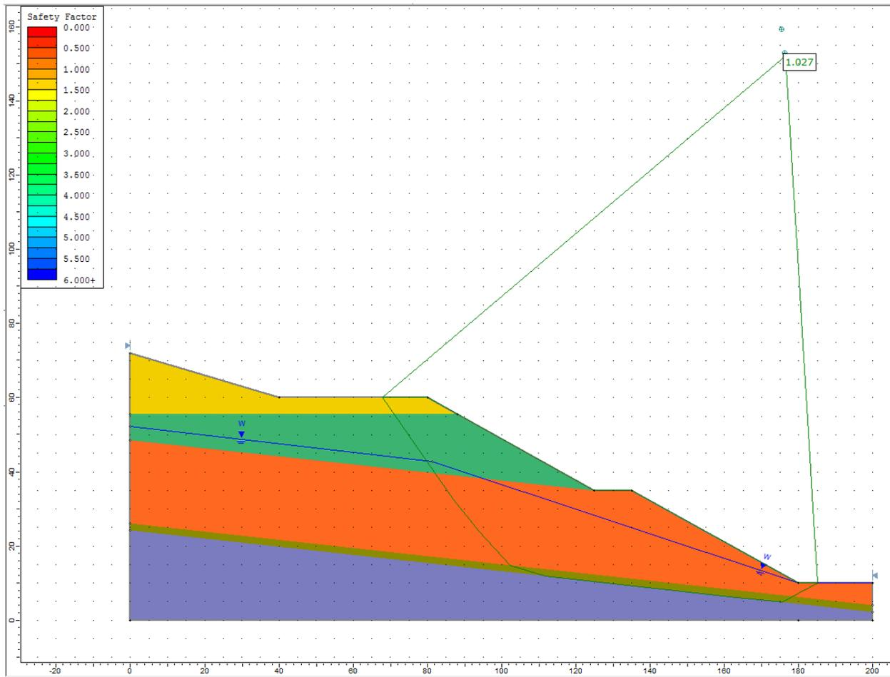
Figure 20.4.6 – Slide Solution Using the Janbu Method
