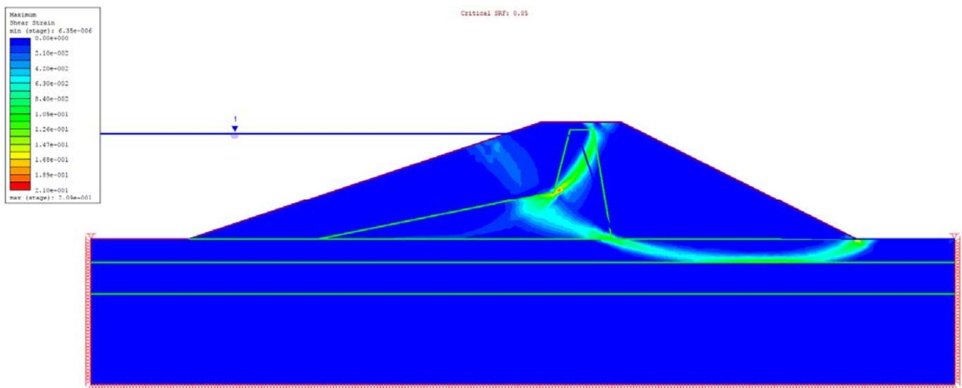
Figure 41.4.9 – RS2 Maximum Shear Strain
