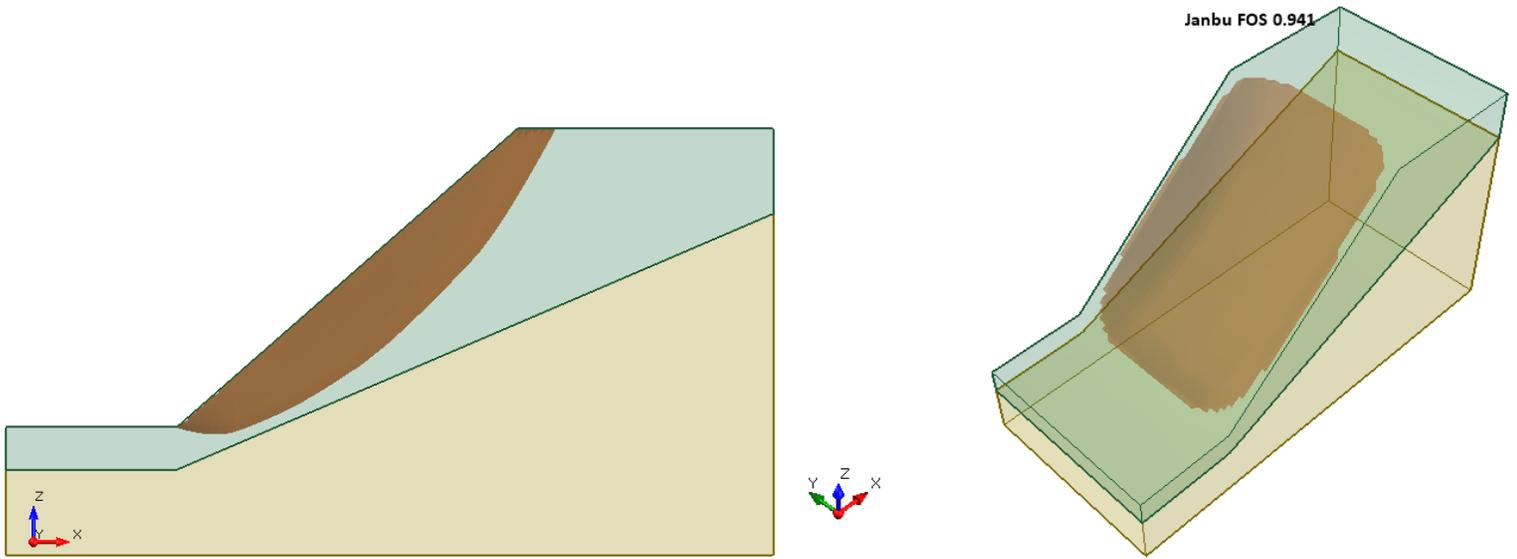
Figure 17.4.5 – Slide3 Solution Using the Janbu Method
