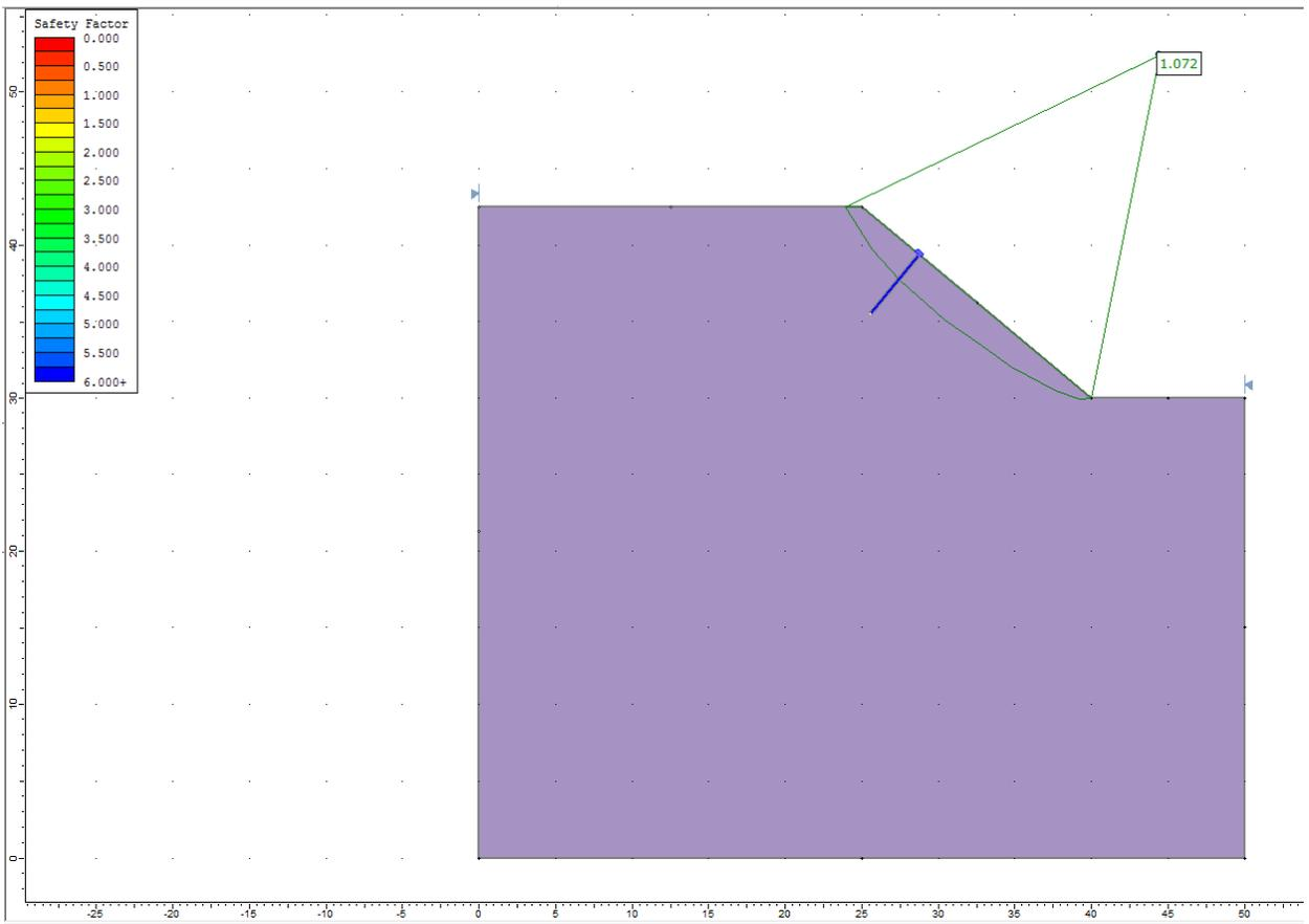
**Figure 22.4.4 – Slide Solution Using the GLE Method**
