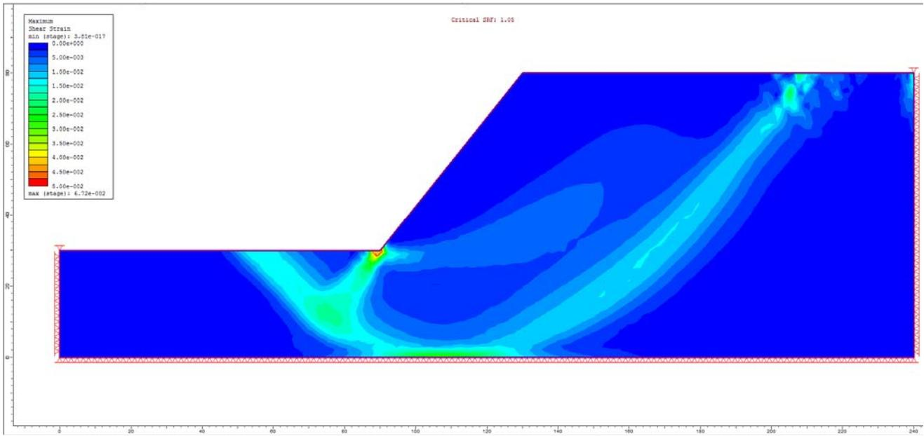
Figure 34.4.7 – RS2 Maximum Shear Strain
