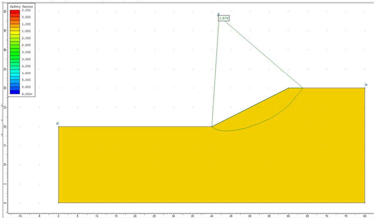
**Figure 19.4.4 – Slide Solution Using the GLE Method**
