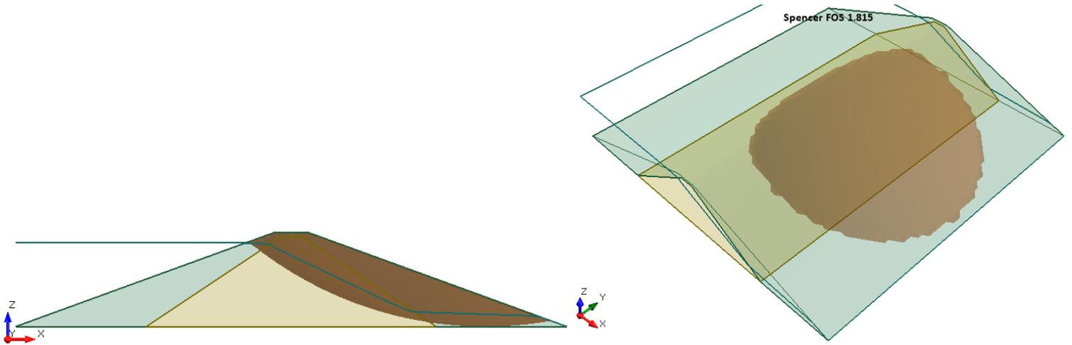
**Figure 32.4.5 – Slide3 Solution Using the Spencer Method**
