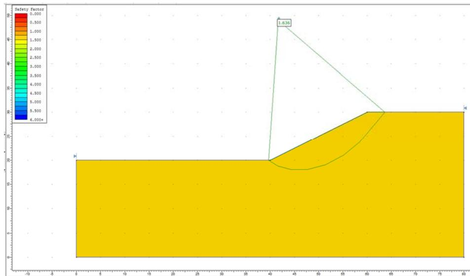
**Figure 19.4.2 – Slide Solution Using the Bishop Method**
