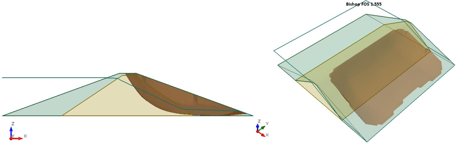
**Figure 33.4.1 – Slide3 Solution Using the Bishop Method**
