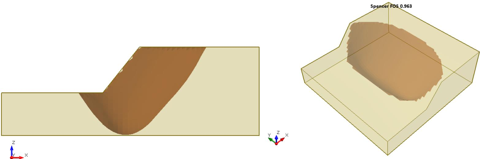
**Figure 37.4.5 – Slide3 Solution Using the Spencer Method**
