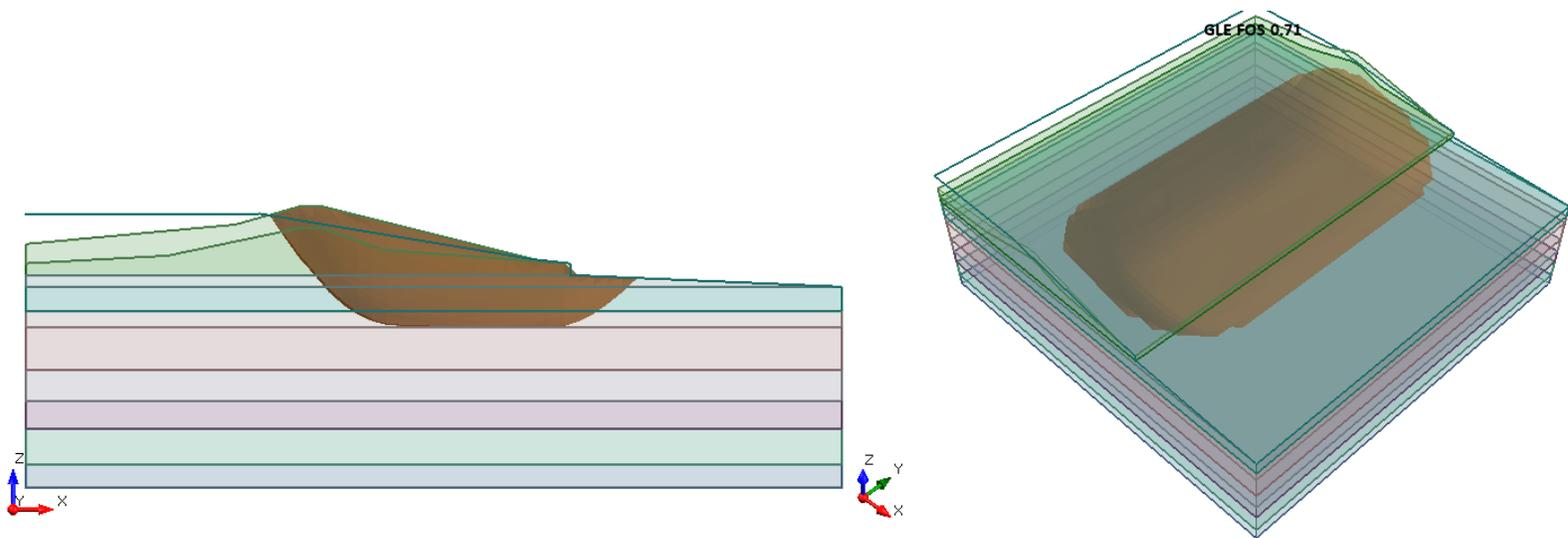
Figure 43.4.3 – Slide3 Solution Using the GLE Method
