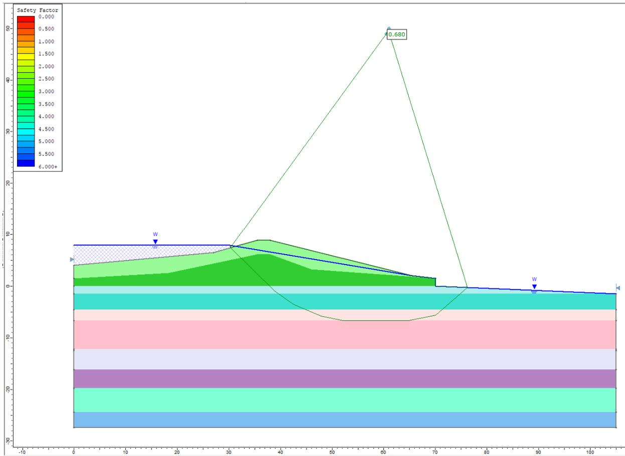
Figure 43.4.8 – Slide Solution Using the Spencer Method
