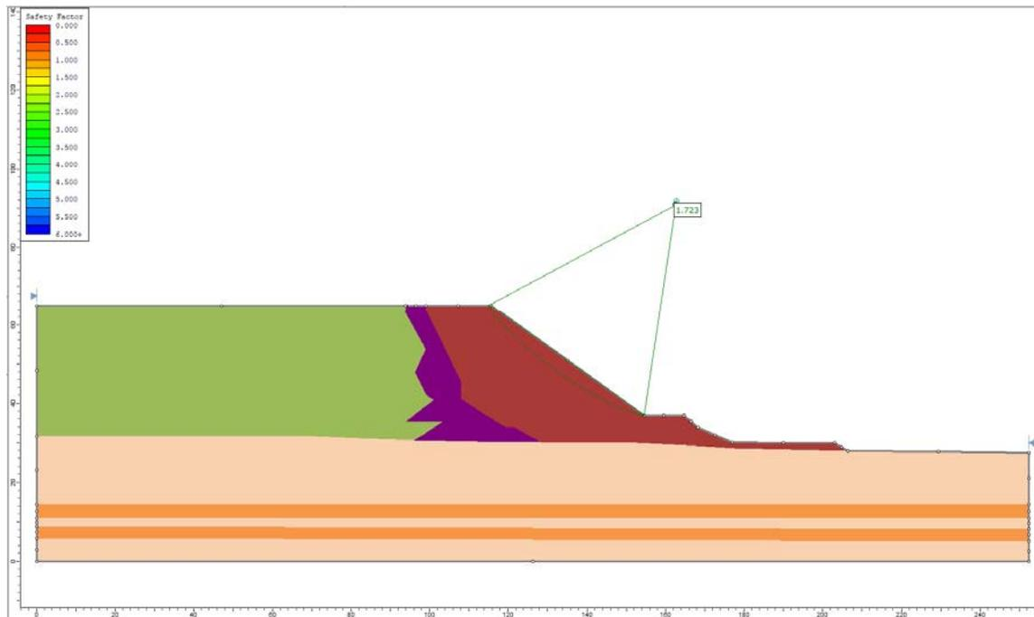
**Figure 46.4.2 – Slide Solution Using the Bishop Method**
