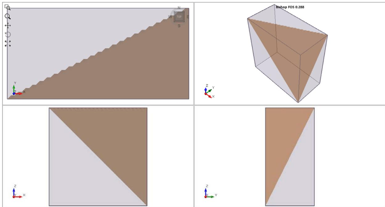
**Figure 38.4.1 – Slide3 Solution Using a Weak Plane Slip Surface**
