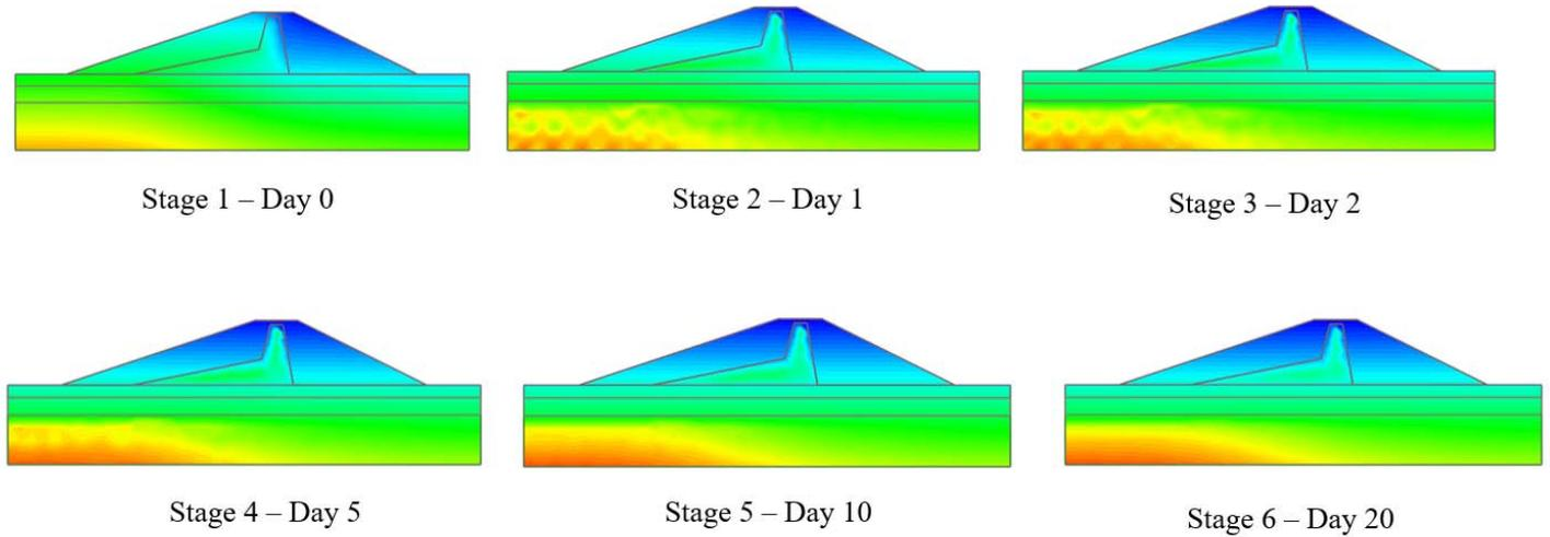
**Figure 42.6.2 – RS3 Pore Pressure by Stage**
