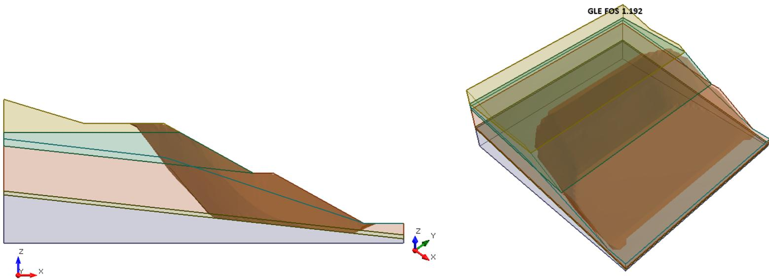
Figure 20.4.3 – Slide3 Solution Using the GLE Method
