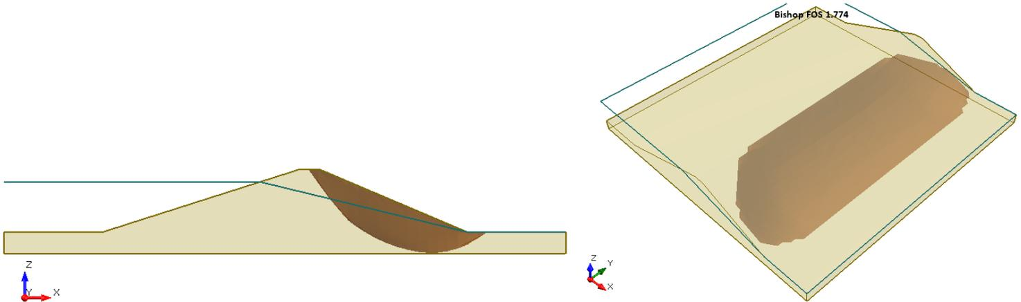
**Figure 13.4.1 – Slide3 Solution Using the Bishop Method**
