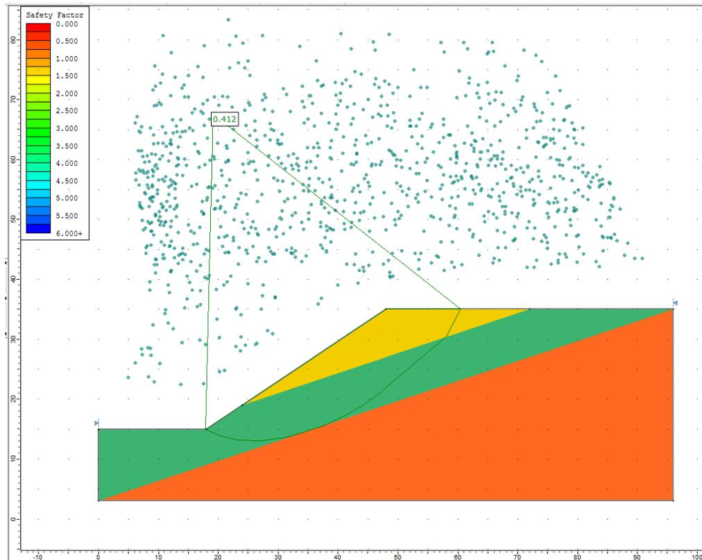
**Figure 11.4.4 – Slide Solution Using the Spencer Method**
