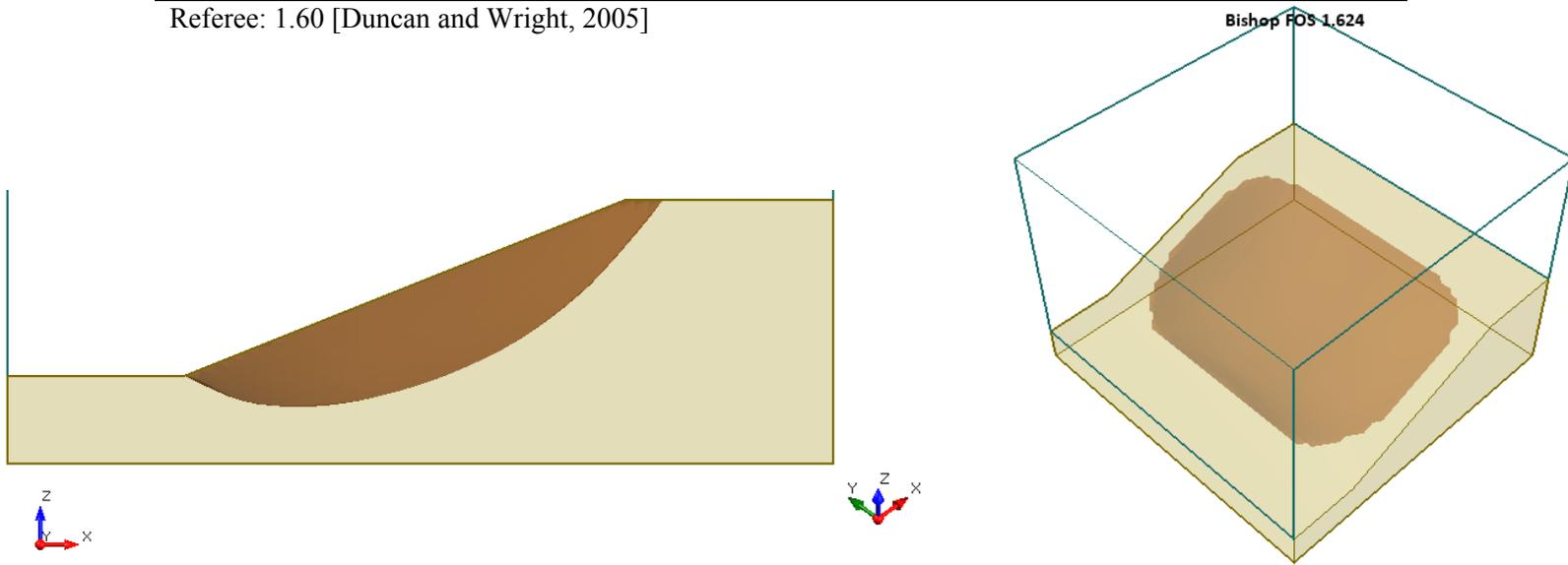
**Figure 28.4.1 – Slide3 Solution Using the Bishop Method**
