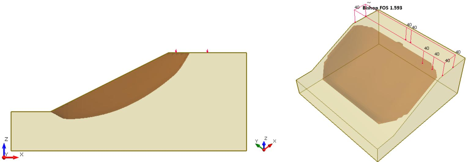
**Figure 21.4.1 – Slide3 Solution Using the Bishop Method**
