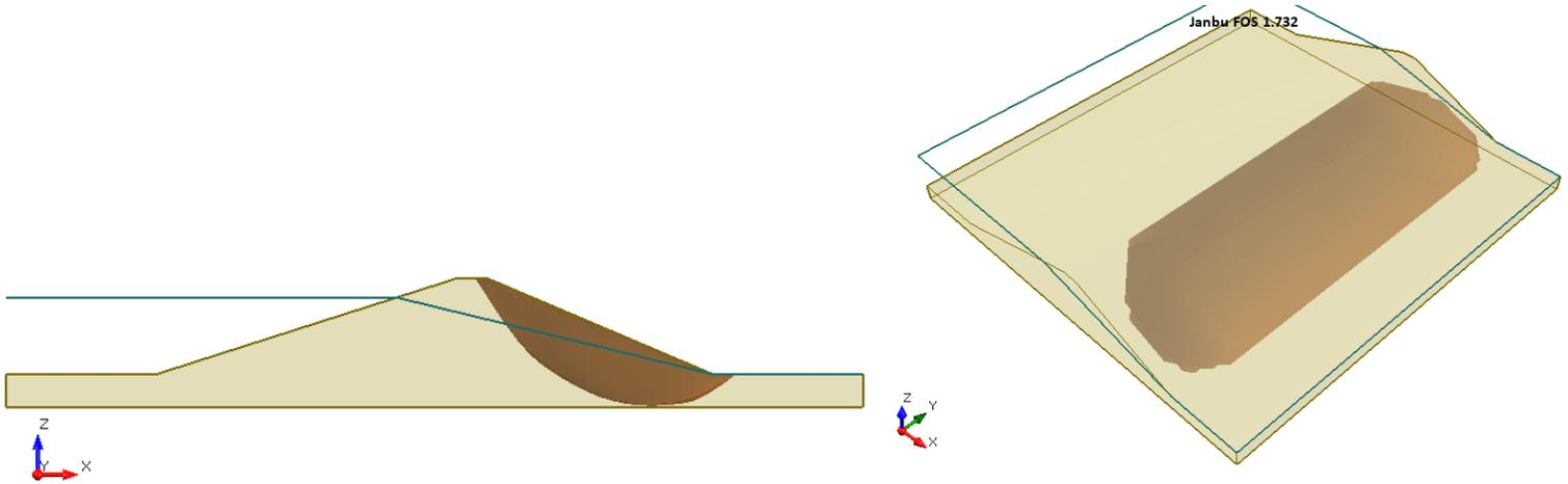
Figure 13.4.5 – Slide3 Solution Using the Janbu Method
