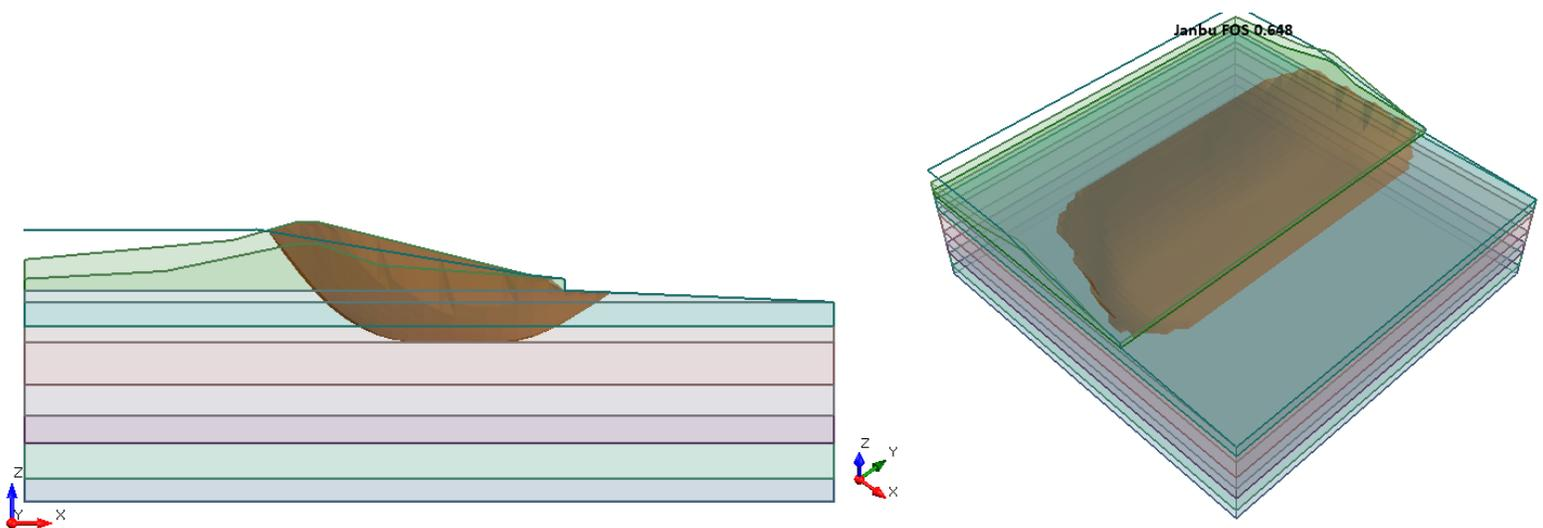
Figure 43.4.5 – Slide3 Solution Using the Janbu Method
