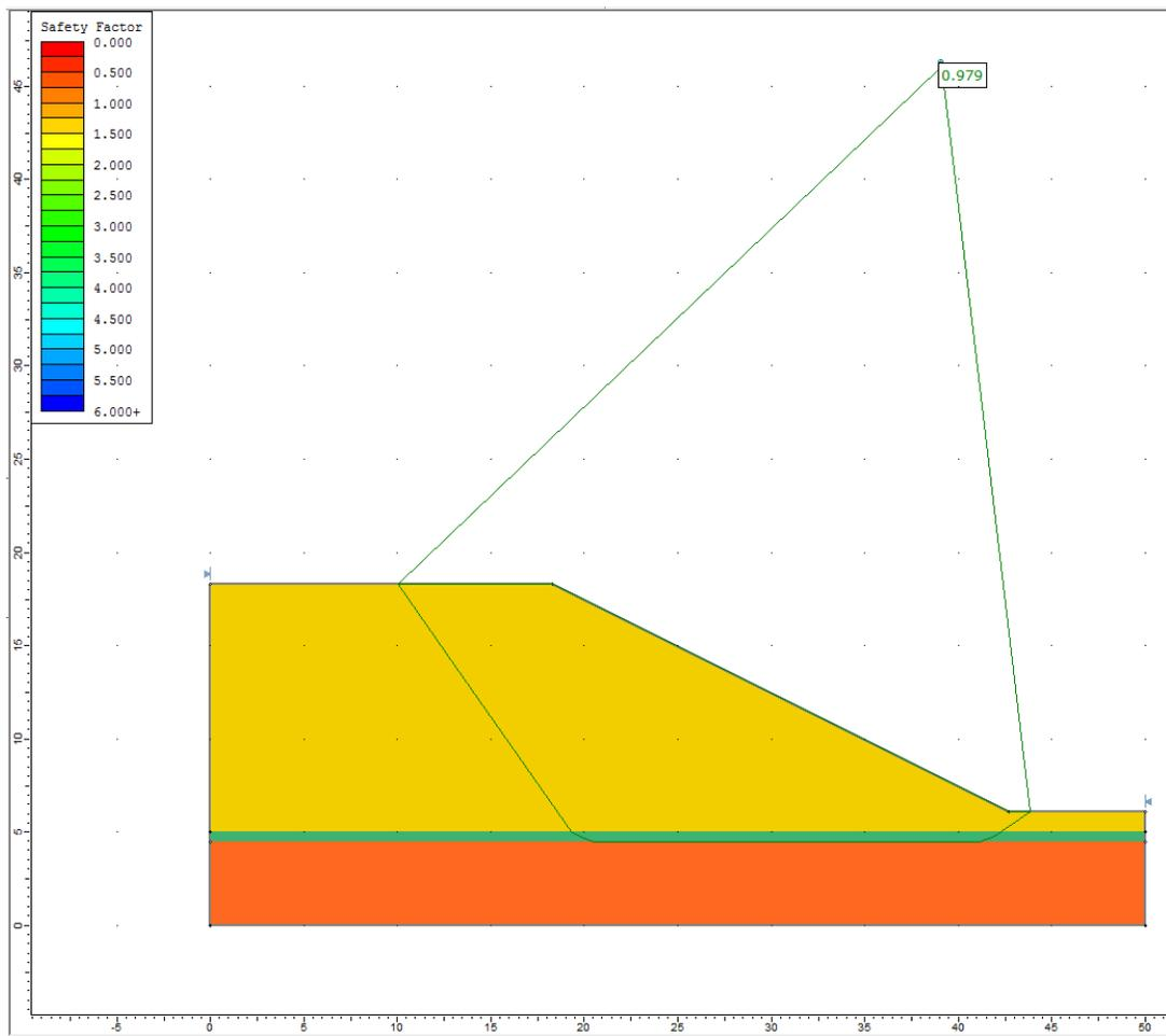
**Figure 15.4.4 – Slide Solution Using the GLE Method**
