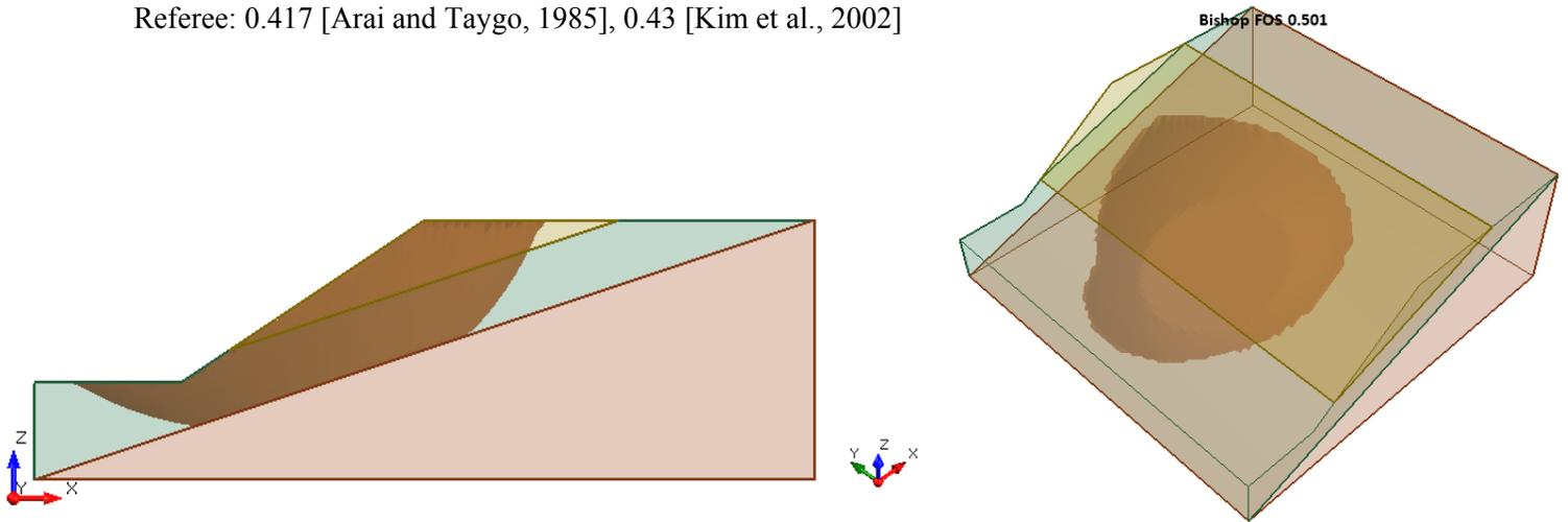
**Figure 10.4.1 – Slide3 Solution Using the Bishop Method**
