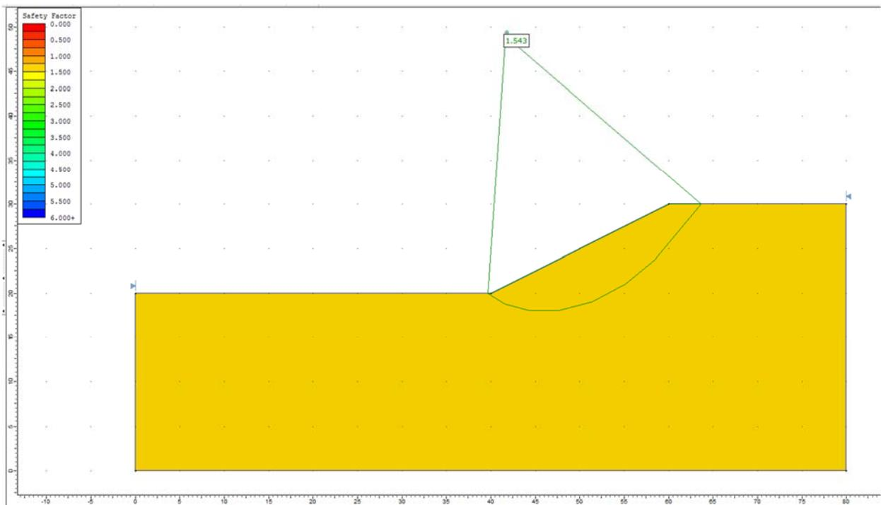
**Figure 19.4.6 – Slide Solution Using the Janbu Method**
