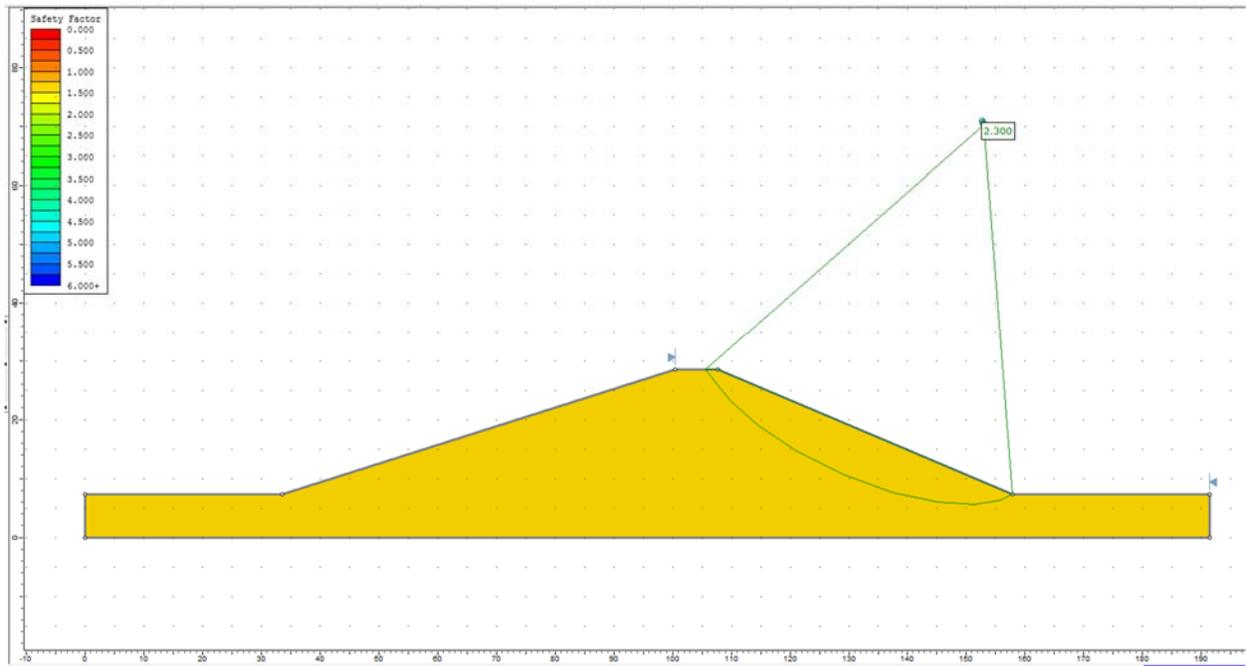
**Figure 12.4.6 – Slide Solution Using the Janbu Method**
