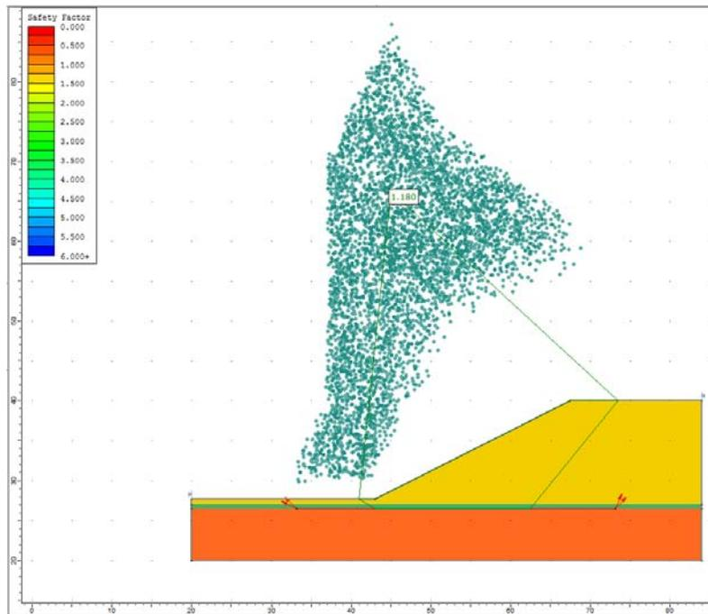
**Figure 7.4.2 – Slide Solution Using the Janbu Method**
