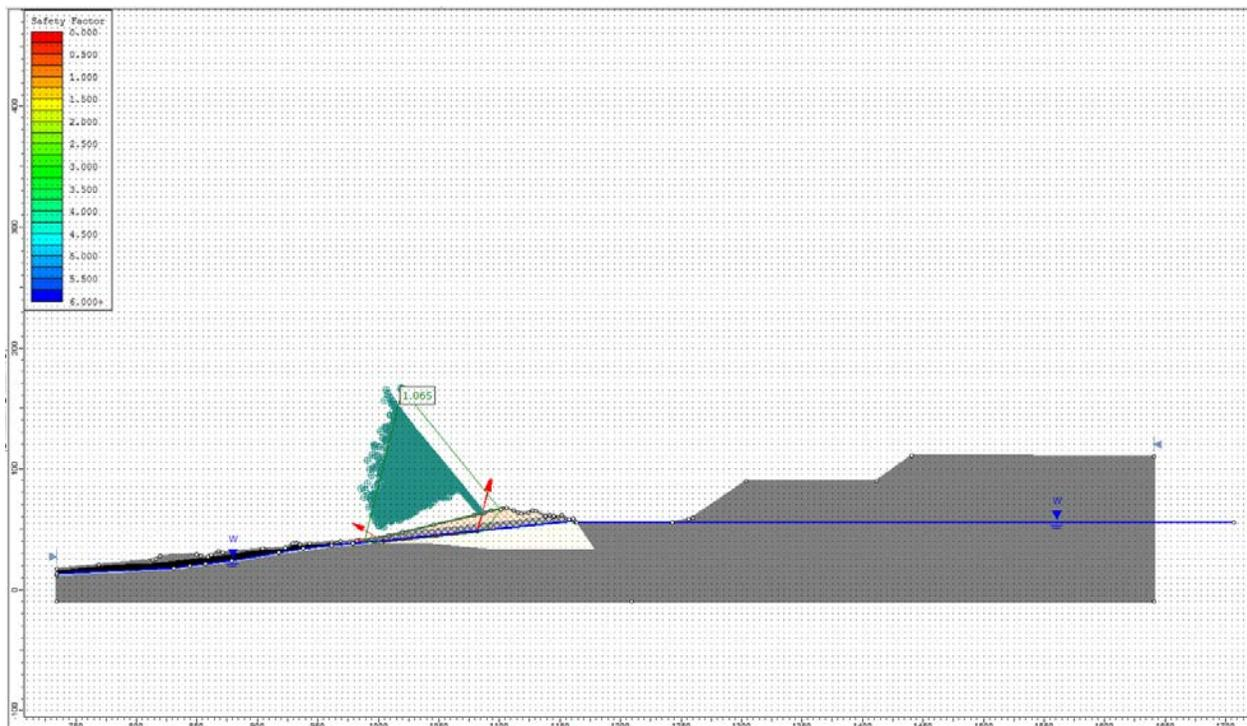
Figure 39.4.4 – Slide Solution Using the GLE Method
