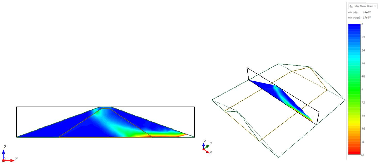
Figure 32.4.8 – RS3 Maximum Shear Strain
