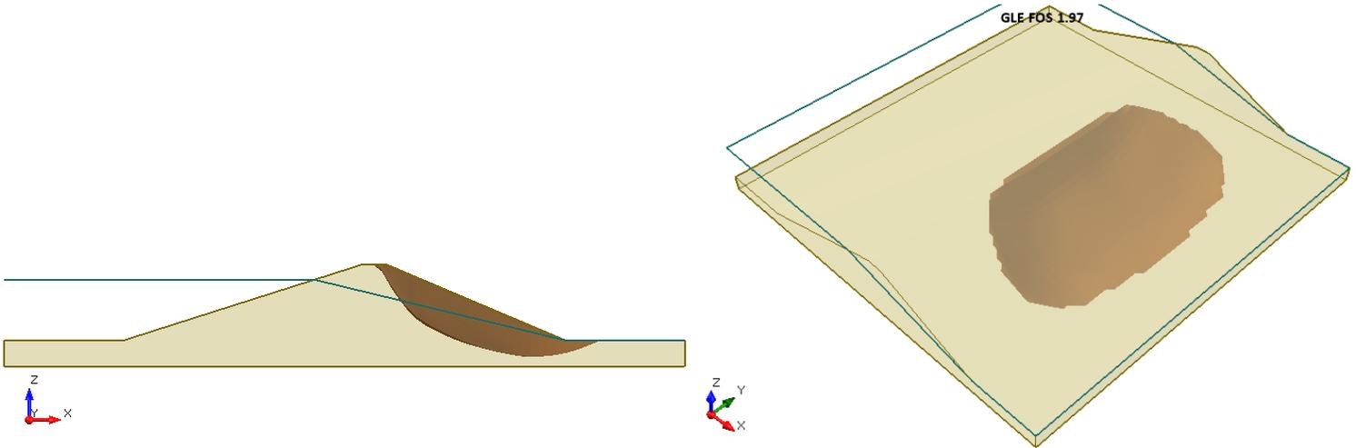
**Figure 13.4.3 – Slide3 Solution Using the GLE Method**
