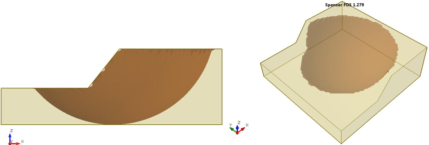
**Figure 36.4.5 – Slide3 Solution Using the Spencer Method**
