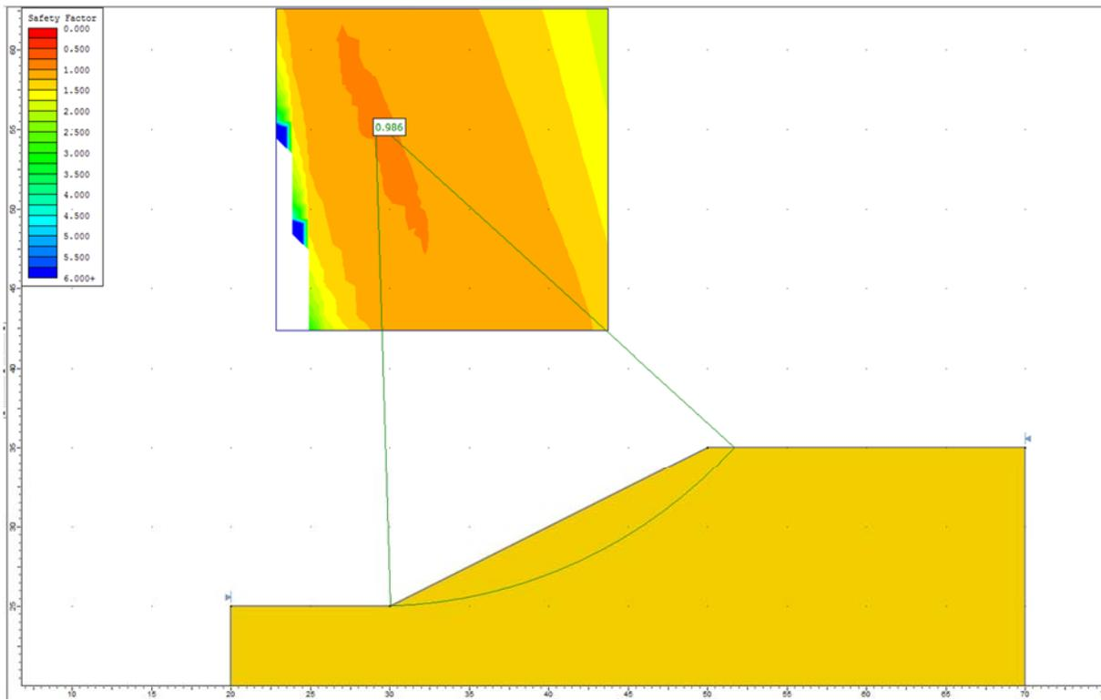
Figure 1.2.6 – Slide Solution Using the GLE Method
