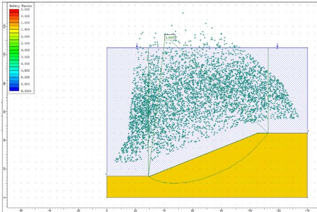
**Figure 28.4.2 – Slide Solution Using the Bishop Method**
