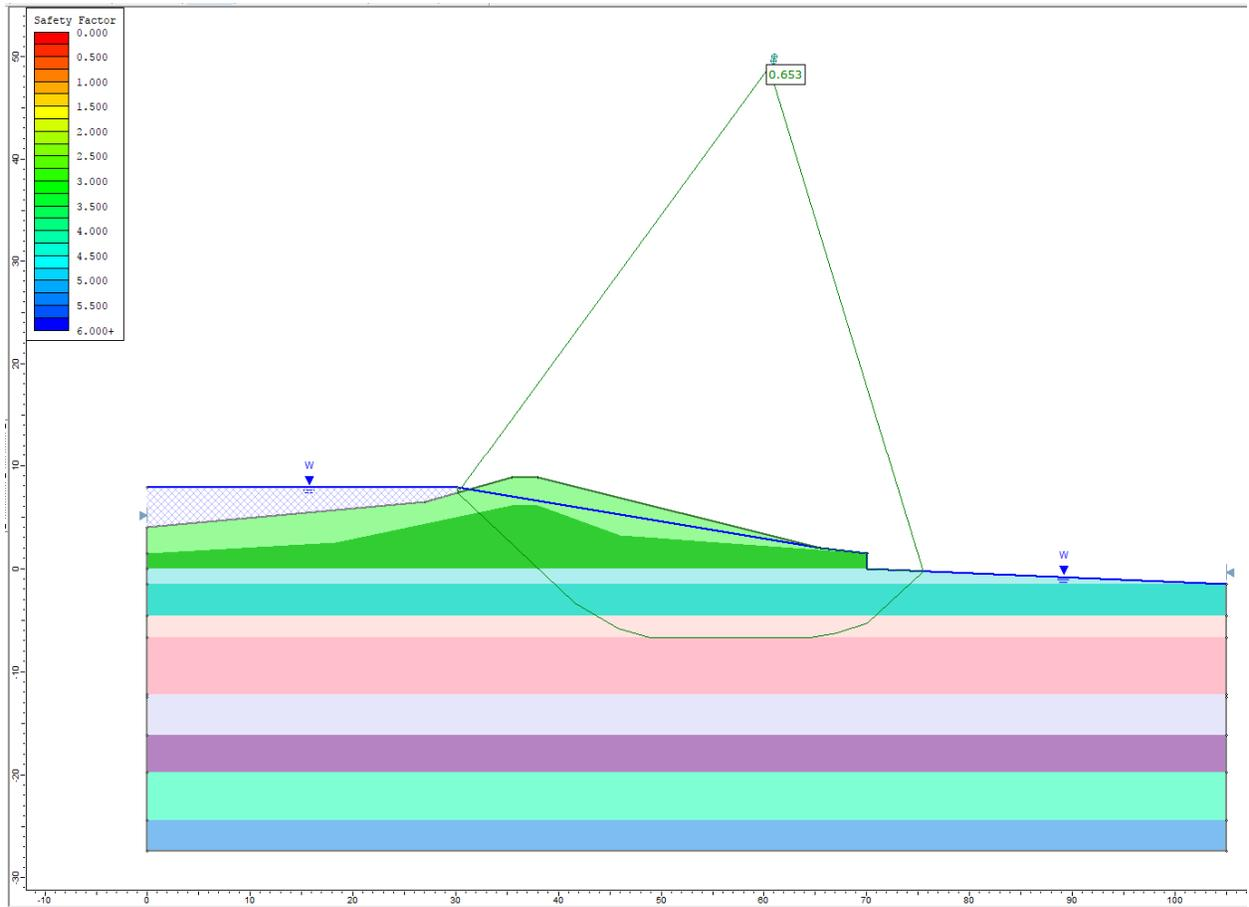
Figure 43.4.2 – Slide Solution Using the Bishop Method
