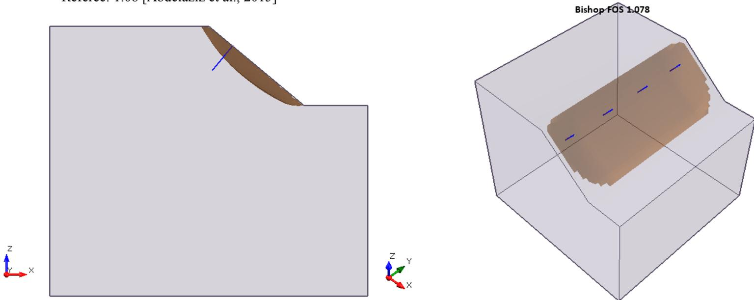
**Figure 22.4.1 – Slide3 Solution Using the Bishop Method**
