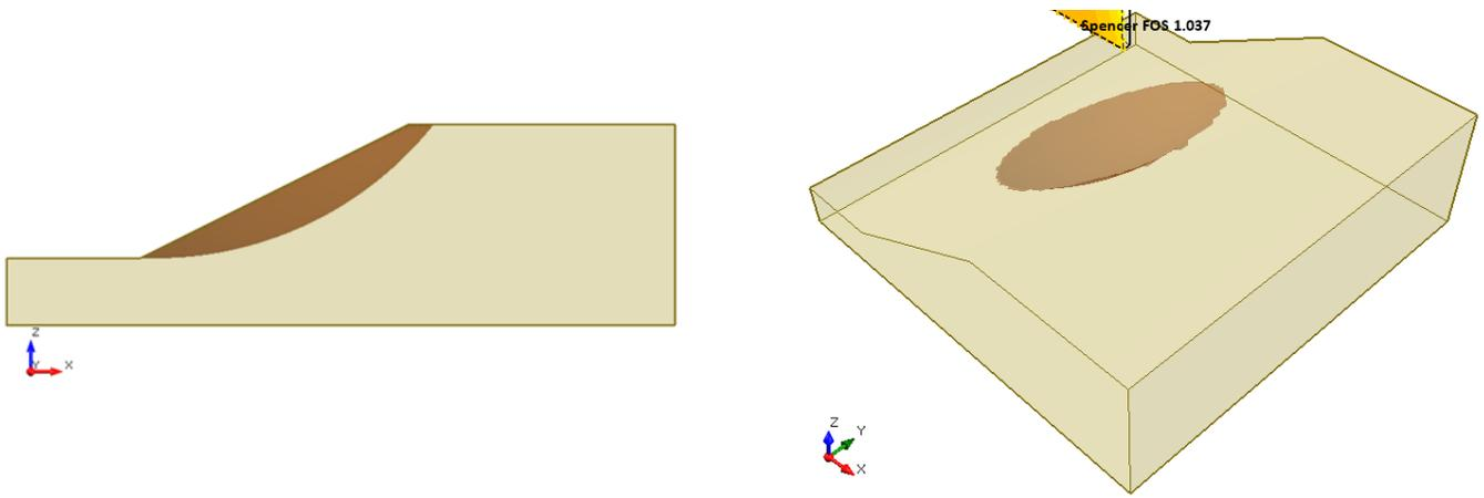
**Figure 1.4.3 – Slide3 Solution Using the Spencer Method**
