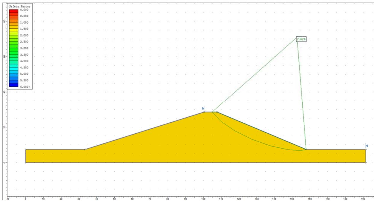
**Figure 12.4.8 – Slide Solution Using the Spencer Method**
