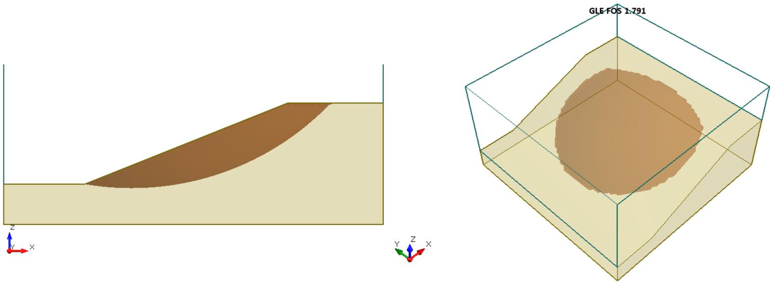
**Figure 27.4.3 – Slide3 Solution Using the GLE Method**
