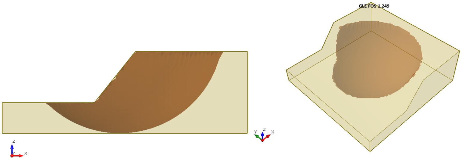
**Figure 34.4.3 – Slide3 Solution Using the GLE Method**
