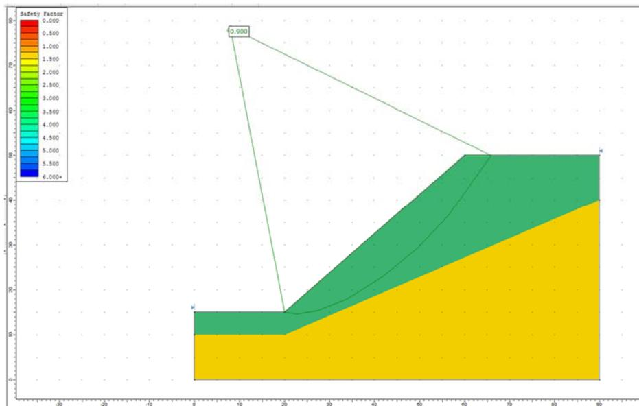
**Figure 17.4.2 – Slide Solution Using the Bishop Method**
