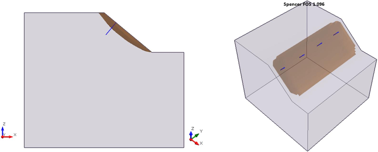
**Figure 22.4.7 – Slide3 Solution Using the Spencer Method**
